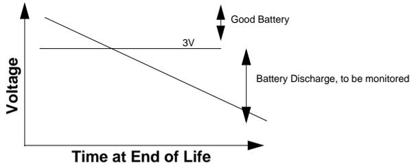
Figure 4. Typical Lithium Voltage vs. Time, Using Constant Current Drain
