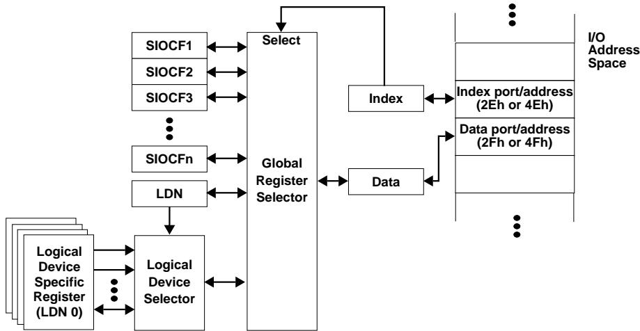
Figure 1. SuperI/O Configuration Registers Access Mechanism
