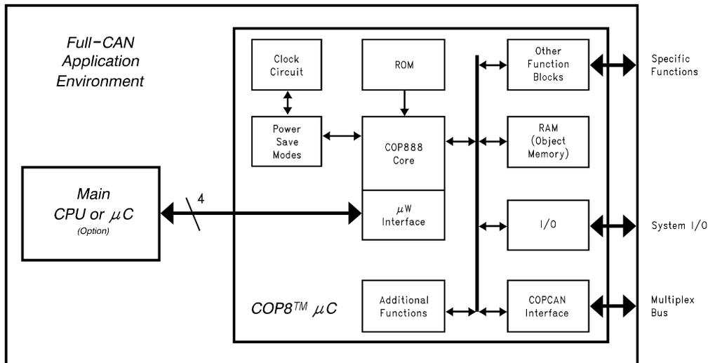
FIGURE 3. COP8-Based Full-CAN Interface
