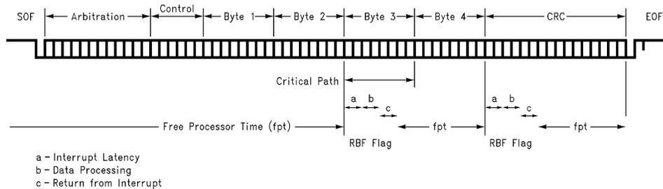
FIGURE 2. Message Processing with the COPCAN Interface
