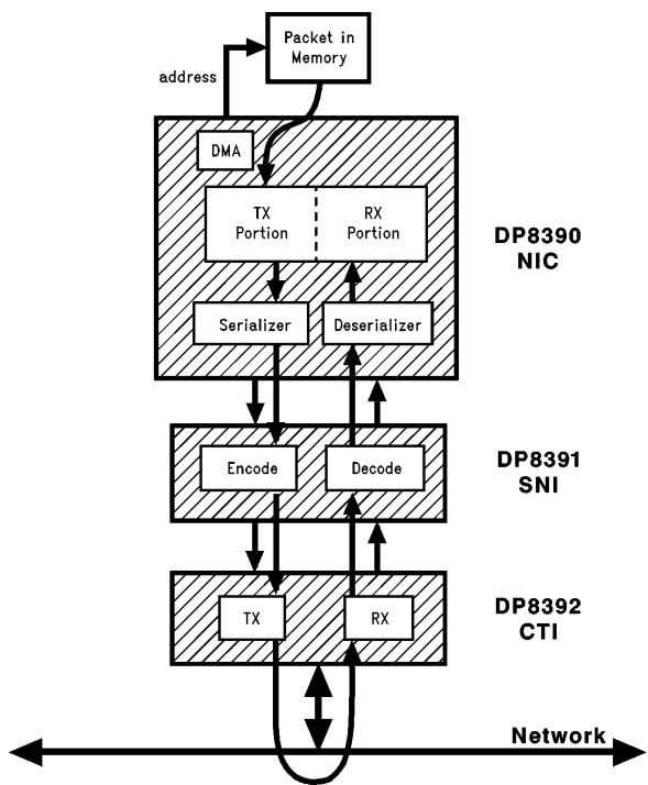
FIGURE 3. Loopback Mode 3: To the Coax
