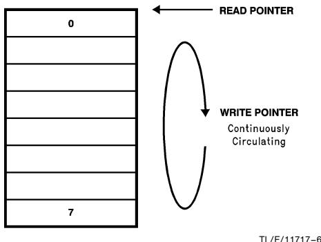
FIGURE 5. Continuously Circulating FIFO
