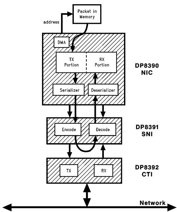
FIGURE 2. Loopback Mode 2: Through the SNI
