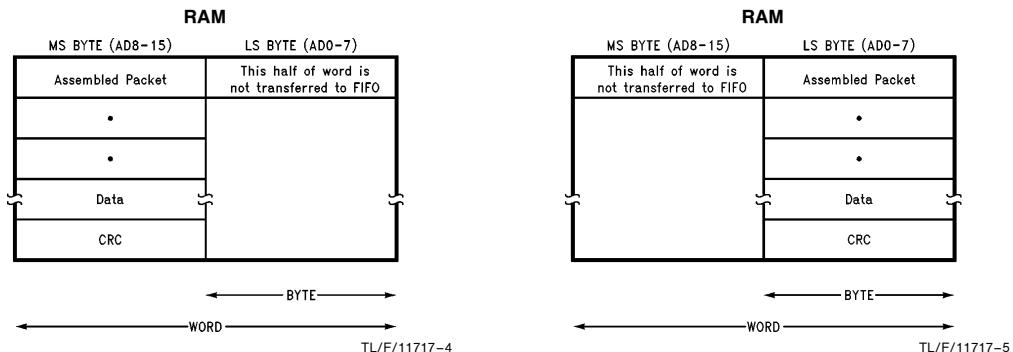
FIGURE 4. Packet Assembly for Loopback Work Wide Transfers
