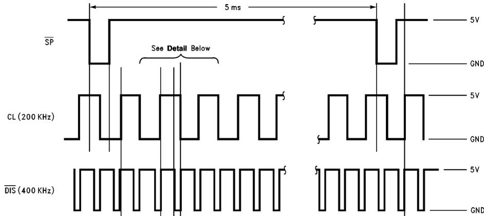
**CIS Scanner Output Signal**
