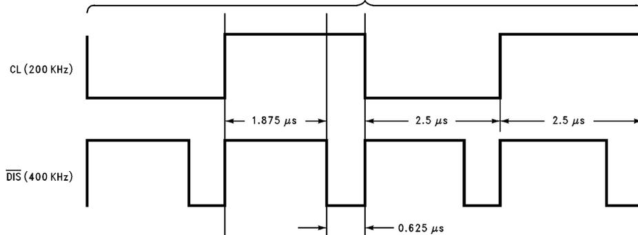
**FIGURE 3. Timing for CIS Scanner Signals Produced by the NS32FX200**
