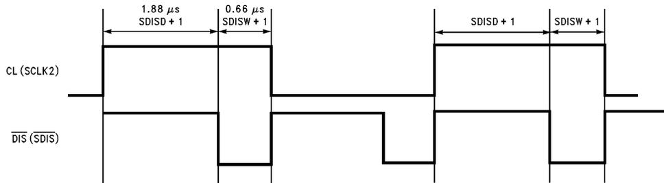
FIGURE 4.  $\overline{SDIS}$  Signal
