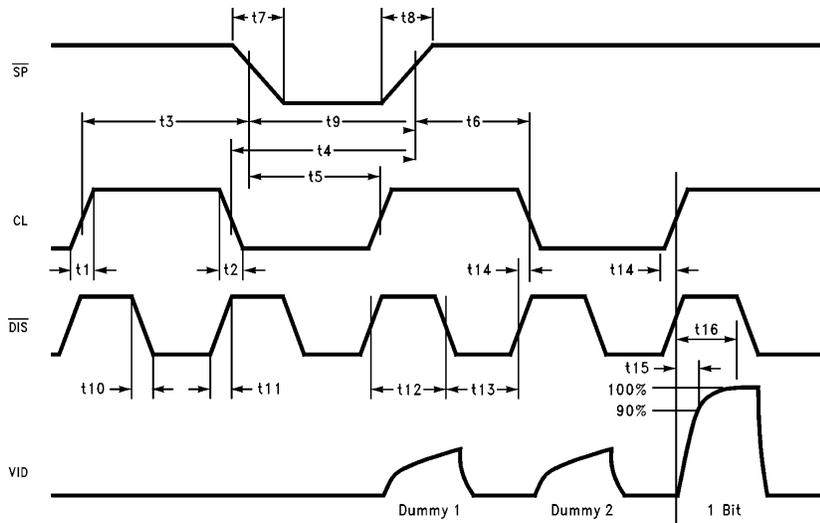
FIGURE 2. Scanner Signal Timing Requirements
