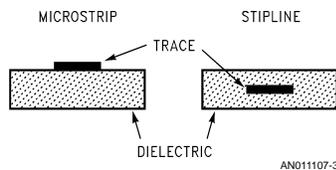
FIGURE 3. PCB Track Cross Section
