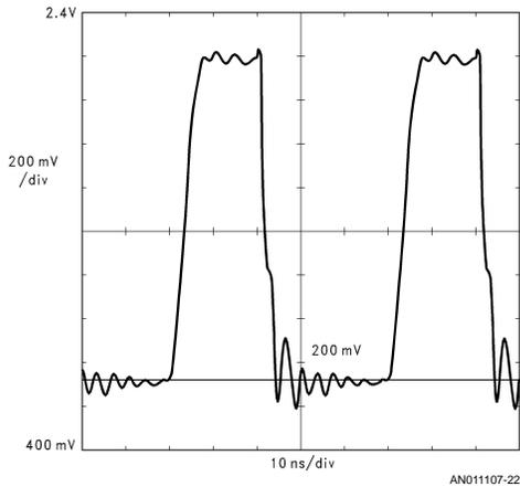
**FIGURE 22. Backplane Probed at Driver = Slot 5, 12 pF Loads in Slots 0 and 6**
