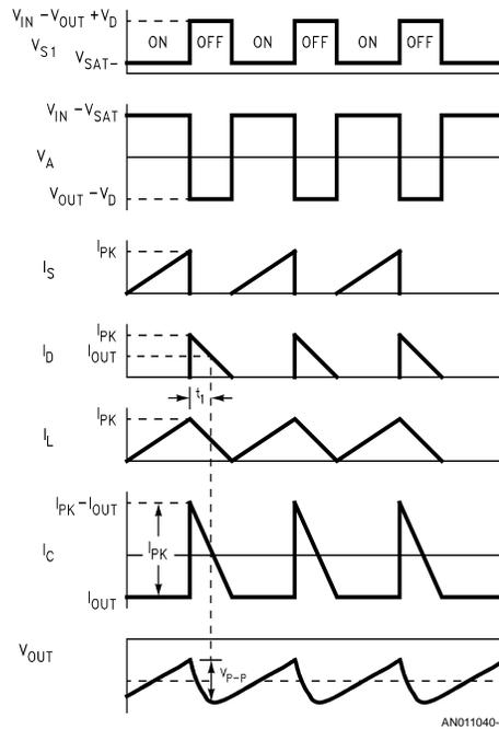
FIGURE 6. Voltage Inverter Waveforms
