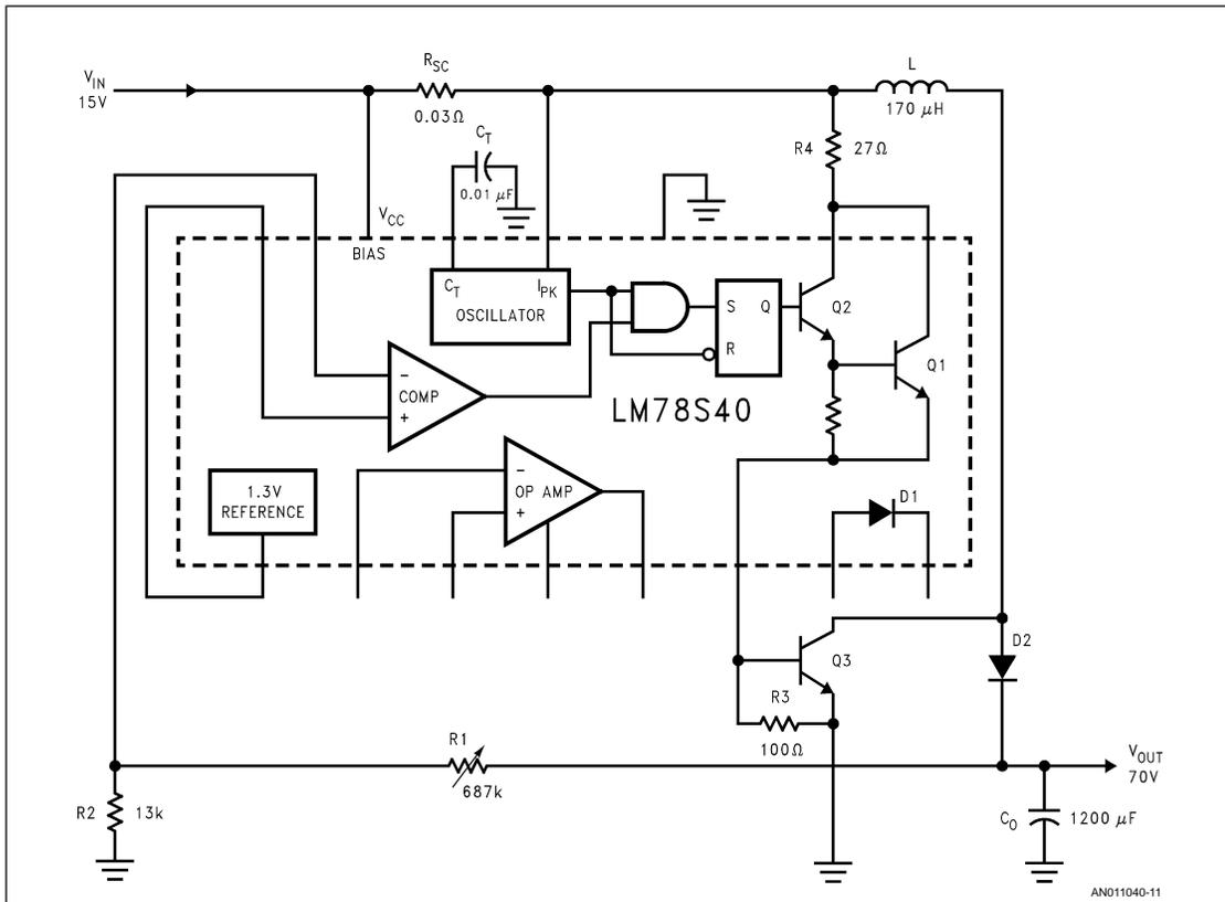
FIGURE 8. Switching Regulator with 15V Input, 70V Output
