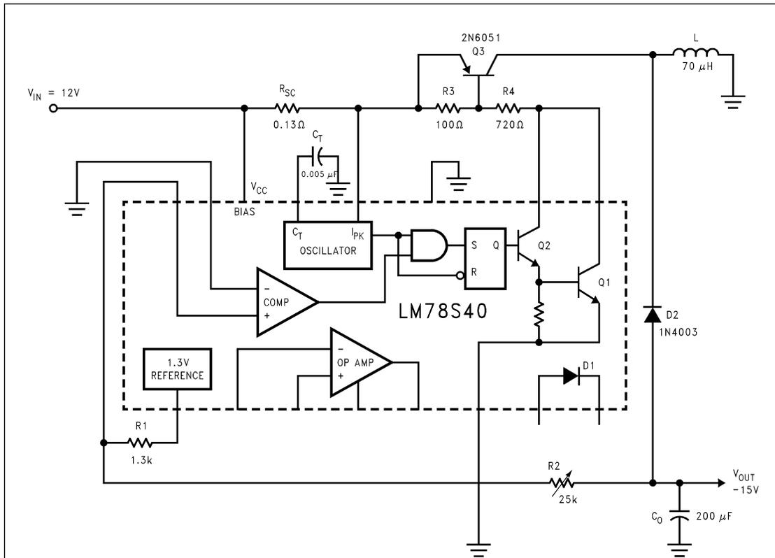
FIGURE 11. Inverting Regulator
