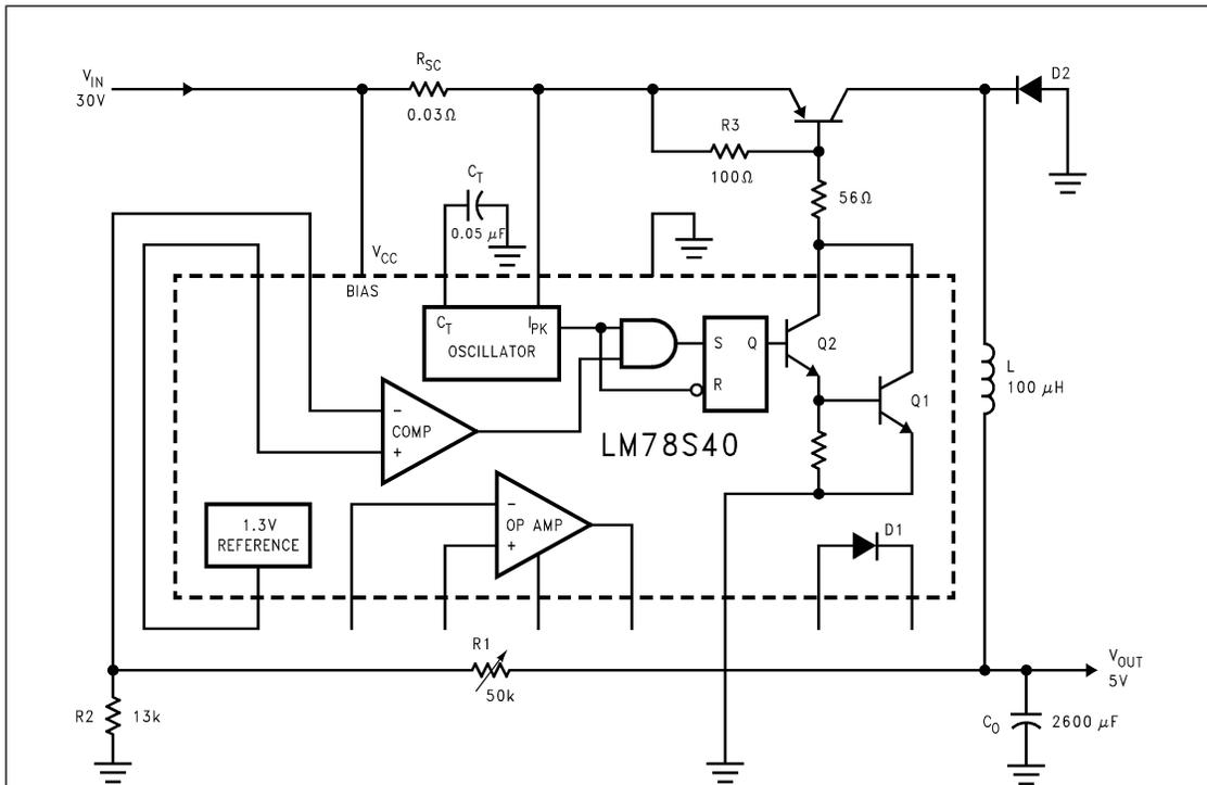
FIGURE 10. Modified Step-Down Regulator with 5A, 5V Output
