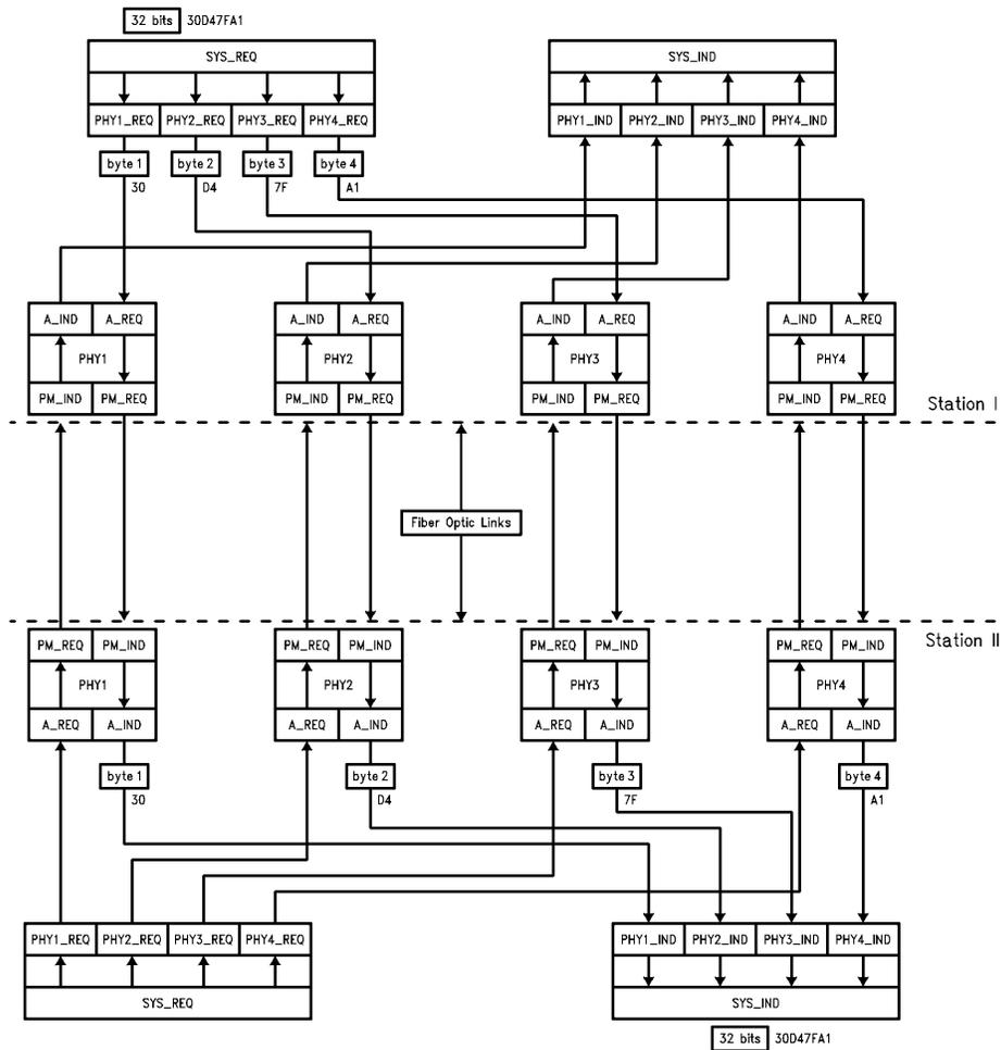
FIGURE 3. System Using Four PHY Layers in Parallel
