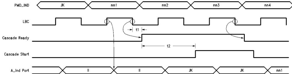
**FIGURE 5a. First PLAYER device to receive a JK symbol in a large skew scenario. The CS signal goes high about 60 ns after the CR line is asserted. This indicates that some of the channels received JK symbols more than one LBC period after the channel shown.**
