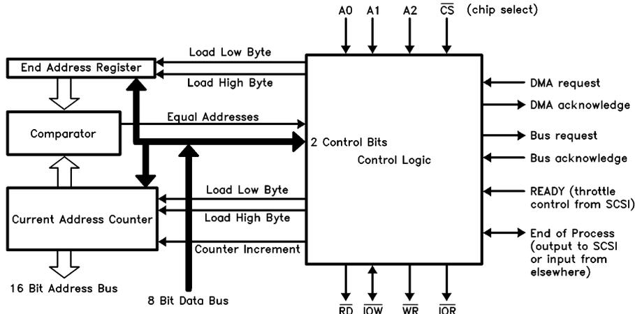
FIGURE 3. Block Diagram of DMA Controller
