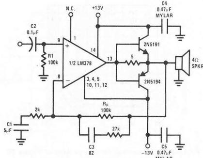
FIGURE 17. 12 Watt Low-Distortion Power Amplifier
