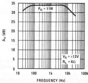
FIGURE 18. Response for Amplifier of Figure 17
