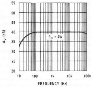
FIGURE 21. Frequency Response, Bridge Amp of Figure 20
