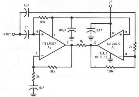
FIGURE 20. 4-Watt Bridge Amplifier
