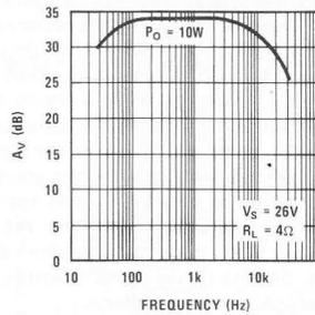
FIGURE 16. 10 Watt Boosted Amplifier, Frequency Response
