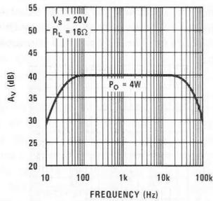
FIGURE 25. Frequency Response, Bridge Amp of Figure 23
