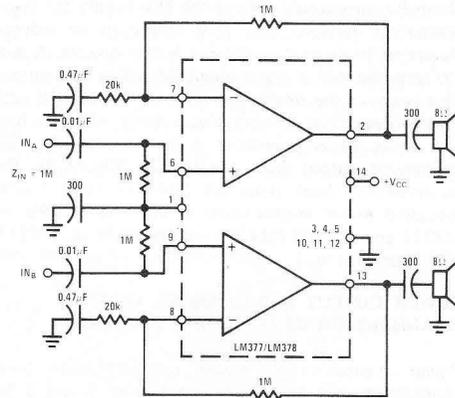
FIGURE 6. Non-Inverting Stereo Amplifier
