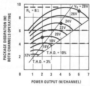
FIGURE A-1. Power Dissipation vs Power Output
