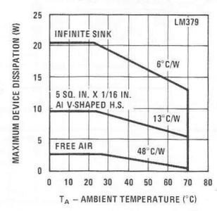
FIGURE A-4. Maximum Dissipation vs Ambient Temperature
