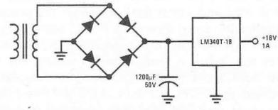
FIGURE 33. Alternate Power Supply for Ambience Circuit
