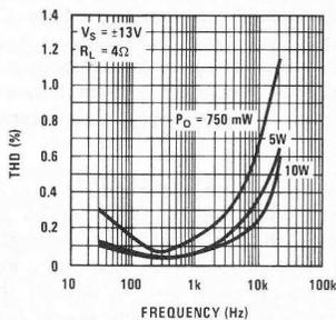
FIGURE 19. Distortion for Amplifier of Figure 17
