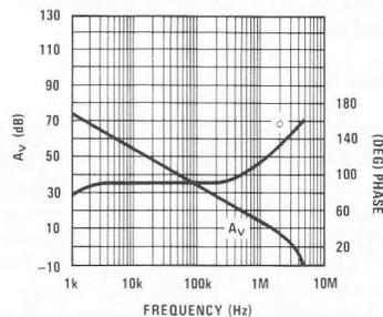
FIGURE 12. Open Loop Bode Plot (Approximately Worst Case)
