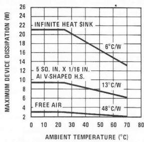
FIGURE 10. LM379 Power Derating
