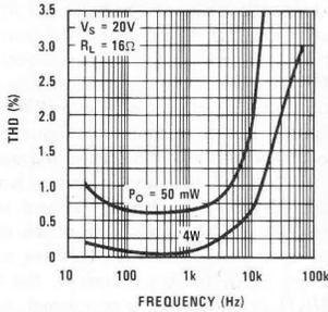
FIGURE 24. Distortion for Bridge Amp of Figure 23
