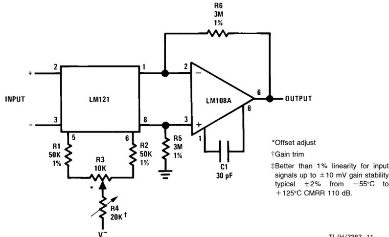
FIGURE 11. Gain of 1000 Instrumentation Amplifier
