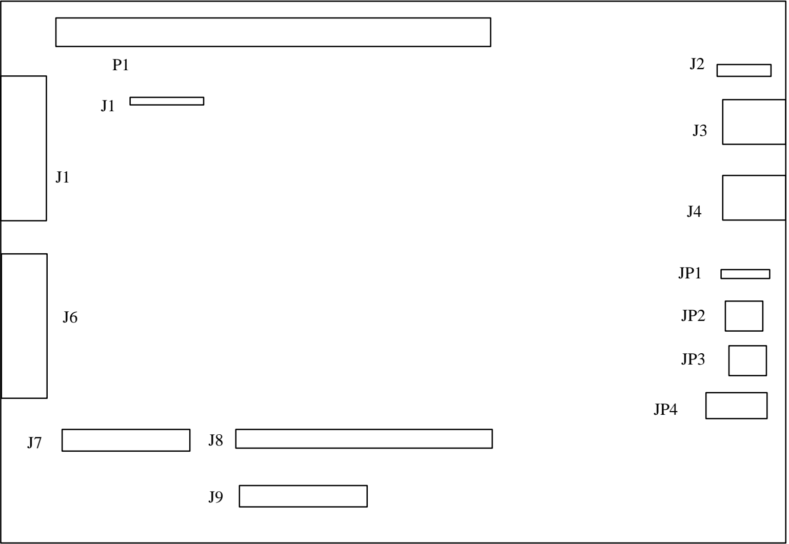
Figure 1.3. Jumper and connector placement.
