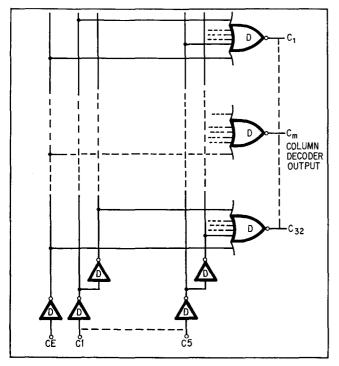
6. Column decoder. Depletion-load inverters drive depletion-mode NOR gates. Decoder uses 32 six-input NOR gates. Selected column is driven by one gate (the only one that provides an output at  $V_{\rm DD}$ ). D indicates circuits with depletion-mode devices.
