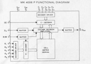
• First 1024-bit RAM in a 16-pin package
