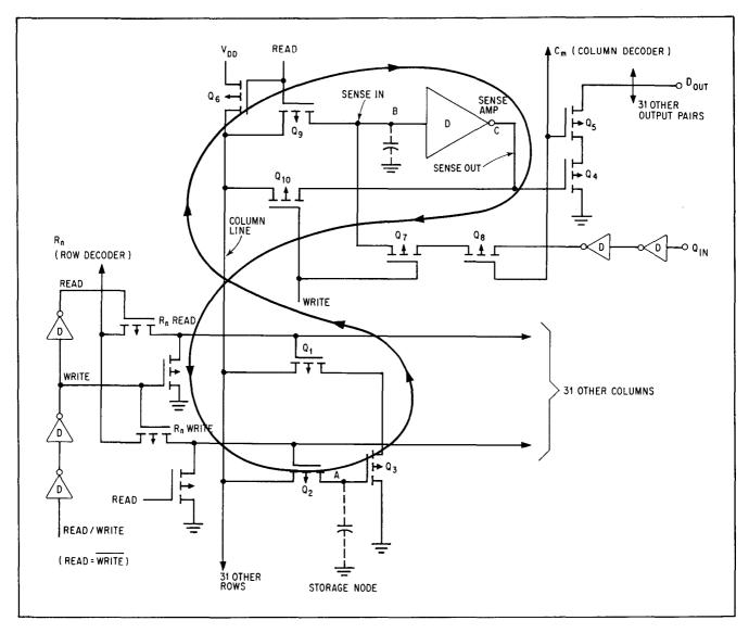
**5. Single cell.** Information entered at D<sub>in</sub> is stored at node A. In refresh mode, data at A travels in figure-eight path from A to column line to node B, through sense amplifier, and back to the column line to refresh A through Q<sub>2</sub>. Circuits with depletion-mode devices are designated D.
