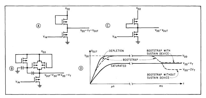
3. Widest swing. Depletion-mode inverter circuit, C, attains  $V_{\rm DD}$  as most negative output level, while bootstrap circuit, B, and enhancement-mode inverter, A, do not offer as wide a range on a dc basis. Depletion-mode circuit also has best speed-power product.
