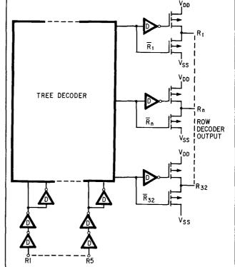
7. Row decoder. Tree decoder drives 32 depletionload inverters and push-pull buffers. Selected row is driven to  $V_{\rm DD}$ — $V_{\rm T}'$ . D indicates circuits with depletion-mode devices.
