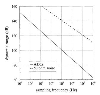
**Figure 15–2.** Monolithic ADC performance 1993.
