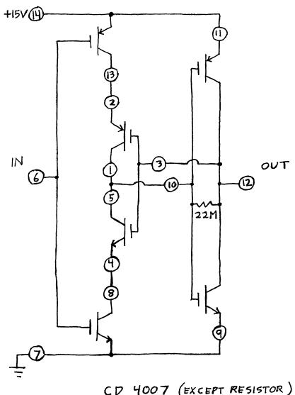
Figure 20–8. "No current" Schmitt trigger.
