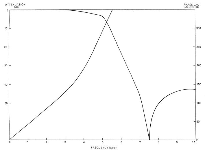
elliptic-like, however, the shunt legs can be easily checked. The voltage across each leg should drop to zero at the frequency of the zero it creates. Once these are working properly, there isn't much left to check.
