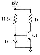
**Q5.** A constant-current lo is fed into the diode connected-transistor Q1 shown in Figure 13–5. What happens to the output voltage Vo as temperature is increased?
