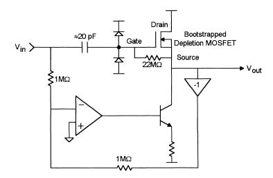
Figure 7–16. A variation on the two-path impedance converter.
