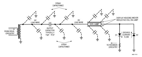
to assume 1% efficiency loss per inch of high voltage lead. Any PC board ground or power planes should be relieved by at least  $\frac{1}{2}$  in the high voltage area. This not only prevents losses, but eliminates arcing paths.
