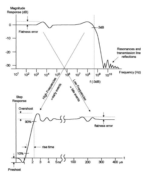
(Kamath 1974). Thus the step response contains information about a very wide band of frequencies, when observed over a long enough time period. For example, looking at the first ten nanoseconds (ns) of the step conveys frequency domain information from the upper bandwidth of the instrument down to approximately 1/(10ns) or 100MHz.
