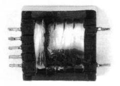
Figure 11-27. Poor loop compensation caused this transformer failure. Arc occurred in high voltage secondary (lower right). Resultant shorted turns caused overheating.
