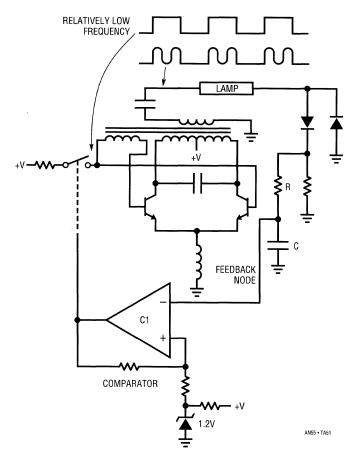
node. The scheme worked, but had poor line rejection, due to the varying waveform vs. supply seen by the RC averaging pair. Also, the "burst" modulation forces the loop to constantly re-start the bulb at the burst rate, wasting energy. Finally, bulb power is delivered by a high crest factor waveform, causing inefficient current-to-light conversion in the bulb.
