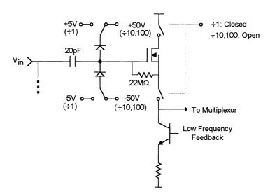
Figure 7–20. Moving the ÷1 switch from the high-impedance input side to the low-impedance output side of the FET.
