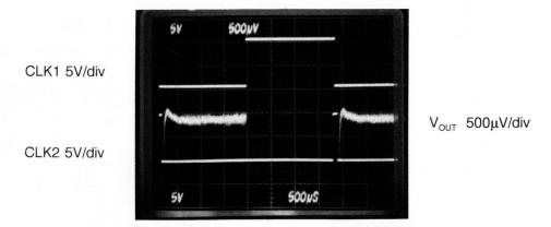
Figure 15–8. Erased positive overdrive ( $V_1 = 5V$ ,  $V_2 = 7V$ ).
