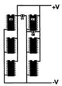
The decoupling path of IC2 is ideal.
