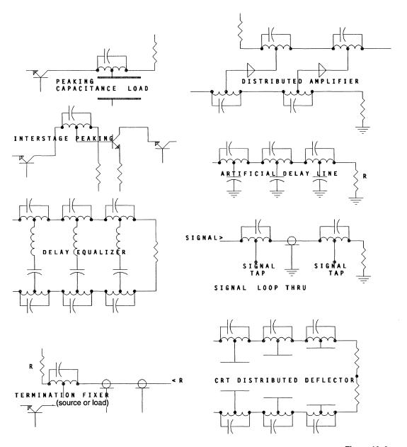
Figure 10–2. The Versatile T-coil.
