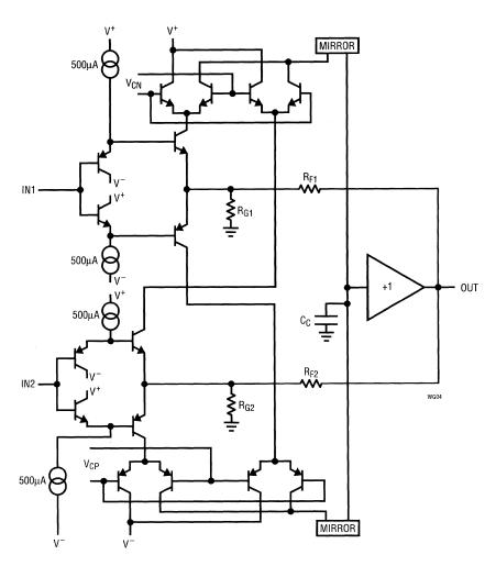
current levels were set based on previous current feedback amplifiers already designed. It was time to proceed to the control section.
