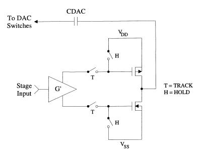
Figure 15–10. CS5016 sampling switch detail.
