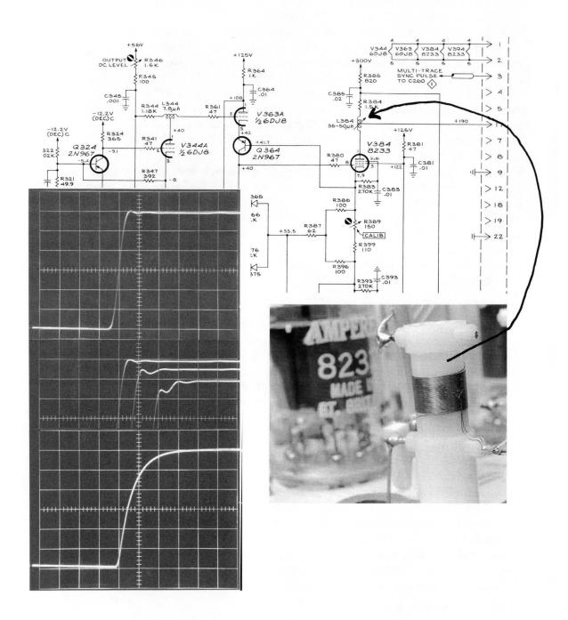
**Figure 10–5.** Step Response Waveforms 3A6 T-coil Peaking.
