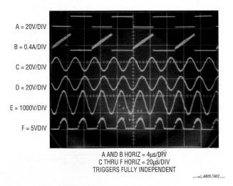
Figure 11–19. Waveforms for the cold cathode fluorescent lamp power supply. Note independent triggering on Traces A and B, and C through F.
