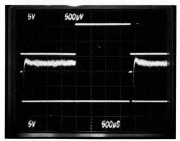
Figure 15–7. Erased negative overdrive ( $V_1 = 5V$ ,  $V_2 = 3V$ ).
