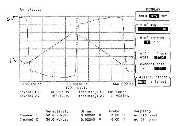
much higher frequency. I couldn't make the breadboard do it. I guessed that the circuit liked the extra stray capacitance of the breadboard. This seemed consistent with the breadboard version refusing to go high. I estimated the stray capacitance on the output, experimentally found the maximum the circuit would tolerate, and picked a value in between. Adding this to the hybrids fixed them all.
