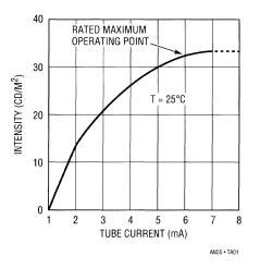
Figure 11–13. Emissivity for a typical 6mA lamp; curve flattens badly above 6mA.
