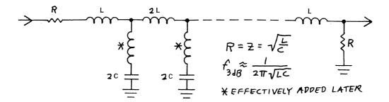
Figure 20–4. Passive low-pass ladder.
