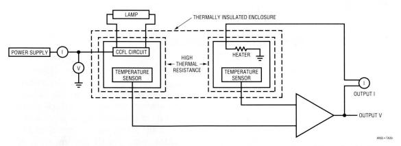
mentation considerations.<sup>5</sup> It is significant that the total uncertainty between electrical and both calorimetric efficiency determinations was 3.3%. The two thermal approaches differed by about 2%. Figure 11–A9 shows the calorimeter and its electronic instrumentation. Descriptions of this instrumentation and thermal measurements can be found in the References section following the main text.
