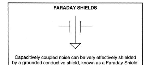
But it must be grounded or it increases the problem. For this reason coil and quartz crystal cans should always be grounded.
