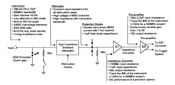
signals) are not allowed! The designer's only defense is to keep the physical dimensions of the circuit very small. To obtain the 1GHz bandwidth we must use microwave components. Microwave transistors and diodes are typically very delicate, yet the front-end has to withstand ±400V excursions and high-voltage electrostatic discharges. Perhaps the most difficult requirement is high gain flatness from DC to a significant fraction of full bandwidth.
