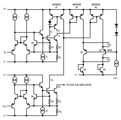
Figure 8–8. The control circuit.
