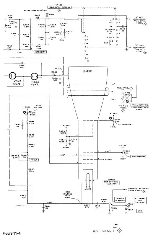
CRT supply used in Tektronix 547. C808 resonates with transformer, creating sine wave drive. (Figure reproduced with permission of Tektronix, Inc.)
