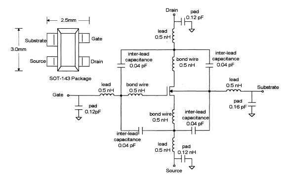
**Figure 7–6.**A MOSFET with SOT-143 surface-mount package parasitics. The model includes the effects of mounting on a 1.6mm (0.063") thick, six-layer epoxy glass circuit board with a ground plane on the fourth layer from the component side of the board.
