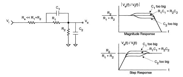
shows one way in which these and the many additional requirements of Figure 7–1 can be met (Rush 1986).
