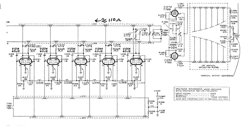
**Figure 10–8.**Tektronix 585 Distributed Amplifier Vertical Output.
