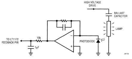
Figure 11–C9. Optically sensed feedback eliminates feedback irregularities, but introduces other problems.
