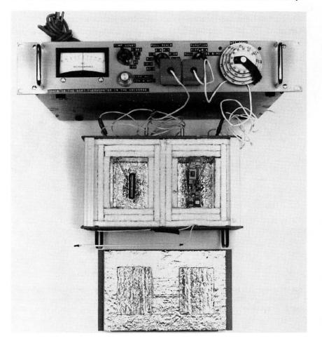
Figure 11-A9. The calorimeter (center) and its instrumentation (top). Calorimeter's high degree of thermal symmetry combined with sensitive servo instrumentation produces accurate efficiency measurements. Lower portion of photo is calorimeter's top cover.
