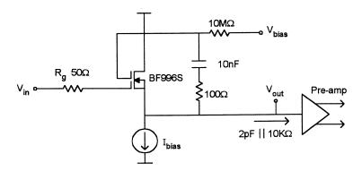
it does not boost the gain at DC and low frequencies. The response therefore is not very flat, but we can fix it later. From 1kHz to 100MHz the gain is greater than 0.985 and therefore highly independent of temperature. The 1% settling time is very good at 1.0ns.
