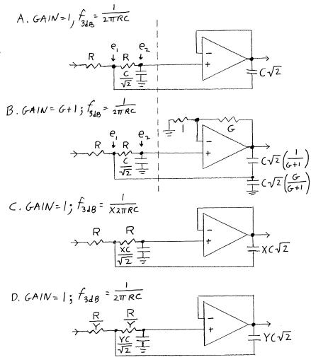
out of the design in about the same time it previously took to make one adjustment and check it. Then I reduced the capacitors by factors of ten, making sure no side problems cropped up. This works for high-frequency filters, too. Get the circuit working correctly at a frequency where the op amps are nearly ideal, then start reducing the capacitors and watch the effects of finite gain-bandwidth (and stray capacitance) show up!
