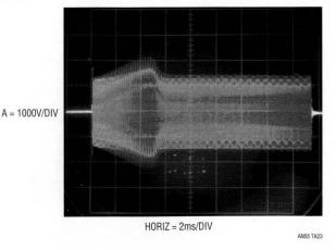
the improvements, more margin is possible if display losses can be controlled. Figures 11–26–11–29 were taken with an exceptionally lossy display. The metal enclosure was very close to the foil wrapped lamps, causing large losses with subsequent high turn-on and running voltages. If the display is selected for lower losses, performance can be greatly improved.
