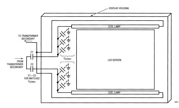
Figure 11–23. Loss paths for a "best case" dual lamp display. Symmetry promotes balanced illumination.
