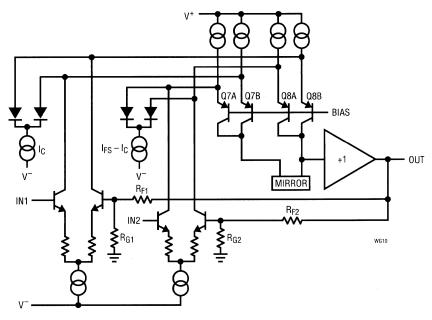
Figure 8–10. Voltage feedback with cascode steering.
