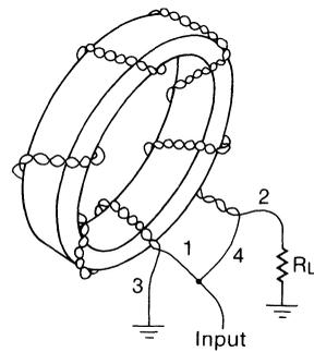
Figure 24. Transmission Line Transformer
