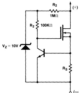
Figure 17. Two-Terminal Current Regulator
