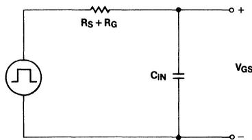
Figure 9. Simple RC Model
