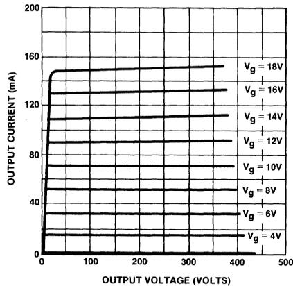
Figure 14. Output Characteristics of Figure 13
