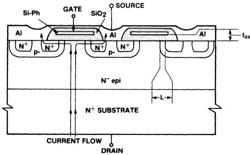
Figure 2. Vertical DMOS Structure
