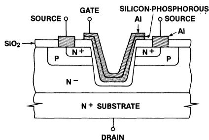
Figure 1. V-Groove MOSFET
