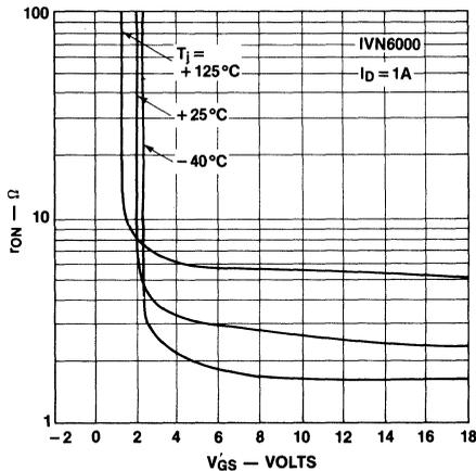
Figure 28. Variation of  $r_{ON}$  with Temperature
