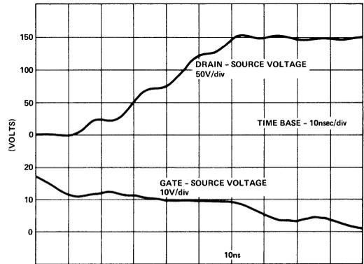
Figure 9. FET Switching Waveforms (5V/25A Load)
