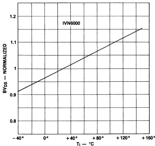
Figure 34. Breakdown Voltage Variation with Temperature
