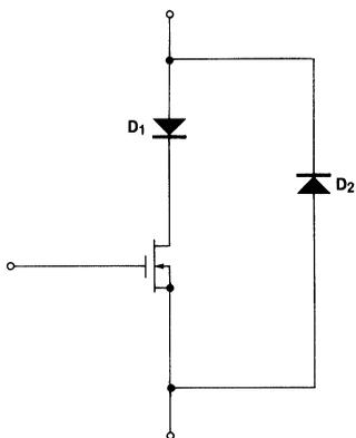
Figure 50. Method for Eliminating Reverse Conduction
