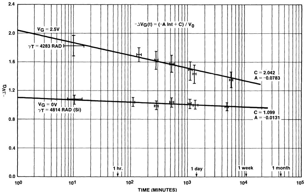
Figure 32. VMOS LINAC Annealing Curves
