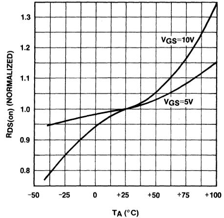
Figure 16. IVN5200  $R_{DS(on)}$  vs.  $T_A$
