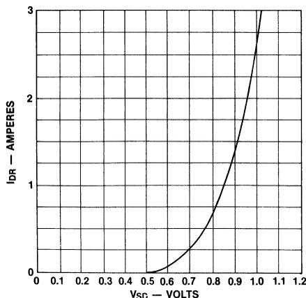
Figure 52. IVN6000 Diode Forward Voltage Characteristic
