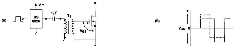
**Figure 22.** Transformer Coupled MOSFET Drive Circuit
