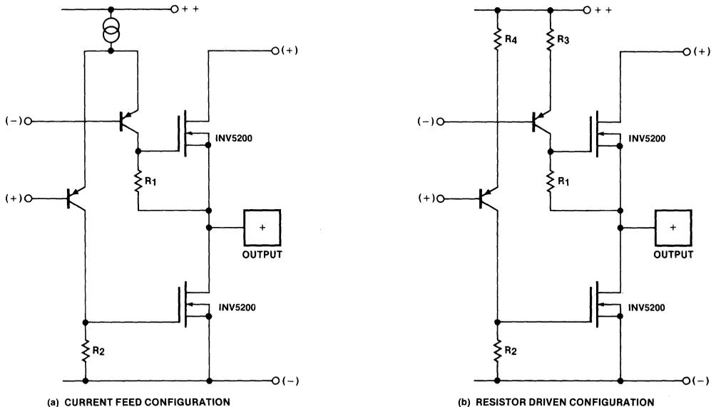
Figures 26a and b. Differential-Complementary Output Configurations
