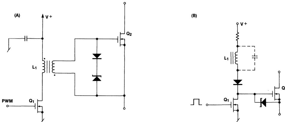
**Figure 21.** MOSFET Drive Circuits Using Stored Energy
