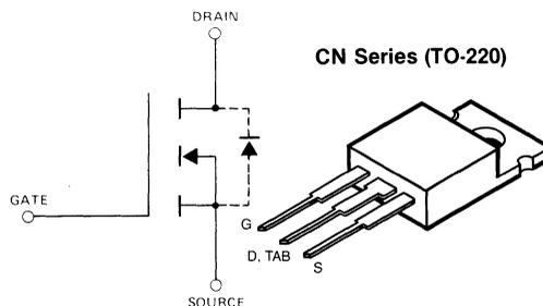
Body internally connected to source.
