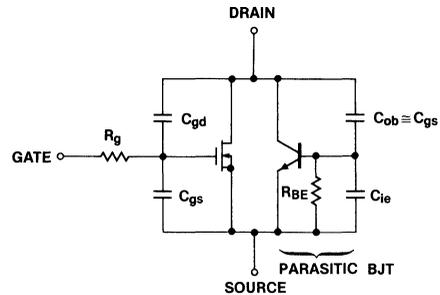
Figure 49. MOSFET Model Including Parasitic BJT
