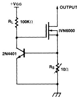
Figure 16. Current Regulator with Loop Gain
