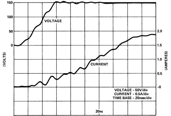
Figure 7b. Voltage/Current Waveforms Expanded, 25A Load.
