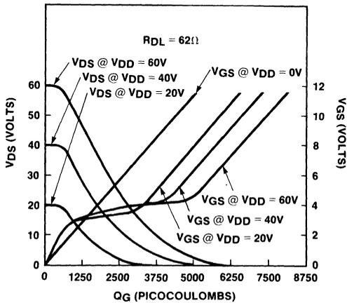
Figure 25. IVN5200 Dynamic Input Characteristics
