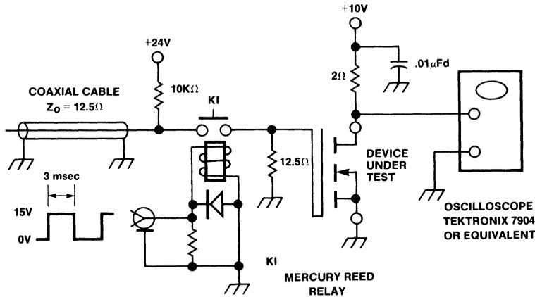
Figure 21. Switching Time Test Circuit IVN5200
