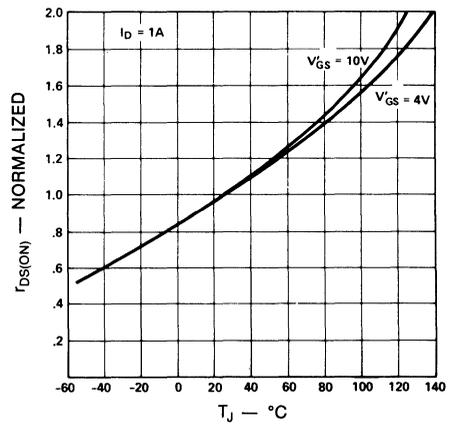
**ON RESISTANCE vs.  $V_{GS}^*$  AS A FUNCTION OF TEMPERATURE**
