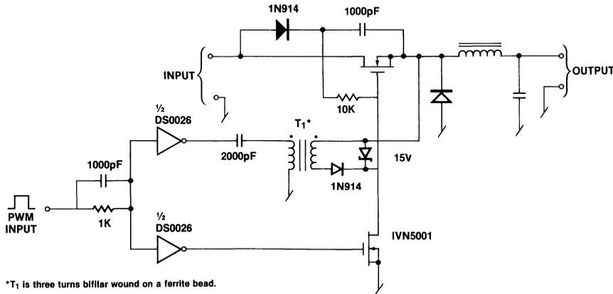
\*T<sub>1</sub> is three turns bifilar wound on a ferrite bead.
