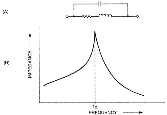
Figure 28. Inductor Self Resonance
