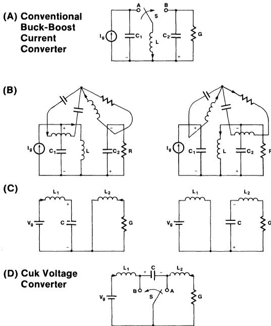
Figure 8: Duality between the Buck-Boost and the Cuk Converters
