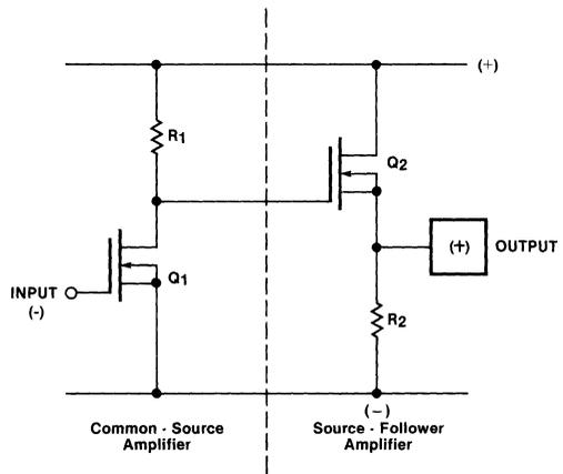
Figure 22. Linear Amplification
