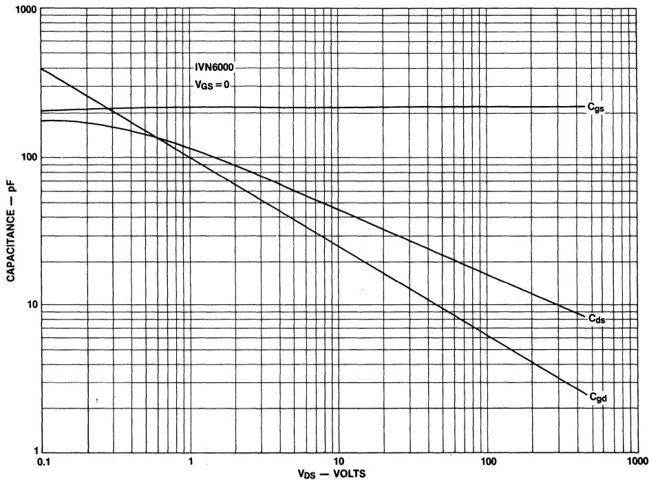
Figure 5. Capacitance Variation with Drain-Source Voltage
