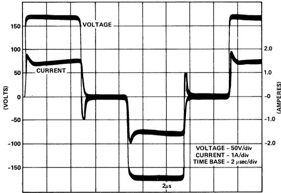
Figure 7a. Voltage/Current Waveforms Across T<sub>2</sub>, 25A Load.
