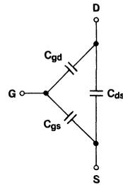
Figure 4. Capacitive Equivalent Circuit
