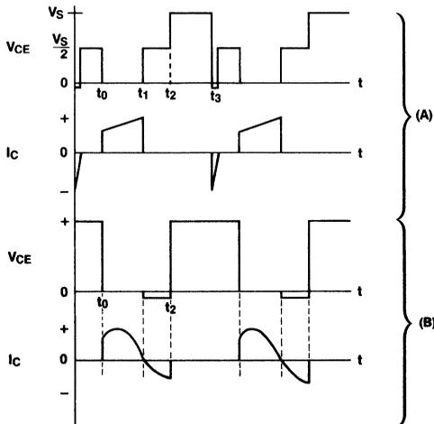
Figure 45. Q<sub>1</sub> Voltage and Current Waveforms
