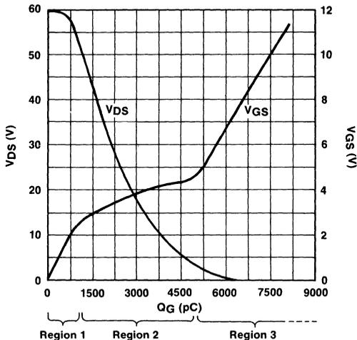
Figure 26. IVN5200  $V_{DS}$  &  $V_{GS}$  vs.  $Q_G$
