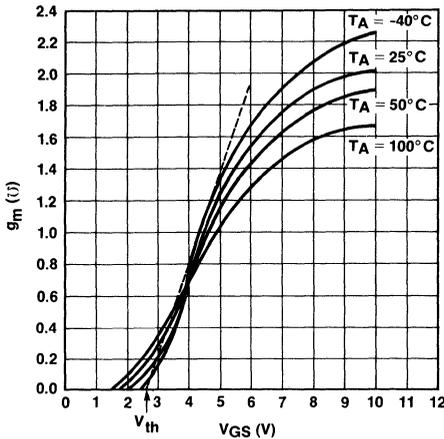
Figure 14. IVN5200  $g_m$  vs.  $V_{GS}$
