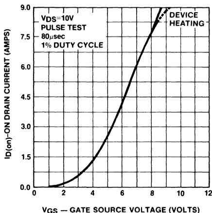
Figure 11. Transfer Characteristic
