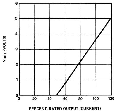
Figure 10. Current Fold-Back Characteristics
