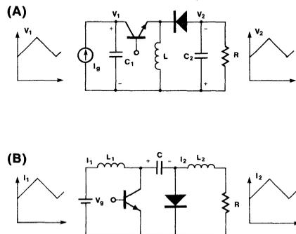
Figure 9: Comparison of Buck-Boost and Cuk Converters
