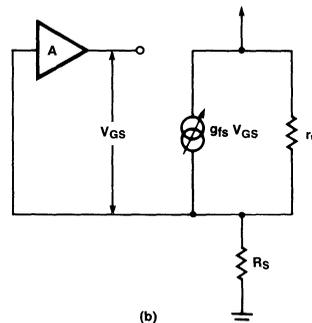
Figure 15b. Small Signal Model
