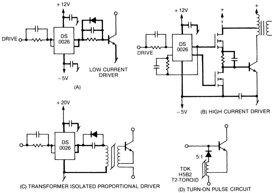
Figure 9. High frequency Base Drive Circuits
