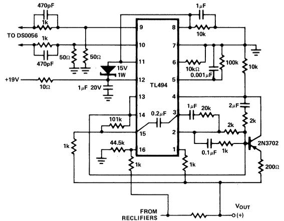
Figure 11. Alternative Control Circuit
