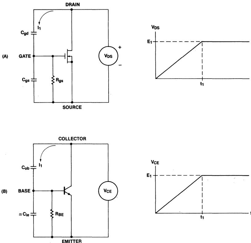
Figure 46. MOSFET and BJT Equivalent Circuits
