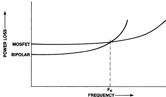
Figure 42. Comparison of BJT and MOSFET Losses
