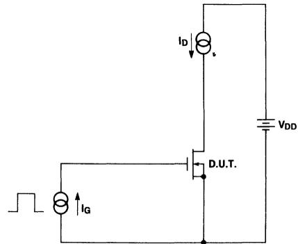
**Figure 7.** Simplified Test Circuit
