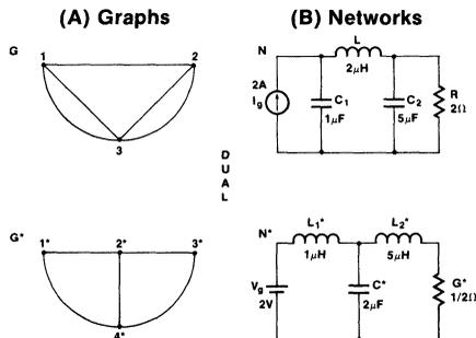
Figure 4: Example of Dual Networks (B) and Their Corresponding Graphs (A)
