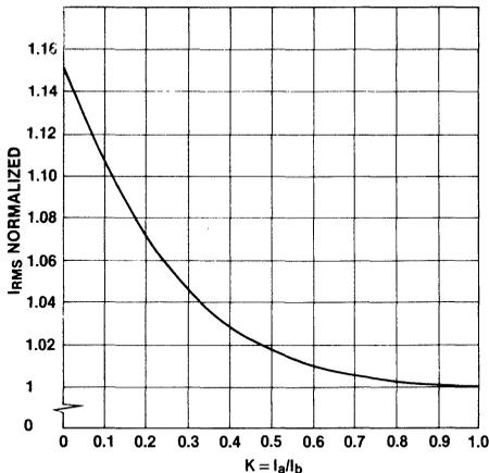
Figure 38. Variation of  $I_{RMS}$  with Trapezoidal Current Ratio
