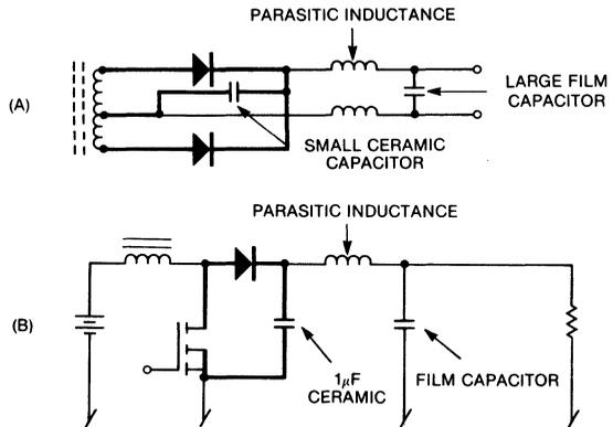
Figure 32. HF Bypassing
