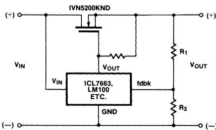
Figure 21. IC-Controlled Regulator
