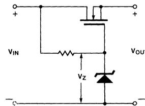
Figure 19. Basic Voltage Regulator
