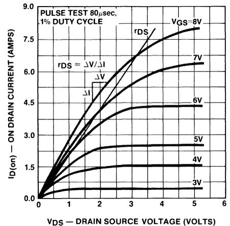
Figure 9. Output Characteristics IVN5200
