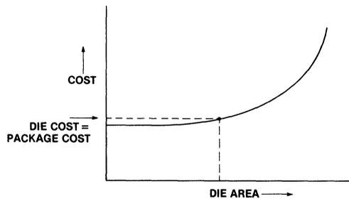
Figure 33. Die Area versus Device Cost
