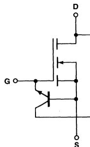
Figure 30. Parasitic NPN Transistor with Internal Zener
