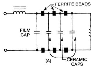
Figure 29. High Frequency Output Filters
