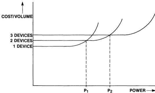
Figure 55. Cost versus Power Dissipation
