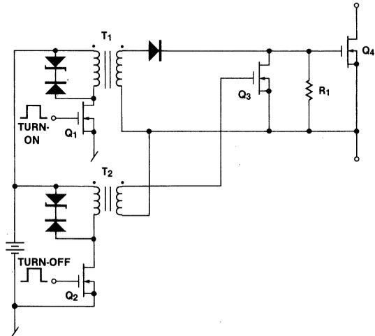
Figure 26. Pulsed Gate Drive Circuit
