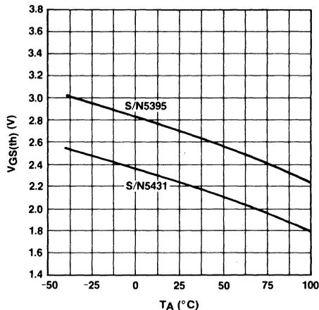
Figure 12. IVN5200  $V_{GS(th)}$  vs.  $T_A$
