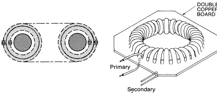
Figure 25. Coaxial Wound Toroid
