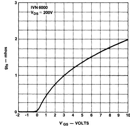
Figure 6. Transconductance vs. Gate-Source Voltage
