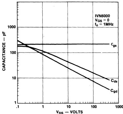
Figure 4. Device Capacitances
