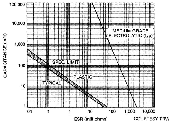
Figure 19. Plastic Film Versus Electrolytic
