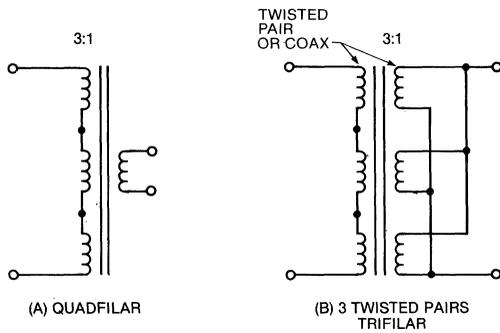
Figure 22. High Frequency Transformer Winding Techniques
