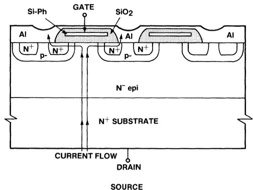
Figure 4. Vertical DMOS Structure
