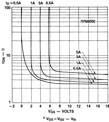
Figure 27. Variation of  $r_{ON}$  with  $V_{GS}$  and  $I_D$
