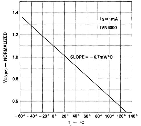
Figure 29. Variation of Threshold Voltage with Temperature
