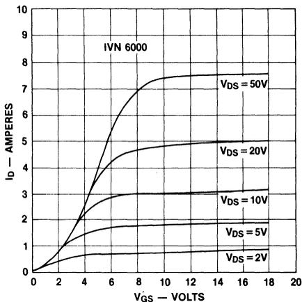
Figure 32. Large Signal Transfer Characteristic
