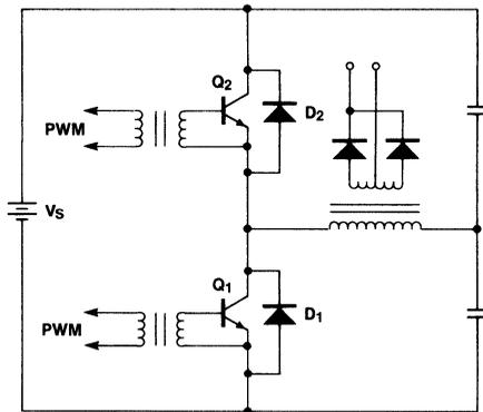
Figure 44. Typical Switching Regulator Circuit
