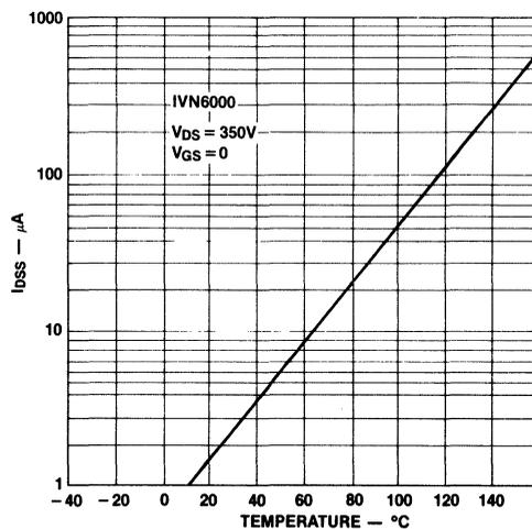
Figure 35. Drain-Source Leakage Current versus Temperature
