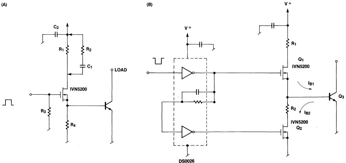
Figure 56. Bipolar Base Drive Using MOSFET
