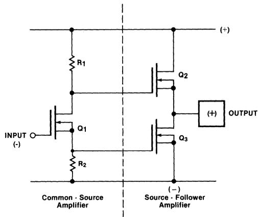
Figure 23. Linear Amplification
