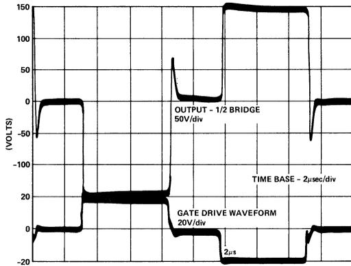
Figure 8. Half Bridge Waveforms (5V/25A Load)
