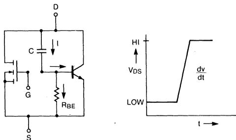
Figure 13. Parasitic NPN Switchback
