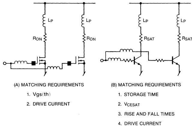
Figure 14. Parallel Switch Connections
