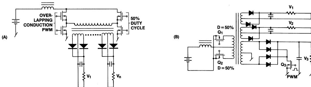
Figure 41. Boost Derived Power Converters
