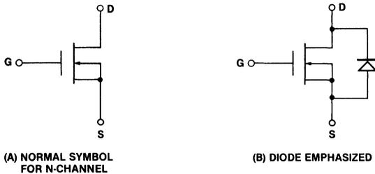
Figure 53. Diode in MOSFET Structure
