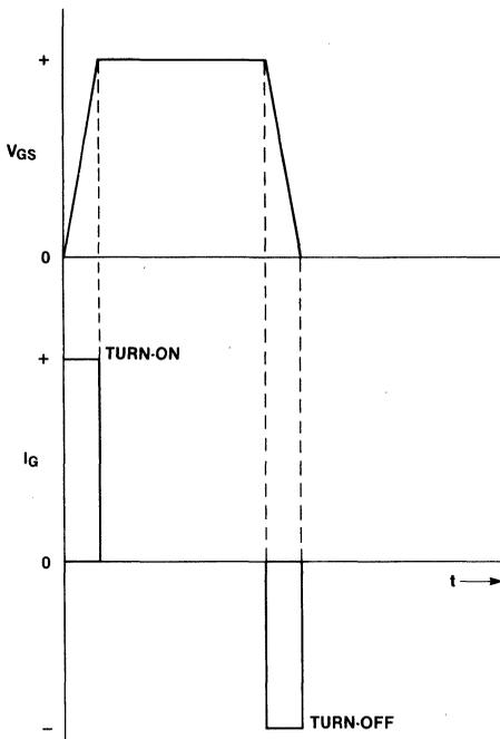
Figure 15. Ideal Gate Drive Waveforms
