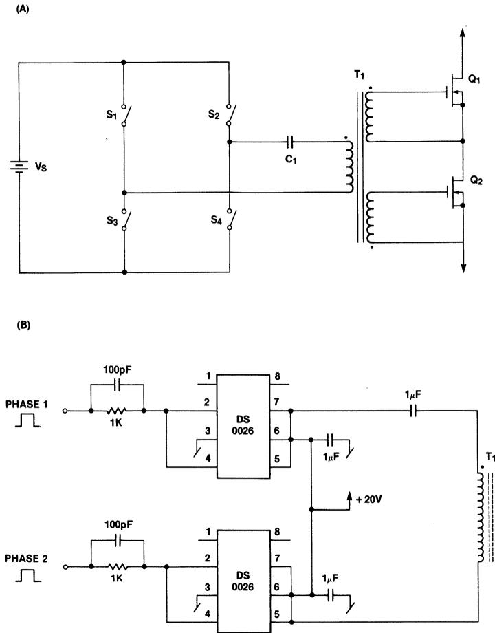
**Figure 23. Symmetrical Transformer Coupled Drive Circuit**
