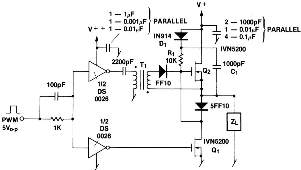
$T_1$  — is three turns 30 bifilar on a ferrite bead.
