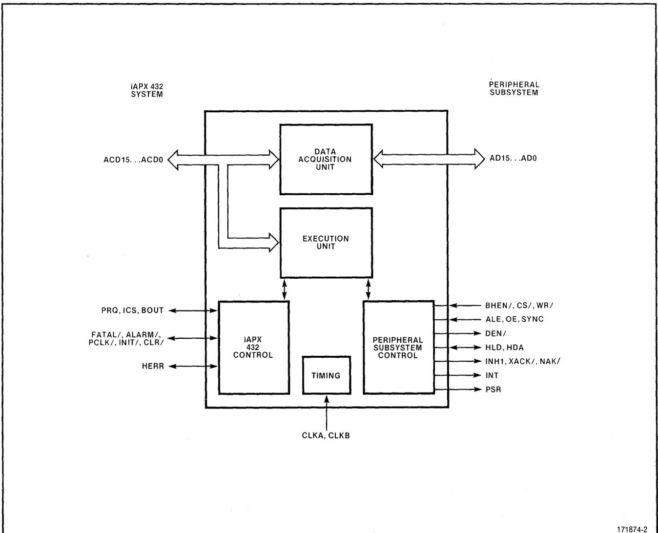
**Figure 2. iAPX 43203 IP Functional Block Diagram**
