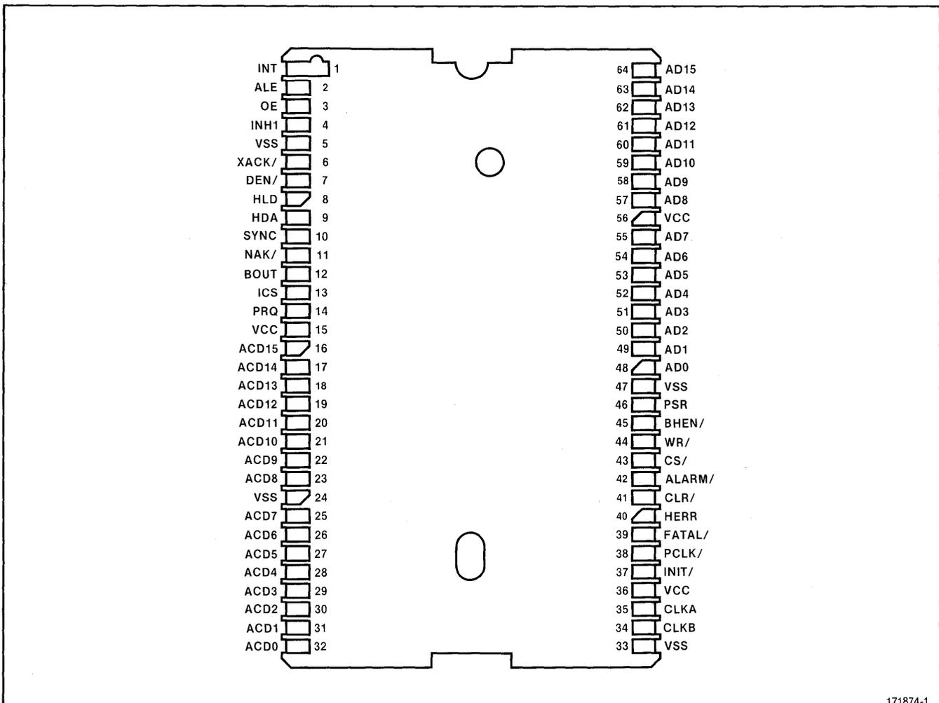
**Figure 1. iAPX 43203 Interface Processor Pin Configuration**
