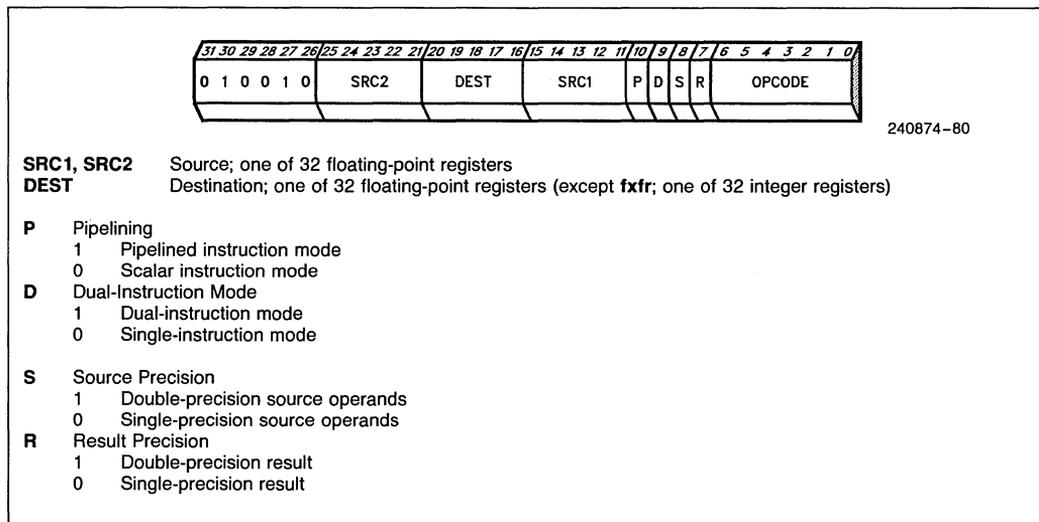
Figure 10.4. Floating-Point Instruction Encoding
