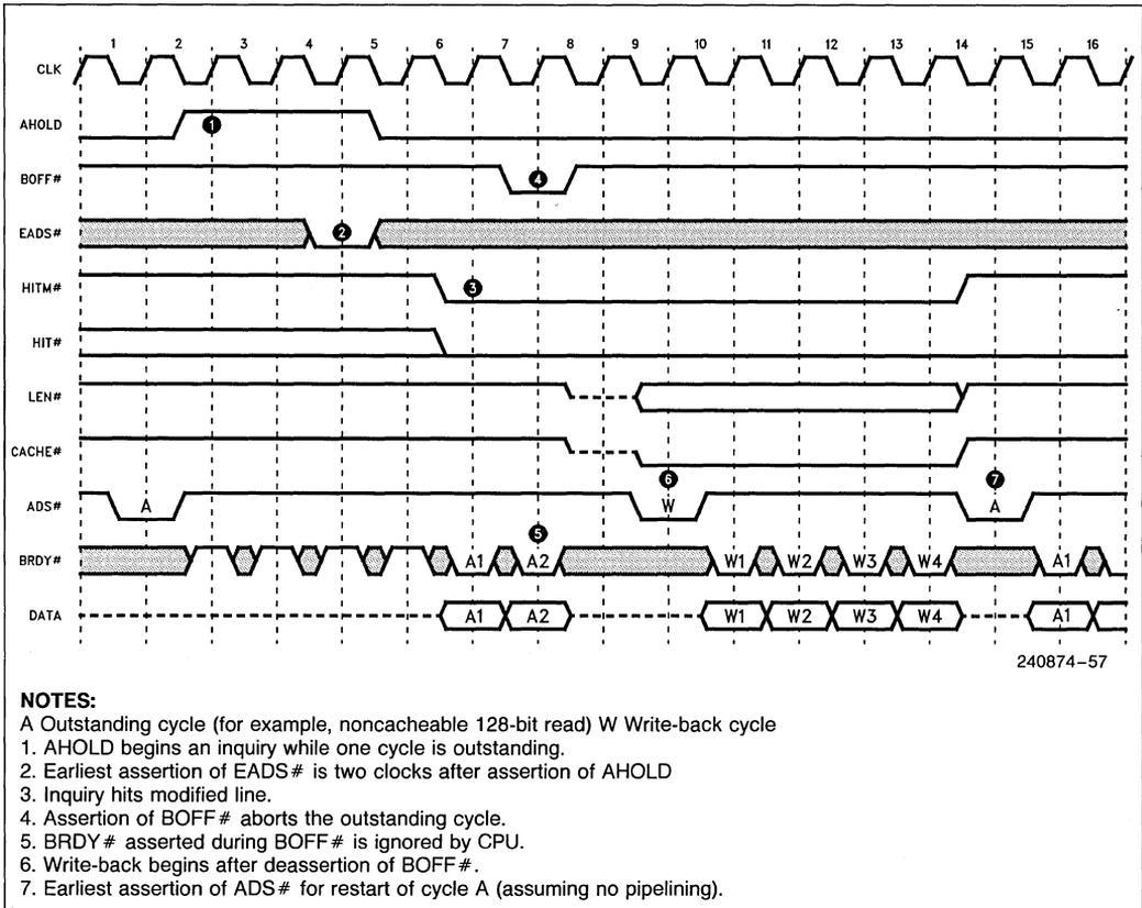
Figure 5.30. Cycle Reordering via BOFF# (Ongoing Burst)
