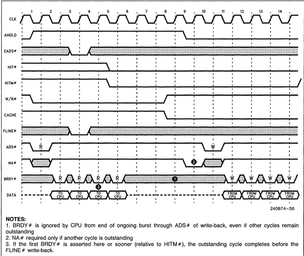
Figure 5.29. Cycle Reordering via FLINE# (Ongoing Burst)
