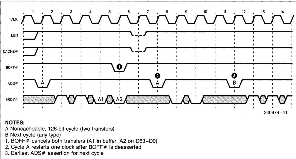
Figure 5.14. One-Clock Late Back-Off Mode (Case 1)
