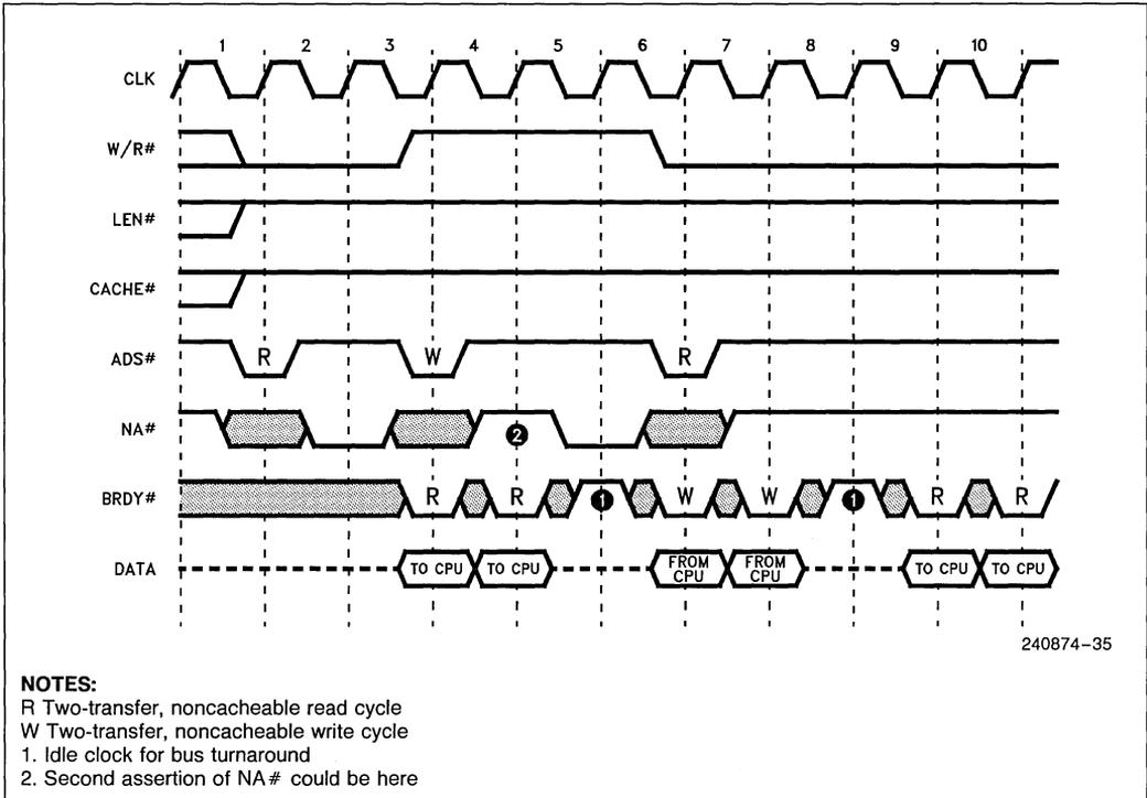
Figure 5.8. Pipelined Back-to-Back Read and Write Cycles
