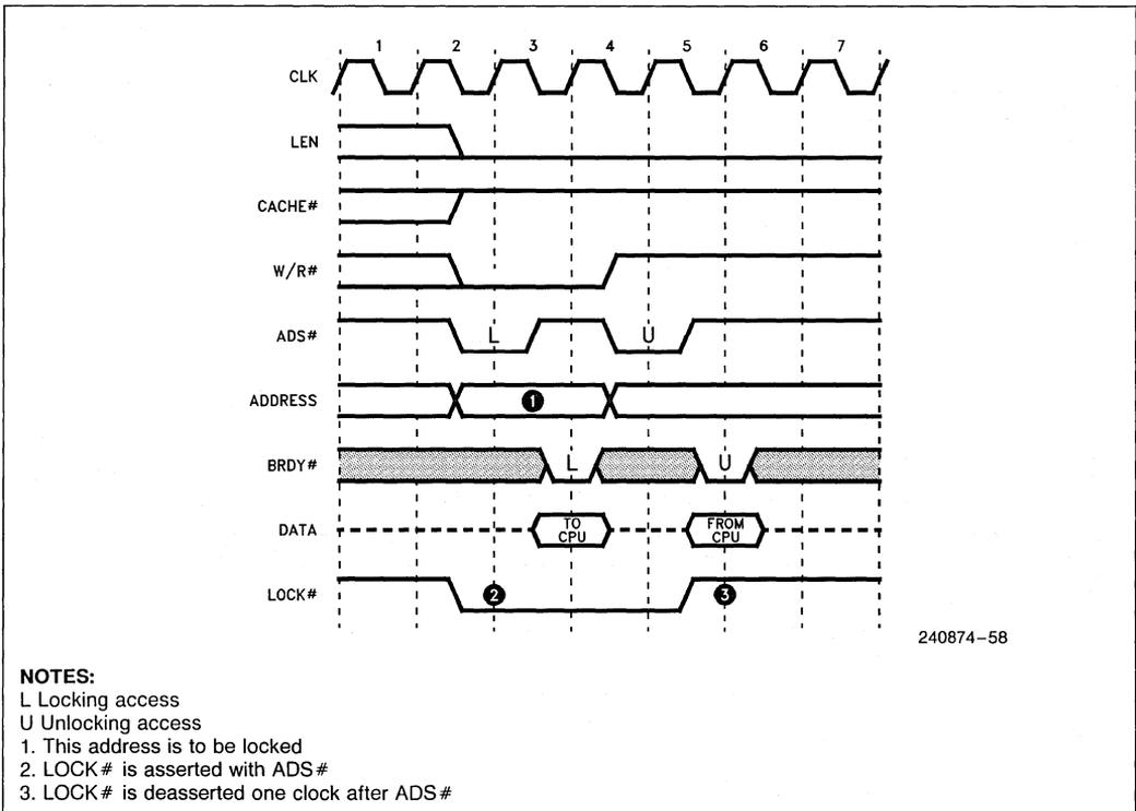
Figure 5.31. LOCK# Timing
