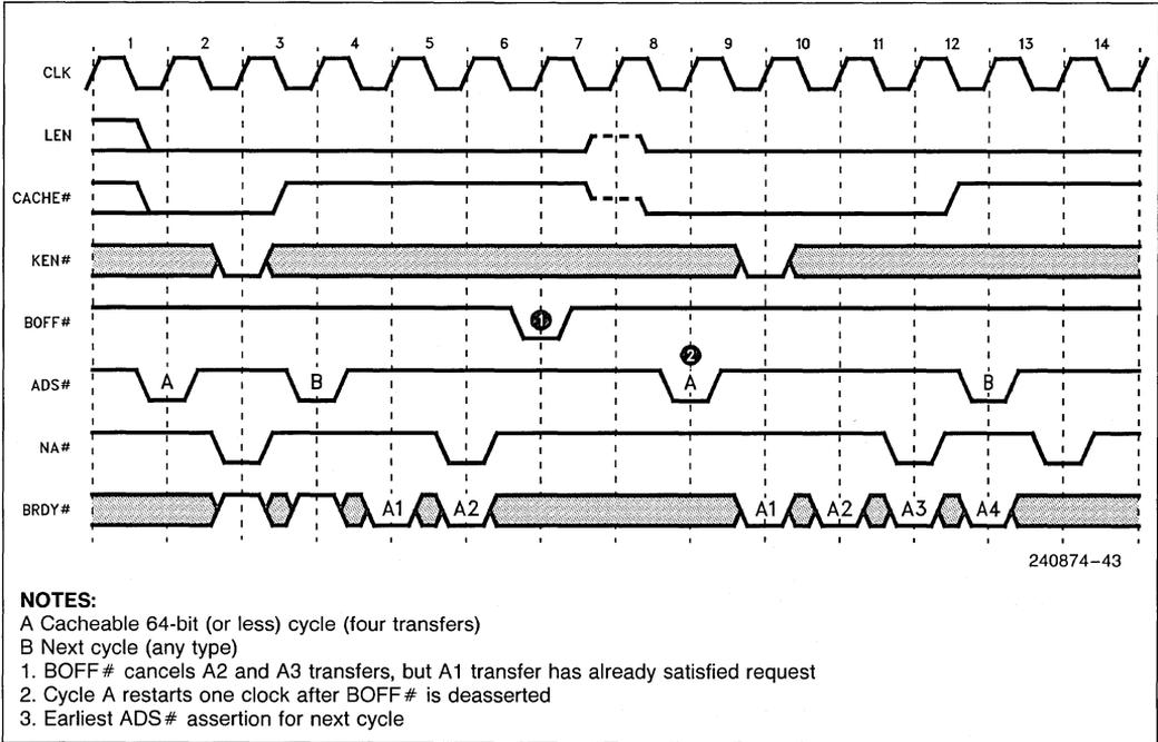
Figure 5.16. One-Clock Late Back-Off Mode (Case 3)
