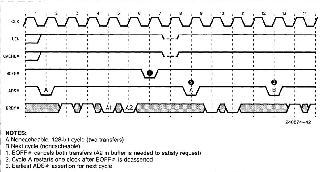
Figure 5.15. One-Clock Late Back-Off Mode (Case 2)
