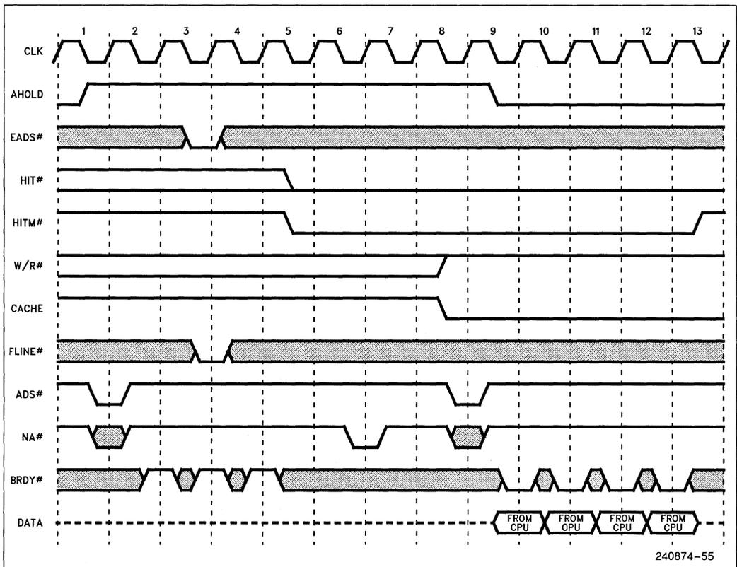
**Figure 5.28. Cycle Reordering via FLINE# (No Ongoing Burst)**
