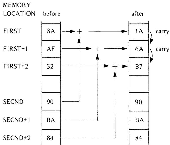
The following routine uses an ADC instruction to add the low-order bytes of the operands. This could cause the result to be high by one if the carry flag were left set by some previous instruction. This routine avoids the problem by clearing the carry flag with the XRA instruction just before LOOP.
