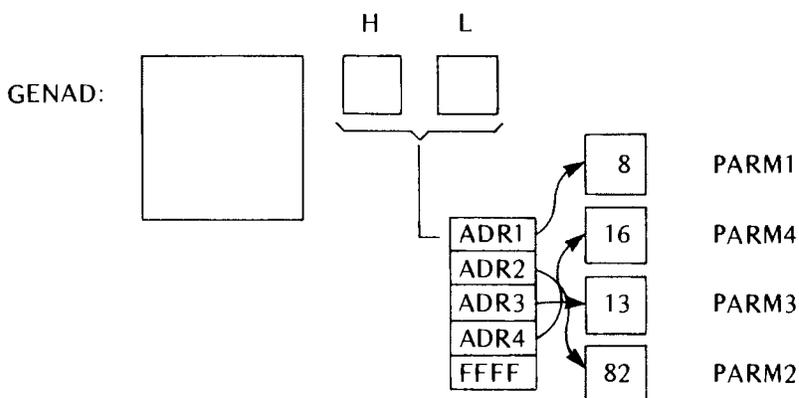
As implemented below, GENAD saves the current sum (beginning with zero) in the C register. It then loads the address of the first parameter into the D and E registers. If this address is greater than or equal to FF00H, it reloads the accumulator with the sum held in the C register and returns to the calling routine. Otherwise, it
