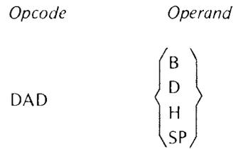
DAD may add only the contents of the B&C, D&E, H&L, or the SP (Stack Pointer) register pairs to the contents of H&L. Notice that the letter H must be used to specify that the H&L register pair is to be added to itself.
