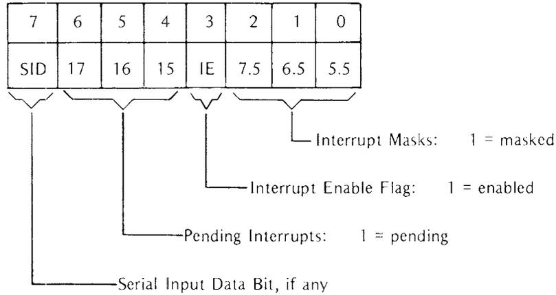
The mask and pending flags refer only to the RST5.5, RST6.5, and RST7.5 hardware interrupts. The IE flag refers to the entire interrupt system. Thus, the IE flag is identical in function and level to the INTE pin on the 8080. A 1 bit in this flag indicates that the entire interrupt system is enabled.
