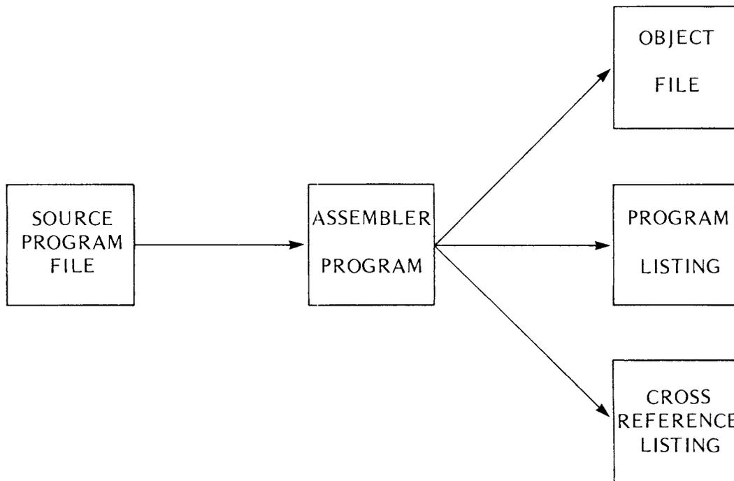
Figure 1-1. Assembler Outputs
