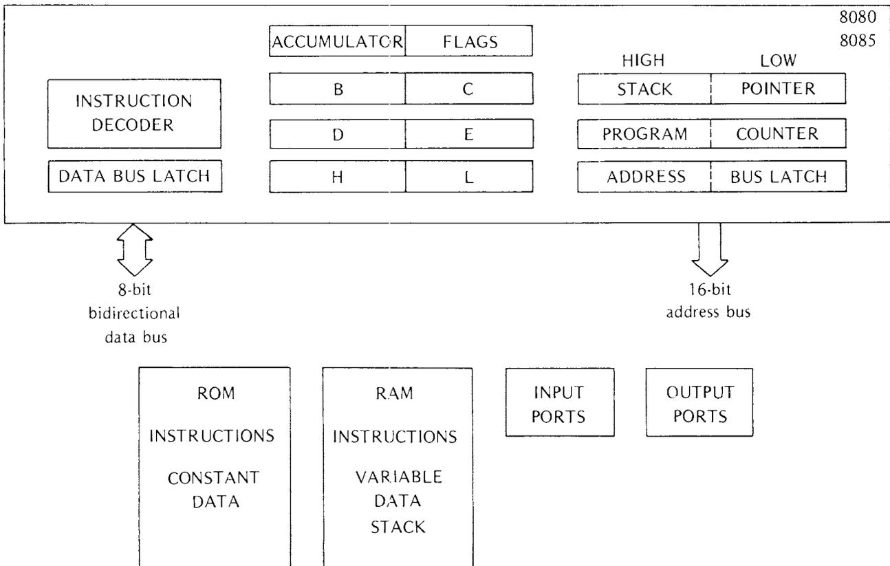
Figure 1-3. 8080/8085 Internal Registers
