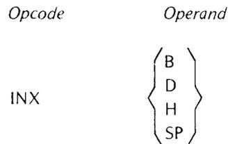
`INX` may increment only the B&C, D&E, H&L, or the SP (Stack Pointer) register pairs. Notice that the letter H must be used to specify the H and L register pair.
