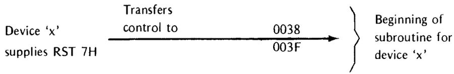
Note that any of these 8-byte subroutines may in turn call longer subroutines to process the interrupt, if necessary.
