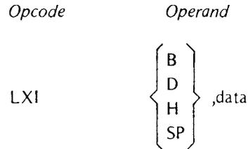
The first operand must specify the register pair to be loaded. LXI can load the B and C register pair, the D and E register pair, the H and L register pair, or the Stack Pointer.
