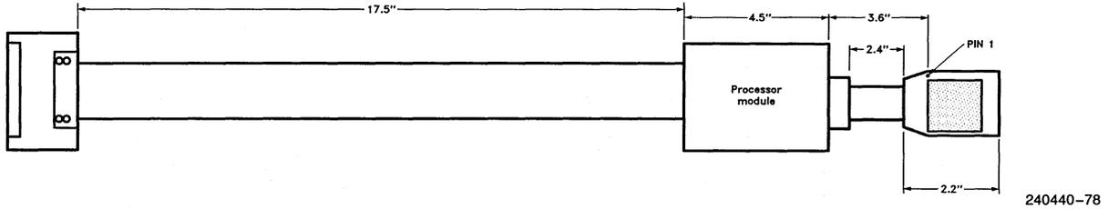
**Processor Module Assembly Dimensions
