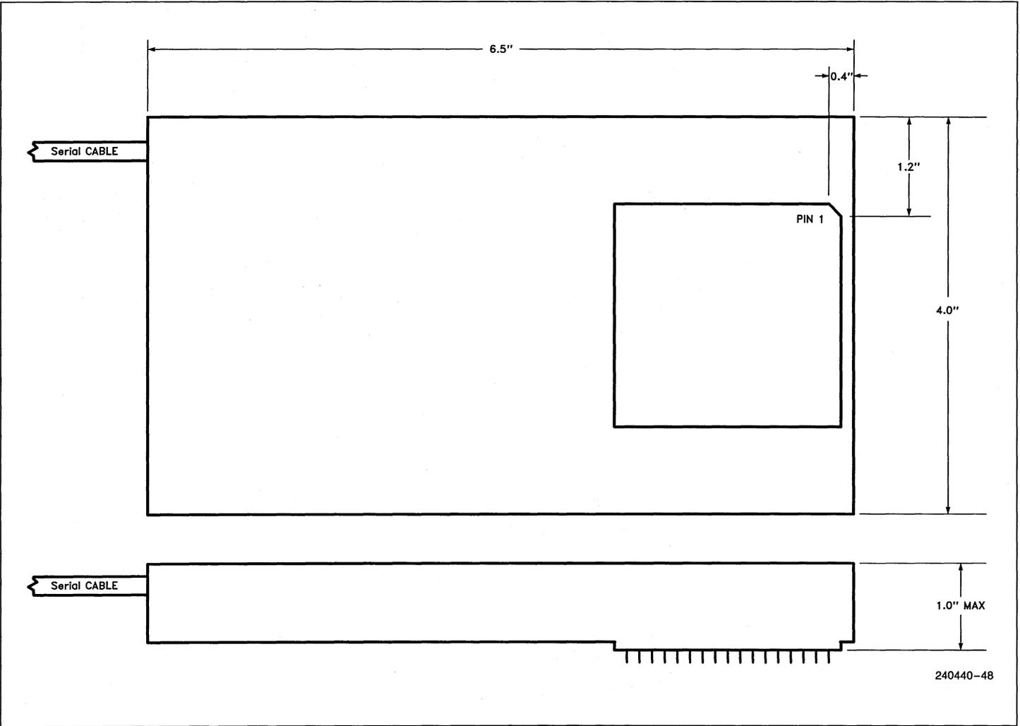
Figure 13.4a. ICD-486™ Probe Dimensions
