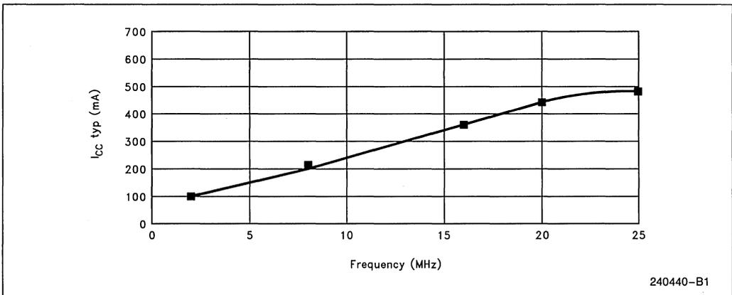
Figure 15.7. Frequency vs I<sub>CC</sub>(typ) (PQFP Version)
