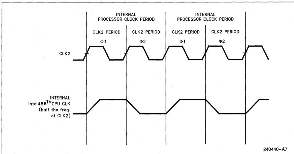
Figure 15.3. CLK2 Signal and Internal Processor Clock
