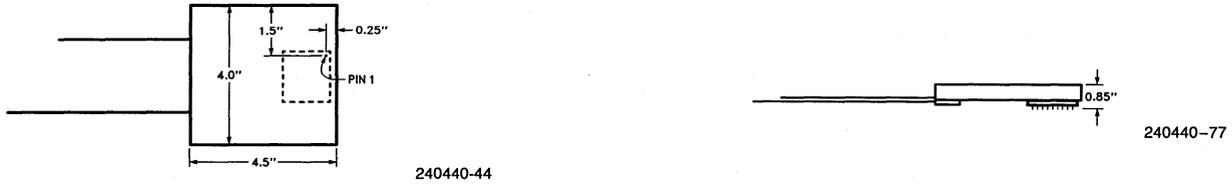
**Processor Module Assembly Dimensions
