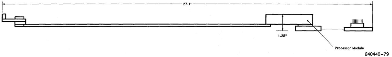
**Processor Module Assembly Dimensions
