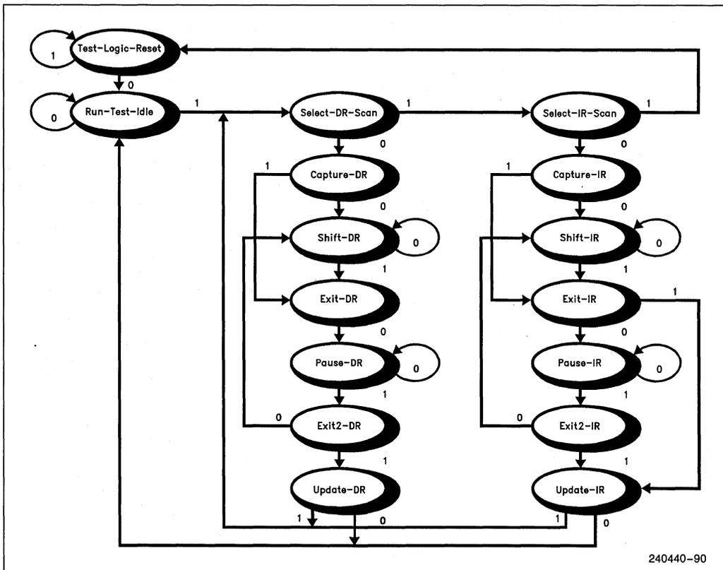
Figure 8.3. TAP Controller State Diagram
