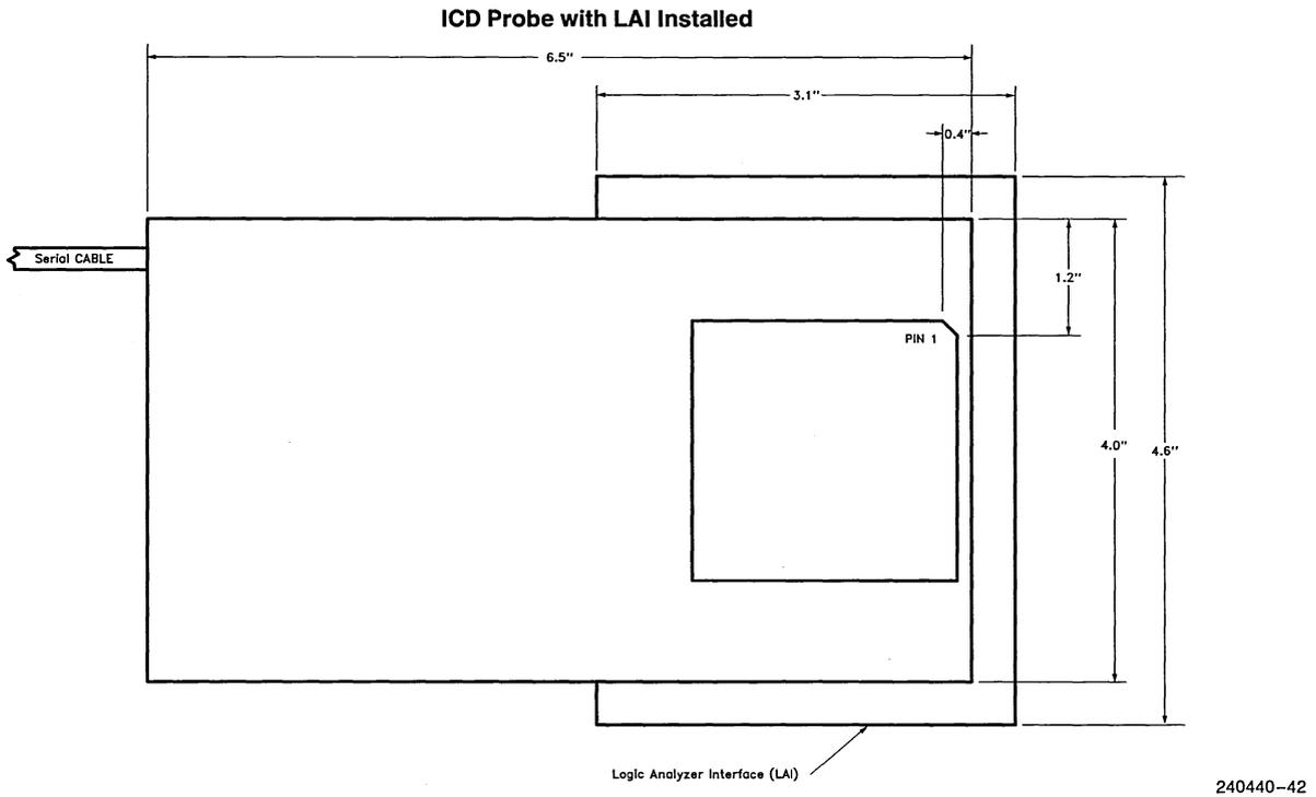
Figure 13.4b. ICD-486™ Probe Dimensions
