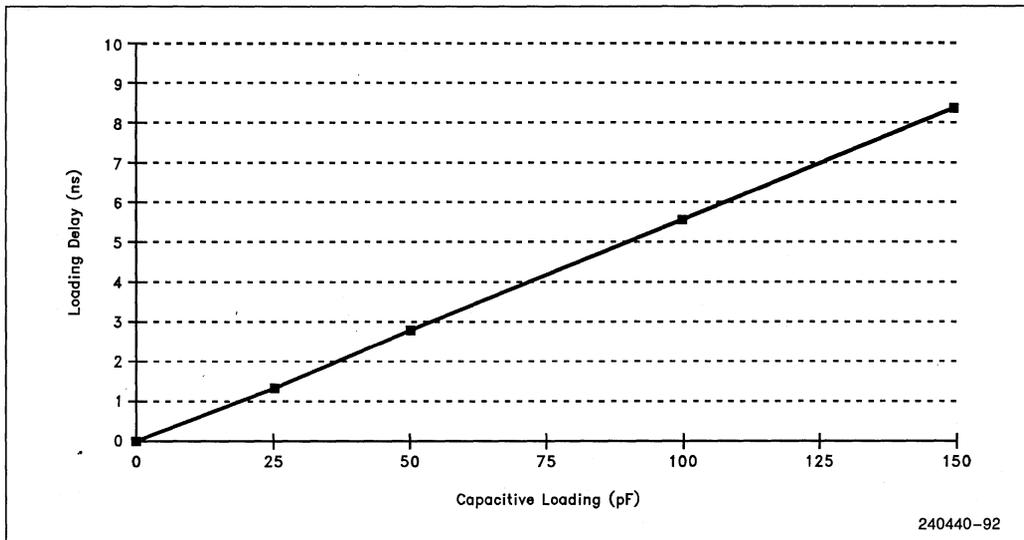
13.4.3.b TYPICAL LOADING DELAY VERSUS CAPACITIVE LOADING UNDER WORST-CASE CONDITIONS FOR A LOW TO HIGH TRANSITION ON THE 50 MHz Intel486 CPU
