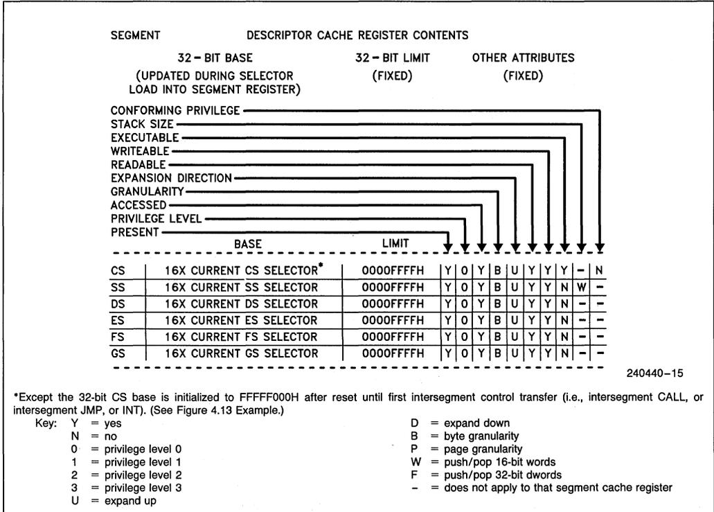
**Figure 4.11. Segment Descriptor Caches for Real Address Mode
