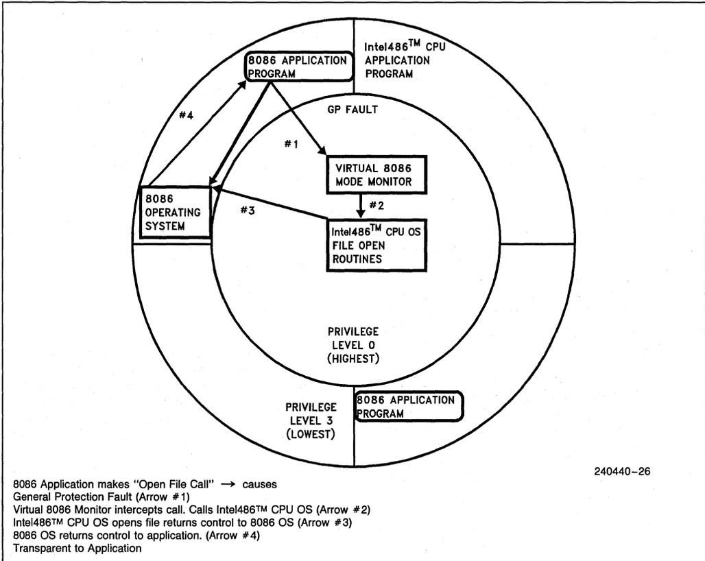
**Figure 4.25. Virtual 8086 Environment Interrupt and Call Handling**
