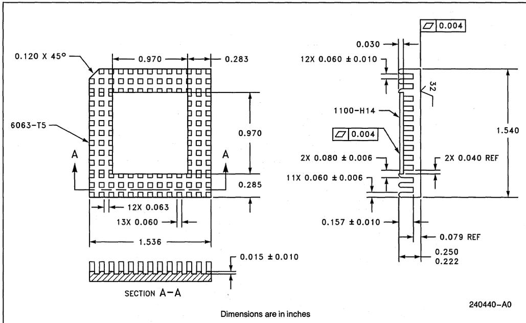
Figure 12.4. Intel OverDrive™ Processor Heat Sink Dimensions
