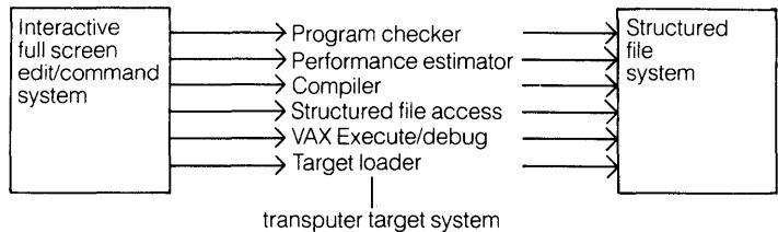
The transputer development system runs on any VAX computer (including MicroVAX) under versions 3 and 4 of VMS. It provides all the facilities of the occam programming system, and is entered by a simple VMS command. Within the system the user edits, compiles and debugs occam programs, exploiting the full screen text editing facilities and using function keys to access the capabilities of the toolset provided by the system.
