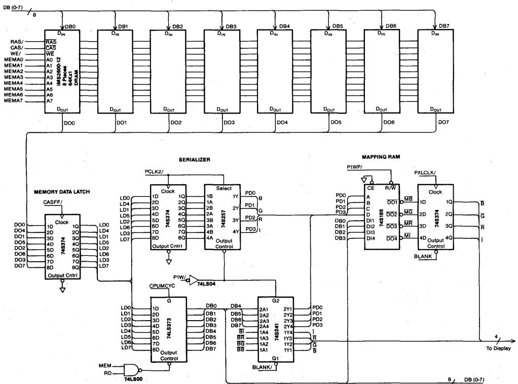
**Figure 4. Data Flow Circuits**
