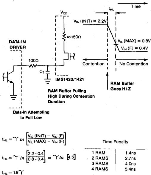
Using:  $C_{I/O} (\text{RAM}) = 7\text{pF}$  &  $C (\text{Board})/\text{RAM} = 2\text{pF}$ ,  $C_T = 9\text{pF}/\text{RAM}$
