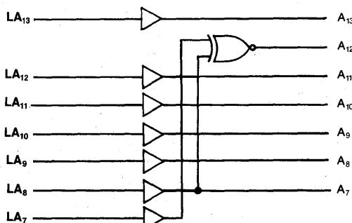
Figure 2: IMS1400 Address Encoder Circuit
