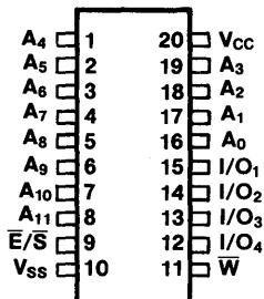
Figure 1: IMS1420/1421 Pin Configuration
