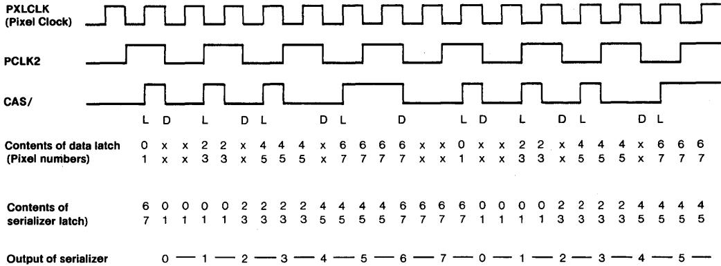
Figure 5. Data Flow Through Serializer
