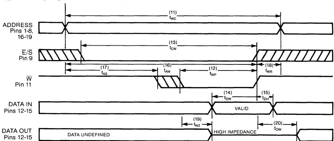
**RECOMMENDED AC OPERATING CONDITIONS** ( $0^{\circ}\text{C} \leq T_A \leq 70^{\circ}\text{C}$ ) ( $V_{\text{CC}} = 5.0\text{V} \pm 10\%$ )**WRITE CYCLE 2:  $\bar{E}/\bar{S}$  CONTROLLED<sup>h</sup>**
