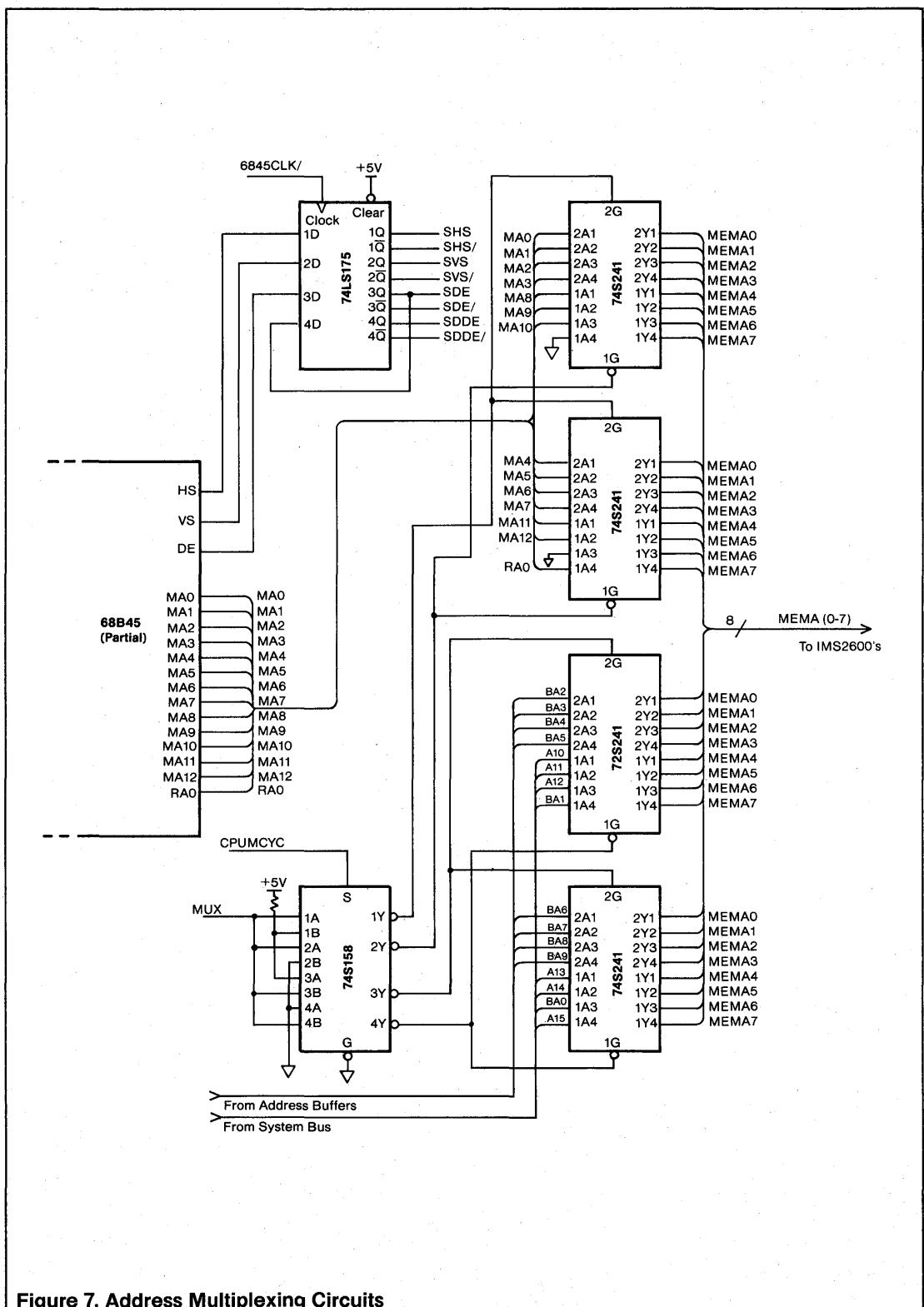
Figure 7. Address Multiplexing Circuits
