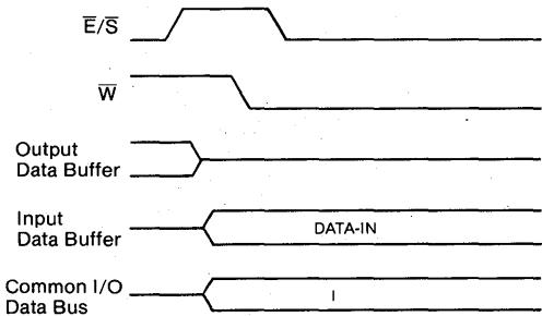
**Figure 4:**  $\overline{E/S}$  Used to Control Output Buffer
