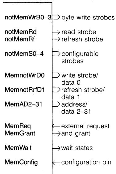
The memory interface uses a 32-bit wide address/data bus and its controller may be configured, on reset, to suit a wide variety of different memory systems. One of 13 preset configurations may be selected or the configuration may be supplied externally.
