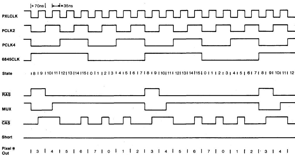
**Figure 2a. Continuous Active Display Accesses**
