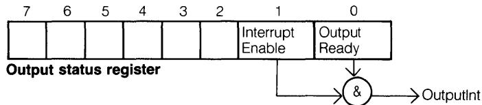
The **output ready** status bit indicates that the serial link is able to receive a byte of data. It is set on reset, and when the C002 receives an acknowledgement from the serial link. It is reset when a data byte is written to the output data register on the parallel interface. **Outputint** is set if both **output ready** and **interrupt enable** are set.
