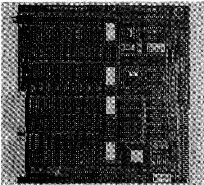
The IMS B002 evaluation board enables users to evaluate and demonstrate the use of transputers. The board is one of a family of compatible evaluation boards. It provides standard buffered INMOS link connections and external control of the transputer's Reset and Analyse functions. This allows it to control a subsystem consisting of other compatible boards, or to be a component of such a subsystem.
