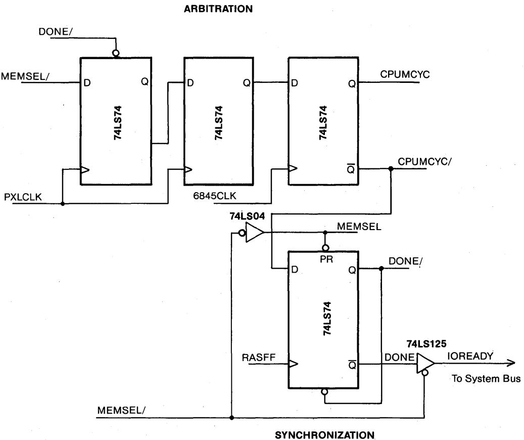
Figure 6. Arbitration and Synchronization
