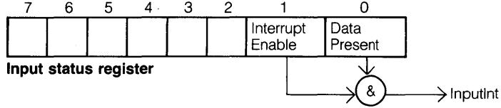
The **data present** status bit indicates that the serial link has received a byte of data. It is reset when the data byte is read from the input data register on the parallel interface, this causes an acknowledgement to be transmitted on the serial link. **Inputint** is set if both **data present** and **interrupt enable** are set.
