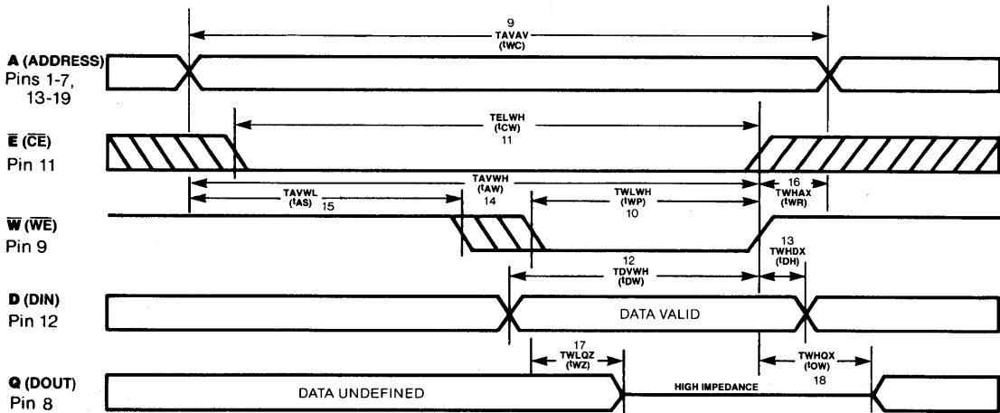
**RECOMMENDED AC OPERATING CONDITIONS** ( $-55^{\circ}\text{C} \leq T_A \leq 125^{\circ}\text{C}$ ) ( $V_{\text{CC}} = 5.0\text{V} \pm 10\%$ )**WRITE CYCLE 2:  $\bar{E}$  CONTROLLED<sup>h</sup>**
