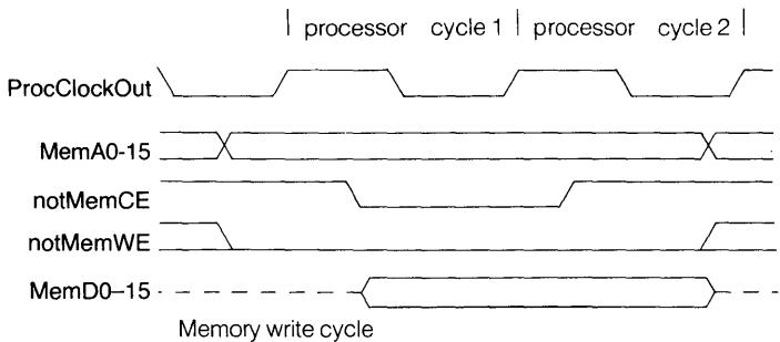
The address is valid at the falling edge of **notMemCE**, and the interface strobes the data from **MemD0–15** on the rising edge of **NotMemCE**.
