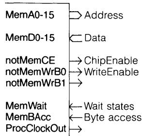
The memory interface consists of a 16 bit address bus and a 16 bit data bus. It performs word reads and word writes in 2 processor cycles. A processor cycle is identified by **ProcClockOut**.
