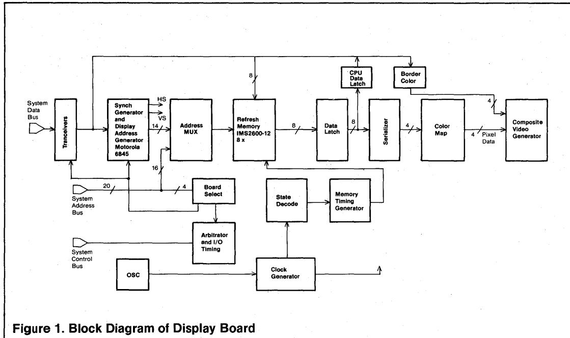
**Figure 1. Block Diagram of Display Board**
