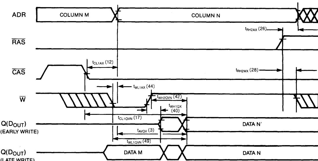
If Column Address N = Column Address M, Cycle is Write-Verify.
