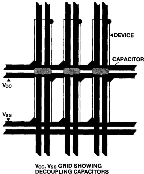
capacitor with a value between  $22\mu F$  and  $47\mu F$  should be placed near the memory board edge connection where the power traces meet the backplane power distribution system. These large capacitors provide bulk energy storage to prevent voltage drop due to the main supply being located off the memory board and at the end of a long inductive path.
