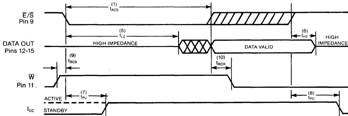
RECOMMENDED AC OPERATING CONDITIONS ( $0^\circ\text{C} \leq T_A \leq 70^\circ\text{C}$ ) ( $V_{CC} = 5.0\text{V} \pm 10\%$ )**WRITE CYCLE 1:  $\bar{W}$  CONTROLLED<sup>h</sup>**
