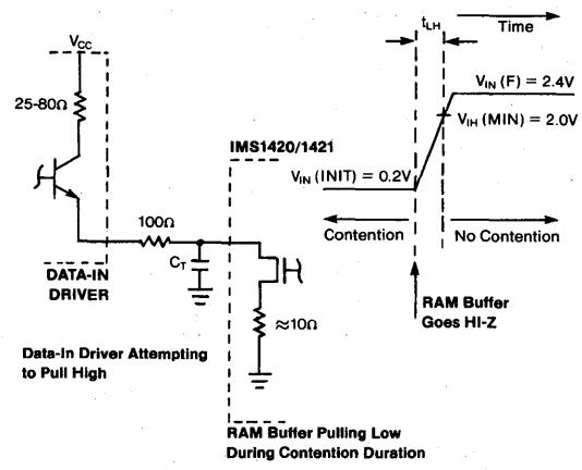
$$t_{LH} = T \ln \left[ \frac{V_{IN}(F) - V_{IN}(\text{INIT})}{V_{IN}(F) - V_{IN}(\text{MIN})} \right]$$
