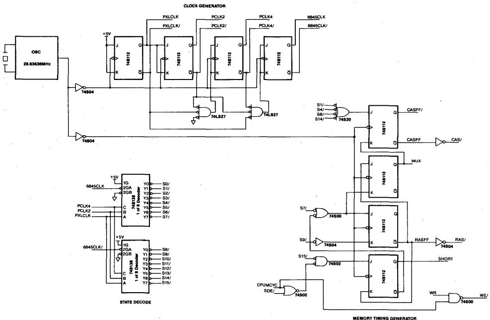
**Figure 3. Timing Generation Circuits**
