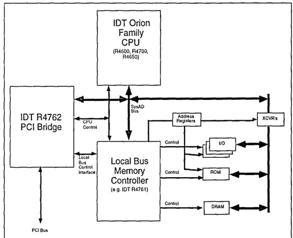
Figure 2: PCI Adapter Card built with R4762
