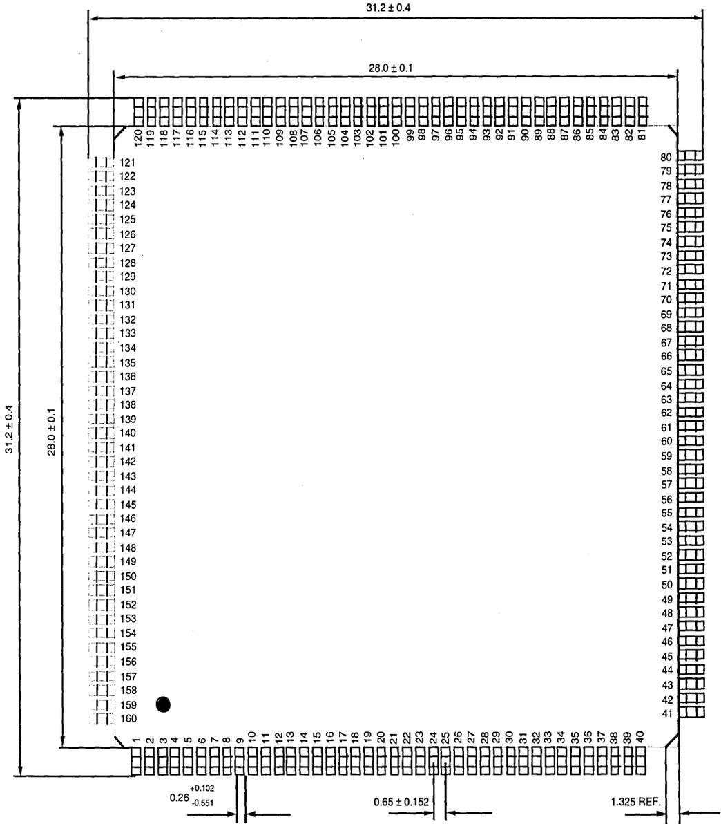
Figure 10.1: 160-Pin Quad Flat Package
