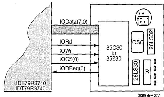
Figure 2.8: DMA-Supported AppleTalk I/O Port
