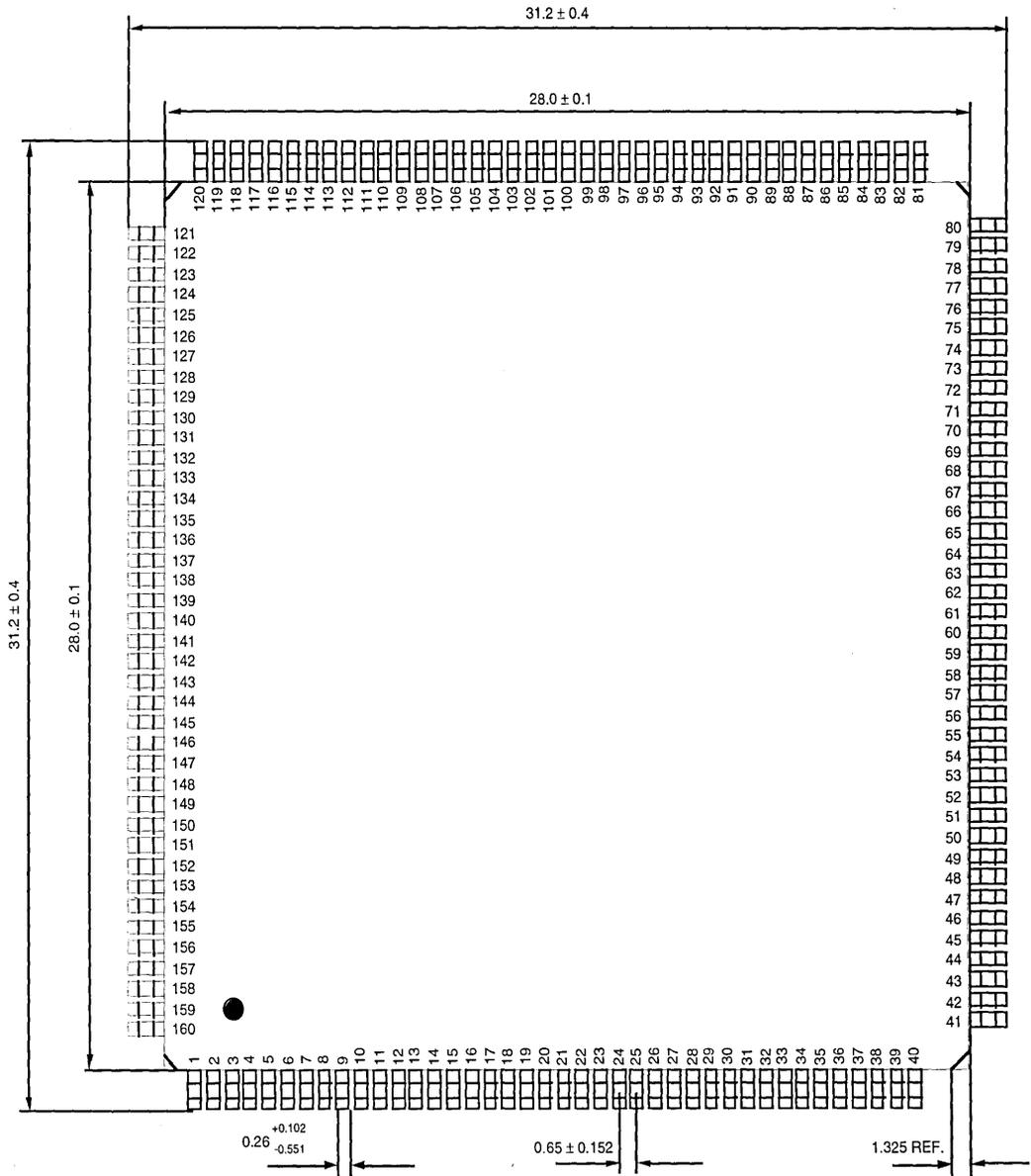
Figure 10.1 160-Pin Quad Flat Package
