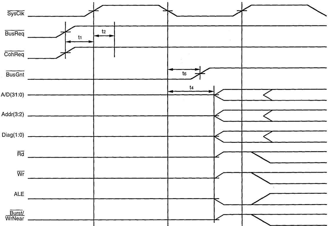
Figure 25. End of Coherent DMA Request
