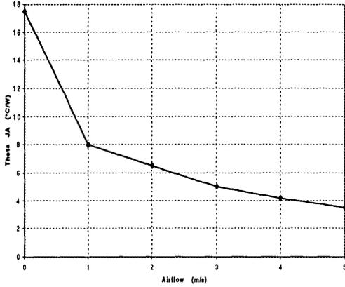
208 Pin PGA Theta JA vs. Airflow
