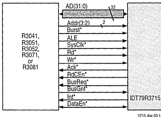
Figure 2.1 RISController to R3715 Interface
