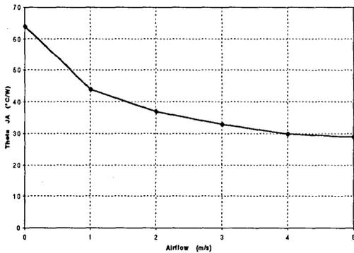
28 Pin SOJ Theta JA vs. Airflow
