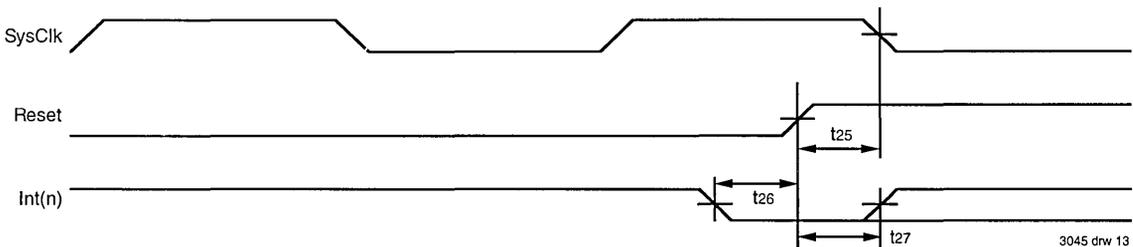
Figure 10. Mode Selection and Negation of Reset
