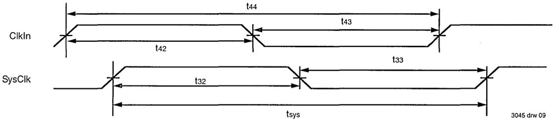
Figure 7 (a). R3071 Clcking (1x clock input mode, full frequency bus)
