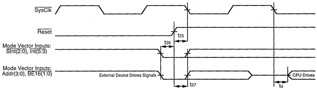
Figure 11. Mode Selection and Negation of Reset
