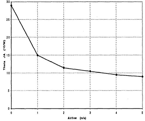
447 Pin PGA Theta JA vs. Airflow
