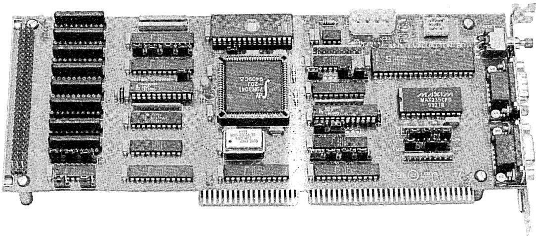
Figure 1. R3041 System Evaluation Board. Actual Size 4.2" x 10.0"
