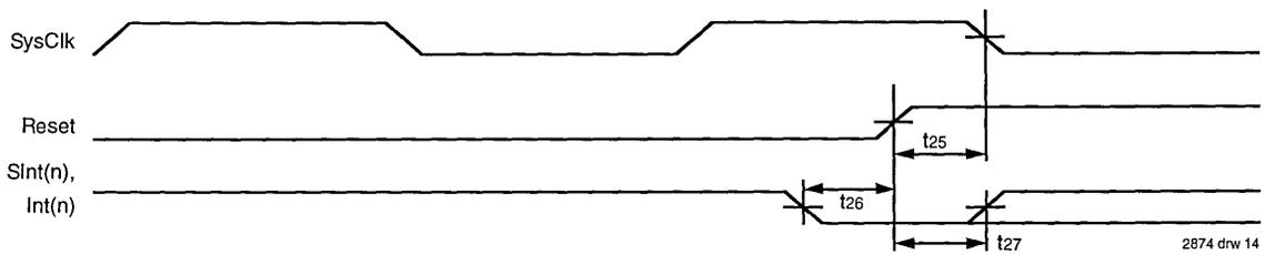
Figure 11. Mode Selection and Negation of Reset
