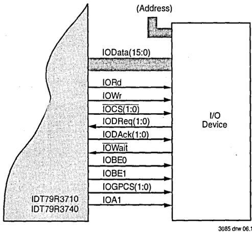
Figure 2.10: General Purpose I/O Device Interface
