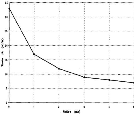
144 Pin PGA Theta JA vs. Airflow
