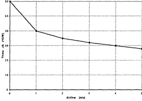
28 Pin Cerpack vs. Airflow
