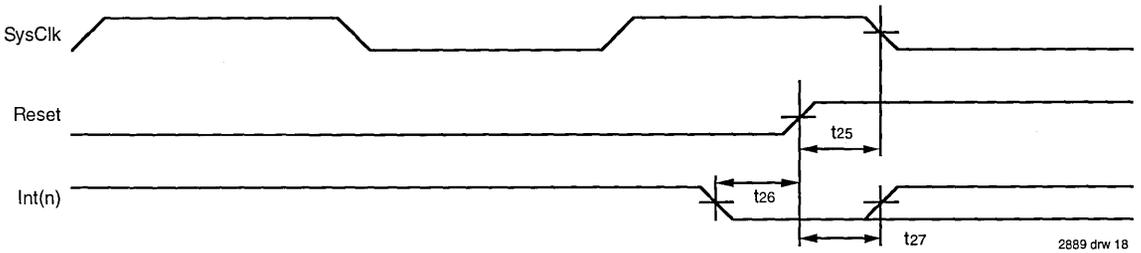
Figure 11. Mode Selection and Negation of Reset
