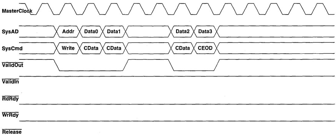
Figure 6: R4650 Block Write Request (64-bit system interface)
