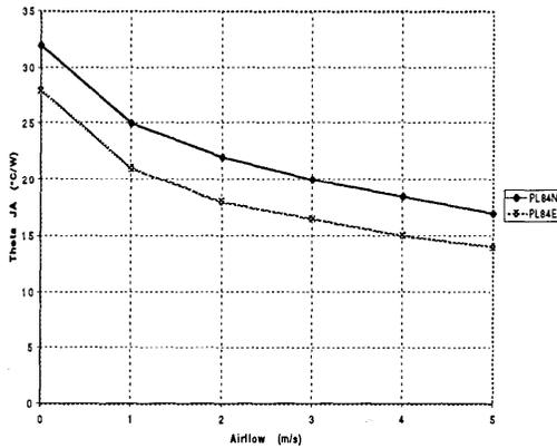
208 Pin PQFP vs. Airflow
