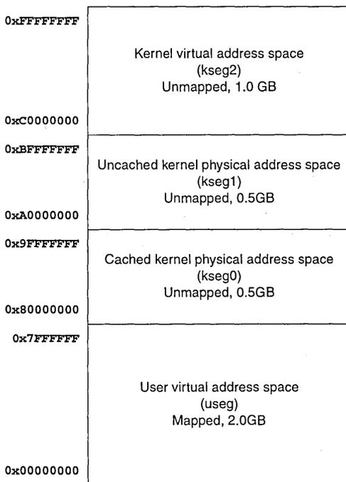
Figure 3: Mode Virtual Addressing (32-bit mode)
