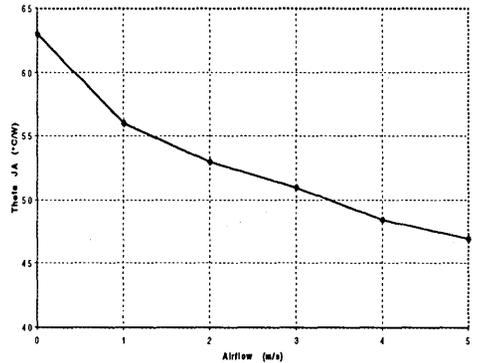
32 Pin SOJ Theta JA vs. Airflow
