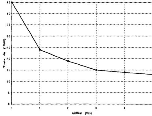
84 Pin PGA Theta JA vs. Airflow
