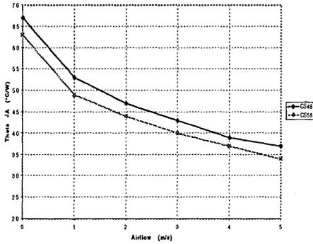
68 Pin PGA Theta JA vs. Airflow
