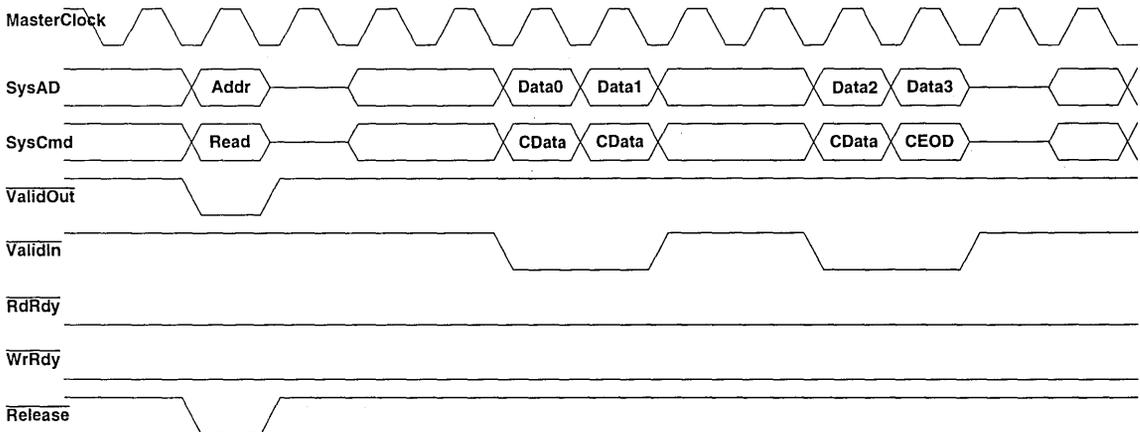
Figure 5: R4650 Block Read Request (64-bit interface option)
