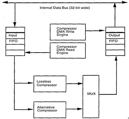
Figure 2.13.b: Compressor Block Diagram
