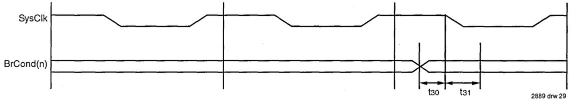
Figure 21. Direct Branch Condition Input Timing
