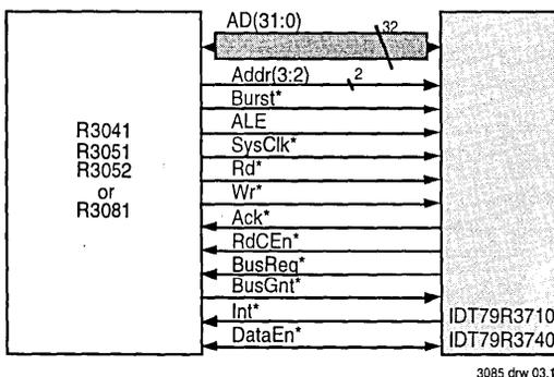
Figure 2.1: RISC Controller to R3710/R3740 Interface
