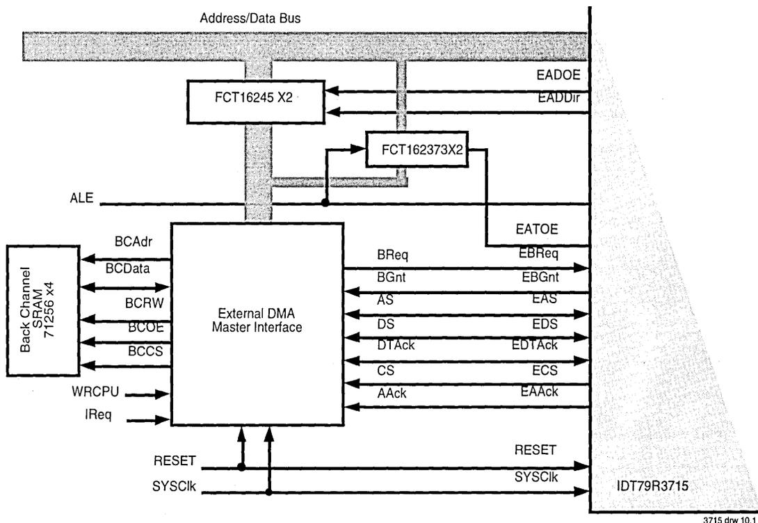
Figure 2.2 External DMA Master Coprocessor Implementation
