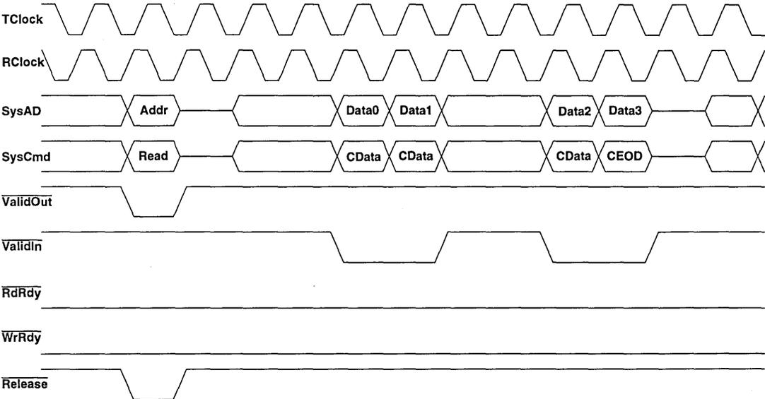
Figure 6: Processor Block Read
