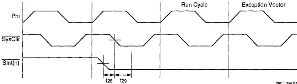
Figure 22. Synchronized Interrupt Input Timing
