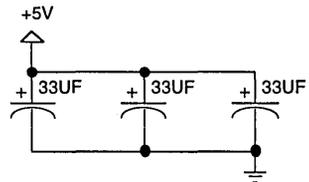
Figure 18. Primary Power Decoupling Capacitors
