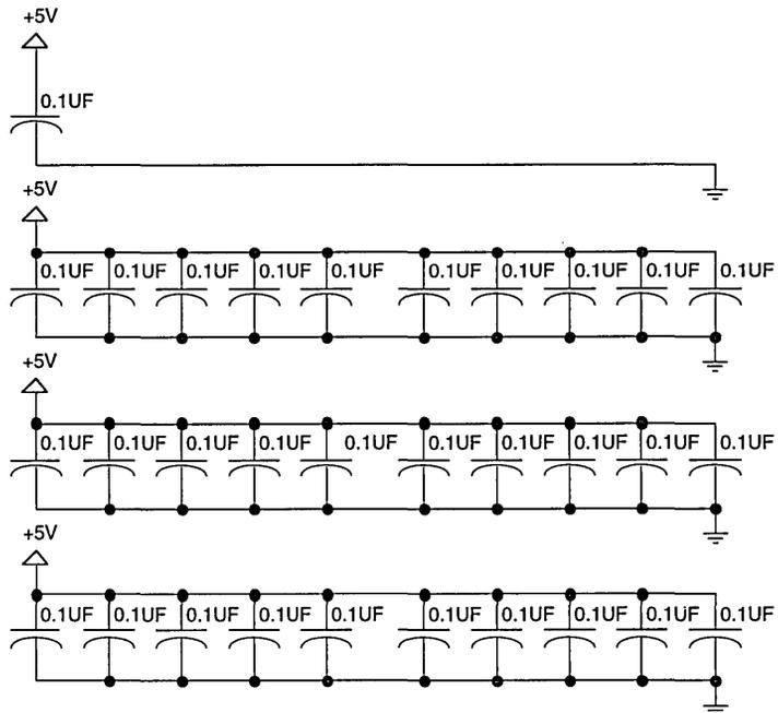
Figure 21. Decoupling Capacitors
