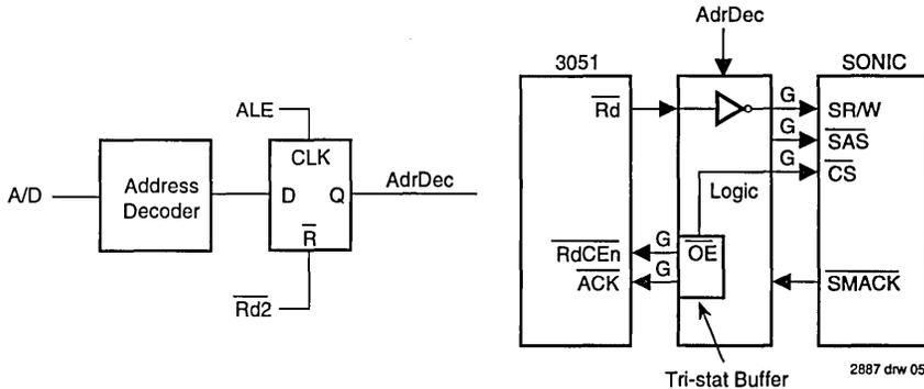
Figure 5. Slave Interface Block Diagram
