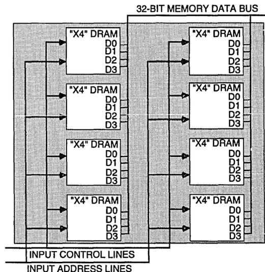
Figure 1a. Single-Bank Non-Interleaved System
