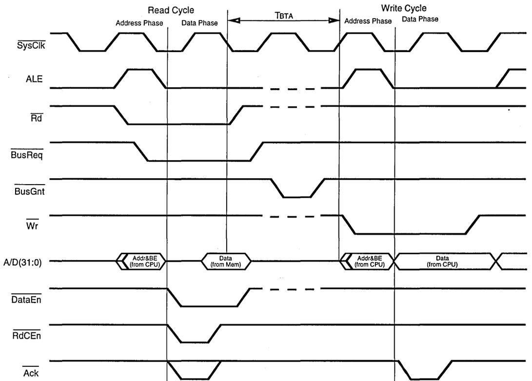
Figure 7. Using BusReq to Add More Bus Turn Around Time
