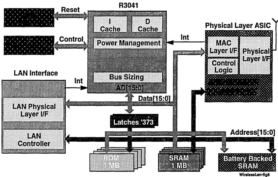
Figure 5. Access Point based on the R3041
