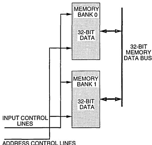
Figure 1b. Two-Bank Non-Interleaved System
