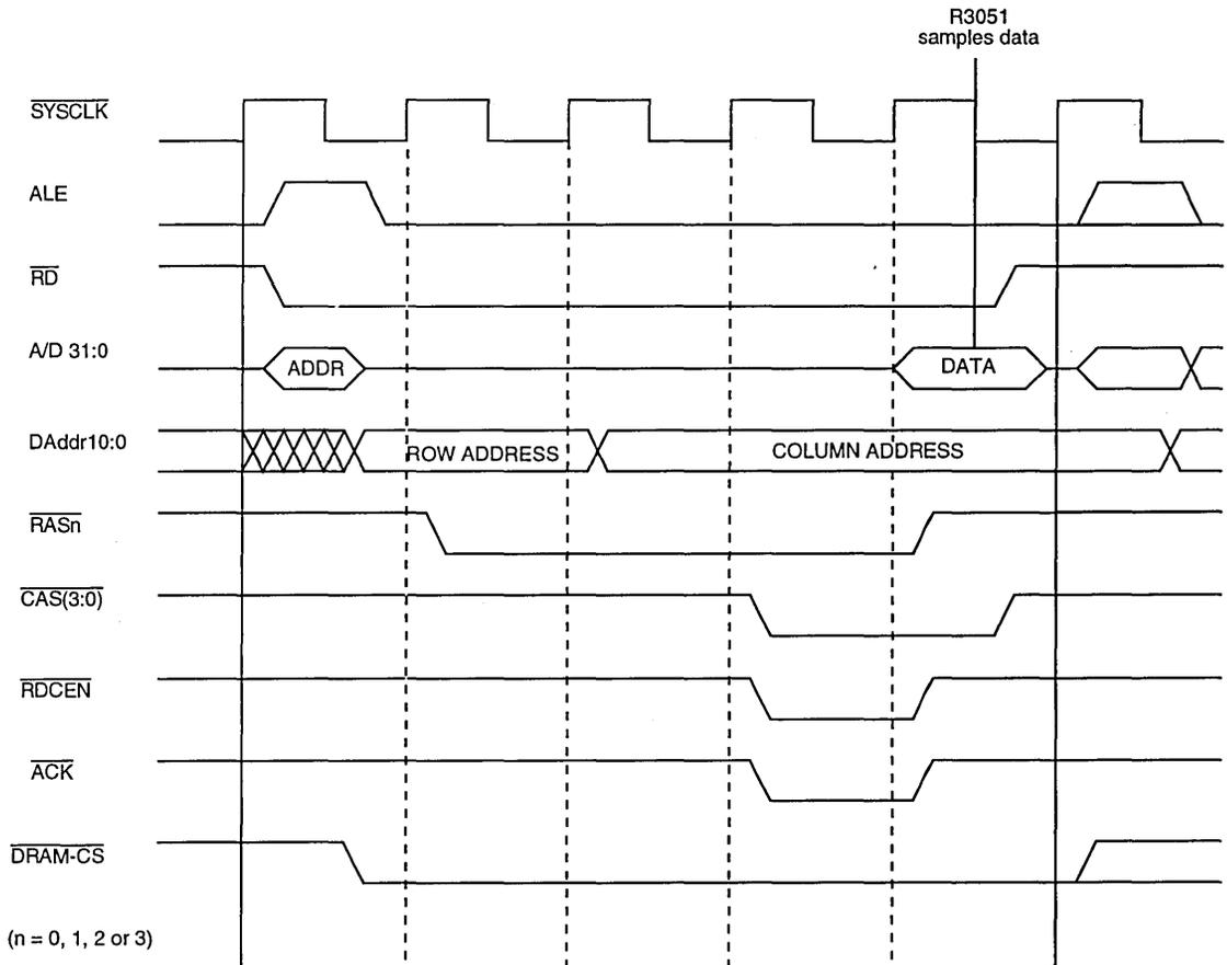
Figure 6. Single-Word Read Access Timing
