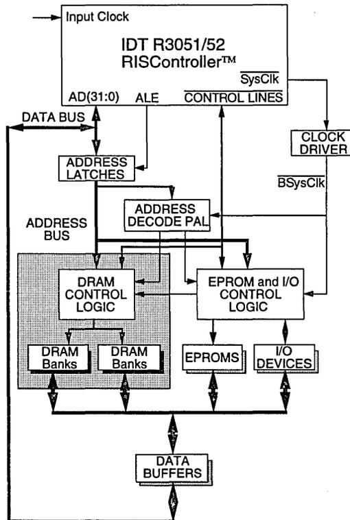
Figure 3. R3051 RISController Family-Based System
