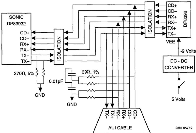
Figure 10. Physical Layer Interface Block Diagram
