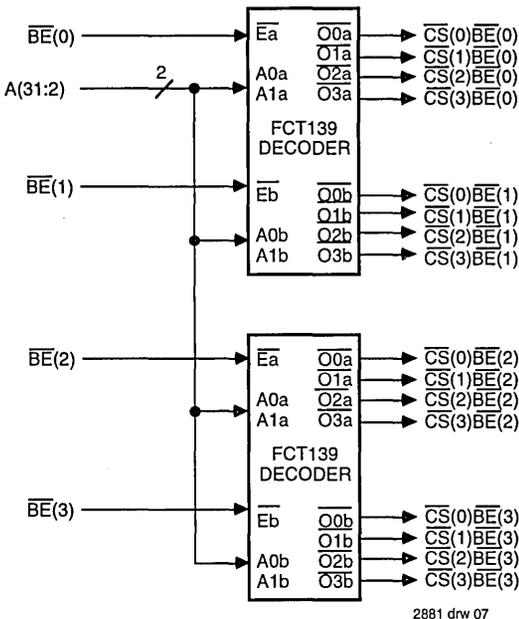
Figure 7. Gating Byte Enables with Chip Selects
