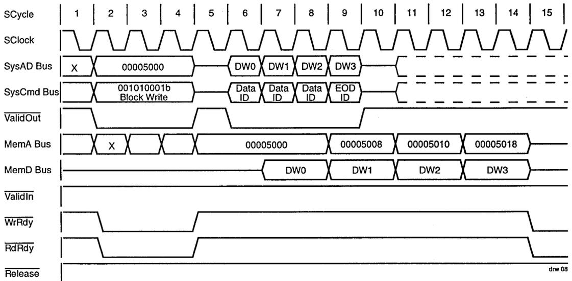
Figure 8. R4000 Write Block Cycle
