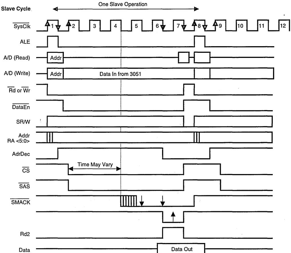
Figure 4. Slave Access Timing Diagram
