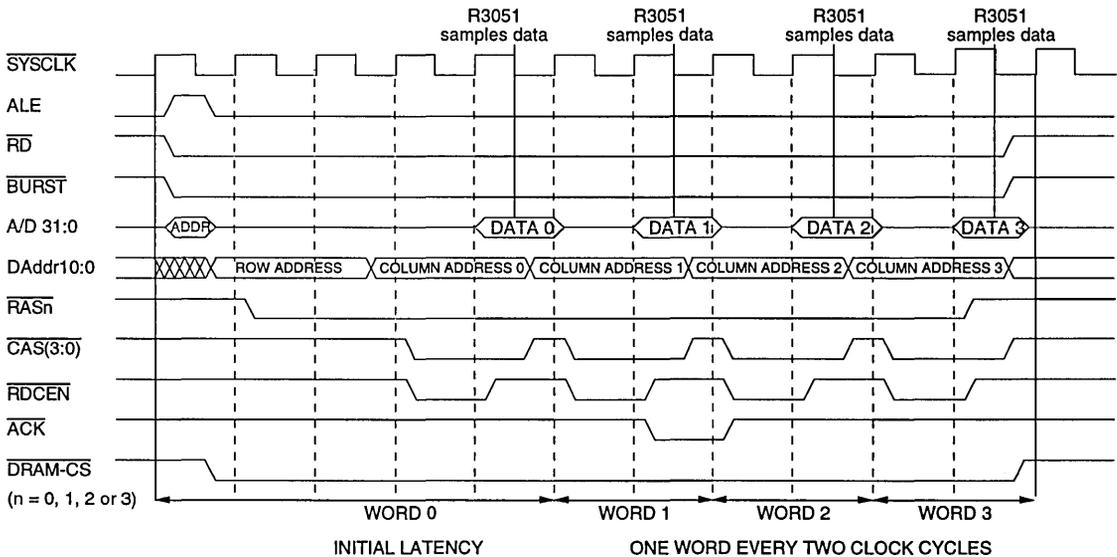
Figure 7. Quad-Word Read Access Timing
