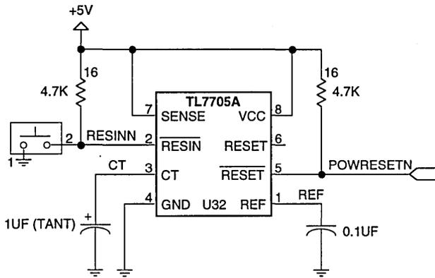
Figure 8. Reset Logic
