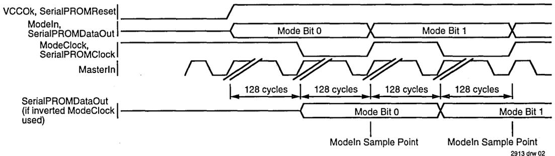
Figure 2. R4000 Serial Initialization Timing
