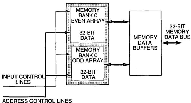
Figure 2. 2-Way Interleaved Single Super Memory Bank
