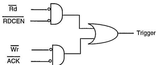
Figure 10. Simple Trigger Logic
