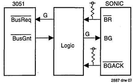
Figure 7. Bus Request Interface Block Diagram
