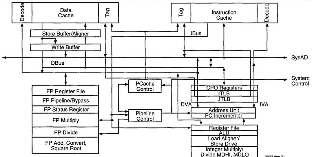
Figure 1. R4000PC Block Diagram
