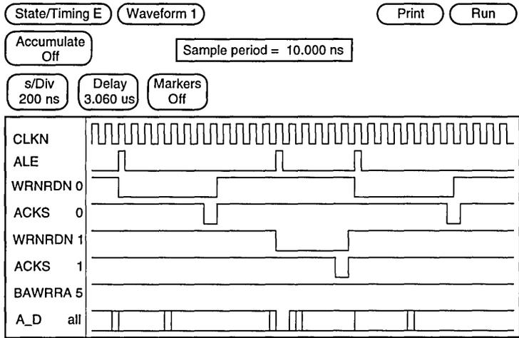
Figure 8. R3051 Timing Mode Waveform
