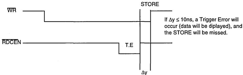
Figure 9.  $\overline{RDCEN}$  Asserted during STORE
