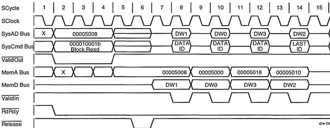
Figure 4. R4000 Block Read Cycle
