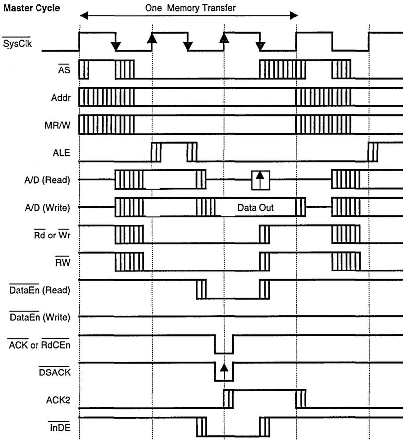
Figure 8. Master Access Timing Diagram
