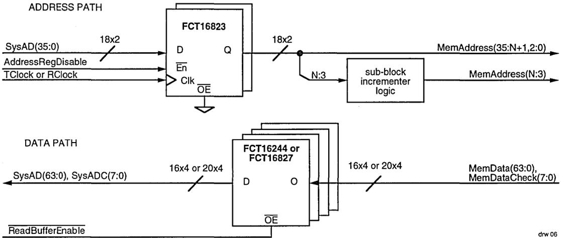
Figure 6. R4000 Single Level Read Buffer
