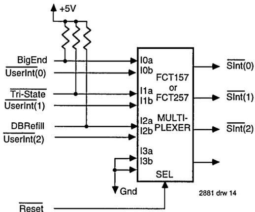
Figure 12. Reset Vector Circuit
