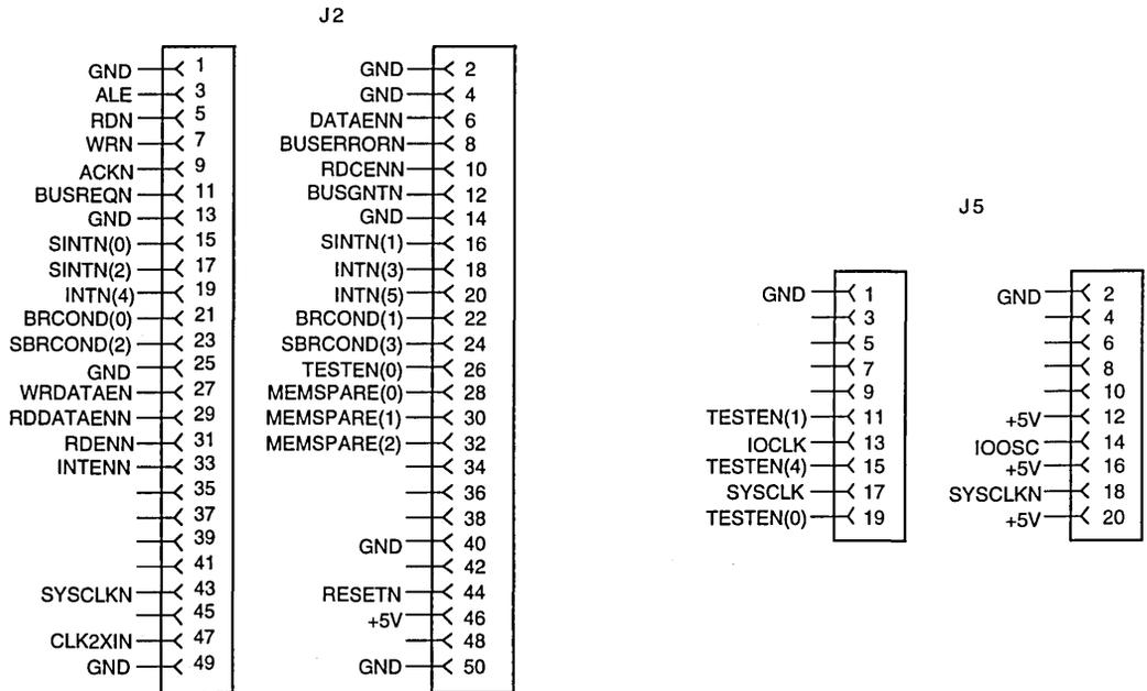
Figure 19. 50-Pin Connector
