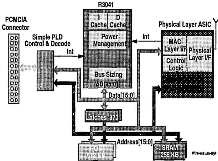
Figure 2. PCMCIA WLAN Adapter Based on the R3041
