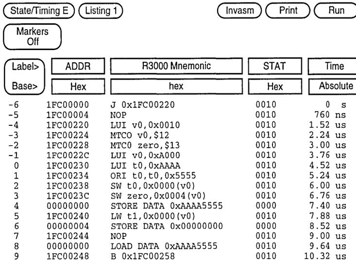
Figure 1. R3051 Address/Data Trace List on a Logic Analyzer
