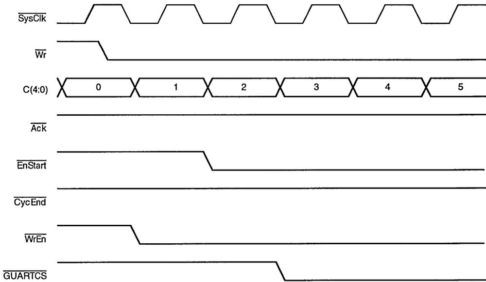
Figure 5. Timing Diagram of Start of GUARTCS
