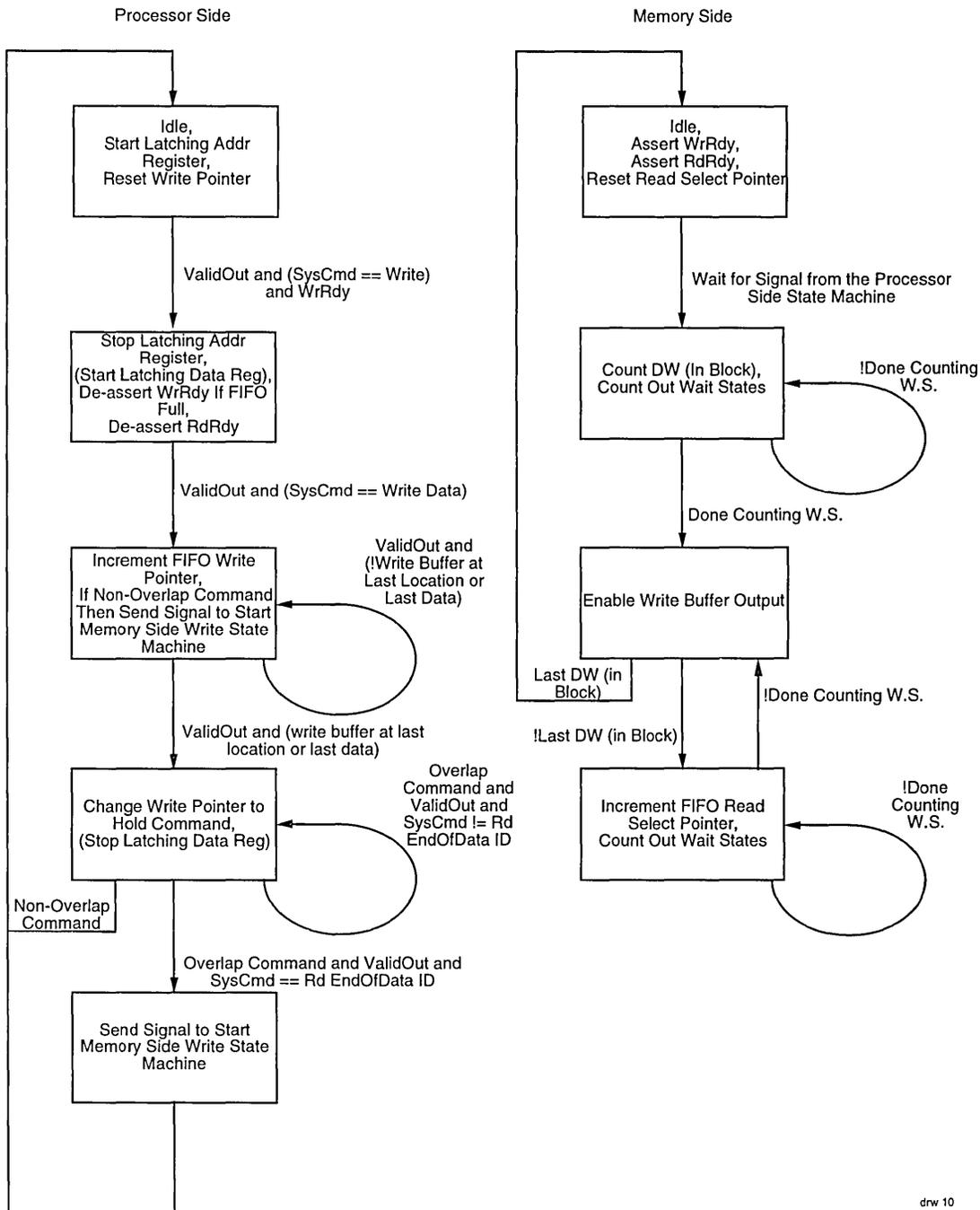
Figure 10. R4000 Write Buffer State Machine
