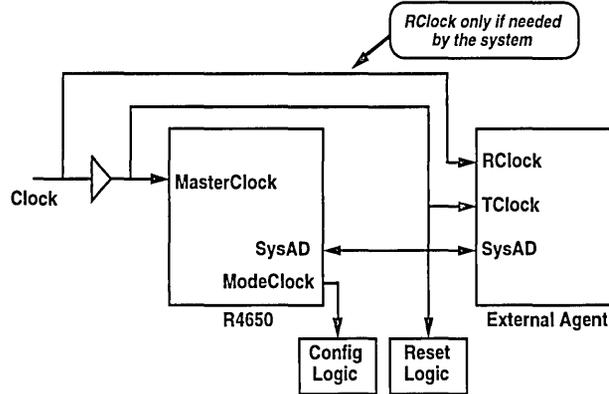
Figure 3. Generating R4600-Compatible Clocks
