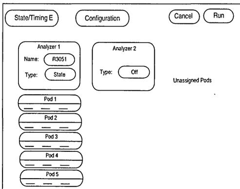
Figure 5. HP16500 State/Timing Mode Display
