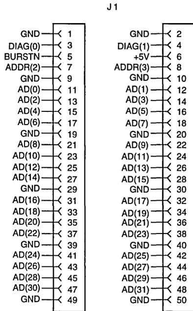
Figure 16. 50-Pin Connector
