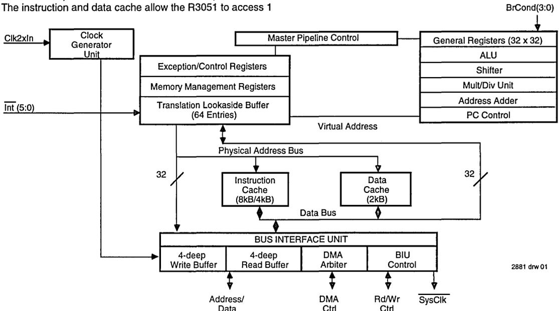
Figure 1. R3051 RISController Internal Architecture
