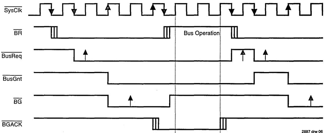
Figure 6. Bus Request Timing Diagram
