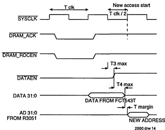
Figure 14. Termination of a Read or Block Refill Access
