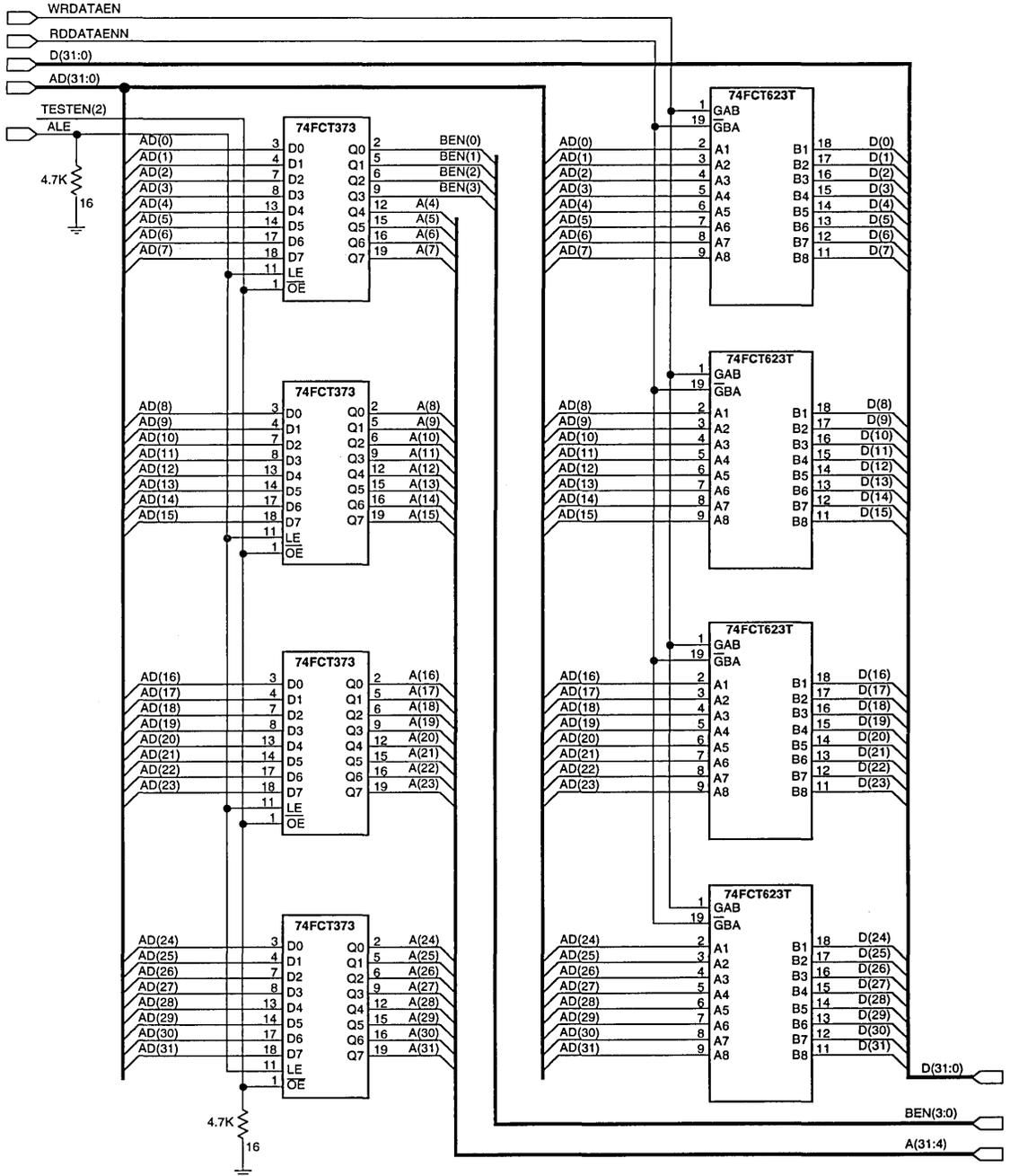
Figure 12. Address Latch Data Transceiver Demultiplexer
