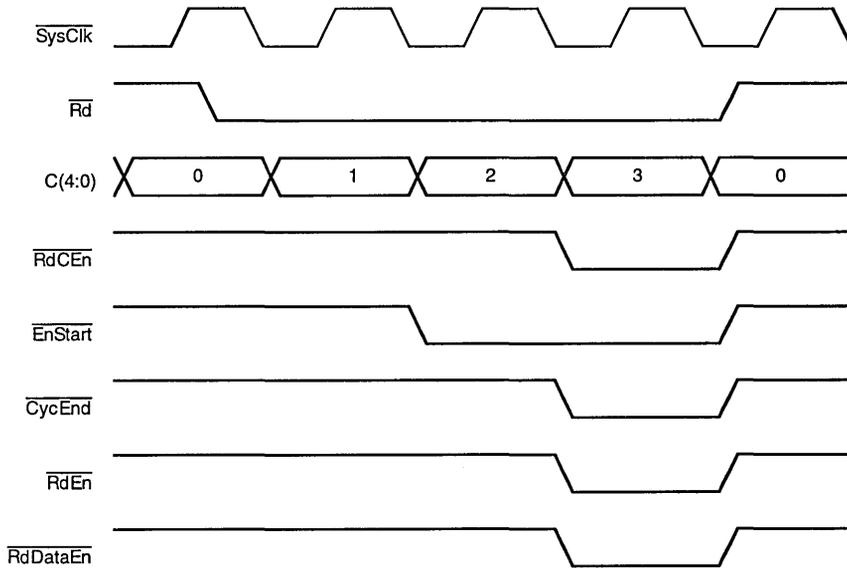
Figure 3. Timing Diagram of  $\overline{\text{RdEn}}$
