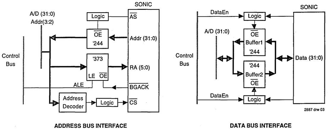
Figure 3. Address and Data Bus Interface
