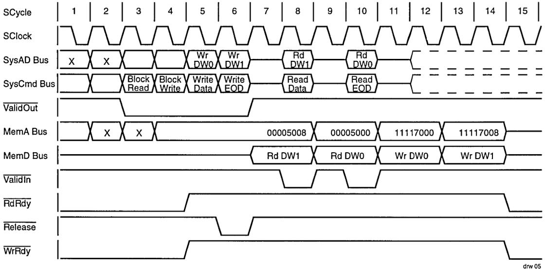
Figure 5. Secondary Cache Overlap Timing
