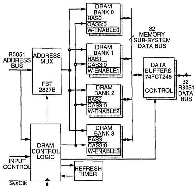
Figure 4. DRAM Memory Subsystem Architecture
