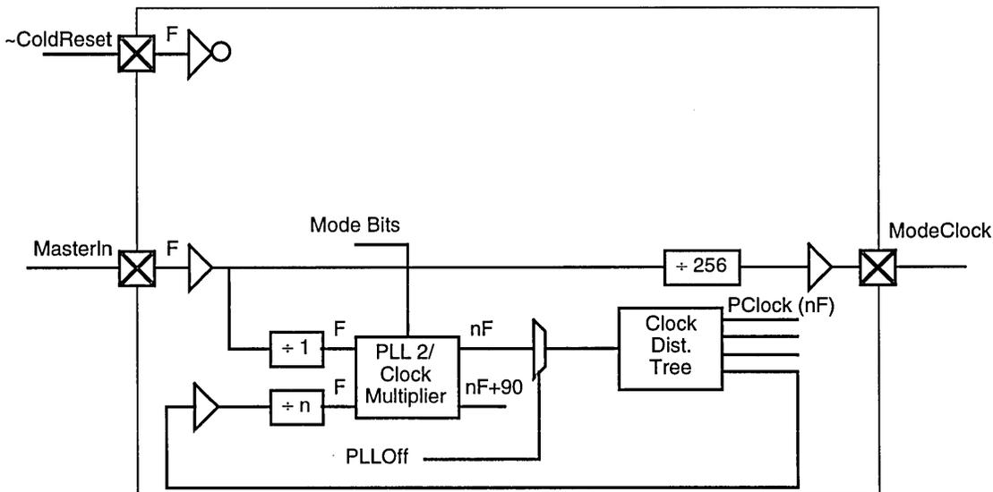
Figure 2. R4650 Clock Distribution Tree and PLL
