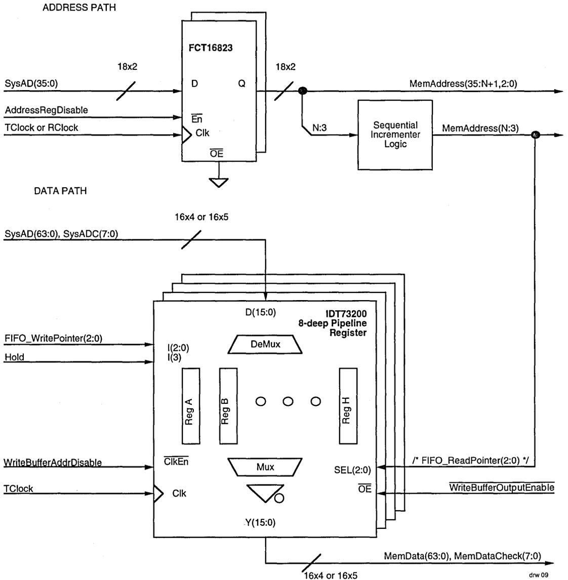
Figure 9. R4000 8-Level, 64-bit Wide Write Buffer
