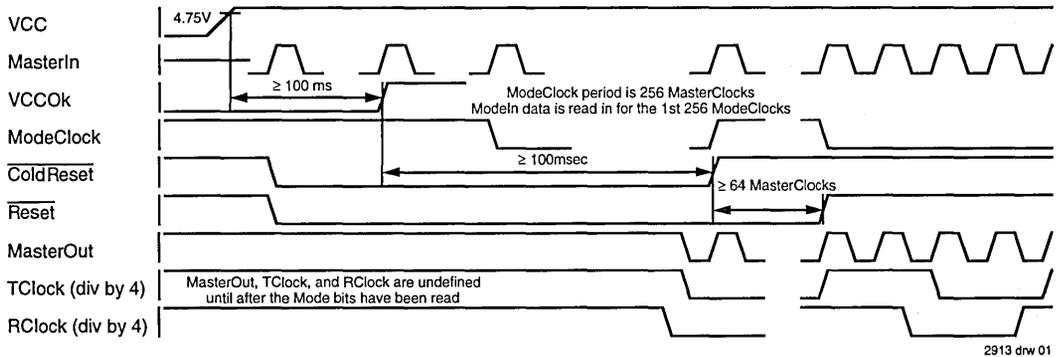
Figure 1. R4000 Reset Timing
