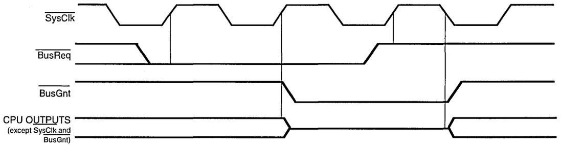
Figure 6. R3051 DMA BusReq and BusGnt Timing
