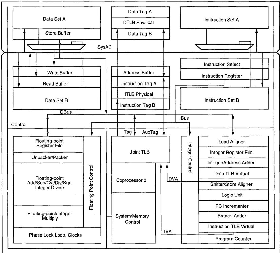
Figure 1. IDT Orion Block Diagram
