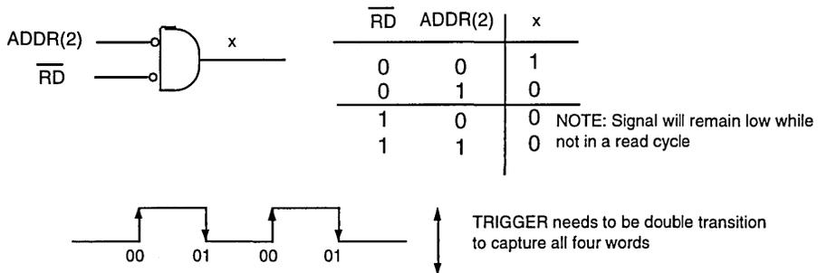
Figure 8. Simulated  $\overline{RDCEN}$  signal
