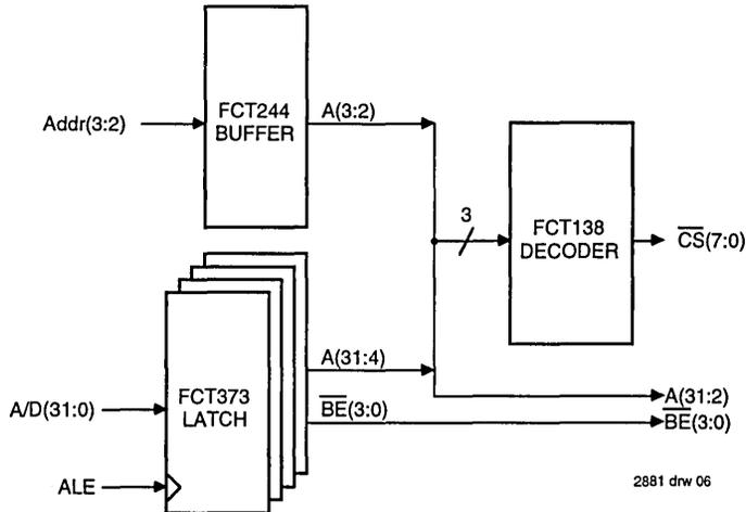
Figure 6. Address De-multiplexer and Decoder
