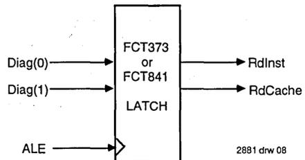
Figure 8. Latching Diag(1:0)
