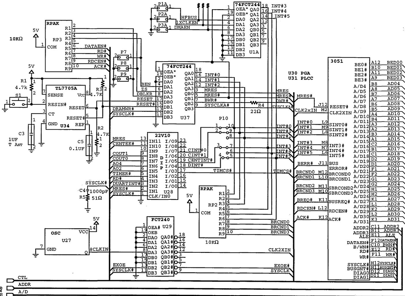
Figure 2. 7RS385 Mode Vector Logic Upgraded for R3081
