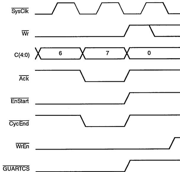
Figure 6. Timing Diagram of End of GUARTCS
