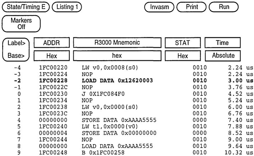
Figure 7. Correctly Synchronized Capture (Note line -2)
