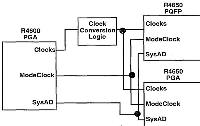
Figure 5. 79S461 Block Diagram
