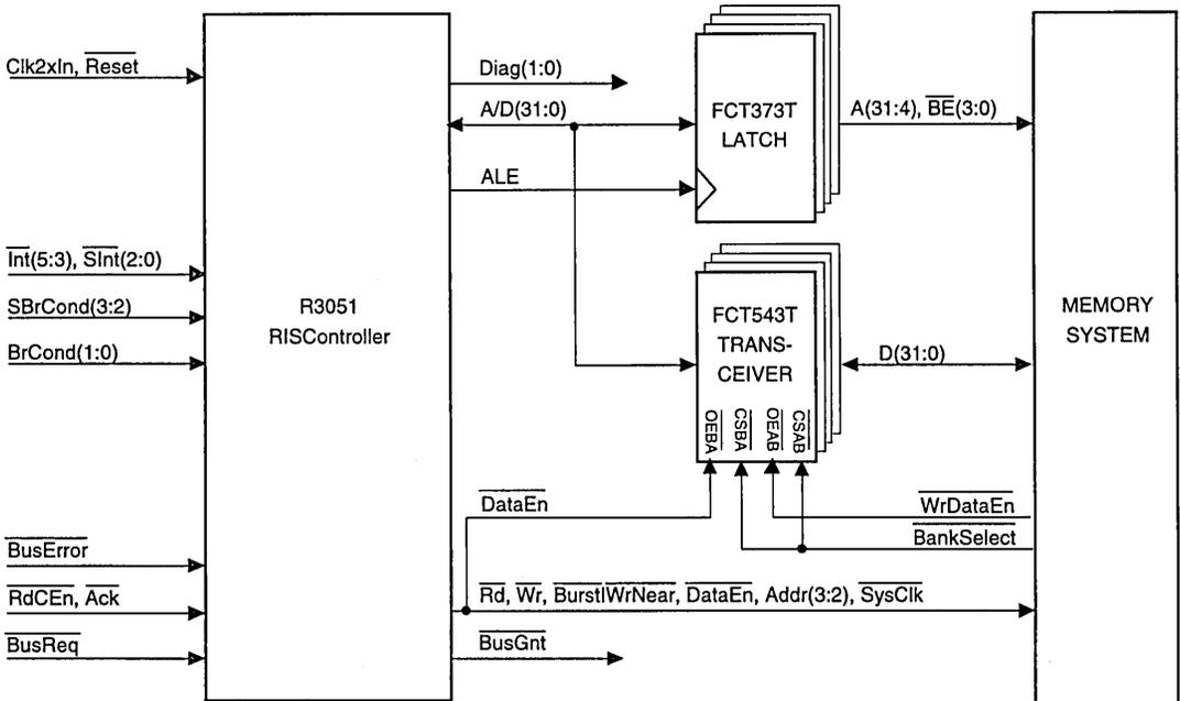
Figure 4. R3051 Memory System Isolated with Transceivers
