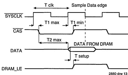
Figure 13. Read or Block Refill Access
