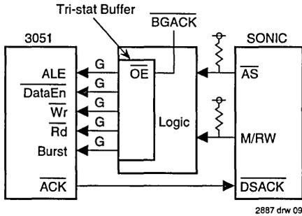
Figure 9. Master Interface Block Diagram
