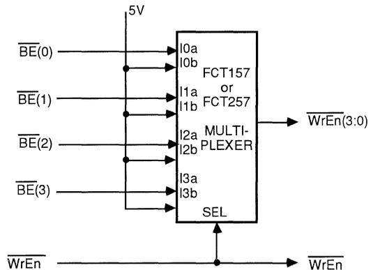
Figure 16. Gating Byte Enables into the Write Enables
