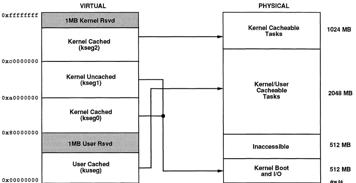
Figure 4. Virtual to Physical Mapping of Base Architecture Versions
