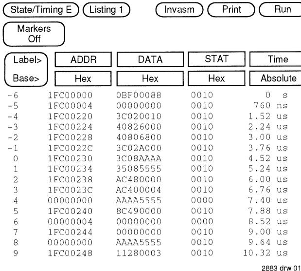
Figure 1. R3051 Address/Data Trace List on a Logic Analyzer
