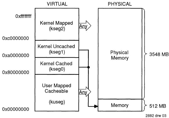
Figure 3. Virtual to Physical Memory Mapping of R3000 Architecture
