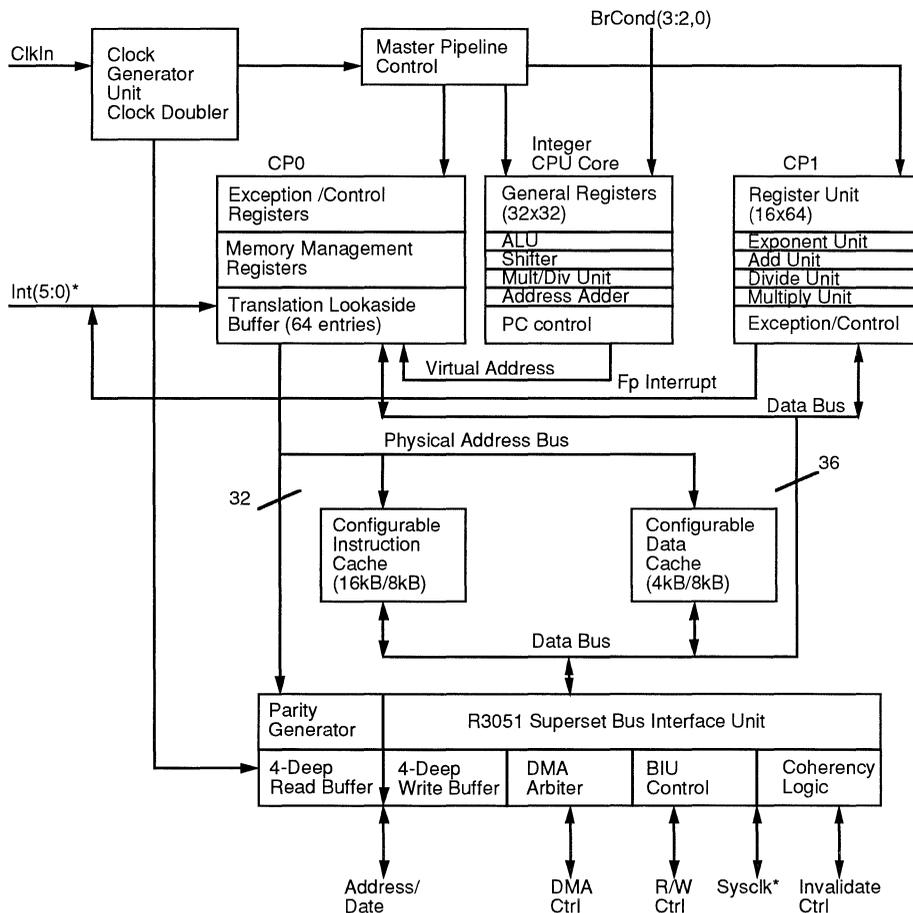
Figure 1. The IDT79R3081 Block Diagram
