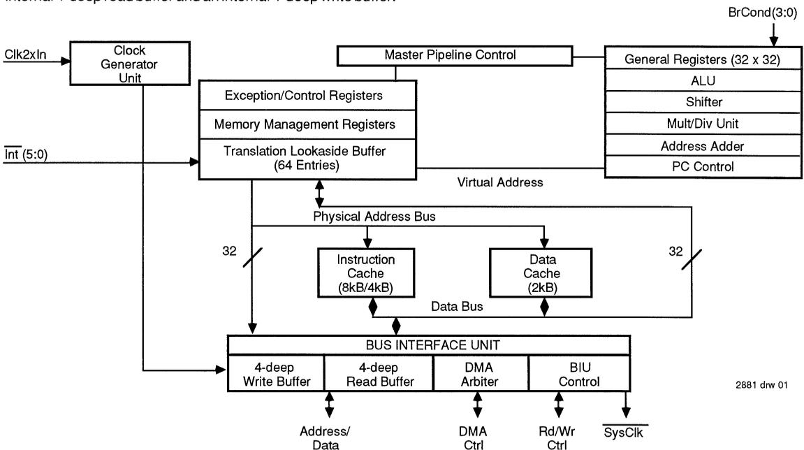
Figure 1. R3051 RISController Internal Architecture
