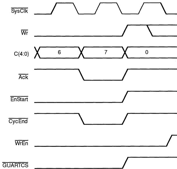
Figure 6. Timing Diagram of End of  $\overline{\text{GUARTCS}}$
