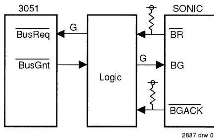
Figure 7. Bus Request Interface Block Diagram
