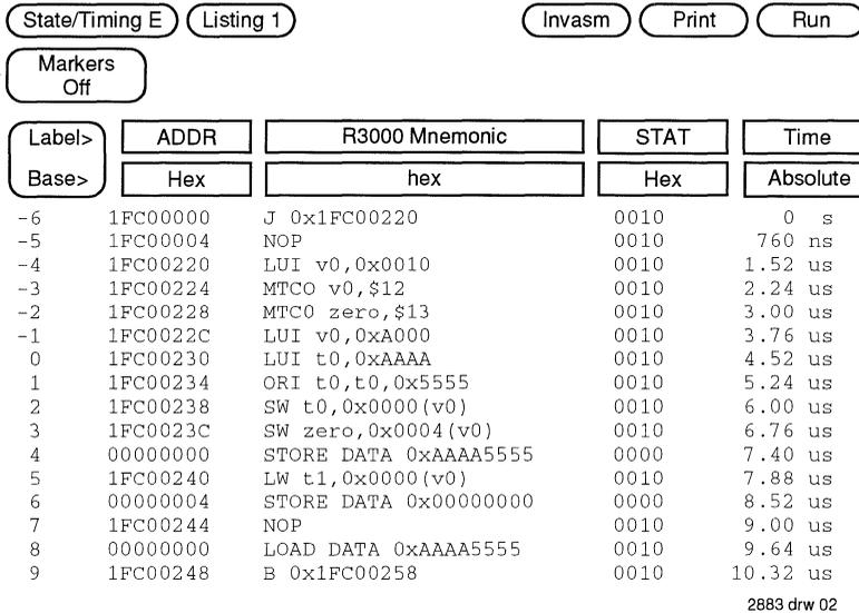
Figure 2. R3051 Instruction Disassembly on the HP16500 Logic Analyzer
