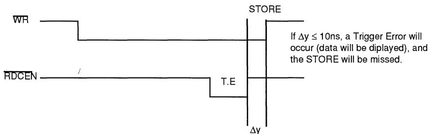
Figure 9.  $\overline{RDCEN}$  Asserted during STORE
