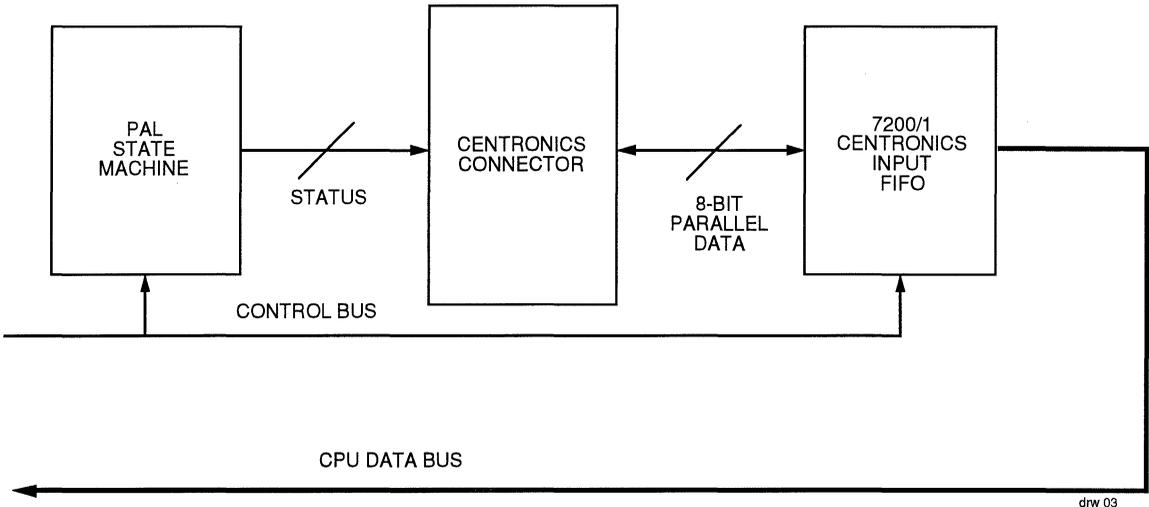
Figure 3. Centronics Interface Block Diagram
