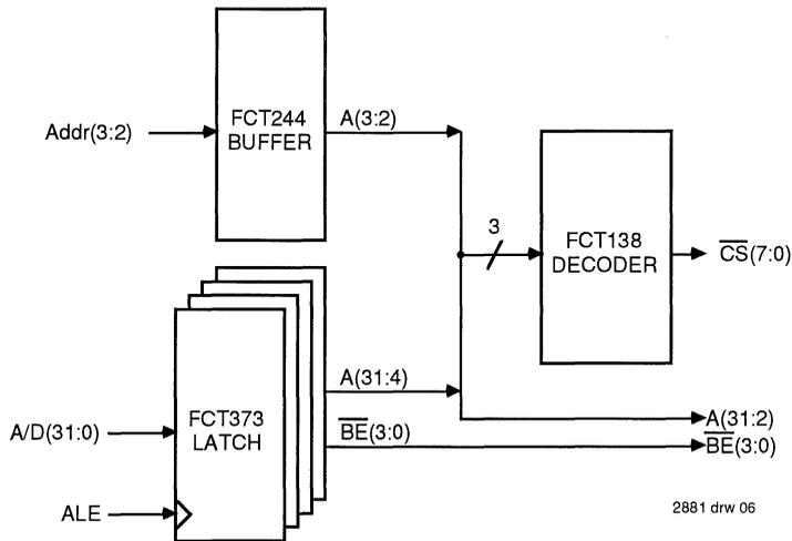
Figure 6. Address Demultiplexer and Decoder
