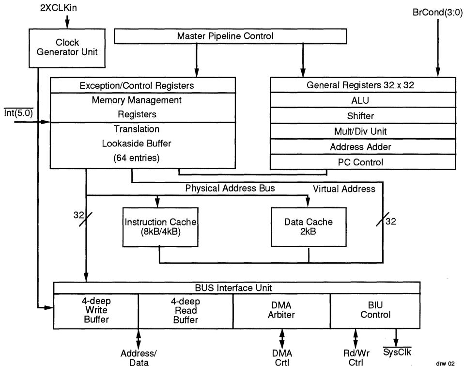
Figure 2. The R3051 RISController
