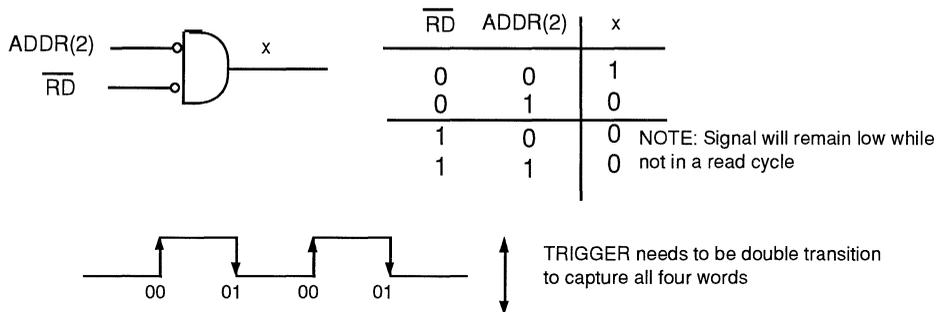
Figure 8. Simulated  $\overline{RDCEN}$  signal
