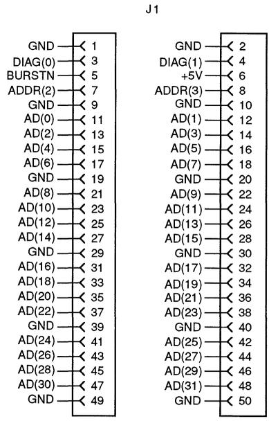
Figure 16. 50-Pin Connector
