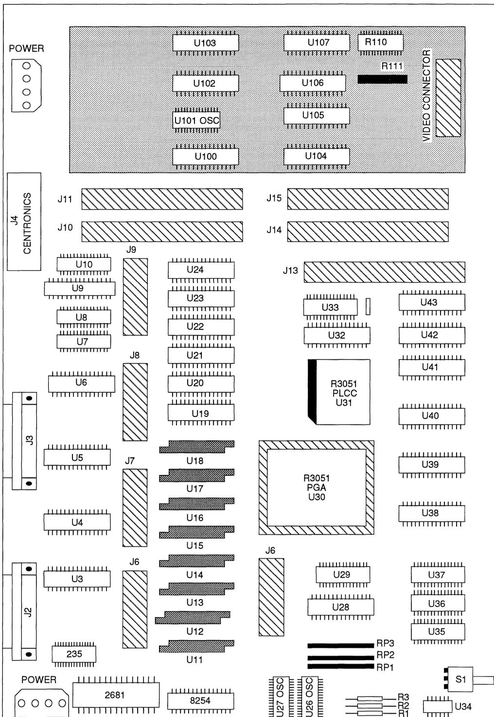
Figure 4. The Physical Layout of the IDT7RS385-LPC
