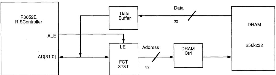
Figure 1. Simplified Block Diagram of 7RS385 DRAM Subsystem
