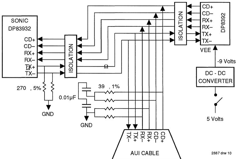
Figure 10. Physical Layer Interface Block Diagram
