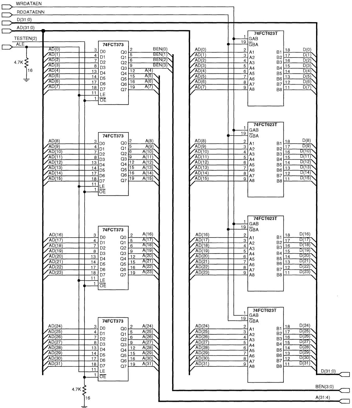
Figure 12. Address Latch Data Transceiver Demultiplexer
