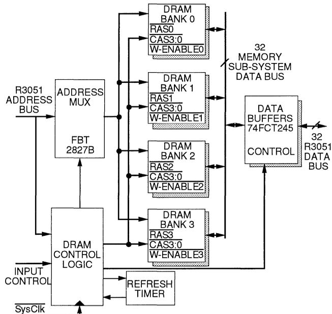
Figure 4. DRAM Memory Subsystem Architecture
