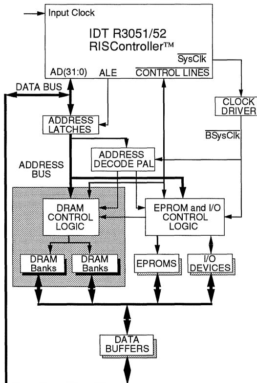
Figure 3. R3051 RISController Family-Based System
