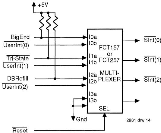
Figure 12. Reset Vector Circuit
