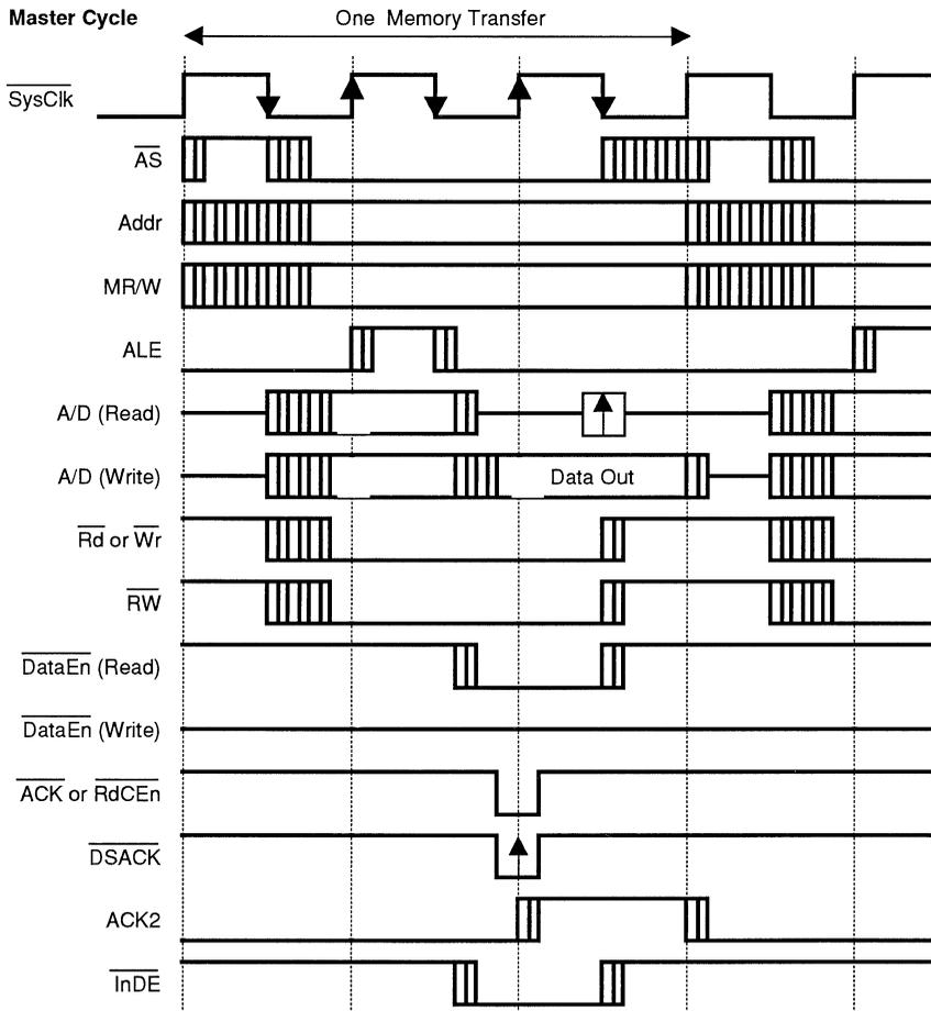
Figure 8. Master Access Timing Diagram
