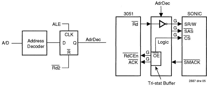
Figure 5. Slave Interface Block Diagram
