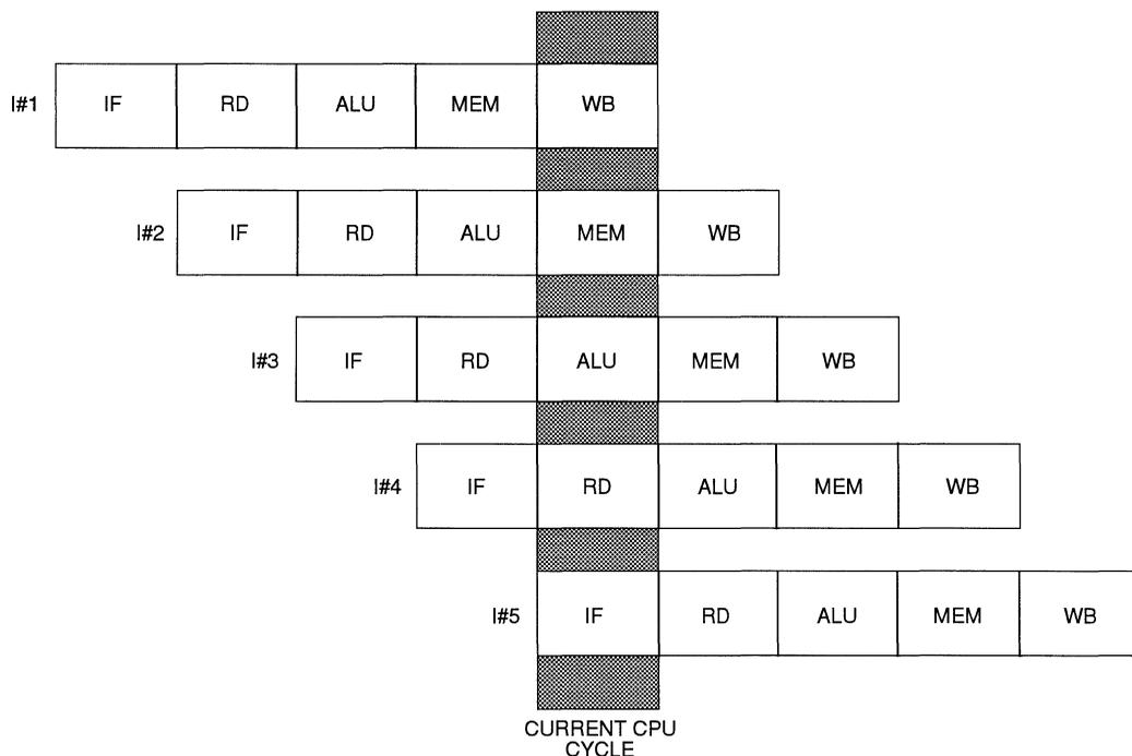
Figure 2. R3081 5-Stage Pipeline
