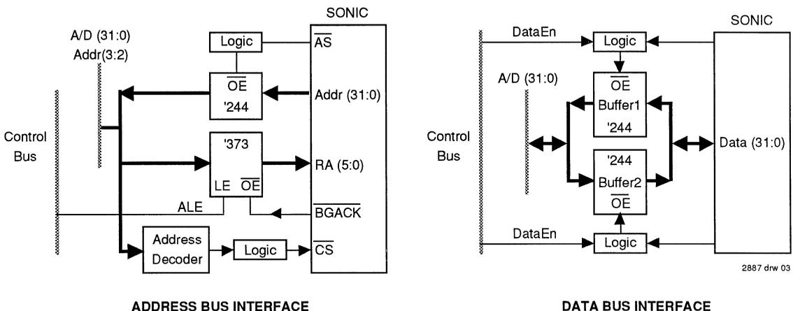
Figure 3. Address and Data Bus Interface
