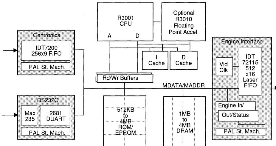
Figure 2. REAL8 Laser Printer Controller Block Diagram
