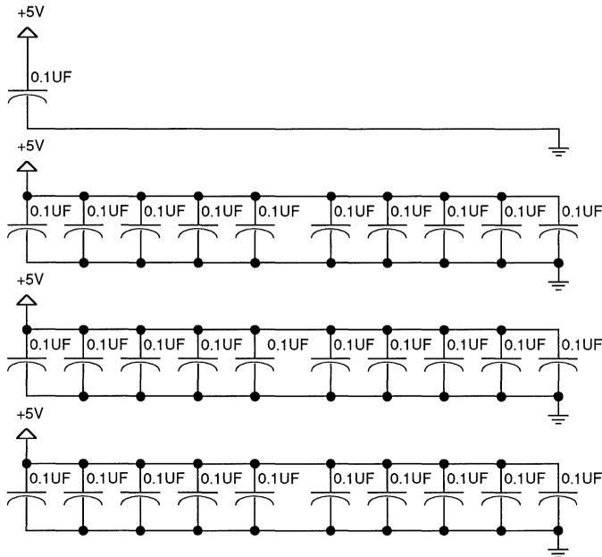
Figure 21. Decoupling Capacitors
