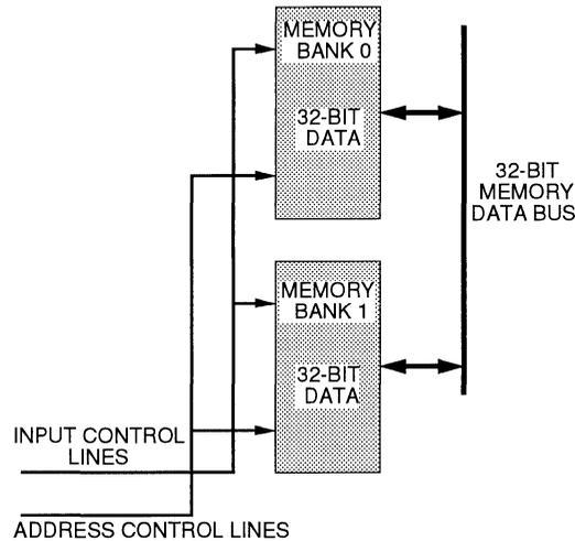
**Figure 1b. Two-Bank Non-Interleaved System**
