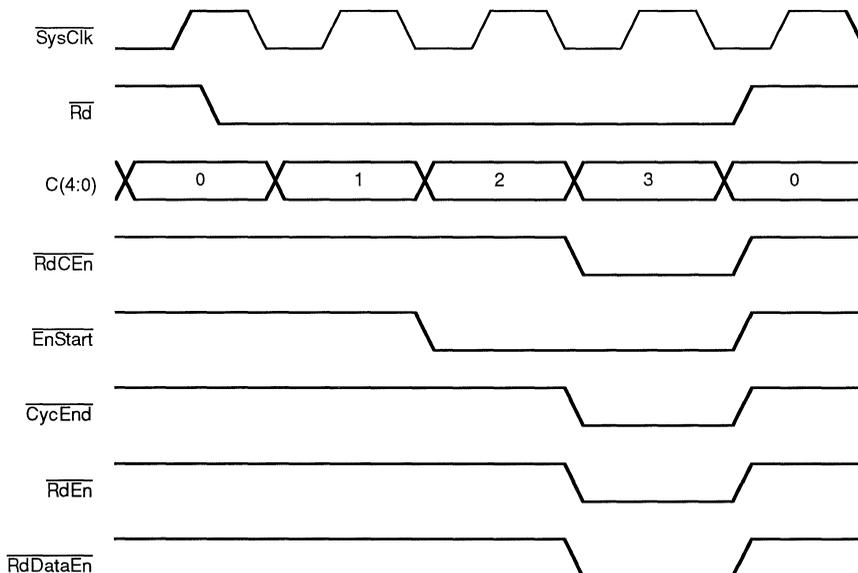
Figure 3. Timing Diagram of RdEn
