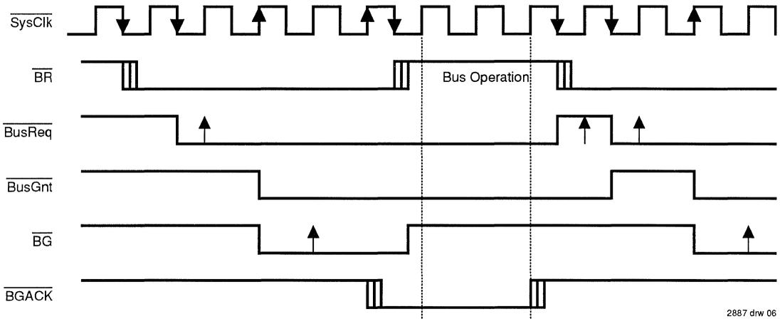
Figure 6. Bus Request Timing Diagram
