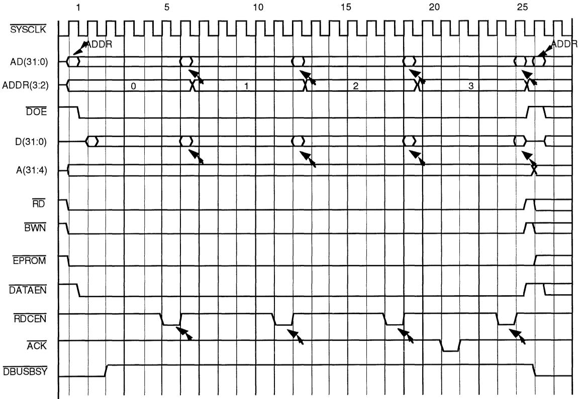
Figure 8. EPROM Quad-Word Read on 7RS385 Board
