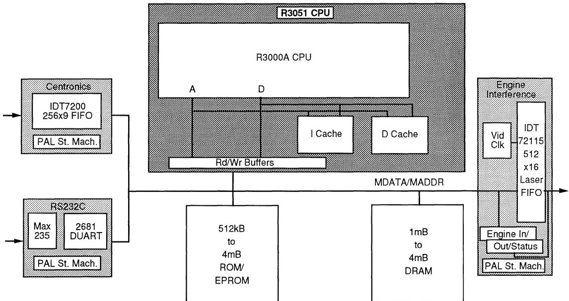
Figure 2. Block Diagram of Laser Printer Controller
