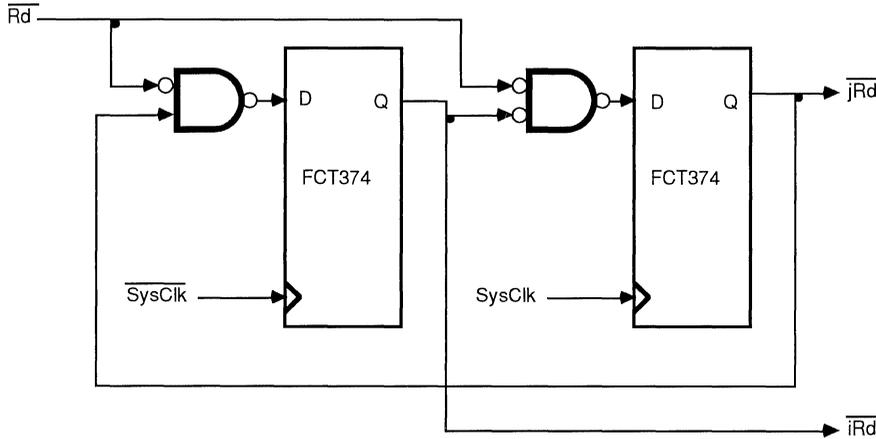
Figure 15. Using Interlocked Registers
