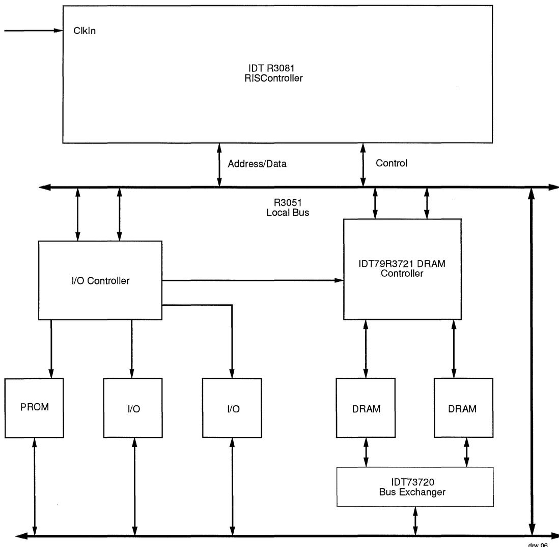
Figure 6. R3081 RISChipset Based System
