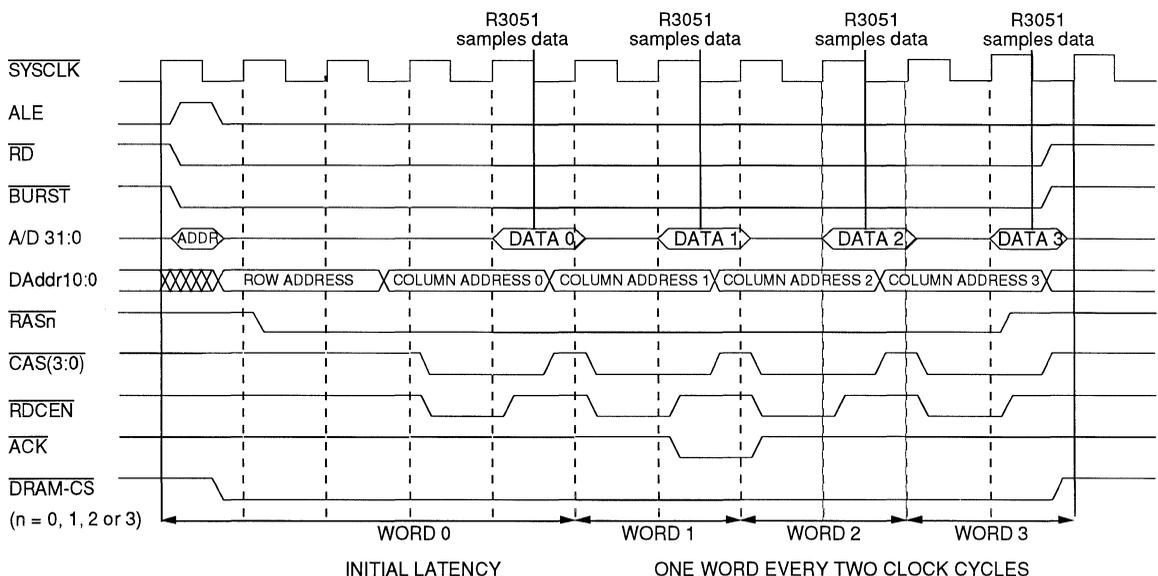
Figure 7. Quad-Word Read Access Timing
