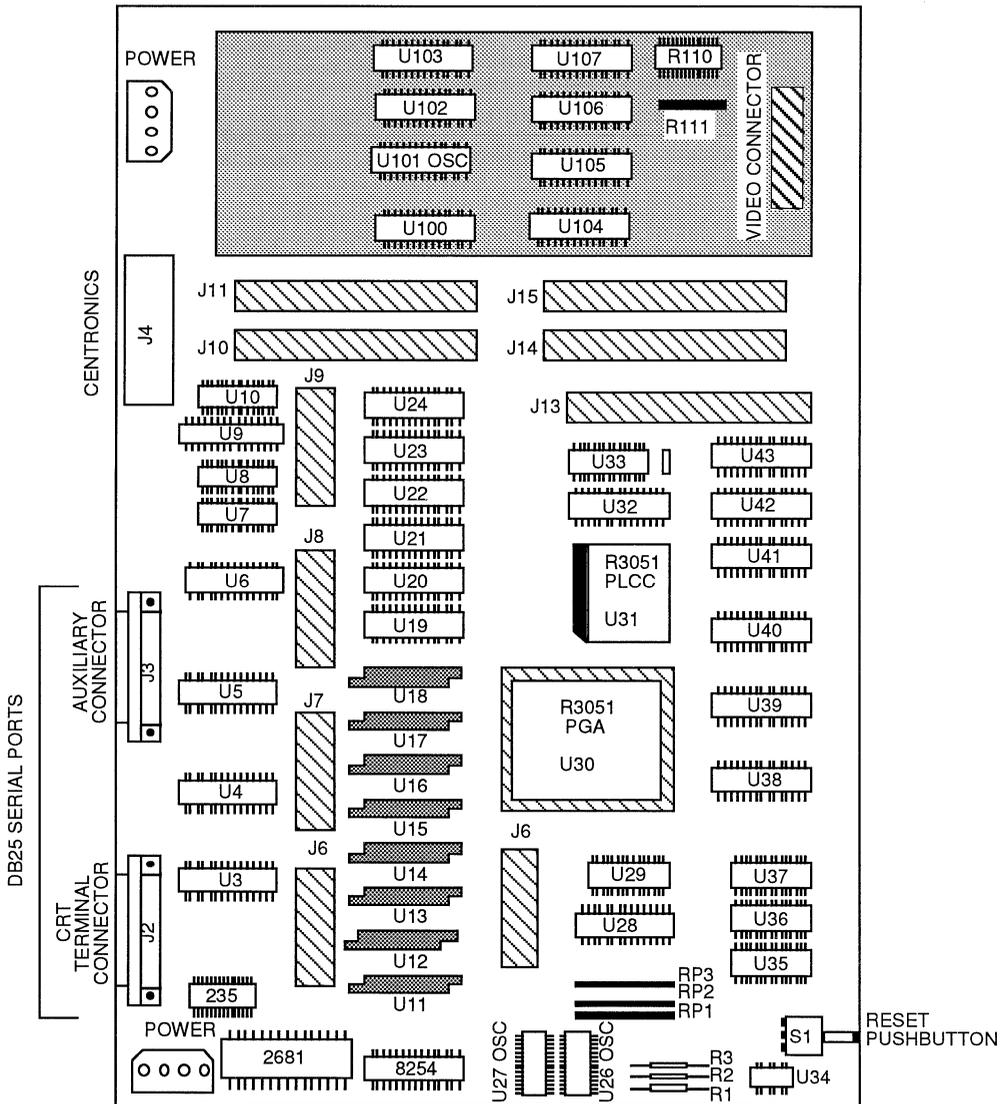
Figure 6. The Physical Layout of the 7RS385\_REAL8 Emulation
