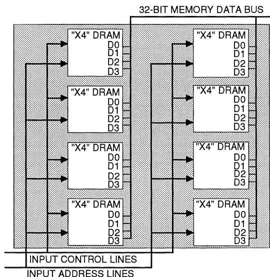
Figure 1a. Single-Bank Non-Interleaved System
