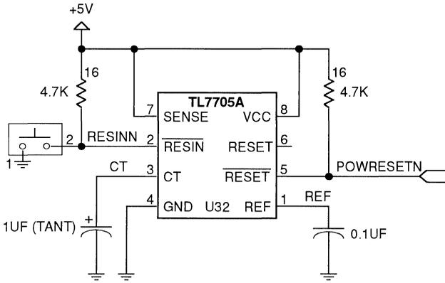
Figure 8. Reset Logic
