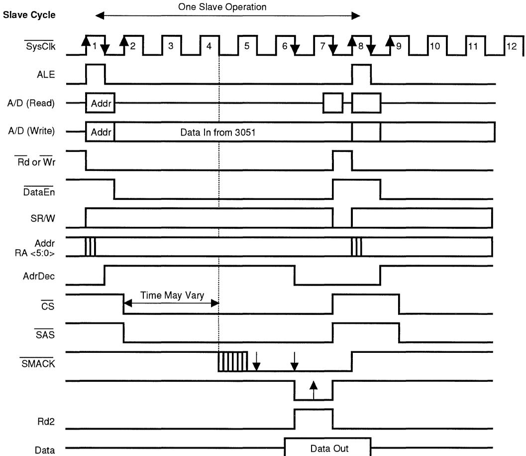
Figure 4. Slave Access Timing Diagram
