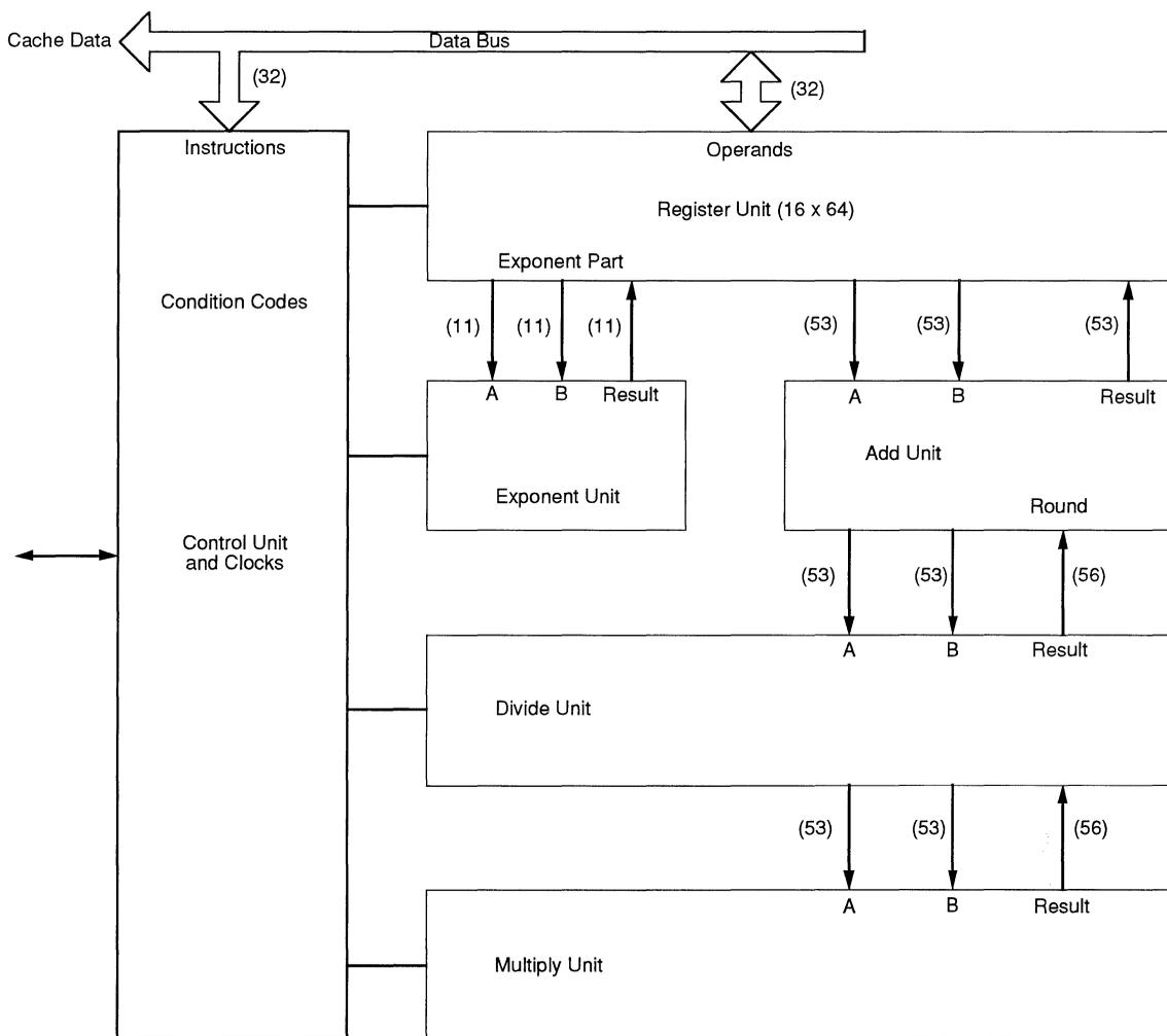
Figure 5. FPA Functional Block Diagram
