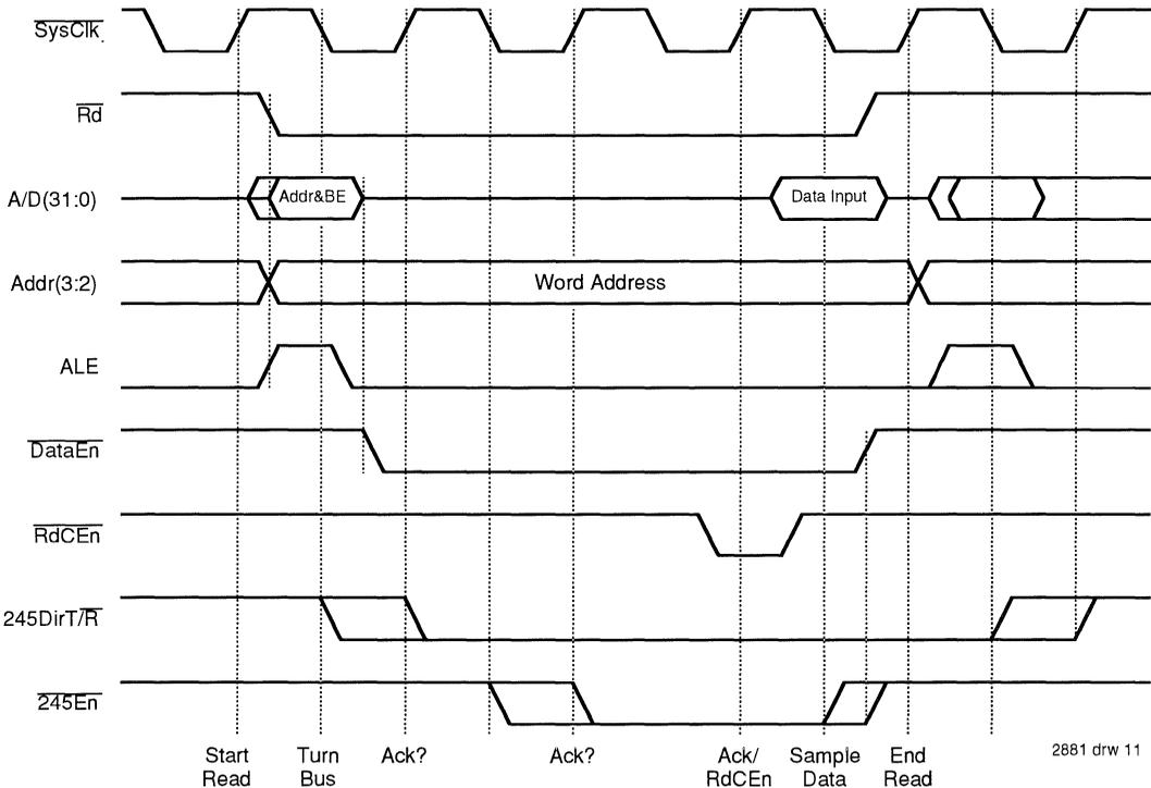
Figure 10a. Timing Diagram of FCT245 Enable and T/R Direction Controls for a Read
