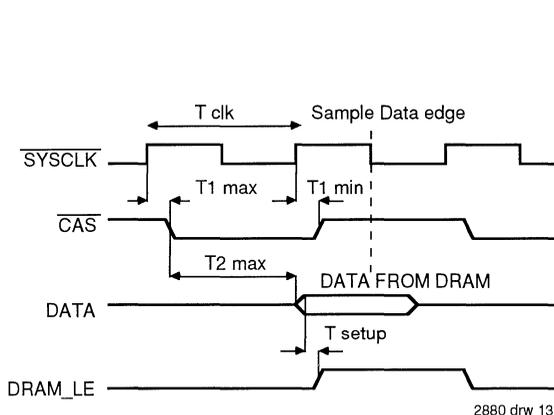
Figure 13. Read or Block Refill Access
