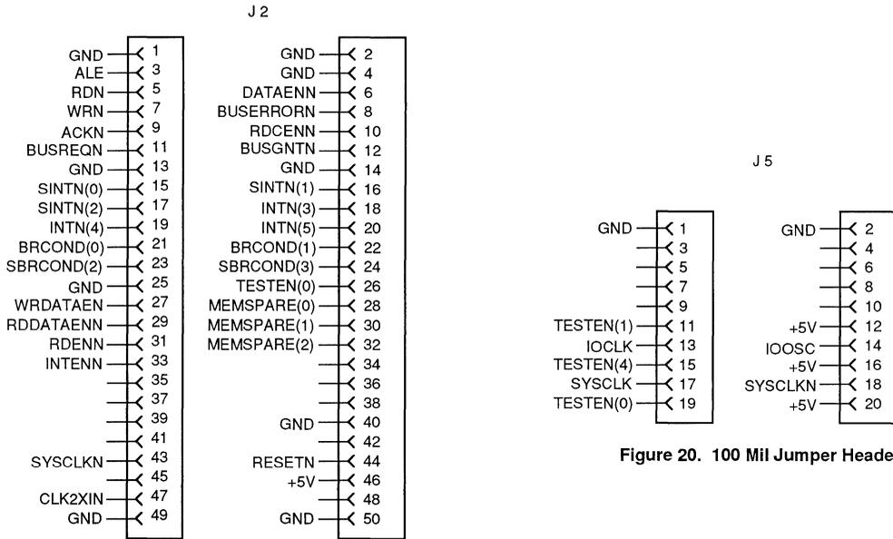
Figure 19. 50-Pin Connector
