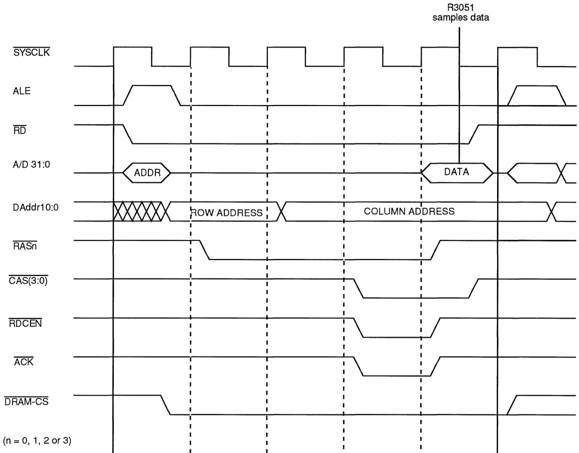
Figure 6. Single-Word Read Access Timing
