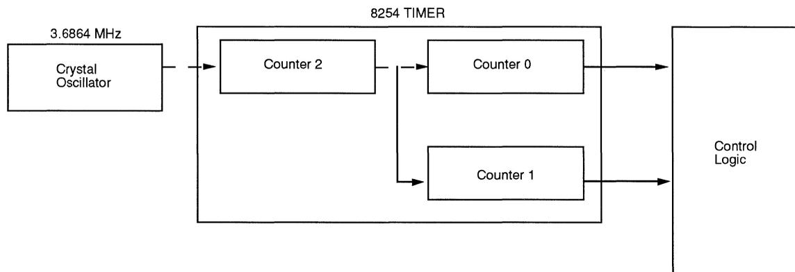
Figure 1. Block Diagram of Timer Function on 7RS385
