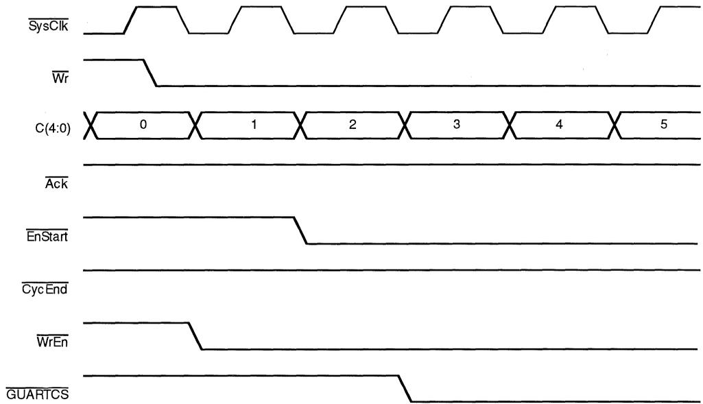
Figure 5. Timing Diagram of Start of  $\overline{\text{GUARTCS}}$
