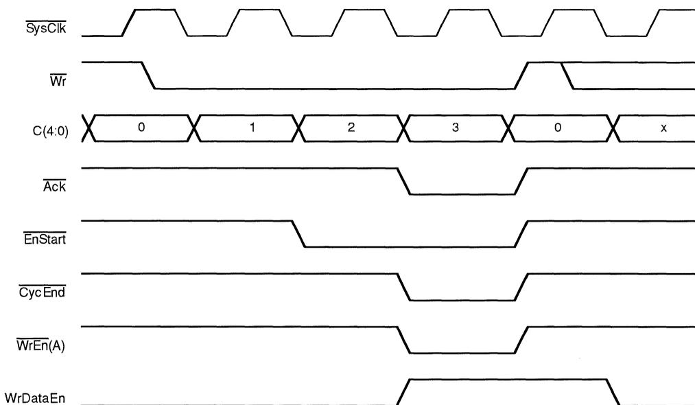
Figure 4. Timing Diagram of WrEn(A)
