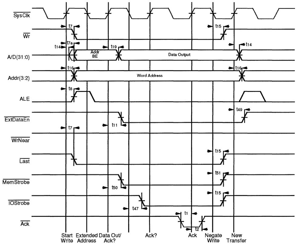
Figure 9.7. Basic 32-Bit Port Write with Wait Cycles
