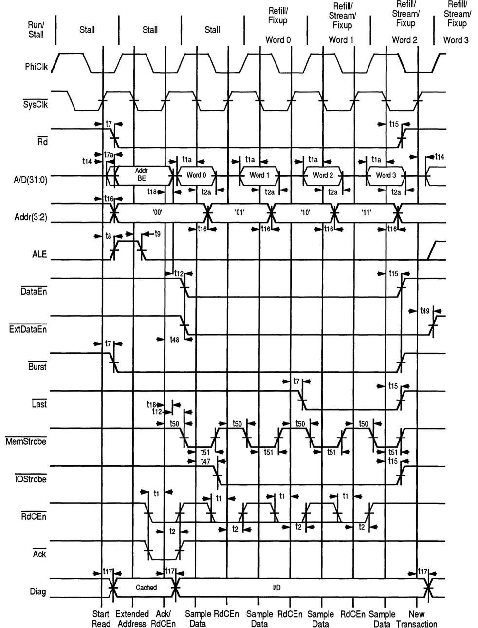
**Figure 8.11. Burst Read With No Wait Cycles**
