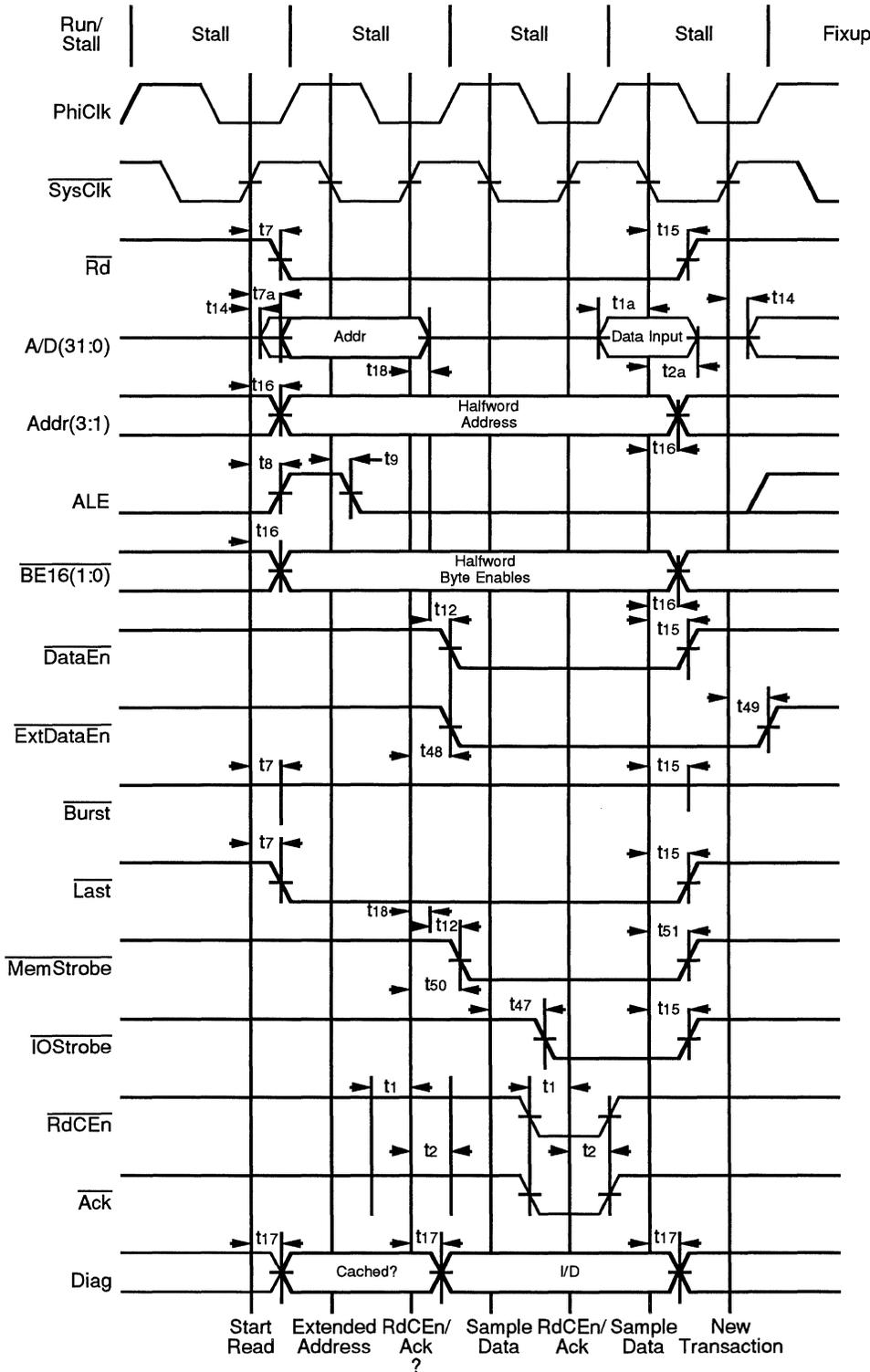
Figure 8.17. Single Halfword Read With Bus Wait Cycle
