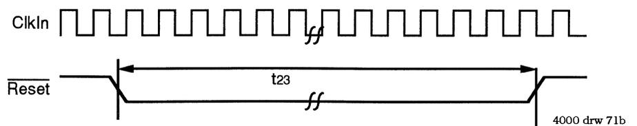
Figure 11.3. Warm Reset when using Internal Pull-Ups
