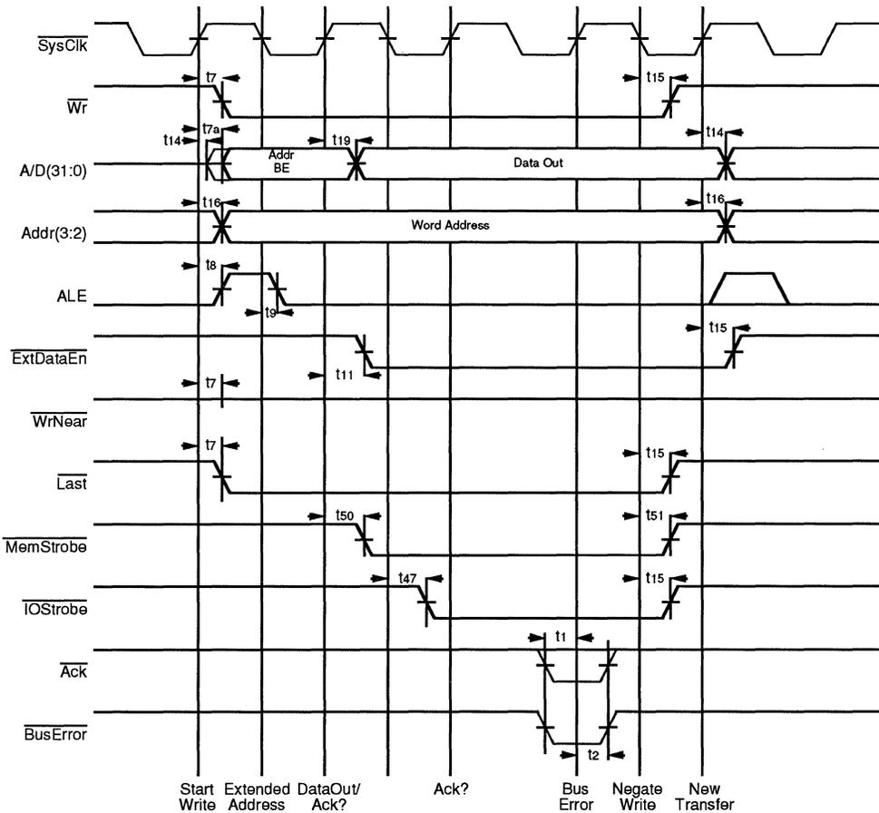
**Figure 9.8. Basic Write Terminated by Bus Error**
