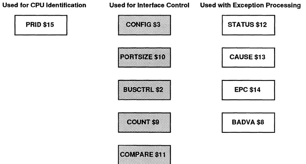
Figure 5.1. R3041 Bus Interface Control Registers
