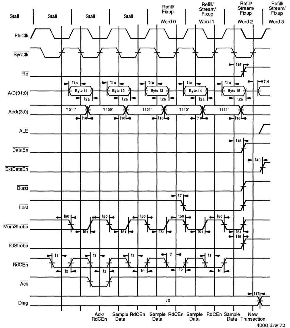
Figure 8.25 (b). End of 16 Byte Burst Read Without Bus Wait Cycles
