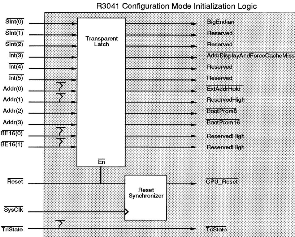
**Figure 11.4. Configuration Mode Initialization Logic**
