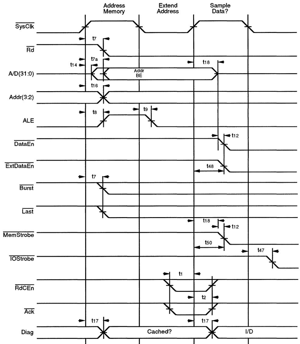
Figure 8.3. Start of Bus Read Operation with Extended Address Hold
