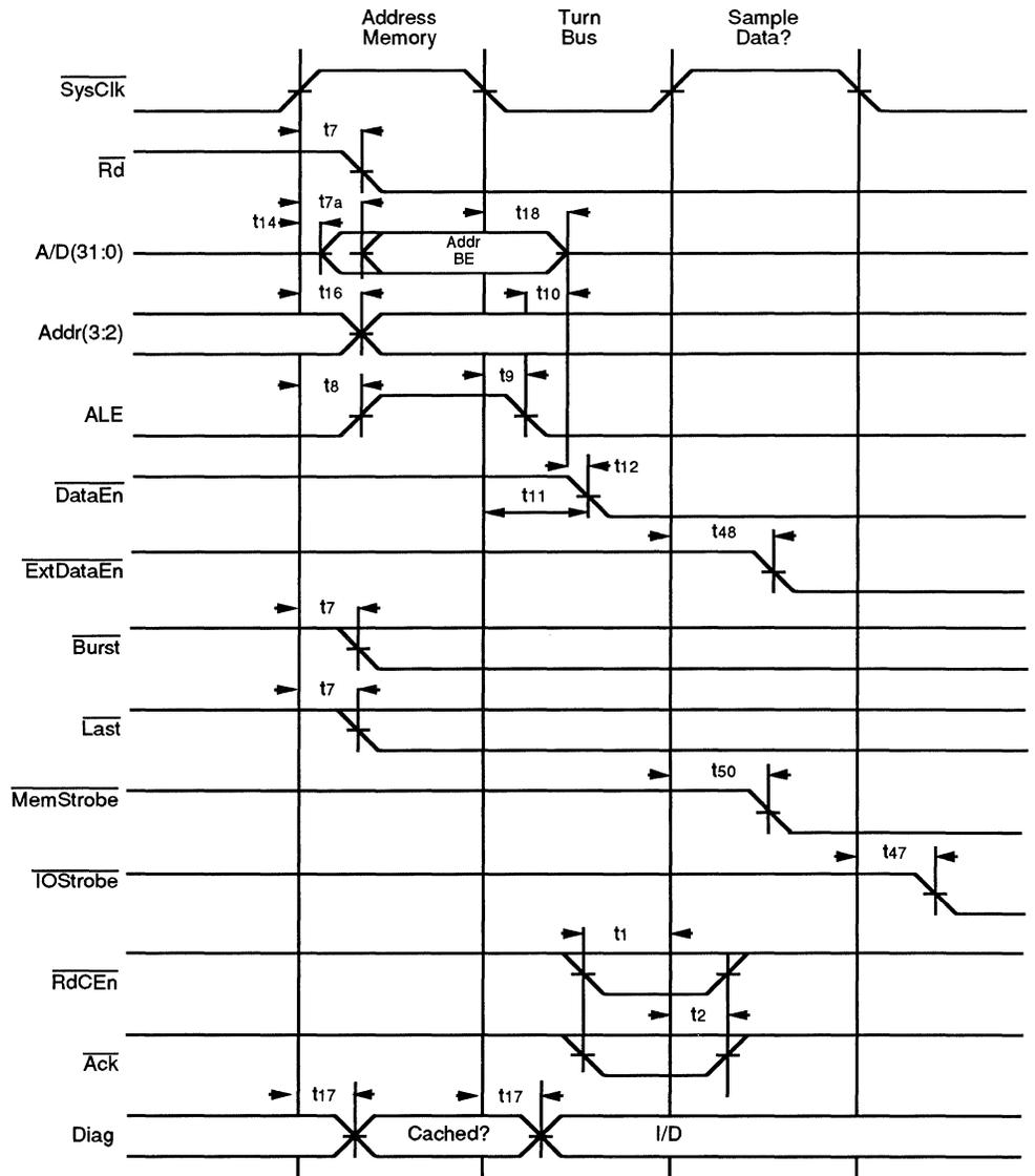
**Figure 8.2. Start of Bus Read Operation Without Extended Address Hold**
