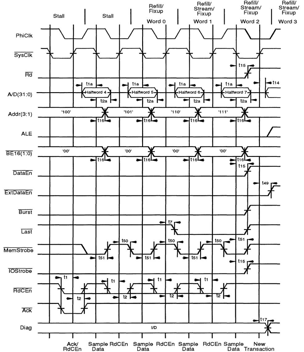
Figure 8.19(b). End of Burst Block Halfword Read Without Bus Wait Cycles
