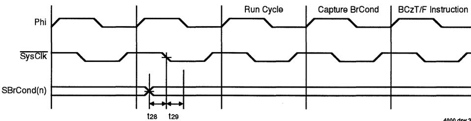
Figure 6.8. Synchronized BrCond Inputs
