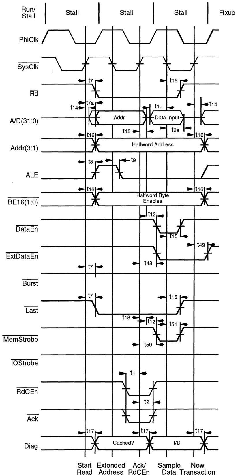
Figure 8.16. Single Halfword Read Without Bus Wait Cycles
