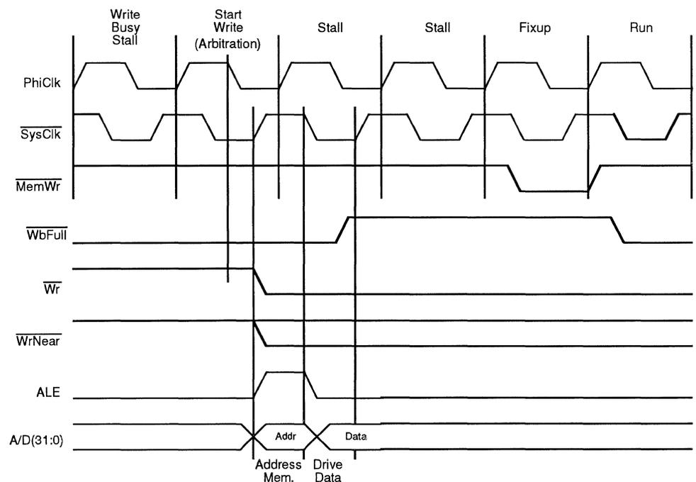
Figure 9.5. Write Buffer Full Operation
