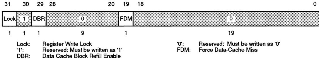
Figure 5.4. R3041 Cache Configuration Register
