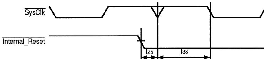
Figure 12.2. R3041 SysClk Phase Initialization Case A
