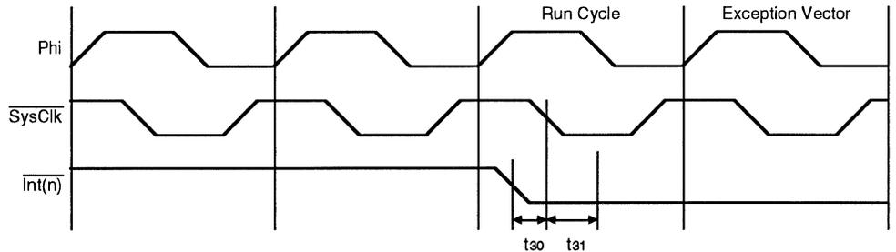
**Figure 6.7. Direct Interrupt Operation**
