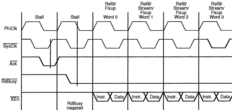
Figure 8.7. Internal Processor States on Burst Read
