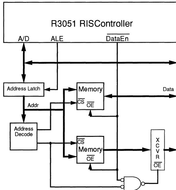
**Figure 8.6. Use of  $\overline{\text{DataEn}}$  as Output Enable Control**
