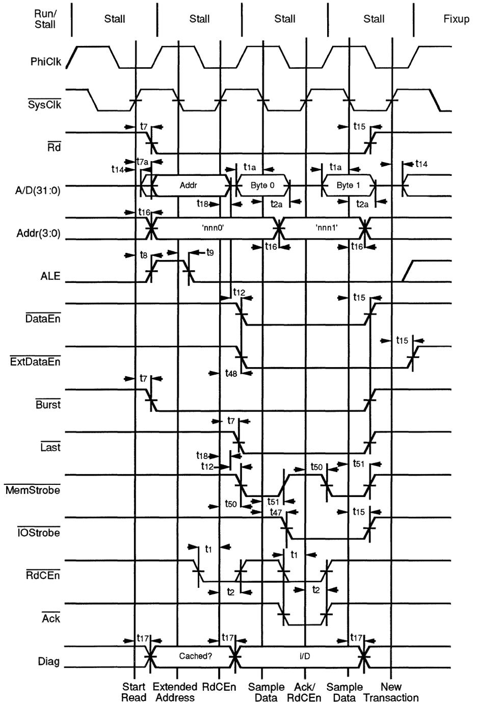
**Figure 8.22. Double Byte Read Without Bus Wait Cycles**
