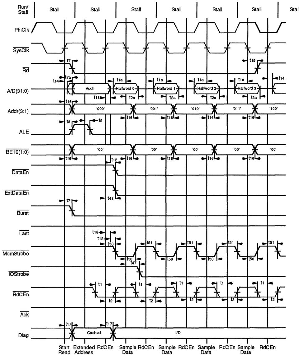
**Figure 8.19(a). Start of Burst Block Halfword Read Without Bus Wait Cycles**
