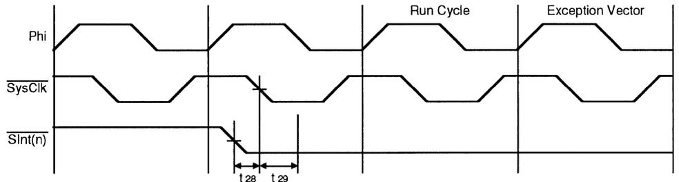
**Figure 6.6. Synchronized Interrupt Operation**
