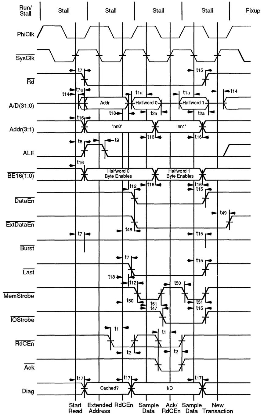
**Figure 8.18. Mini-Burst Halfword Read Without Bus Wait Cycles**
