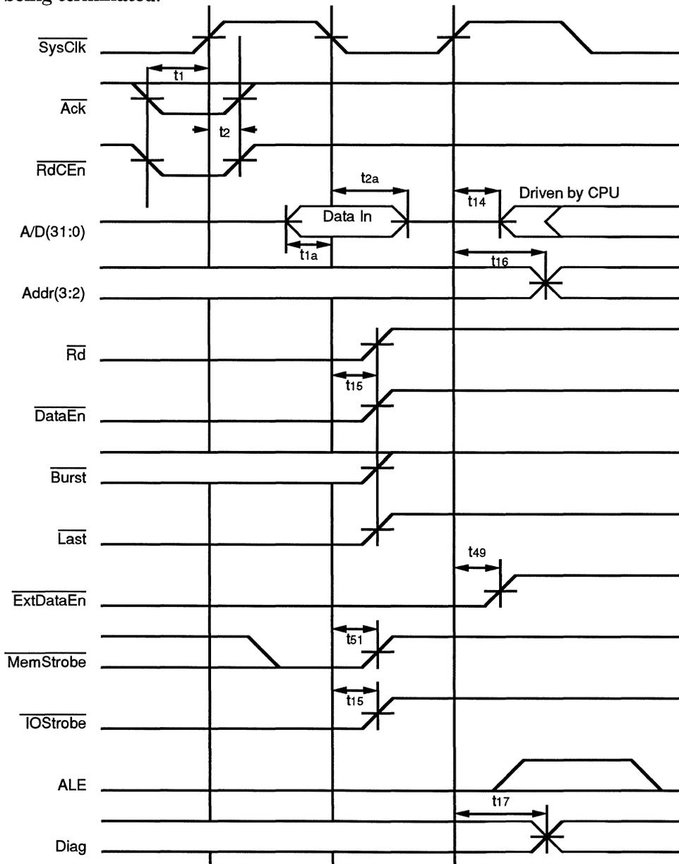
Figure 8.5. Read Cycle Termination
