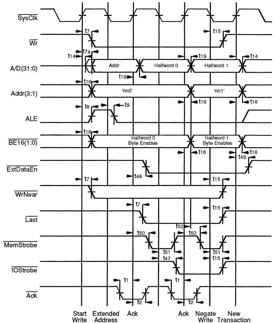
Figure 9.11. Mini-Burst 16-Bit Port Write
