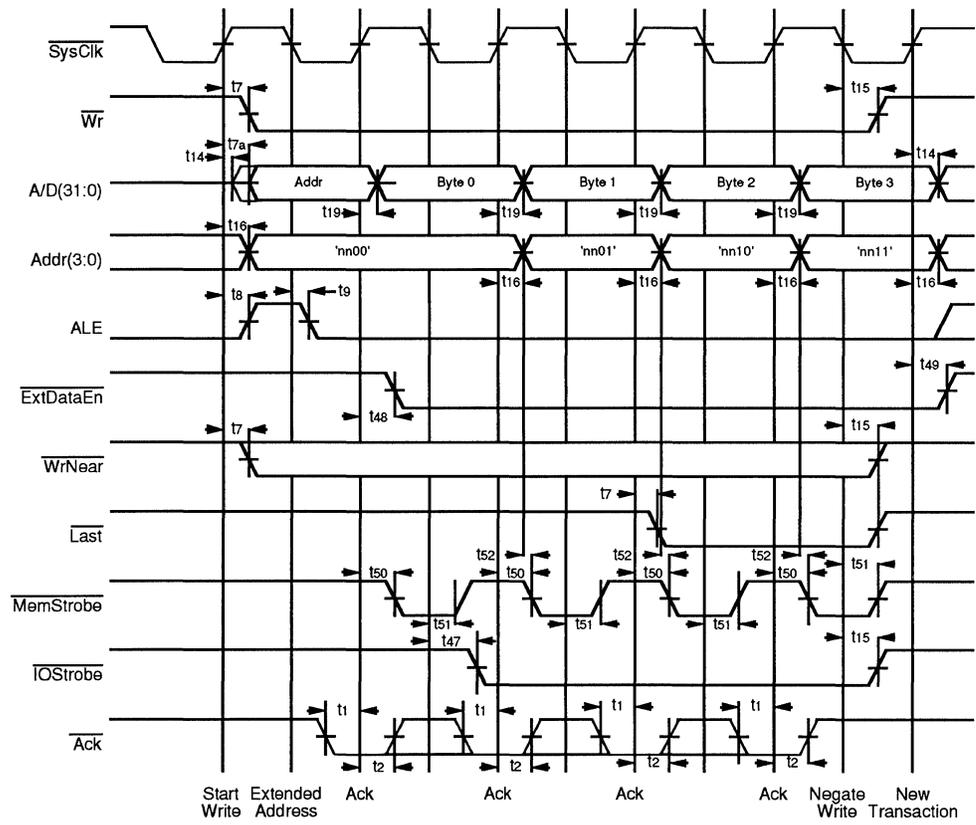
Figure 9.17. Four Byte Mini-Burst 8-Bit Port Write
