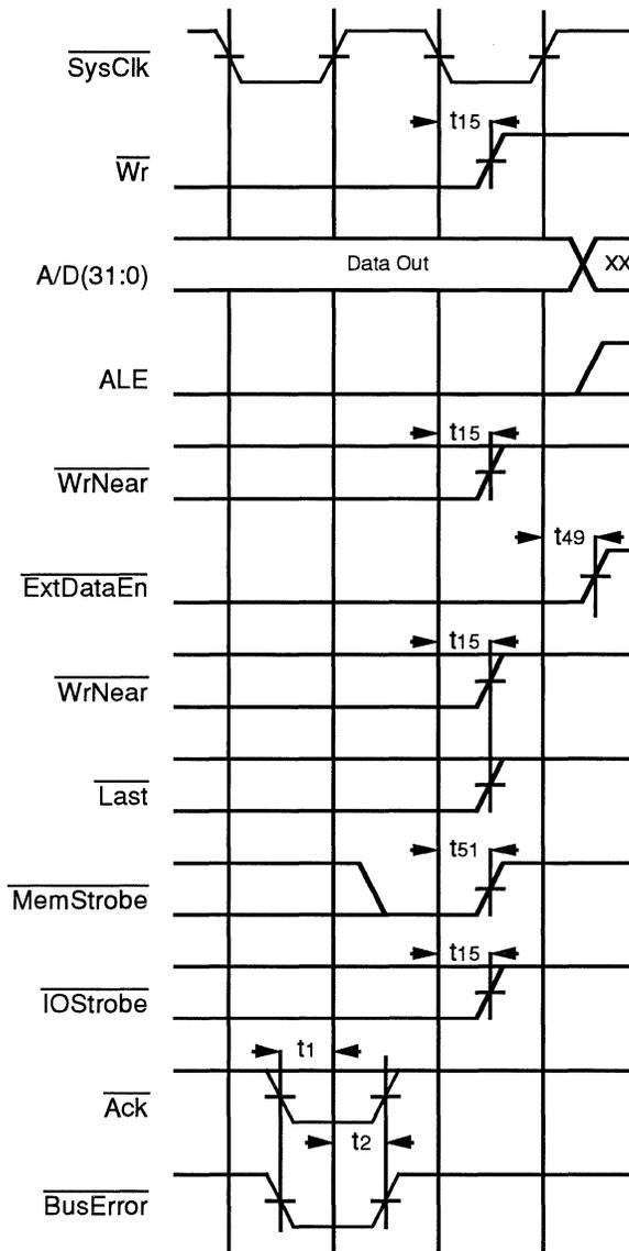
**Figure 9.12. 16-Bit Write Terminated by Bus Error**
