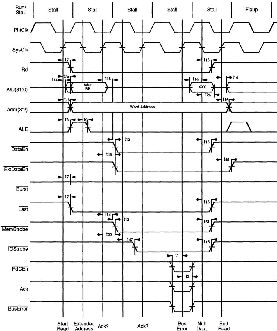
**Figure 8.14. Single Word Read Terminated by Bus Error**
