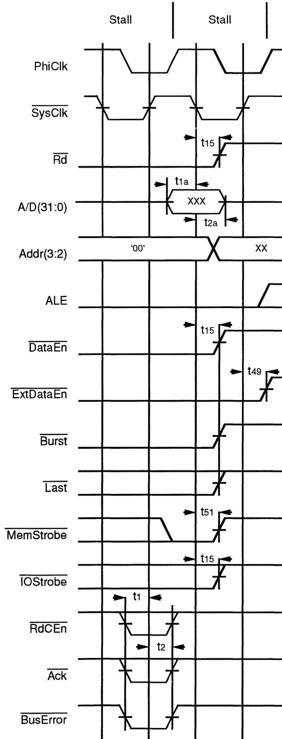
Figure 8.15. Block Read Terminated by Bus Error
