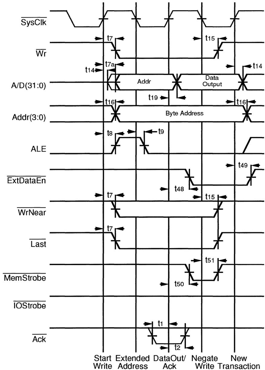
Figure 9.13. Single Byte 8-Bit Port Write with No Wait Cycles
