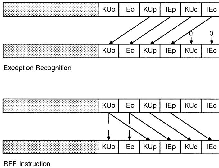
**Figure 6.12. Kernel and Interrupt Status Being Saved on Interrupts**
