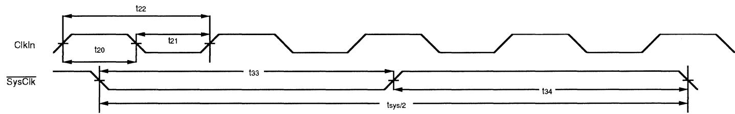
Figure 11.6 (d). R3081 Family Clocking (2x ClkIn, Half-Frequency Bus Mode)
