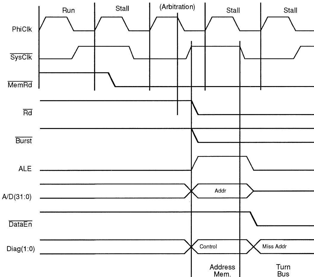
**Figure 8.1(b). CPU Latency to Start of Read (Half Frequency Mode)**
