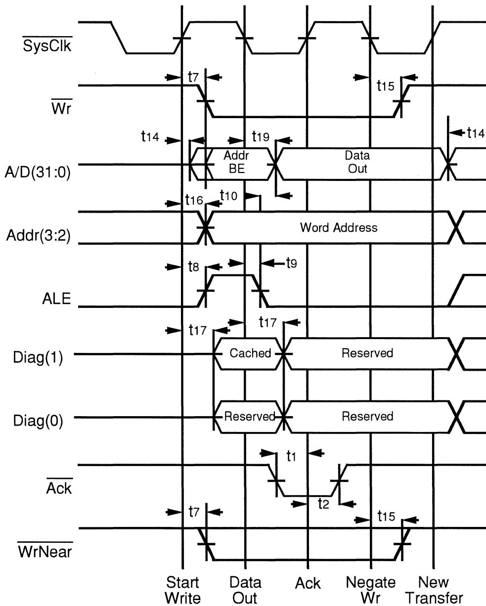
Figure 9.5. Bus Write With No Wait Cycles
