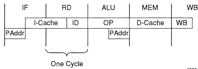
**Figure 2.5. 5-Stage Pipeline**
