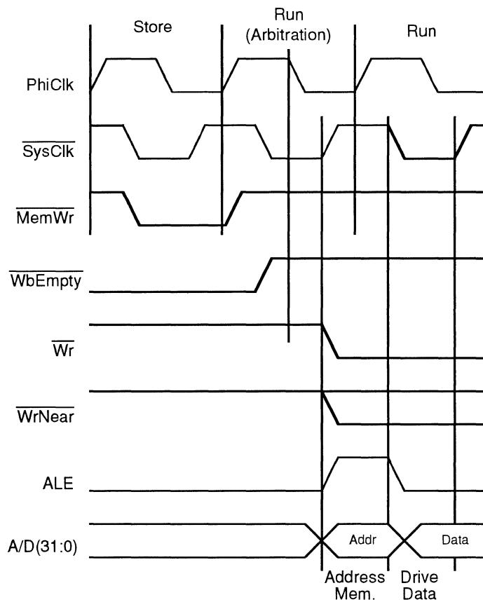
Figure 9.1 (a). Start of Write Operation – BIU Arbitration
