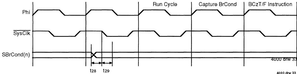
**Figure 6.10. Synchronized BrCond Inputs**
