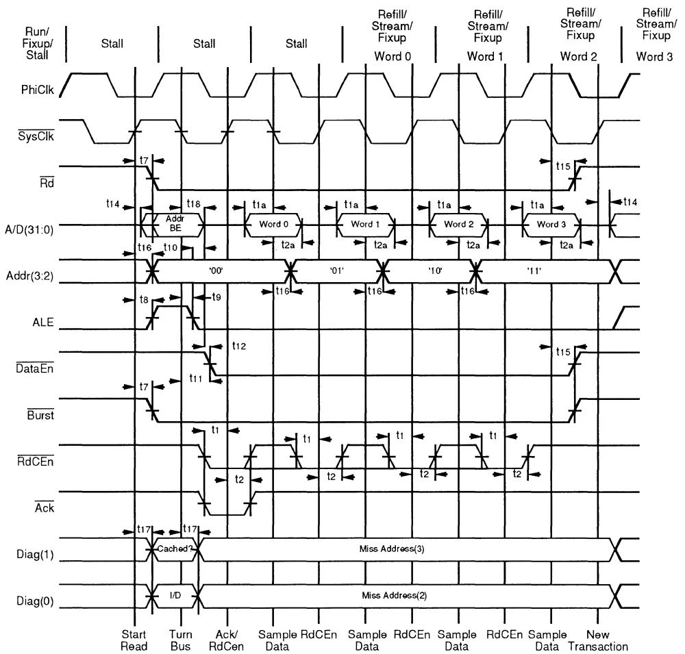
Figure 8.10. Burst Read With No Wait Cycles
