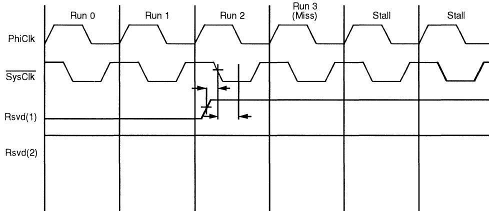
**Figure 12.2. Forcing an Instruction Cache Miss in Debug Mode**
