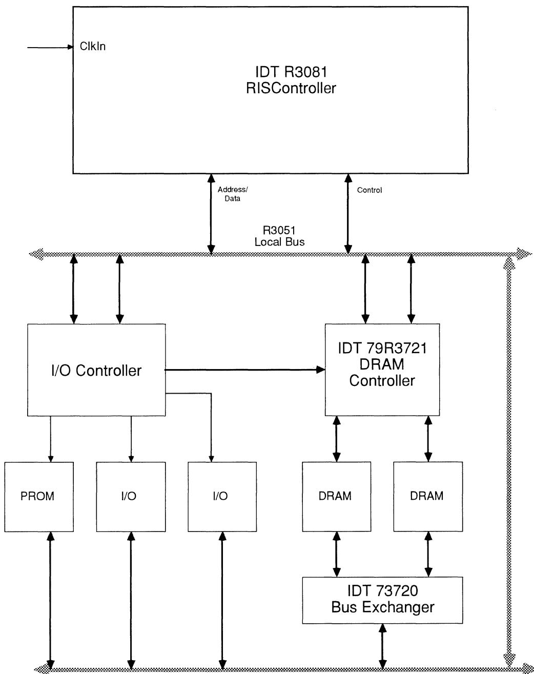
**Figure 1.2. System Diagram**
