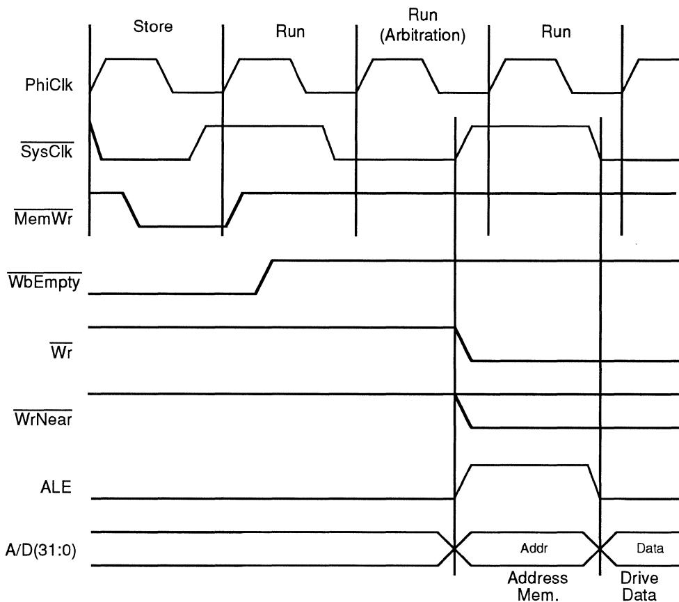
Figure 9.1 (b). Start of Write Arbitration - Half-frequency Mode
