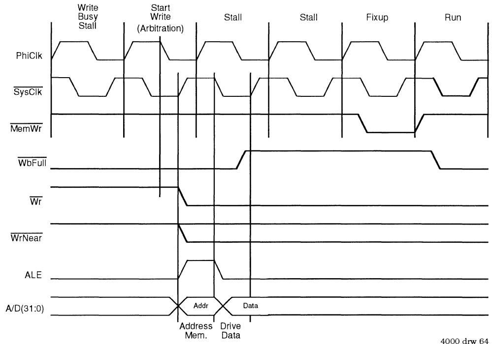
**Figure 9.4. Write Buffer Full Operation**
