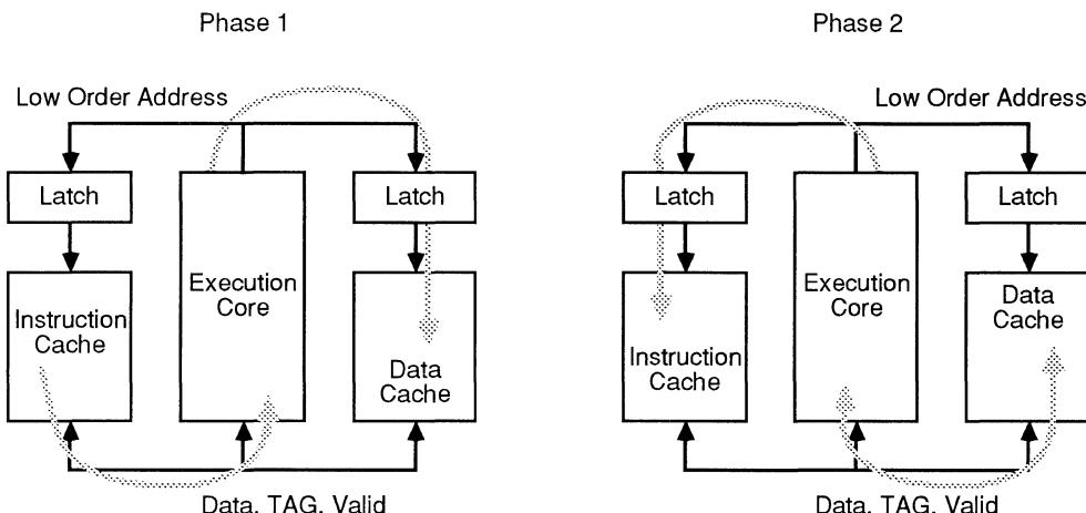
**Figure 4.4. Phased Access of Instruction and Data Caches**
