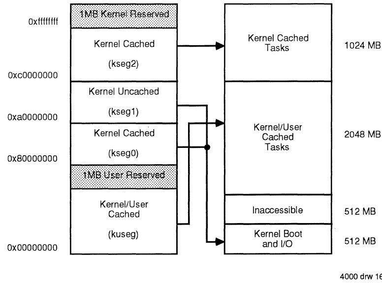
**Figure 5.2. Virtual to Physical Address Translation in Base Versions**
