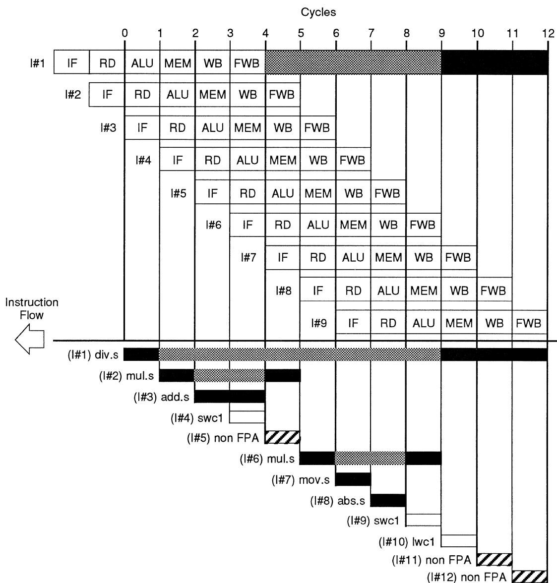
Figure 3.13. Overlapped Instructions in FPA Pipeline
