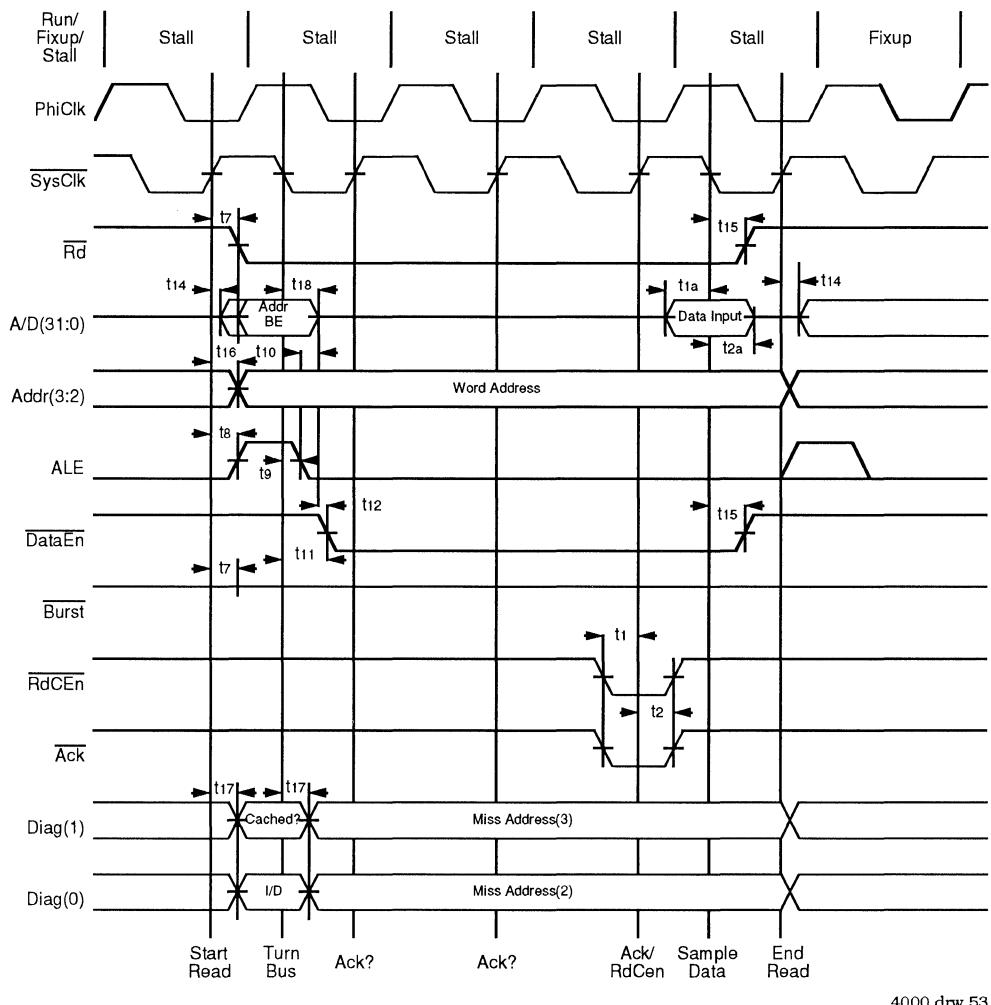
**Figure 8.9. Single Word Read With Bus Wait Cycles**
