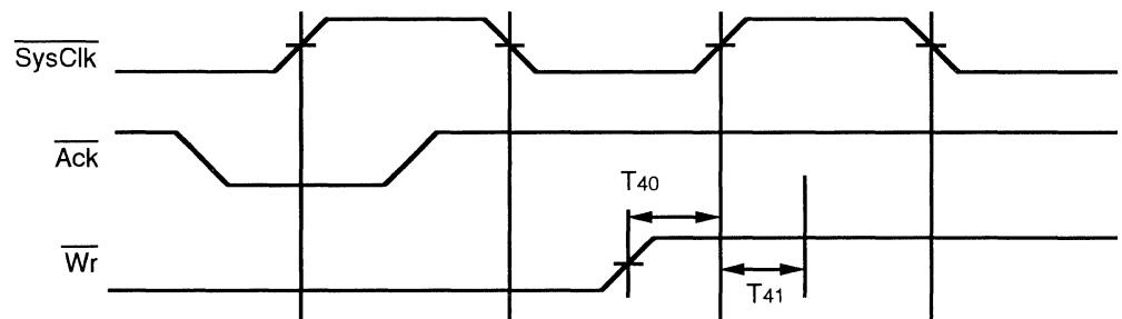
Figure 10.6. Terminating a Coherent Write Sequence
