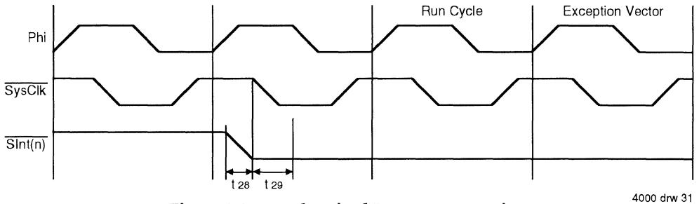
Figure 6.8. Synchronized Interrupt Operation
