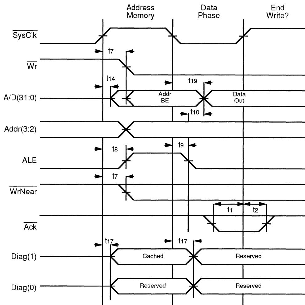
Figure 9.2. Memory Addressing and Start of Write
