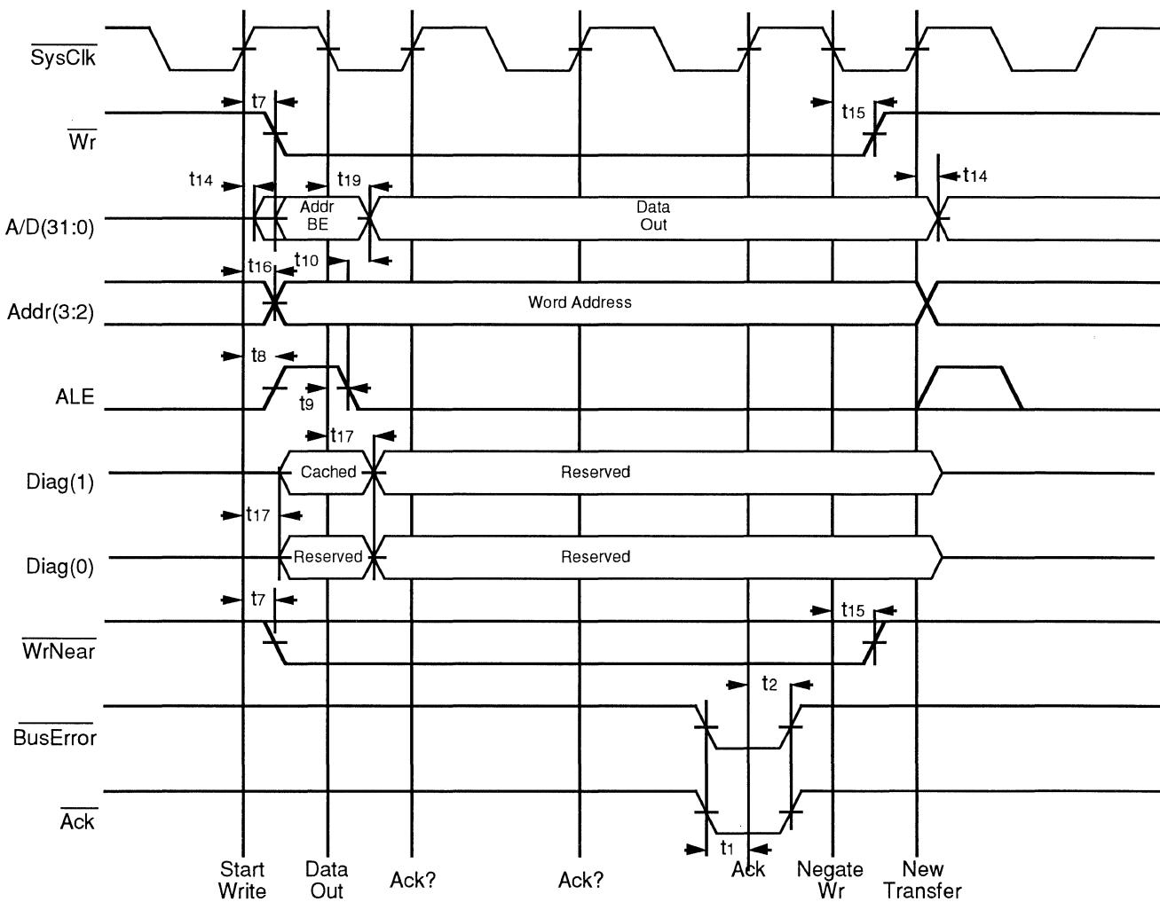
Figure 9.7. Bus Error on Write
