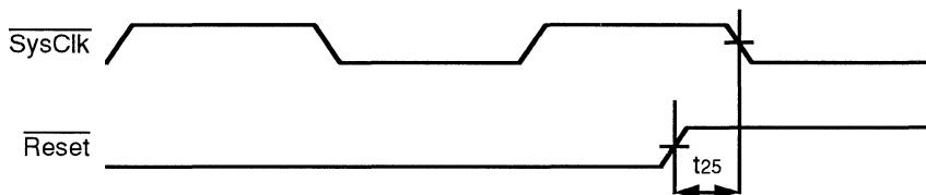
**Figure 11.5. Reset Timing**
