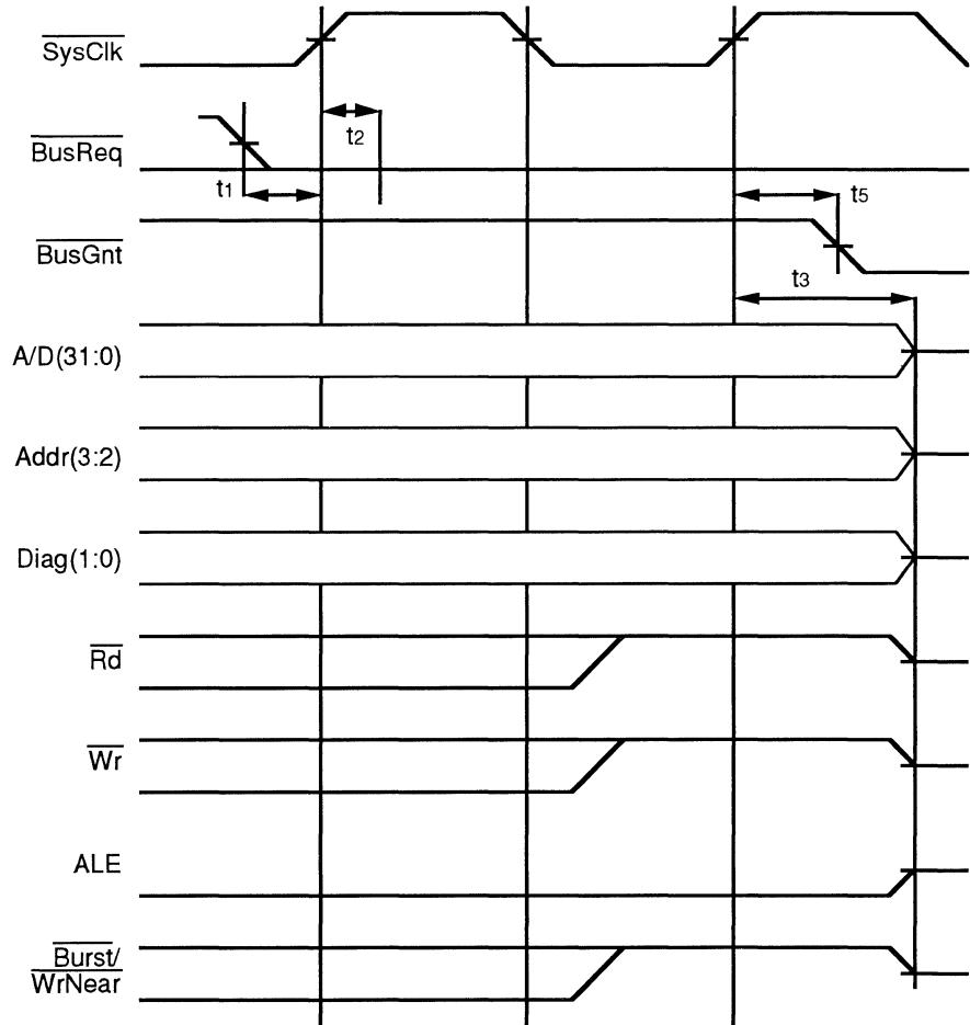
Figure 10.1. Bus Grant and Start of DMA Transaction
