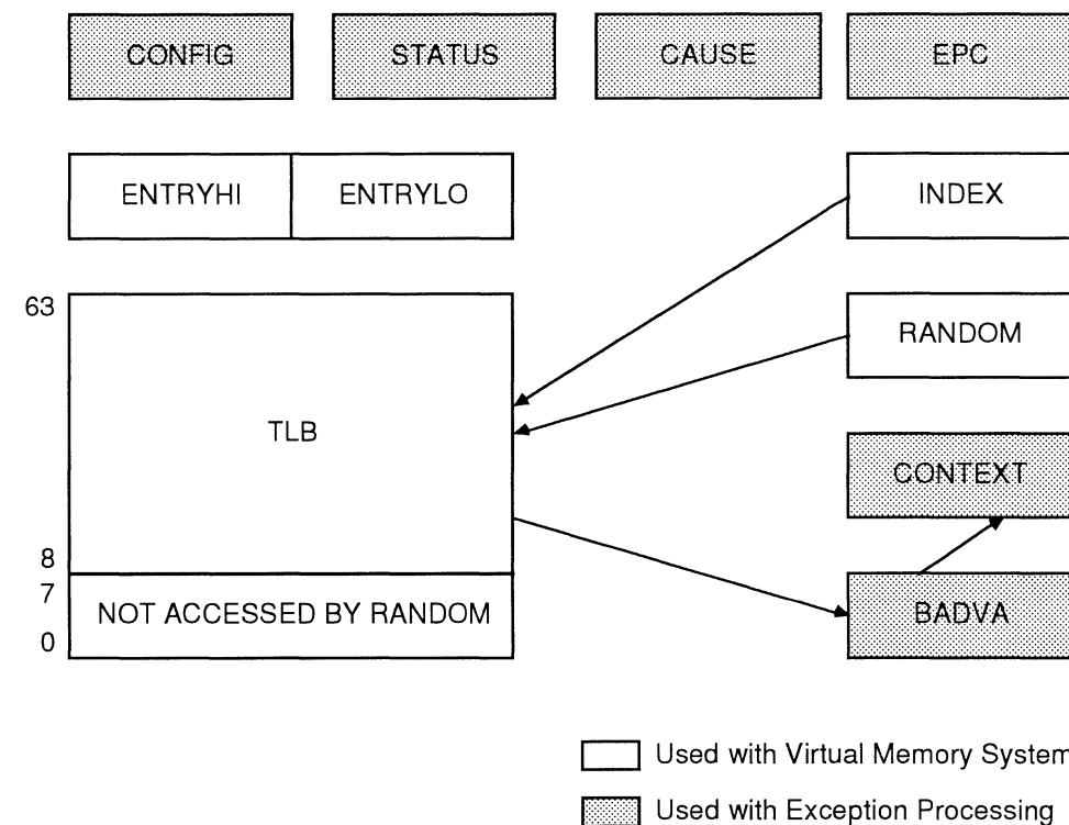
**Figure 5.4. The System Coprocessor Registers**
