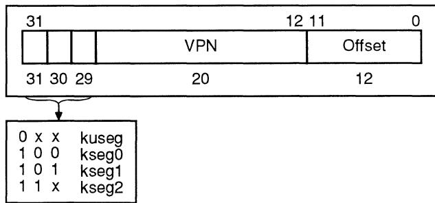
Figure 5.1. Virtual Address Format
