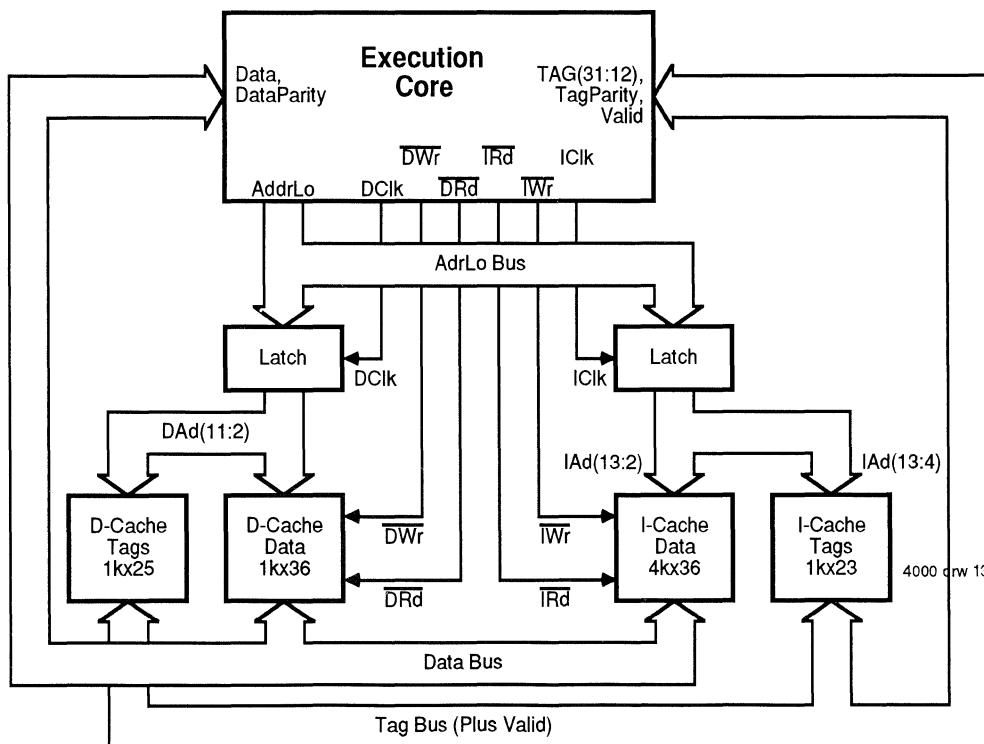
**Figure 4.2. R3081 Execution Core and Cache Interface
