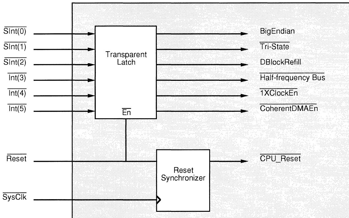
Figure 11.3. R3081 Internal Mode Vector Logic
