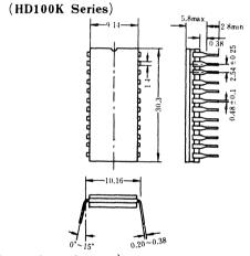
Fig.2 Package (Dimensions in mm)
