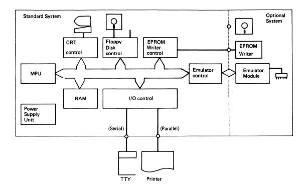
As shown in the above figure, the standard system of the H68SD5 consists of a power supply unit, 7 function blocks, a console display and one Floppy disk driver. User's system can be developed easily with this Floppy disk based system.
