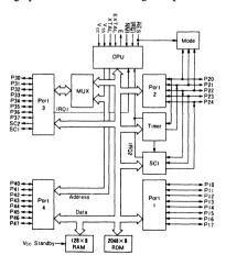
Fig. 3. Block diagram of HD6801S0.
