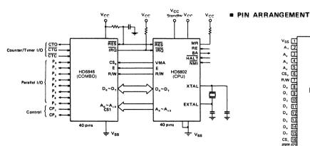
This is a block diagram of a typical cost effective microcomputer. The MPU is the center of the microcomputer system and is shown in a minimum system interfacing with a ROM combination chip. It is not intended that this system be limited to this function but that it be expandable with other parts in the HMCS6800 Microcomputer family.
