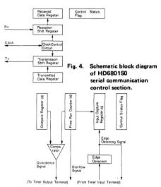
Fig. 5. Schematic block diagram of HD6801S0 timer.
