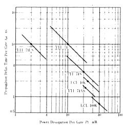
Fig.1 Propagation Delay Time vs. Power Dissipation
