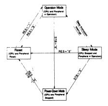
Fig. 7. Mode transition diagram of HD6301V.
