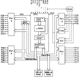
Fig. 6. Block diagram of HD6301.
