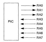
Here, the low 3 bits of port RA are used as output-only, while the high 5 bits are used as input-only. During power on reset (MCLR low), the latches in the I/O ports will be set high, turning off all pull down transistors as represented by  $Q_2$  in Figure 13. During program execution if we wish to interrogate an input pin, then, for example,
