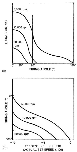
NOTE: Starting from no motor movement at all, the first load line of the motor—which corresponds to a small firing angle—is followed up to the first speed switch point, where the next firing angle takes over. This process continues until the motor runs out of torque.
