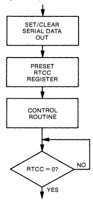
After the RTCC rolls over to zero, one bit has been transmitted.
