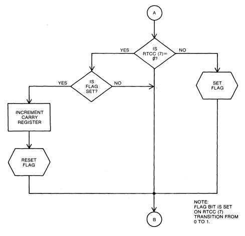
The RTCC register can also be used to time events or the interval between events. These events may be input via the input/output ports or may be generated by the program.
