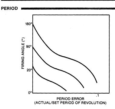
NOTE: For small changes in speed, the change in the period of motor revolution is the same as its change in speed. Consequently, the error in the motor period is proportional to its speed error and can therefore replace that variable in the firing-angle mapping.
