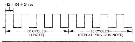
The note data is in the form of a table. The software fetches each note data in turn, decodes it and outputs as shown in Figure 32.
