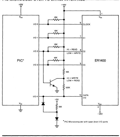
Fig. 46 PIC MICROCOMPUTER TO ER1400 INTERFACE
