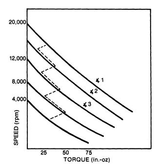
NOTE: Torque is a nonlinear function of both triac firing angle and motor speed (a). For linear motor speed regulation, the speed error must be mapped into firing angle (b). If done properly, a linear speed-error versus torque curve is achieved.
