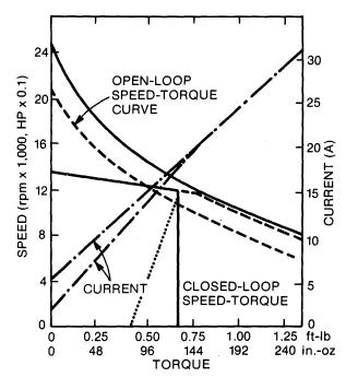
NOTE: The speed-torque curve of a universal motor determines the motor's operating point for a constant voltage input and applied load. Only a closed-loop controller will allow the speed to be kept relatively constant in the face of a variable load.
