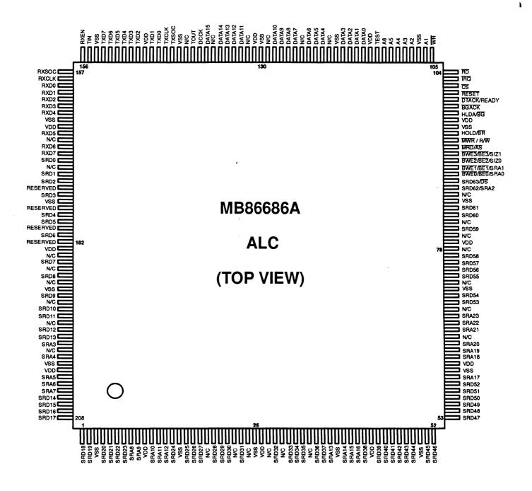
Fig 63 – ALC Pin Assignment
