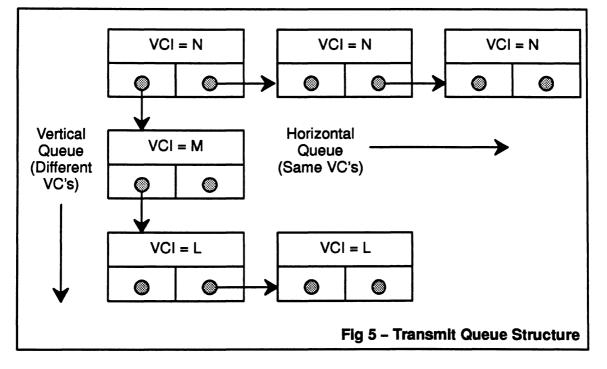
Packets with the same circuit reference, ie same VPI/VCI or MID are queued horizontally. Packets with different circuit references for transmission on the same service rate queue are queued vertically. Horizontally queued packets will be serviced when the packet at the front of the queue is completed.
