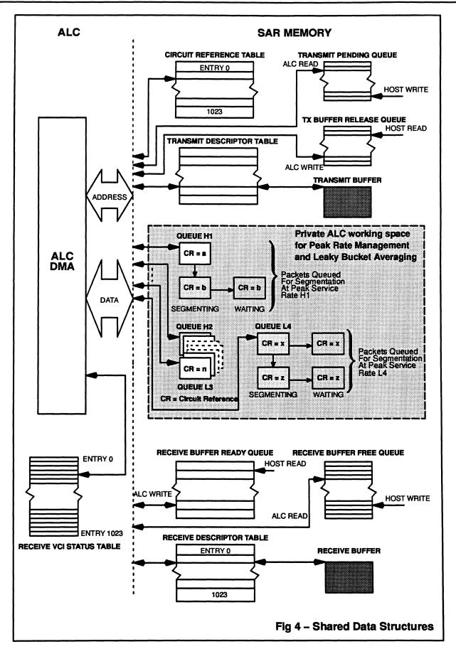
After a packet has been transmitted, the ALC will return the Transmit Buffer used to the host via the Transmit Buffer Release Queue. Each entry in this queue contains a pointer to the relevant descriptor in the Transmit Descriptor Table.
