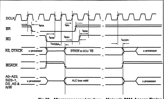
Fig 58 – Microprocessor Interface – Motorola DMA Access Timing
