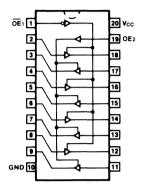
Pin Assignment for DIP, Flatpak and SOIC
