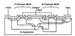
FACT devices have been specifically designed to reduce the possibility of latch-up occurring; Fairchild accomplished this by lowering the gain of the parasitic transistors, reducing substrate and p-well resistivity to increase external drive current required to cause a parasitic to turn ON, and careful design and layout to minimize the substrate-injected current coupling to other circuit areas.
