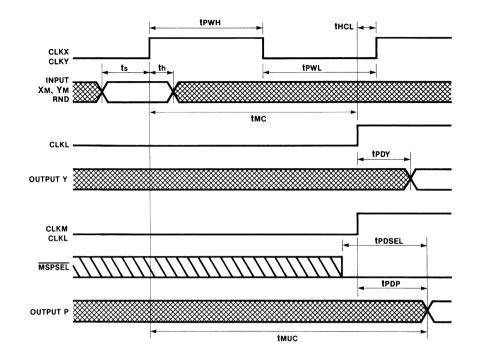
Figure 12: Simplified Timing Diagram — Typical Application
