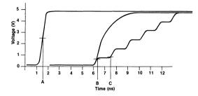
would be required before the comparator would detect the level. It is this added delay time caused by the transmission line environment of the ATE that may cause parts to fail customers' incoming tests, even though the device meets specifications. The figure below graphically shows this stepout.
