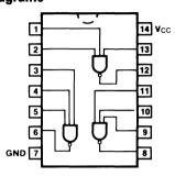
Pin Assignment for DIP, Flatpak and SOIC
