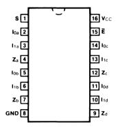
**Pin Assignment** for DIP, Flatpak and SOIC
