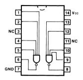
Pin Assignment for DIP, Flatpak and SOIC
