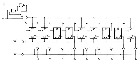
Please note that this diagram is provided only for the understanding of logic operations and should not be used to estimate propagation delays. The 'ACI'ACT824 also has the same logic diagram with inverting outputs.
