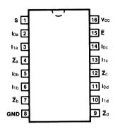
Pin Assignment for DIP, Flatpak and SOIC
