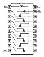
Pin Assignment for DIP, Flatpak and SOIC
