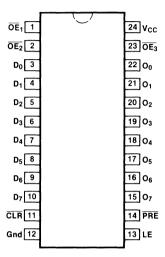
Pin Assignment for DIP, Flatpak and SOIC
