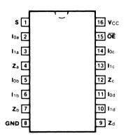
Pin Assignment for DIP, Flatpak and SOIC
