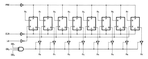
Please note that this diagram is provided only for the understanding of logic operations and should not be used to estimate propagation delays. The 'ACI'ACT846 has the same logic diagram with inverting outputs.
