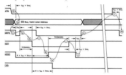
Figure 7: Timing Diagram for Listen Address Sequence
