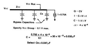
Place one decoupling capacitor adjacent to each package driving any transmission line and distribute others evenly thoughout the logic. One capacitor per three packages.
