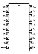
Pin Assignment for DIP, Flatpak and SOIC
