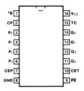
Pin Assignment for DIP, Flatpak and SOIC
