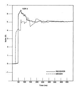
Figure 2-3a: Resultant Waveforms Driving 50 Ohm Line — Actual
