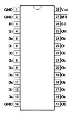
Pin Assignment for DIP and Flatpak
