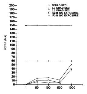
For total dose testing, all devices were subjected up to a 1 Mrad(Si) limit. There were no functional failures. Yet, based on the testing, parametric changes did occur. Transient dose testing evaluated how these devices would respond to quick bursts of radiation energies. Results were varied due to biasing and input conditions. Devices were generally free of transient upset and/or latch-up up to the range of  $3 \times 10^{\circ}$  to  $4.4 \times 10^{\circ}$  rads(Si)/second.
