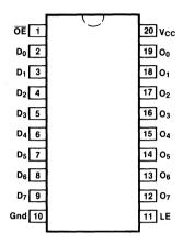
Pin Assignment for DIP, Flatpak and SOIC
