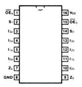
Pin Assignment for DIP, Flatpak and SOIC
