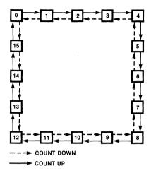
to be loaded into the flip-flops on the next rising edge of CP. With  $\overline{\text{MR}}$ ,  $\overline{\text{SR}}$  and  $\overline{\text{PE}}$  HIGH,  $\overline{\text{CEP}}$  and  $\overline{\text{CET}}$  permit counting when both are LOW. Conversely, a HIGH signal on either  $\overline{\text{CEP}}$  or  $\overline{\text{CET}}$  inhibits counting.
