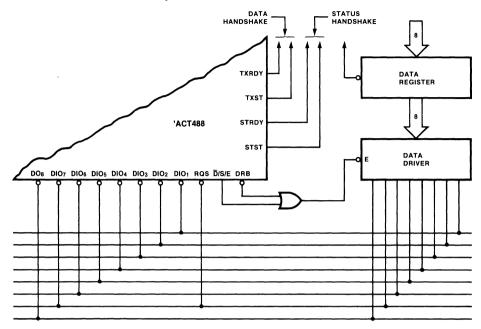
Figure 5: Status Byte Multiplexing
