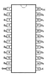
Pin Assignment for DIP, Flatpak and SOIC
