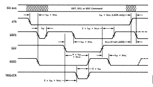
Figure 13: Timing Diagram for Device Clear and Device Trigger Commands
