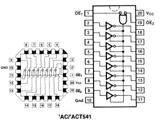
Pin Assignment Pin Assignment for LCC for DIP, Flatpak and SOIC
