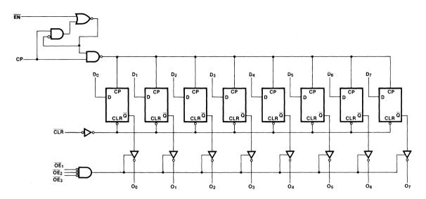
Please note that this diagram is provided only for the understanding of logic operations and should not be used to estimate propagation delays. The 'AC/'ACT826 also has the same logic diagram with inverting outputs.
