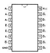
Pin Assignment for DIP, Flatpak and SOIC
