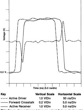
This figure shows traces taken on a test fixture designed to exaggerate the amplitude of crosstalk pulses.
