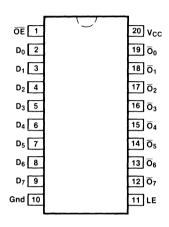
Pin Assignment for DIP, Flatpak and SOIC
