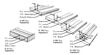
Local high frequency decoupling is required to supply power to the chip when it is transitioning from a LOW to a HIGH value. This power is necessary to charge the load capacitance or drive a line impedance. Figure 4-13 displays various Vcc and ground layout schemes along with associated impedances.
