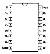
Pin Assignment for DIP, Flatpak and SOIC
