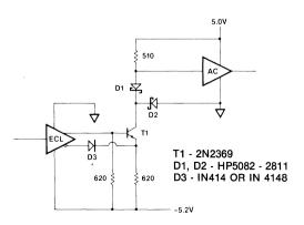
It should be understood that for FACT, as with other CMOS technologies, input levels that are between specified input values will cause both transistors in the CMOS structure to be conducting. This will cause a low resistive path from the supply rail to ground, increasing the power consumption by several orders of magnitude. It is important that CMOS inputs are always driven as close as possible to the rail.
