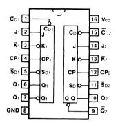
Pin Assignment for DIP, Flatpak and SOIC
