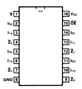
Pin Assignment for DIP, Flatpak and SOIC
