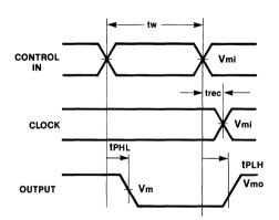
$V_{mi} = 50\%$  Vcc for 'AC devices; 1.5 V for 'ACT devices Vmo = 50% for 'AC/'ACT devices
