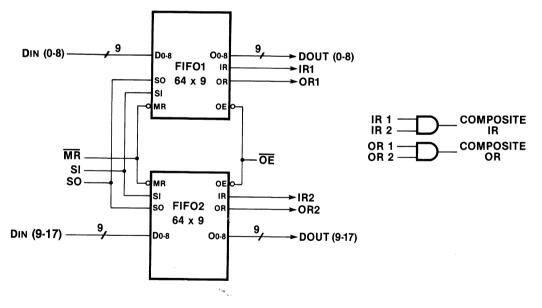
Note: Monitor flags from any one FIFO or AND the corresponding flags to obtain a composite signal.
