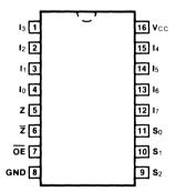
Pin Assignment for DIP, Flatpak and SOIC
