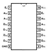
Pin Assignment for DIP, Flatpak and SOIC
