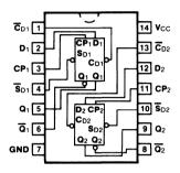
Pin Assignment for DIP, Flatpak and SOIC
