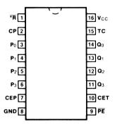
Pin Assignment for DIP, Flatpak and SOIC
