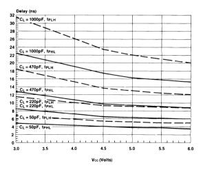
Figure 2-13: Propagation Delay vs. CL (AC00)
