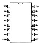
Pin Assignment for DIP, Flatpak and SOIC
