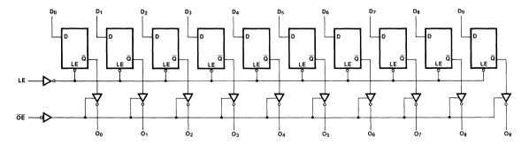
Please note that this diagram is provided only for the understanding of logic operations and should not be used to estimate progagation delays. The 'AC/'ACT842 has the same logic diagram with inverting outputs.
