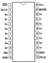
Pin Assignment for DIP, Flatpak and SOIC
