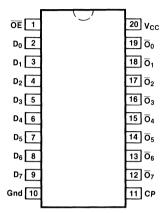
Pin Assignment for DIP, Flatpak and SOIC
