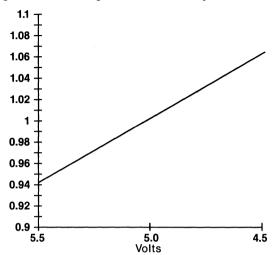
Figure 2-11d: FACT Process Effects on Delay Times
