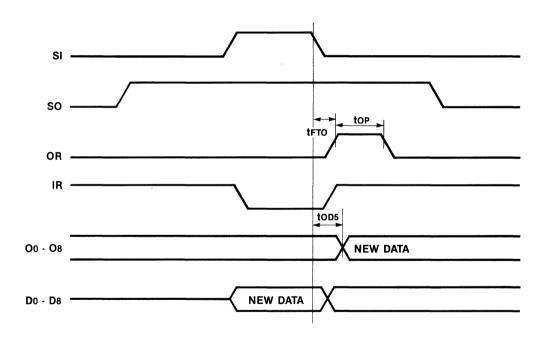
Note: MR is HIGH; OE is LOW; toor = tro-toos — data output transition, valid data arrives at output stage toor after OR is HIGH.
