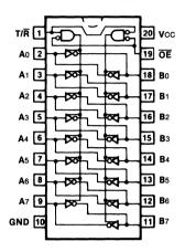
Pin Assignment for DIP, Flatpak and SOIC
