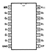
Pin Assignment for DIP, Flatpak and SOIC
