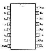
Pin Assignment for DIP, Flatpak and SOIC
