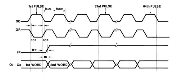
Note: SI and  $\overline{OE}$  are LOW;  $\overline{MR}$  is HIGH; D<sub>0</sub> - D<sub>8</sub> are immaterial.
