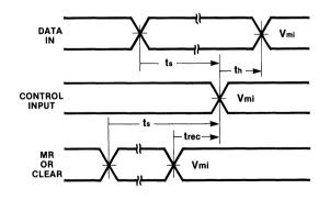
$V_{mi} = 50\%$  Vcc for 'AC devices; 1.5 V for 'ACT devices Vmo = 50% Vcc for 'ACI'ACT devices **Propagation Delays, fmax, Set and Hold Times** A 1.0 MHz square wave is recommended for most propagation delay tests. The repetition rate must necessarily be increased for testing fmax. A 50% duty cycle should always be used when testing fmax. Two pulse generators are usually required for testing such parameters as setup time, hold time, recovery time, etc.
