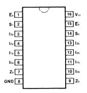
Pin Assignment for DIP, Flatpak and SOIC
