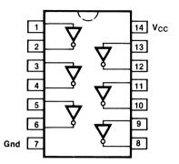
Pin Assignment for DIP, Flatpak and SOIC
