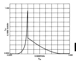
The Delta Icc specification is the increase in Icc. For each input at Vcc-2.1 V, the Delta Icc value should be added to the quiescent supply current to arrive at the circuit's worst-case static Icc value.
