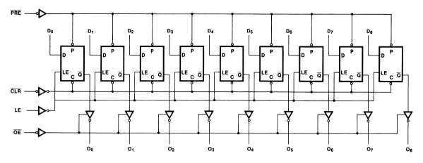
Please note that this diagram is provided only for the understanding of logic operations and should not be used to estimate propagation delays. The 'AC/'ACT844 has the same logic diagram with inverting outputs.
