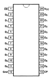
Pin Assignment for DIP, Flatpak and SOIC
