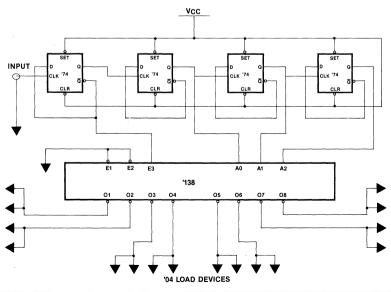
The circuit shown in Figure 2-9 was used to compare the power consumption of FACT versus ALS devices.
