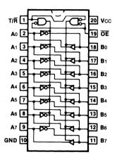
Pin Assignment for DIP, Flatpak and SOIC
