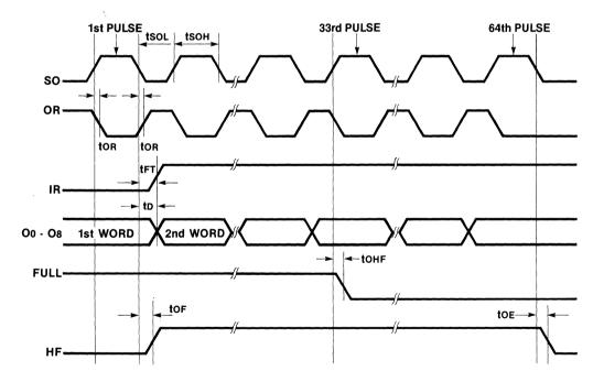
Note: SI and  $\overline{OE}$  are LOW;  $\overline{MR}$  is HIGH; D<sub>0</sub> - D<sub>8</sub> are immaterial.
