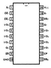
Pin Assignment for DIP, Flatpak and SOIC
