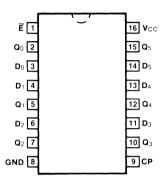
Pin Assignment for DIP, Flatpak and SOIC
