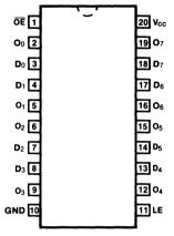
Pin Assignment for DIP, Flatpak and SOIC
