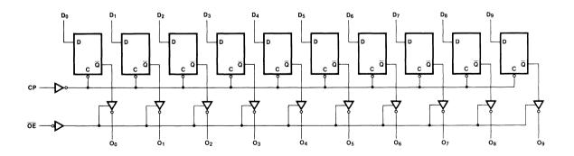
Please note that this diagram is provided only for the understanding of logic operations and should not be used to estimate progagation delays. The 'ACI'ACT822 also has the same logic diagram with inverting outputs.
