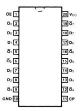
Pin Assignment for DIP, Flatpak and SOIC
