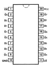
Pin Assignment for DIP, Flatpak and SOIC
