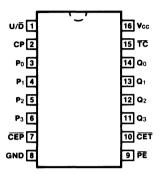
Pin Assignment for DIP, Flatpak and SOIC
