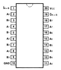
Pin Assignment for DIP, Flatpak and SOIC
