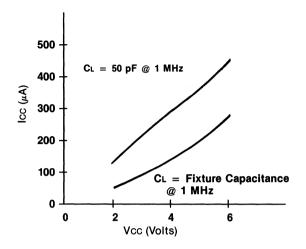
Figure 2-1 illustrates the effects of Icc versus power supply voltage (Vcc) for two load capacitance values: 50 pF and stray capacitance. The clock frequency was 1 MHz for the measurements.
