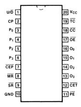
Pin Assignment for DIP, Flatpak and SOIC
