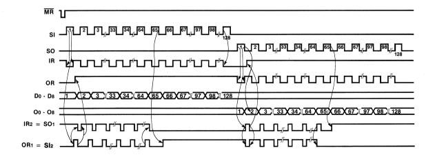
Note: The numbers for SI and SO indicate the pulse numbers. The numbers for data in and data out indicate data words: 1 is the first data word, 2 is the second data word, etc.
