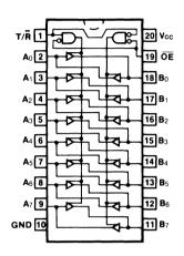
Pin Assignment for DIP, Flatpak and SOIC
