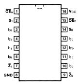
Pin Assignment for DIP, Flatpak and SOIC
