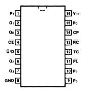
Pin Assignment for DIP, Flatpak and SOIC
