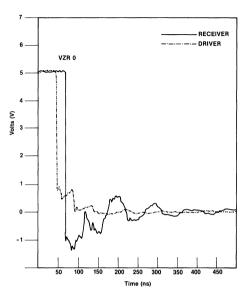
Figure 2-3b: Resultant Waveforms Driving 50 Ohm Line — Theoretical
