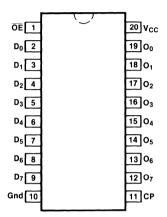
Pin Assignment for DIP, Flatpak and SOIC
