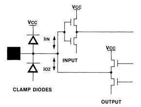
device will also float, and an excessive amount of current will flow from Vcc to ground. A simple rule to follow is to treat any output which is disabled as an input. This will help insure the integrity of an Icc test.
