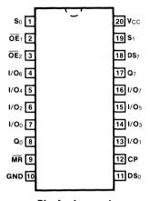
Pin Assignment for DIP, Flatpak and SOIC
