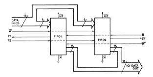
Notes: Flag detection is accomplished by monitoring FF, EF and HF on any device used in the width expansion configuration. Output signals should not be connected together.
