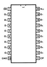
Pin Assignment for DIP, Flatpak and SOIC
