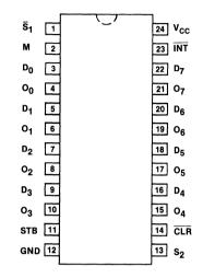
Pin Assignment for DIP and SOIC
