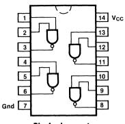
**Pin Assignment** for DIP and SOIC
