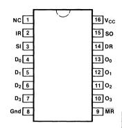
Pin Assignment for DIP and SOIC
