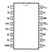
Pin Assignment for DIP and SOIC
