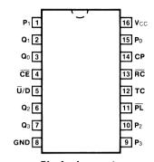
Pin Assignment for DIP and SOIC
