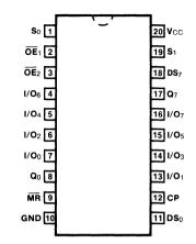
Pin Assignment for DIP and SOIC
