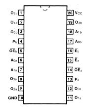
Pin Assignment for DIP and SOIC
