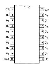
Pin Assignment for DIP and SOIC
