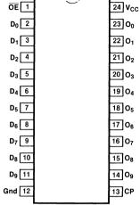
Pin Assignment for DIP and SOIC
