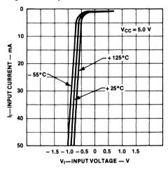
Fig. 2-17 Input Characteristics—'F00 or 'F244
