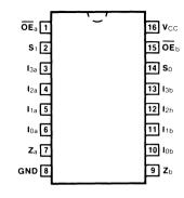
Pin Assignment for DIP and SOIC
