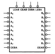
Pin Assignment for DIP and SOIC
