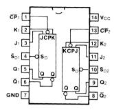
Pin Assignment for DIP and SOIC
