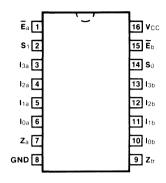
Pin Assignment for DIP and SOIC
