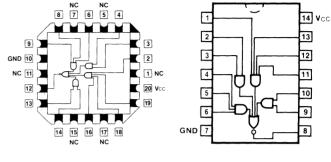
Pin Assignment for LCC and PCC Pin Assignment for DIP and SOIC
