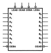
Pin Assignment for DIP and SOIC
