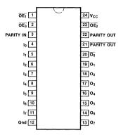
Pin Assignment for DIP and SOIC
