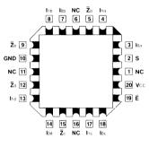
Pin Assignment for LCC and PLCC
