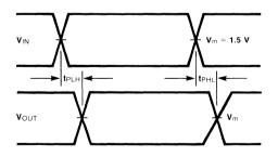
Fig. 3-12 3-State Output LOW Enable and Disable Times
