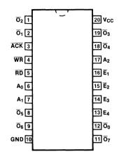
Pin Assignment for DIP and SOIC
