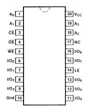
**Pin Assignment** for DIP and SOIC
