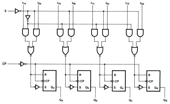
Please note that this diagram is provided only for the understanding of logic operations and should not be used to estimate propagation delays.
