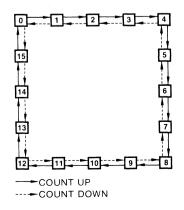
Clock will cause  $\overline{TC}_U$  to go LOW.  $\overline{TC}_U$  will stay LOW until CP<sub>U</sub> goes HIGH again, thus effectively repeating the Count Up Clock, but delayed by two gate delays. Similarly, the  $\overline{TC}_D$  output will go LOW when the circuit is in the zero state and the Count Down Clock goes LOW. Since the  $\overline{TC}$  outputs repeat the clock waveforms, they can be used as the clock input signals to the next higher order circuit in a multistage counter.
