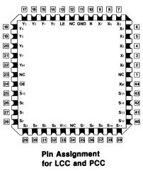
Pin assignments shown are for 'F558. LE and R shown in parentheses are pin assignments for 'F557.
