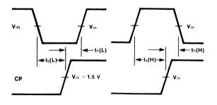
Fig. 3-6 Setup and Hold Times, Falling-Edge Clock
