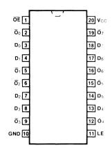
Pin Assignment for DIP and SOIC
