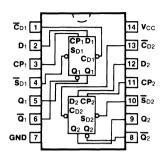
Pin Assignment for DIP and SOIC
