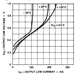
Fig. 2-12 Output LOW Characteristics—'F244
