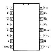
Pin Assignment for DIP and SOIC
