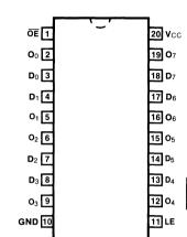
Pin Assignment for DIP and SOIC
