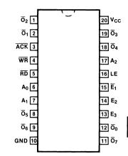
Pin Assignment for DIP and SOIC
