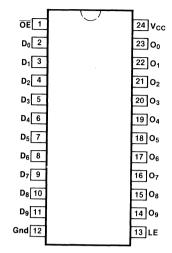
**Pin Assignment** for DIP and SOIC
