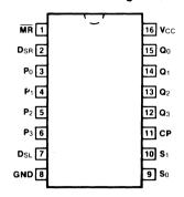
Pin Assignment for DIP and SOIC
