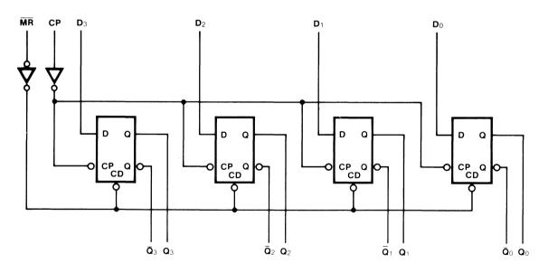
Please note that this diagram is provided only for the understanding of logic operations and should not be used to estimate propagation delays.
