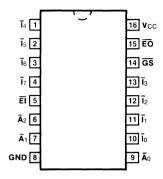
Pin Assignment for DIP and SOIC
