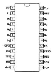
Pin Assignment for DIP and SOIC
