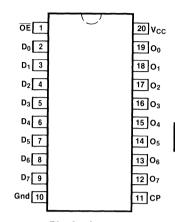
Pin Assignment for DIP and SOIC
