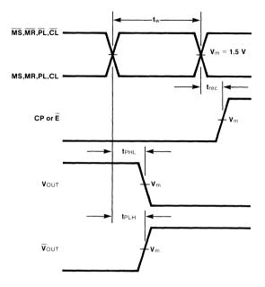
Fig. 3-10 Whether Response is Inverting or Non-Inverting Depends on Specific Truth Table Conditions
