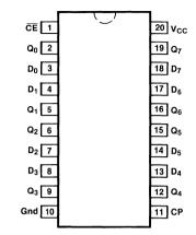
Pin Assignment for DIP and SOIC
