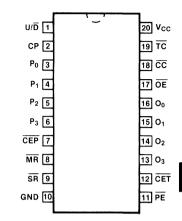
Pin Assignment for DIP and SOIC
