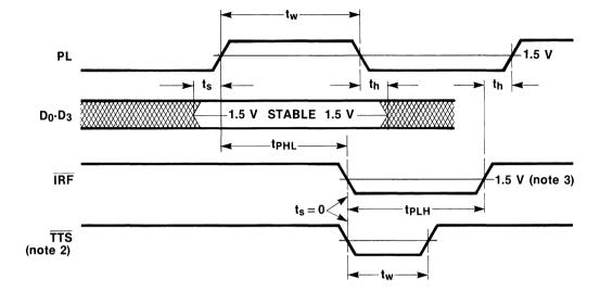
Fig. 403-g Parallel Load Mode, 4-Bit Word (Unexpanded) or master in Parallel Expansion
