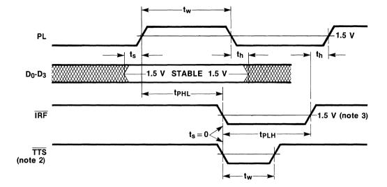
Fig. 433-g Parallel Load Mode, 4-Bit Word (Unexpanded) or Master in Parallel Expansion
