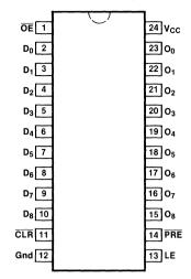
**Pin Assignment** for DIP and SOIC
