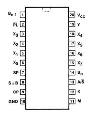
Pin Assignment for DIP and SOIC
