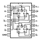
Pin Assignment for DIP and SOIC
