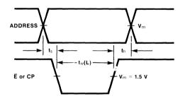
Fig. 3-14 Setup and Hold Times to Active LOW Enable or Parallel Load
