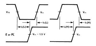
Fig. 3-17 Test Input Signal Levels
