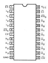
Pin Assignment for DIP and SOIC
