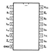
Pin Assignment for DIP and SOIC
