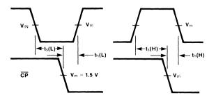
Fig. 3-8 Propagation Delays from Falling- Edge Clock or Enable
