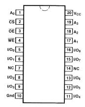
**Pin Assignment** for DIP and SOIC
