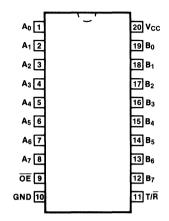
Pin Assignment for DIP and SOIC
