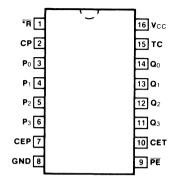
Pin Assignment for DIP and SOIC
