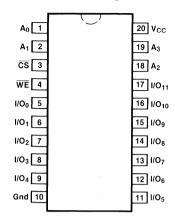
Pin Assignment for DIP and SOIC
