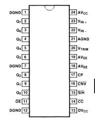
Pin Assignment for DIP and SOIC
