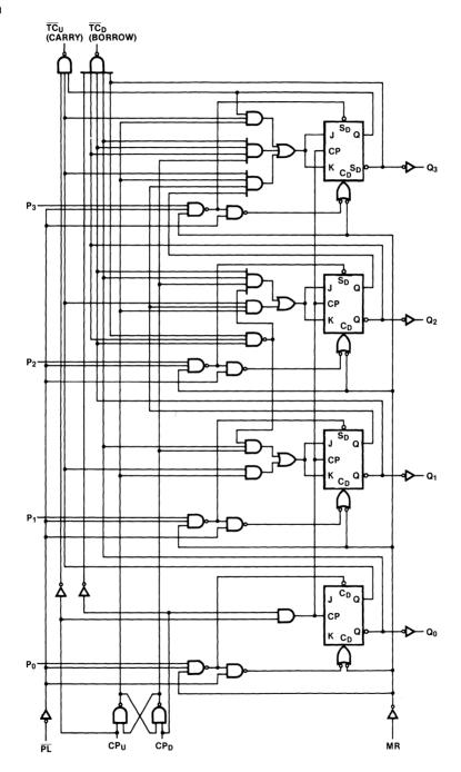
Please note that this diagram is provided only for the understanding of logic operations and should not be used to estimate propagation delays.
