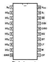
Pin Assignment for DIP and SOIC
