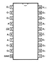
Pin Assignment for DIP and SOIC
