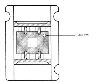
Standard carrier loading locates Lead One of the device adjacent to the side with the double notch, mark side up.
