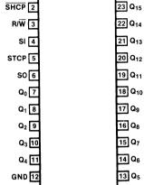
Pin Assignment for DIP and SOIC
