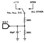
**\*INCLUDES JIG AND PROBE CAPACITANCE**
