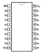
Pin Assignment for DIP and SOIC
