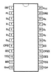
Pin Assignment for DIP and SOIC
