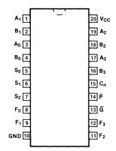
Pin Assignment for DIP and SOIC
