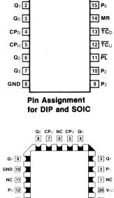
The 'F193 is a 4-bit binary synchronous up/down (reversible) counter. It contains four edge-triggered flip-flops, with internal gating and steering logic to provide master reset, individual preset, count up and count down operations.
