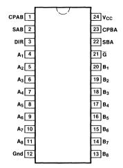
Pin Assignment for DIP and SOIC
