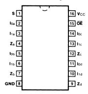
Pin Assignment for DIP and SOIC
