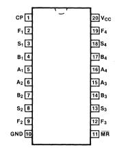
Pin Assignment for DIP and SOIC
