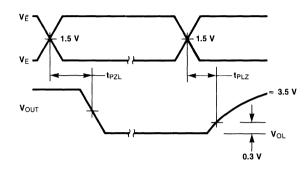
Fig. 3-15 Setup and Hold Times to Active HIGH Enable or Parallel Load
