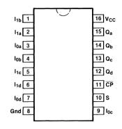
Pin Assignment for DIP and SOIC
