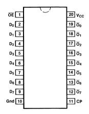
Pin Assignment for DIP and SOIC
