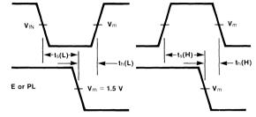
Fig. 3-13 3-State Output HIGH Enable and Disable Times
