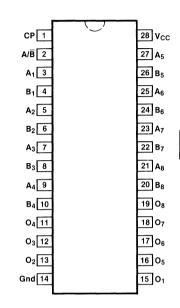
Pin Assignment for DIP and SOIC
