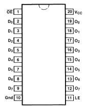
Pin Assignment for DIP and SOIC
