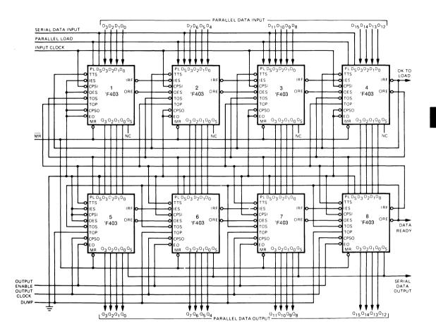
Fig. 7 Serial Data Entry for Array of Fig. 6
