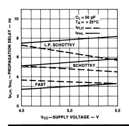
LOW delays. These improved characteristics offered by FAST circuits make it easier to predict system performance early in the design phase, before loading details are precisely known. The curves show that the skew between HIGH-to-LOW and LOW-to-HIGH delays for the FAST gate is only about 0.5 ns, over a broad range of load capacitance, whereas the skew for the S-TTL gate is 1 ns or greater, depending on loading.
