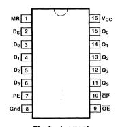
Pin Assignment for DIP and SOIC
