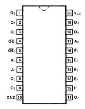
Pin Assignment for DIP and SOIC
