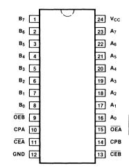
Pin Assignment for DIP and SOIC
