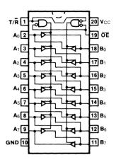
Pin Assignment for DIP and SOIC
