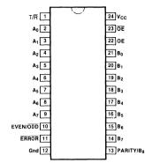
Pin Assignment for DIP and SOIC
