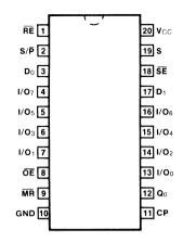
Pin Assignment for DIP and SOIC
