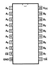
Pin Assignment for DIP and SOIC
