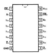
**Pin Assignment** for DIP and SOIC
