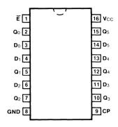
Pin Assignment for DIP and SOIC
