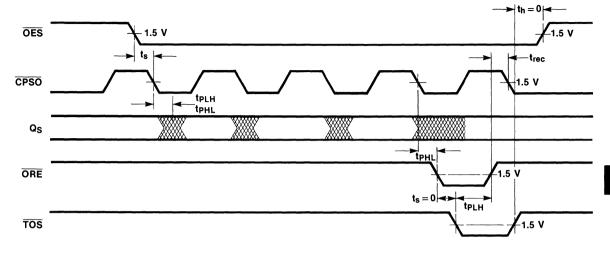
Fig. 433-d Serial Output, Slave Operation
