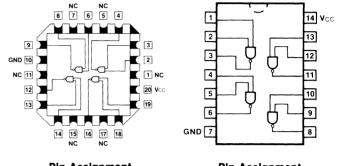
Pin Assignment for DIP and SOIC
