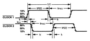
c) Color Subcarrier Timing and Reset Detail
