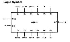
$V_{SS}$  = Pin 20 (24-Pin DIP), Pin 16 (16-Pin DIP)  $V_{GG}$  = Pin 6 (24-Pin DIP), Pin 5 (16-Pin DIP)
