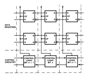
A Master Reset control is provided to set all the control registers' status markers to "0". Note that the data registers are not reset by MR.
