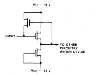
More specifically, the input current increases significantly when  $V_{IN}$  starts to exceed  $V_{II}$  (the pull-up initiation voltage). This current reaches a peak value of I<sub>IP</sub> (the input barrier current) when  $V_{IN} = V_{IP}$  (the peak input current voltage point) after which it decreases as  $V_{IN}$  rises to its  $V_{IH}$  value.
