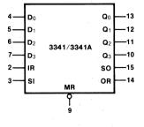
$V_{SS} = Pin 16$  $V_{DD} = Pin 8$  $V_{GG} = Pin 1$
