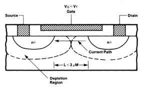
Since vertical dimensions like oxide thickness also shrink during scaling, storage capacitance per unit area for future devices will remain roughly the same as for present-day NMOS. However, since the power supply voltage must be scaled to maintain a constant electric field, the charge written into a dynamic memory cell will be reduced since it is a product of the cell capacitance and writing voltage.
