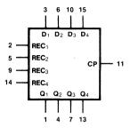
$V_{SS} = Pin 16$  $V_{DD} = Pin 8$  $V_{GG} = Pin 12$
