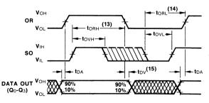
Both SO and OR must be HIGH for  $t_{\mbox{OVH}}.$  Similarly both SO and OR must be LOW for  $t_{\mbox{OVL}}.$  Data will remain stable for  $t_{\mbox{DV}}$  after both SO and OR are LOW.
