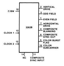
$V_{SS} = Pin 16$  $V_{DD} = Pin 9$  $V_{GG} = Pin 8$
