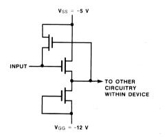
More specifically, the input current increases significantly when V<sub>IN</sub> starts to exceed V<sub>II</sub> (the pull-up initiation voltage). This current reaches a peak value of I<sub>IP</sub> (the input barrier current) when V<sub>IN</sub> = V<sub>IP</sub> (the peak input current voltage point) after which it decreases as V<sub>IN</sub> rises to its V<sub>IH</sub> value.
