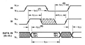
Input data must remain stable during timing window  $t_{\mbox{DH}}$ . Both SI and IR must be HIGH for t<sub>OVH</sub>. Similarly, both SI and IR must be LOW for tOVL.
