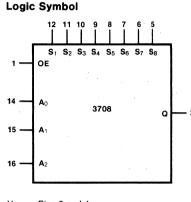
$V_{SS} = Pins 2 and 4$  $V_{DD} = Pin 13$
