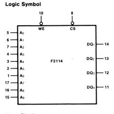
$V_{CC} = Pin \ 18$ GND = Pin 9
