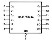
$V_{SS} = Pin 16$  $V_{DD} = Pin 8$  $V_{GG} = Pin 1$
