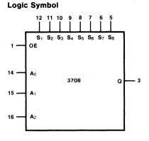
$V_{SS} = Pins 2 and 4$  $V_{DD} = Pin 13$
