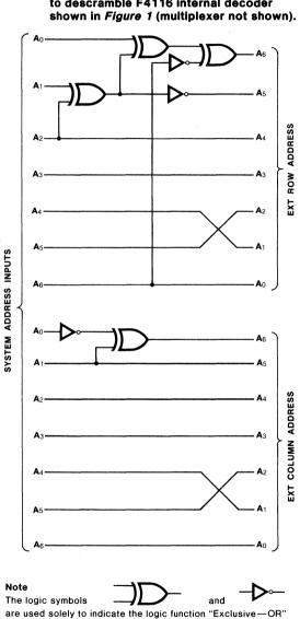
Fig. 4 External address transformation required to descramble F4116 internal decoder shown in *Figure* 1 (multiplexer not shown)
