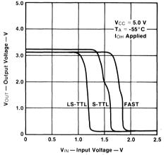
Fig. 2-4 Transfer Functions at Low Temperature
