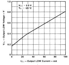
Fig. 2-14 Output LOW Characteristic
