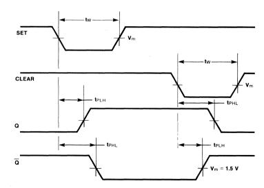
Fig. 2-22 Propagation Delays from Set and Clear (or Reset)
