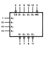
V<sub>CC</sub> = Pin 16 GND = Pin 8
