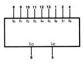
V<sub>CC</sub> = Pin 14 GND = Pin 7
