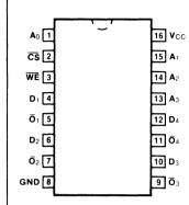
**DESCRIPTION** — The 'F289 is a high speed 64-bit RAM organized as a 16word by 4-bit array. Address inputs are buffered to minimize loading, and addresses are fully decoded on-chip. Outputs are open-collector type and are in the off (HIGH) state whenever the Chip Select ( $\overline{CS}$ ) input is HIGH. The outputs are active only in the Read mode; output data is the complement of the stored data.
