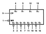
V<sub>CC</sub> = Pin 16 GND = Pin 8
