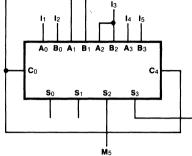
Fig. c 5-Input Encoder
