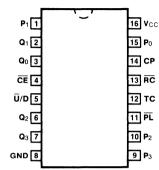
DESCRIPTION -- The 'F190 is a reversible BCD (8421) decade counter featuring synchronous counting and asynchronous presetting. The preset feature allows the 'F190 to be used in programmable dividers. The Count Enable input, the Terminal Count output and the Ripple Clock output make possible a variety of methods of implementing multistage counters. In the counting modes, state changes are initiated by the rising edge of the clock.
