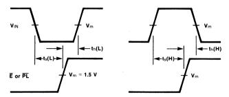
Fig. 2-28 Setup and Hold Times to Active-LOW Enable or Parallel Load
