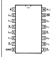
**DESCRIPTION** — The 'F258 is a quad 2-input multiplexer with 3-state outputs. Four bits of data from two sources can be selected using a common data select input. The four outputs present the selected data in the complement (inverted) form. The outputs may be switched to a high impedance state with a HIGH on the common Output Enable  $(\overline{OE})$  input, allowing the outputs to interface directly with bus oriented systems.
