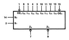
V<sub>CC</sub> = Pin 16 GND = Pin 8
