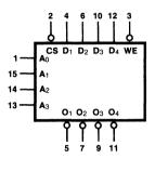
V<sub>CC</sub> = Pin 16 GND = Pin 8
