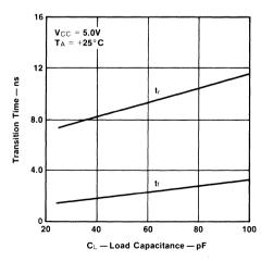
Fig. 2-13 Transition Time vs Load Capacitance
