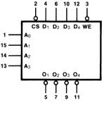
$V_{CC} = Pin 16$ GND = Pin 8
