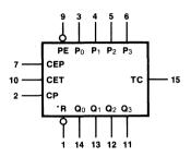
V<sub>CC</sub> = Pin 16 GND = Pin 8 \*MR for '160 \*SR for '162
