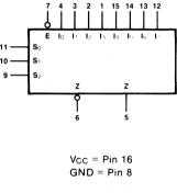
**FUNCTIONAL DESCRIPTION** — The 'F151 is a logical implementation of a single pole, 8-position switch with the switch position controlled by the state of three Select inputs,  $S_0$ ,  $S_1$ ,  $S_2$ . Both assertion and negation outputs are provided. The Enable input ( $\overline{E}$ ) is active LOW. When it is not activated, the negation output is HIGH and the assertion output is LOW regardless of all other inputs. The logic function provided at the output is:
