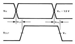
Fig. 2-23 Whether Response is Inverting or Non-Inverting Depends on Specific Truth Table Conditions
