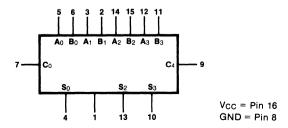
**FUNCTIONAL DESCRIPTION** — The 'F283 adds two 4-bit binary words (A plus B) plus the incoming carry  $C_0$ . The binary sum appears on the Sum ( $S_0 - S_3$ ) and outgoing carry ( $C_4$ ) outputs. The binary weight of the various inputs and outputs is indicated by the subscript numbers, representing powers of two.
