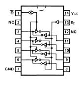
V<sub>CC</sub> = Pin 14 GND = Pin 7
