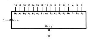
V<sub>CC</sub> = Pin 20 GND = Pin 10
