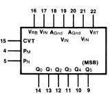
$V_{CC} = Pin 7$   $V_{EE} = Pins 1, 6$   $D_{Gnd} = Pin 8$ NC = Pins 2, 3
