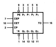
V<sub>CC</sub> = Pin 16 GND = Pin 8 \*MR for '161 \*SR for '163
