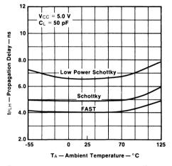
Fig. 2-10 Propagation Delay tPLH vs Temperature
