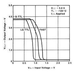
Fig. 2-6 Transfer Functions at High Temperature
