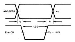
Fig. 2-30 Storage Address Setup and Hold Times
