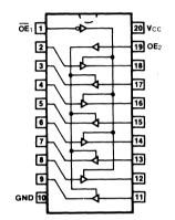
**DESCRIPTION** — The F240, 'F241 and 'F244 are octal buffers and line drivers designed to be employed as memory address drivers, clock drivers and bus oriented transmitters/receivers which provide improved PC board density.
