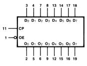
$V_{CC} = Pin 20$ GND = Pin 10
