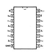
**DESCRIPTION** — The 'F157 is a high speed quad 2-input multiplexer. Four bits of data from two sources can be selected using the common Select and Enable inputs. The four buffered outputs present the selected data in the true non-inverted form. The 'F157 can also be used to generate any four of the 16 different functions to two variables.
