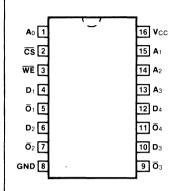
DESCRIPTION - The 'F189 ia a high speed 64-bit RAM organized as a 16word by 4-bit array. Address inputs are buffered to minimize loading and are fully decoded on-chip. The outputs are 3-state and are in the high impedance state whenever the Chip Select  $(\overline{CS})$  input is HIGH. The outputs are active only in the Read mode and the output data is the complement of the stored data. LOGIC SYMBOL
