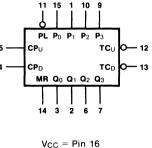
**FUNCTIONAL DESCRIPTION** — The 'F192 and 'F193 are asynchronously presettable decade and 4-bit binary synchronous up/down (reversible) counters. The operating modes of the 'F192 decade counter and the 'F193 binary counter are identical, with the only difference being the count sequences as noted in the State Diagram. Each circuit contains four edge-triggered flip-flops, with internal gating and steering logic to provide master reset, individual preset, count up and count down operations.
