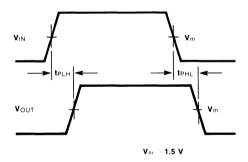
Fig. 2-19 Waveform for Non-Inverting Functions
