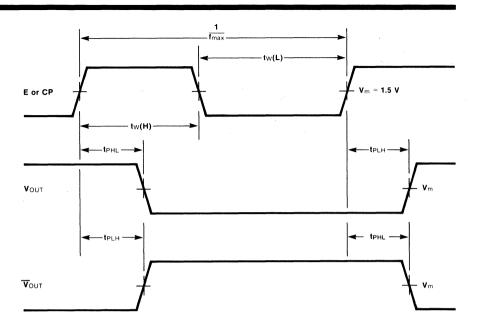
Fig. 2-21 Propagation Delays from Rising-Edge Clock or Enable
