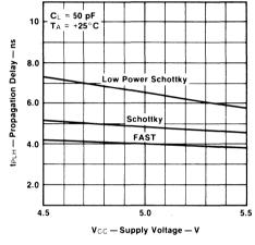
Fig. 2-8 Propagation Delay tPLH vs VCC
