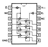
$V_{CC} = Pin 14$ GND = Pin 7
