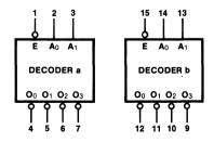
Vcc = Pin 16 GND = Pin 8 1-of-10 Decoder
