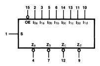
V<sub>CC</sub> = Pin 16 GND = Pin 8
