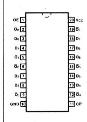
liminan DESCRIPTION - The F534 is a high speed, low power octal D-type flip-flop featuring separate D-type inputs for each flip-flop and 3-state outputs for bus oriented applications. A buffered Clock (CP) and Output Enable (OE) are common to all flip-flops. The 'F534 is the same as the 'F374 except that the outputs are inverted.
