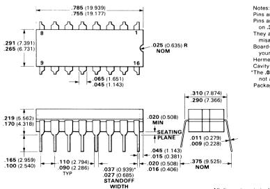
Pins are tin-plated 42 alloy Pins are intended for insertion in hole rows on .300 (7.62) centers
