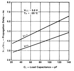
Fig. 2-12 Propagation Delay vs Load Capacitance
