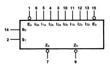
V<sub>CC</sub> = Pin 16 GND = Pin 8
