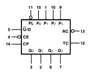
V<sub>CC</sub> = Pin 16 GND = Pin 8
