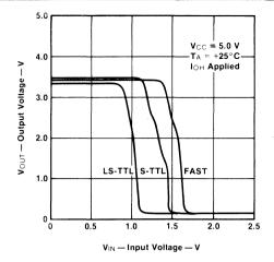
Fig. 2-5 Transfer Functions at Room Temperature
