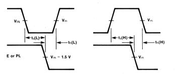
Fig. 2-29 Setup and Hold Times to Active-HIGH Enable or Parallel Load
