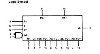
V<sub>CC</sub> = Pin 20 GND = Pin 10
