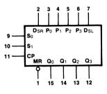
V<sub>CC</sub> = Pin 16 GND = Pin 8
