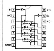
retiminati DESCRIPTION --- The 'F242 and 'F243 are quad bus transmitters/receivers designed for 4-line asynchronous 2-way data communications between data buses.
