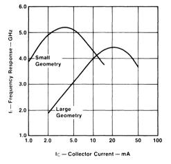
Fig. 2-2 Isoplanar Transistor Frequency Response
