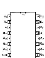
CONNECTION DIAGRAM PINOUT A
