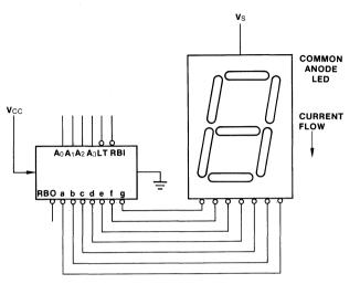
Fig. c Separate Supply for LED Displays
