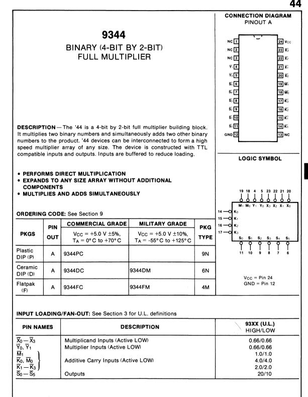
**FUNCTIONAL DESCRIPTION** — The '44 is a binary full multiplier for 4-bit by 2-bit words. It is easily expandable in an array to form a high speed parallel multiplier of any length. The functional equation is illustrated below:
