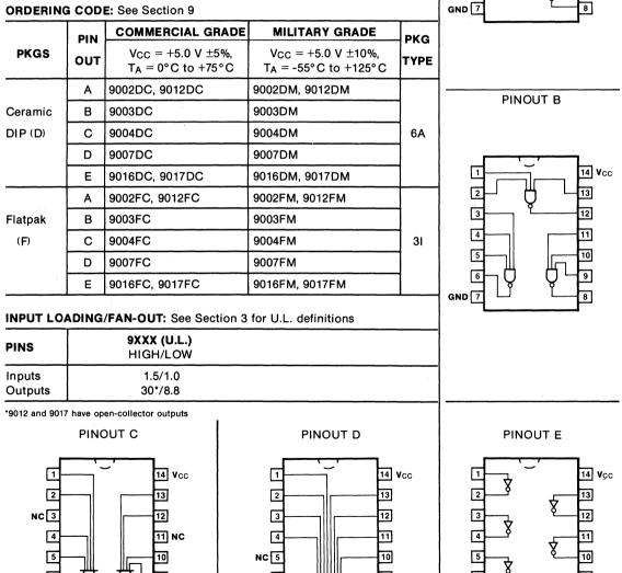
CONNECTION DIAGRAMS PINOUT A
