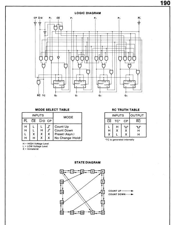
**FUNCTIONAL DESCRIPTION** — The '190 is a synchronous up/down BCD decade counter and the '191 is a synchronous up/down 4-bit binary counter. The operating modes of the '190 decade counter and the '191 binary counter are identical, with the only difference being the count sequences as noted in the state diagrams. Each circuit contains four master/slave flip-flops, with internal gating and steering logic to provide individual preset, count-up and count-down operations.
