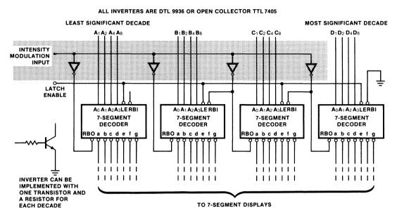
Fig. d Intensity Control by RBO Pulse Duty Cycle
