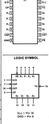
CONNECTION DIAGRAM PINOUT A
