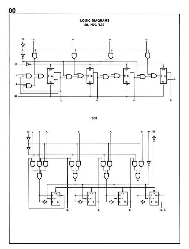
**FUNCTIONAL DESCRIPTION** — The Logic Diagrams and Truth Table indicate the functional characteristics of the '00 4-bit shift register. The device is useful in a wide variety of shifting, counting and storage applications. It performs serial, parallel, serial-to-parallel, or parallel-to-serial data transfers.
