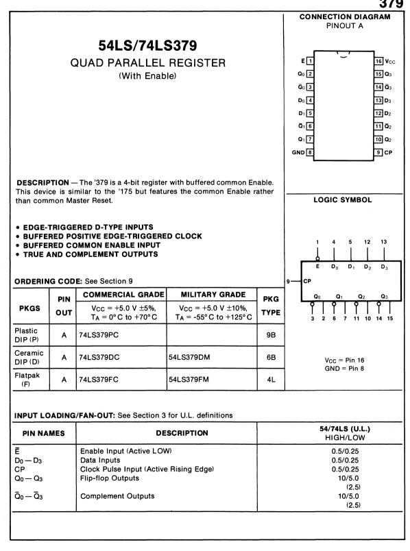
FUNCTIONAL DESCRIPTION - The '379 consists of four edge-triggered D-type flip-flops with individual D inputs and Q and Q outputs. The Clock (CP) and Enable (E) inputs are common to all flip-flops. When the E input is HIGH, the register will retain the present data independent of the CP input. The D<sub>n</sub> and  $\overline{E}$  inputs can change when the clock is in either state, provided that the recommended setup and hold times are observed.
