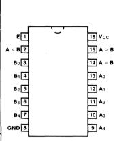
**FUNCTIONAL DESCRIPTION** — The '24 5-bit comparators use combinational circuitry to directly generate "A greater than B" and "A less than B" outputs. As evident from the logic diagram, these outputs are generated in only three gate delays. The "A equals B" output is generated in one additional gate delay by decoding the "A neither less than nor greater than B" condition with a NOR gate. All three outputs are activated by the active LOW Enable Input ( $\overline{E}$ ).
