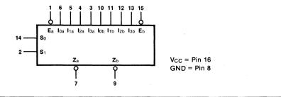
CONNECTION DIAGRAM PINOUT A
