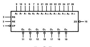
V<sub>CC</sub> = Pin 28 GND = Pin 14
