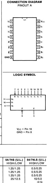
**DESCRIPTION** — The '151 is a high speed 8-input digital multiplexer. It provides in one package, the ability to select one line of data from up to eight sources. The '151 can be used as a universal function generator to generate any logic function of four variables. Both assertion and negation outputs are provided.
