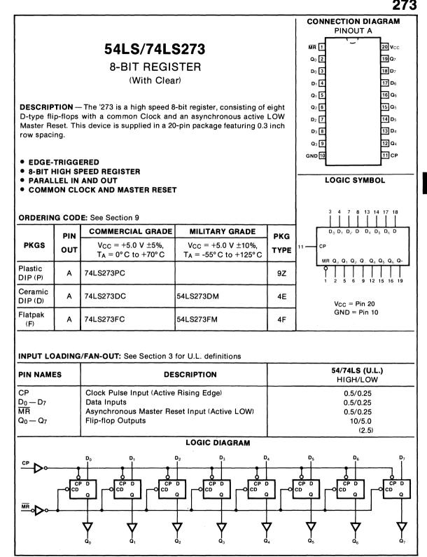
**FUNCTIONAL DESCRIPTION** — The '273 is an 8-bit parallel register with a common Clock and common Master Reset. When the  $\overline{MR}$  input is LOW, the Q outputs are LOW, independent of the other inputs. Information meeting the setup and hold time requirements of the D inputs is transferred to the Q outputs on the LOW-to-HIGH transition of the clock input.
