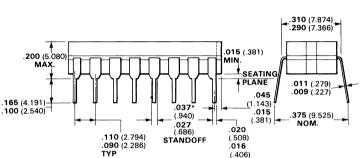
NOTES: Pins are tin-plated 42 alloy Pins are intended for insertion in hole rows on .300" (7.62) centers
