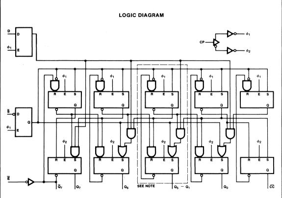
Note: Cell logic is repeated for register stages Q5 to Q1.
