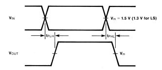
Fig. 3-20 Whether Response is Inverting or Non-Inverting Depends on Specific Truth Table Conditions
