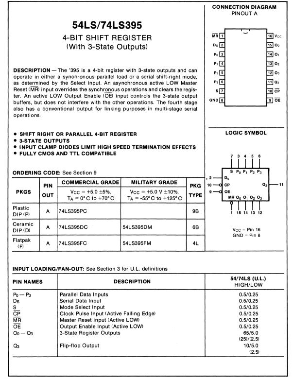
**FUNCTIONAL DESCRIPTION** — The '395 contains four D-type edge-triggered flip-flops and auxiliary gating to select a D input either from a Parallel ( $P_n$ ) input or from the preceding stage. When the Select input is HIGH, the  $P_n$  inputs are enabled. A LOW signal on the S input enables the serial inputs for shift-right operations, as indicated in the Truth Table.
