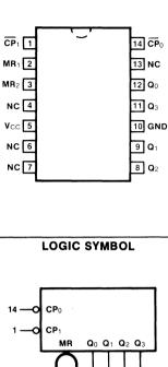
CONNECTION DIAGRAM **PINOUT A**
