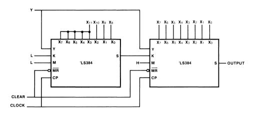
Fig. c A 12-Bit by N-Bit Two's Complement Multiplier
