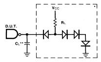
\*Not Used for LS-TTL \*\*Includes Jig and Probe Capacitance
