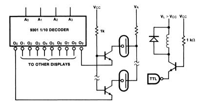
Fig. 2-33 Non-Inverting High Voltage Drivers
