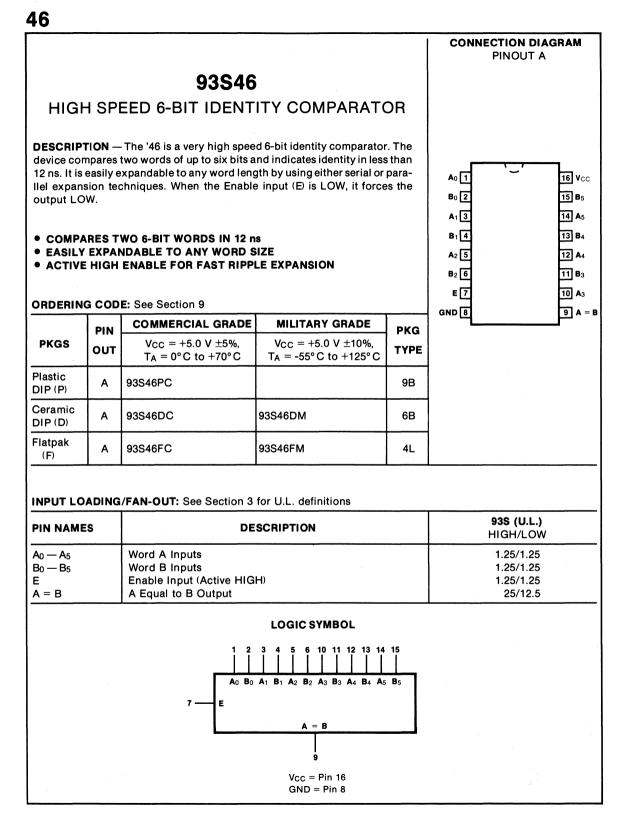
**FUNCTIONAL DESCRIPTION** — The '46 is a very high speed 6-bit identity comparator. The A = B output is HIGH when the Enable (E) is HIGH and the two 6-bit words are equal. Equality is determined by Exclusive-NOR circuits which individually compare the equivalent bits from each word. When any two of the equivalent bits from each word have different logic levels, the A = B output is LOW.
