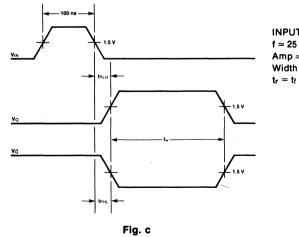
$\begin{array}{l} \text{INPUT PULSE} \\ \text{f} \simeq 25 \text{ kHz} \\ \text{Amp} \simeq 3.0 \text{ V} \\ \text{Width} \simeq 100 \text{ ns} \\ \text{t}_r = \text{t}_f \leq 10 \text{ ns} \end{array}$
