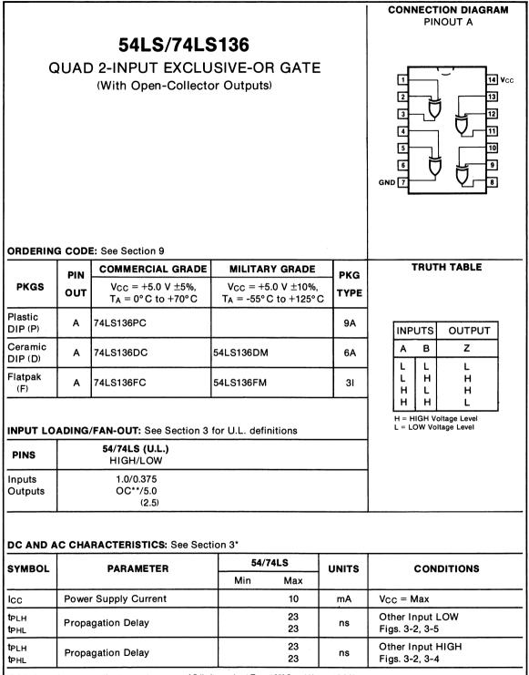
\*DC limits apply over operating temperature range; AC limits apply at  $T_A = +25^{\circ}$  C and  $V_{CC} = +5.0$  V.
