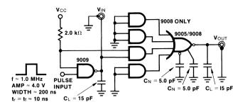
Note: Capacitance includes probe and jig capacitance
