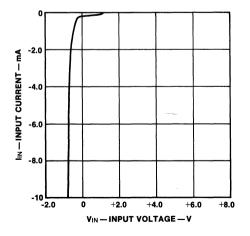
Fig. 2-11 LS-TTL Input Characteristics
