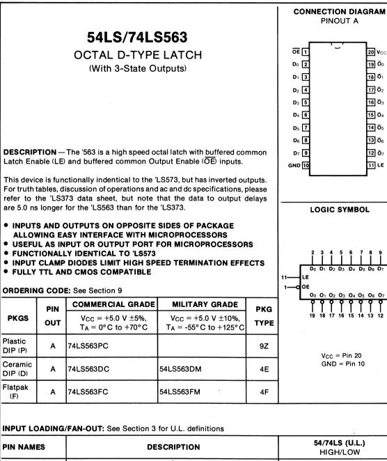
$D_0 - D_7$ Data Inputs0.5/0.25LELatch Enable Input (Active HIGH)0.5/0.25 $\overline{OE}$ 3-State Output Enable Input (Active LOW)0.5/0.25 $\overline{O}_0 - \overline{O}_7$ 3-State Latch Outputs65/15(25)/(7.5)(25)/(7.5)
