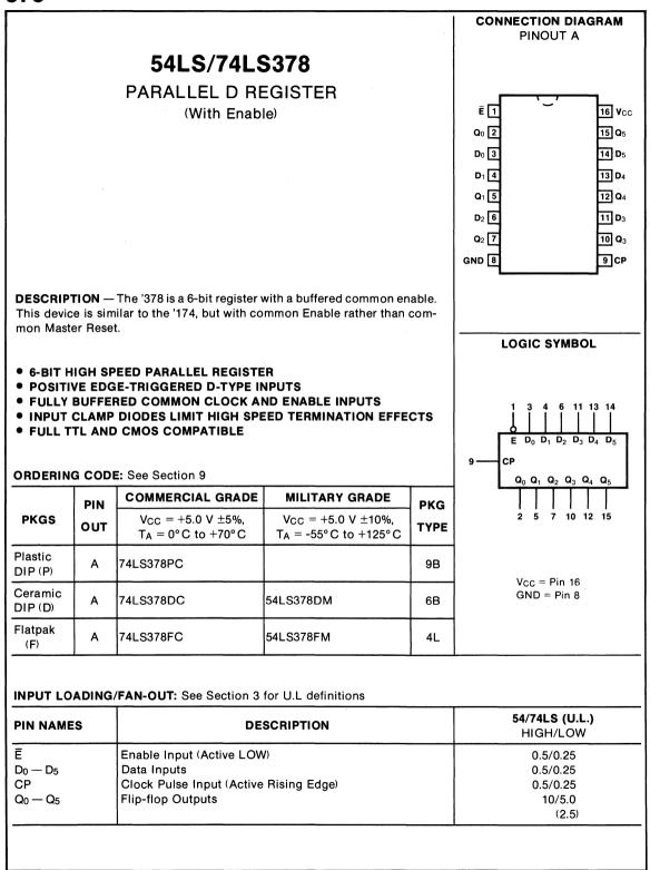
**FUNCTIONAL DESCRIPTION** — The '378 consists of eight edge-triggered D-type flip-flops with individual D inputs and Q outputs. The Clock (CP) and Enable  $(\vec{E})$  inputs are common to all flip-flops.
