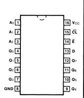
CONNECTION DIAGRAM PINOUT A
