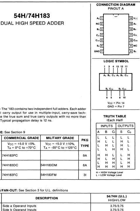
DESCRIPTION - The '183 contains two independent full adders. Each adder has an individual carry output for use in multiple-input, carry-save techniques to produce the true sum and true carry outputs with no more than two gate delays. Typical propagation delay is 12 ns.
