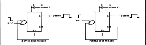
4. An overriding active LOW level direct clear is provided on each multivibrator. By applying a LOW to the clear, any timing cycle can be terminated or any new cycle inhibited until the LOW reset input is removed. Trigger inputs will not produce spikes in the output when the reset is held LOW. A LOW-to-HIGH transition on C
