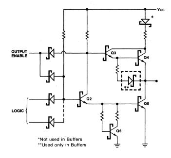
Fig. 2-18 Typical 3-State Output Control
