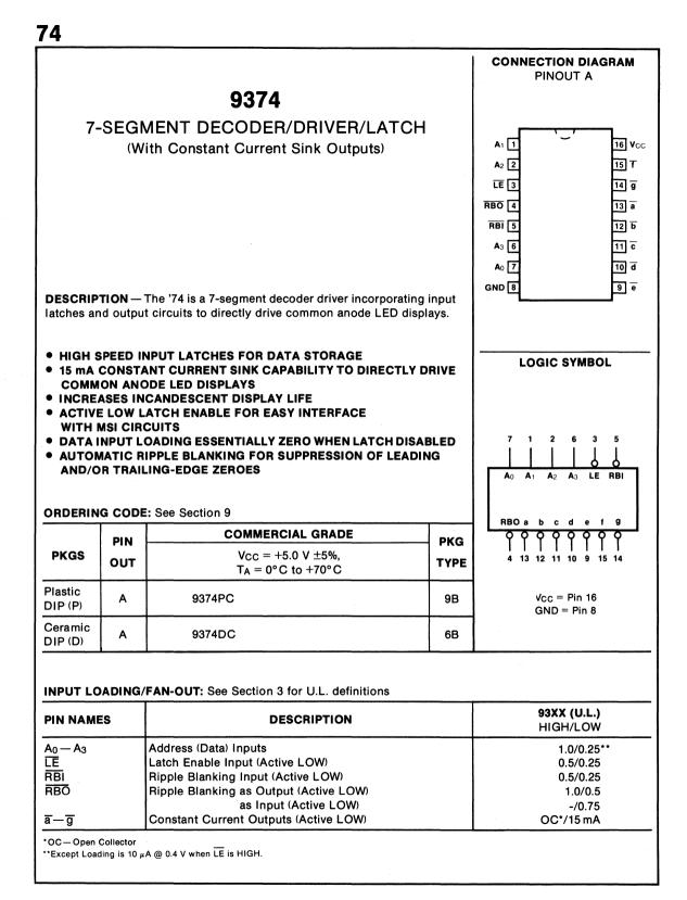
**FUNCTIONAL DESCRIPTION**—The '74 is a 7-segment deconder/driver with latches on the address inputs and active LOW constant current outputs to drive LEDs directly. This device accepts a 4-bit binary code and produces output drive to the appropriate segments of the 7-segment display. It has a decode format which produces numeric codes "0" through "9" and other codes.
