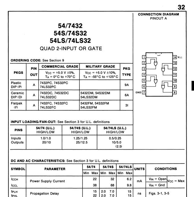
\*DC limits apply over operating temperature range; AC limits apply at  $T_A = +25^{\circ}$  C and  $V_{CC} = +5.0$  V.
