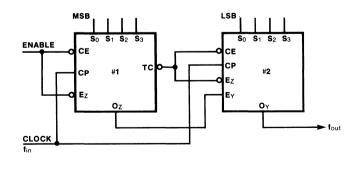
Fig. a Cascading for 2-Digit Rate Select
