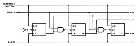
Fig. c Synchronous N-Stage Counter with Parallel Gated Carry/Borrow
