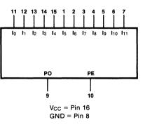
**FUNCTIONAL DESCRIPTION** — The '48 is a 12-input parity generator. It provides odd and even parity for up to 12 data bits. The Even Parity output (PE) will be HIGH if an even number of logic ones are present on the inputs. The Odd Parity output (PO) will be HIGH if an odd number of logic ones are present on the inputs. The logic equations for the outputs are shown below.
