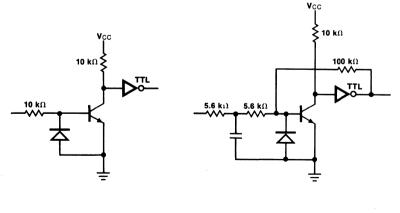
Fig. 2-34 Transistors Driving TTL
