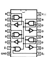
CONNECTION DIAGRAM PINOUT A
