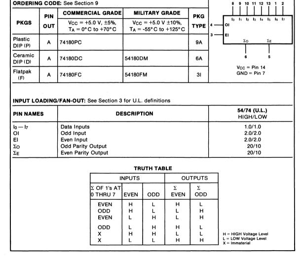
**DESCRIPTION** — The '180 is a monolithic. 8-bit parity checker/generator which features control inputs and even/odd outputs to enhance operation in either odd or even parity applications. Cascading these circuits allows unlimited word length expansion. Typical application would be to generate and check parity on data being transmitted from one register to another. Typical power dissipation is 170 mW.
