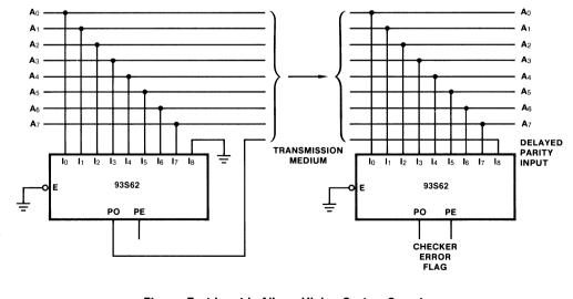
Fig. a Fast Input I<sub>8</sub> Allows Higher System Speed
