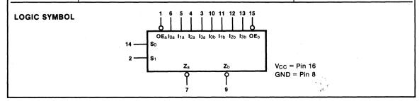
**FUNCTIONAL DESCRIPTION** — The '353 contains two identical 4-input multiplexers with 3-state outputs. They select two bits from four sources selected by common Select inputs (S<sub>0</sub>, S<sub>1</sub>). The 4-input multiplexers have individual Output Enable ( $\overline{OE}_a$ ,  $\overline{OE}_b$ ) inputs which when HIGH, force the outputs to a high impedance (high Z) state. The logic equations for the outputs are shown below:
