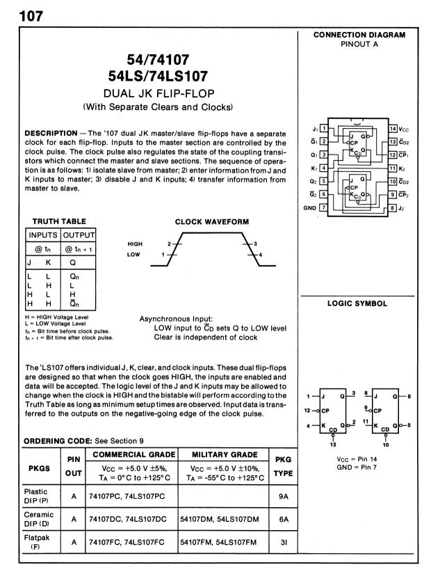
INPUT LOADING/FAN-OUT: See Section 3 for U.L. definitions
