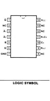
CONNECTION DIAGRAM PINOUT A
