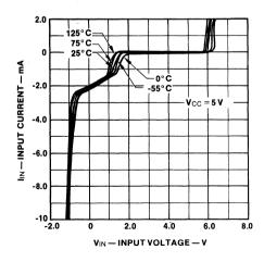
Fig. 2-10 TTL Buffer Input Characteristics
