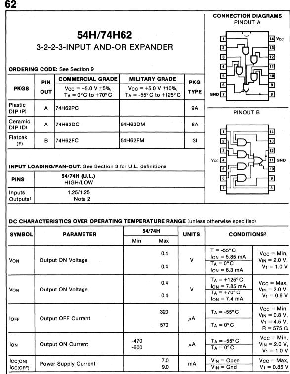
1. A maximum of one expander may be connected to one expandable AND-OR-Invert gate
