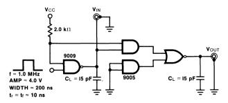
Note: Capacitance includes probe and jig capacitance
