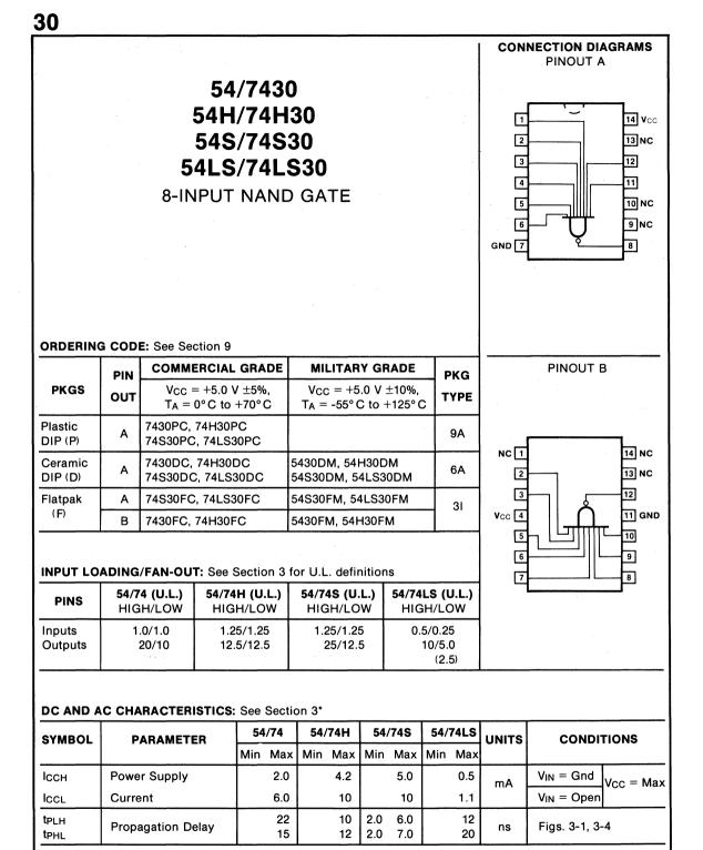
\*DC limits apply over operating temperature range; AC limits apply at  $T_A = +25^{\circ}$ C and  $V_{CC} = +5.0$  V.
