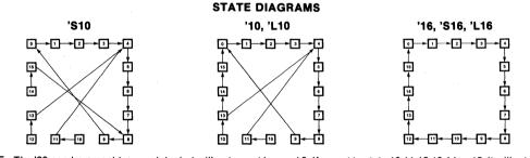
NOTE: The '20 can be preset to any state, but will not count beyond 9. If preset to state 10,11,12,13,14 or 15, it will return to its normal sequence within two clock pulses.
