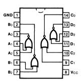
$V_{CC} = Pin 8$ GND = Pin 1
