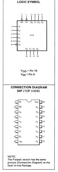
**FUNCTIONAL DESCRIPTION** – The 4710 consists of a 16  $\times$  4-bit RAM selected by four address inputs (A<sub>0</sub> – A<sub>3</sub>) and an edge-triggered 4-bit Output Register with 3-state Output Buffers.
