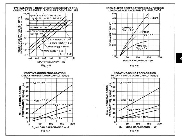
The best choice for slow applications is 5 V. For reasonably fast systems, choose 10 or 12 V. Any application requiring 15 V to achieve short delays and fast operation should be investigated for excessive power dissipation and should be weighed against an LS-TTL approach.
