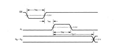
Fig. 16 FALL THROUGH TIME Conditions: TTS connected to IRF, TOS connected to ORE, IES, OES, EO, CPSO LOW, TOP HIGH
