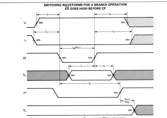
PROPAGATION DELAY, CP TO  $\overline{0}_n$  , MINIMUM  $\overline{EX}$  PULSE WIDTH AND SET-UP AND HOLD TIMES,  $I_n$  TO  $\overline{EX}$  ,  $\overline{EX}$  TO CP AND  $I_n$  TO CP
