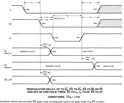
NOTES: a. Condition which occurs when EX goes LOW considerably before CP goes LOW (T<sub>s1</sub>EX is met). b. Condition which occurs when EX goes LOW slightly before or after CP goes LOW (Either t<sub>s2</sub>EX or t<sub>s3</sub>EX are met). c. Set-up and Hold Times are shown as positive values but may be specified as negative values.
