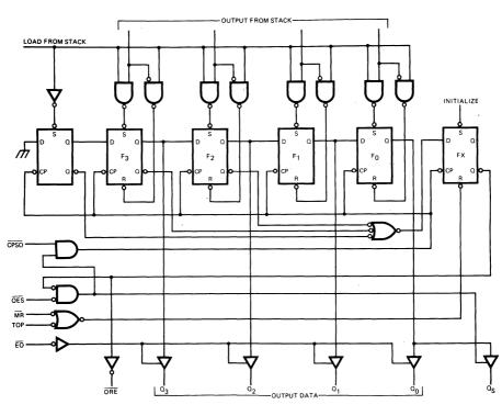
Fig. 3 CONCEPTUAL OUTPUT SECTION
