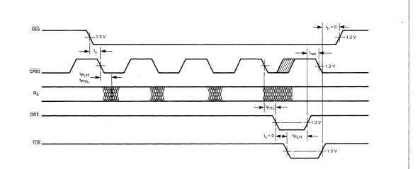
Fig. 14 SERIAL OUTPUT, SLAVE OPERATION Conditions: data in stack, TOP HIGH, IES HIGH when initiated
