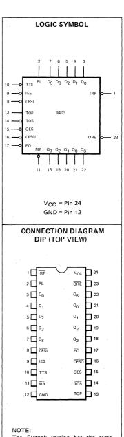
The Flatpak version has the same pinouts (Connection Diagram) as the Dual In-line Package.
