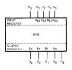
Fig. 2 FINAL POSITIONS IN A 9403 RESULTING FROM A 64-BIT SERIAL TRAIN **Output Register (Data Extraction)** – The Output Register receives 4-bit data words from the bottom stack location, stores it and outputs data on a 3-state 4-bit parallel data bus or on a 3-state serial data bus. The output section generates and receives the necessary status and control signals. *Figure 3* is a conceptual logic diagram of the output section.
