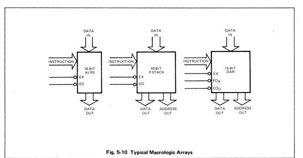
The instruction inputs of the arrays must be controlled by the microinstruction fields. However, what are the chances of two different Macrologic arrays performing two different operations on the same input data during the same clock cycle? This situation occurs very rarely; therefore, individual control fields are seldom needed.
