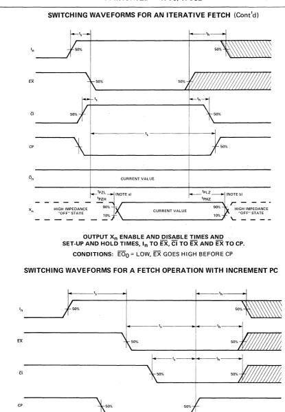
NOTES: a.  $X_0 - X_3$  turn on delay measured from time both  $\overline{\text{EX}}$  and CP go LOW. b.  $X_0 - X_3$  turn off delay measured from time either  $\overline{\text{EX}}$  or CP goes HIGH.
