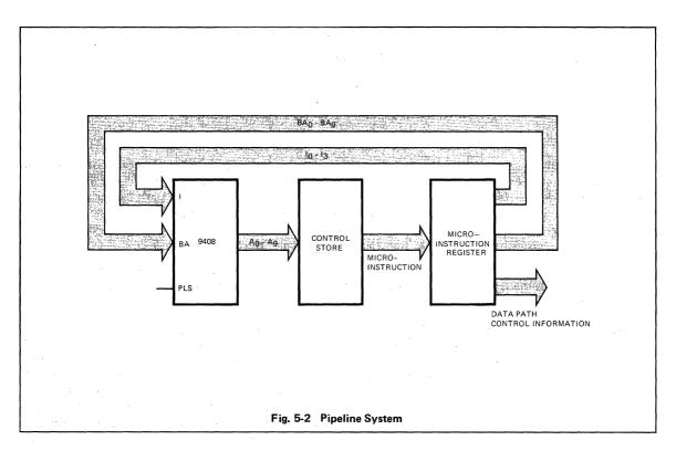
In many instances, a microprogram written for non-pipeline system cannot be executed in pipeline mode. However, 9408 architecture is designed so that the same microprogram can be executed in pipeline or non-pipeline mode without any modification. This feature gives the user a distinct advantage since he can design his high end product with pipeline execution and lower end product with non-pipeline. No microprogram changes are required thus significant cost advantages can be realized.
