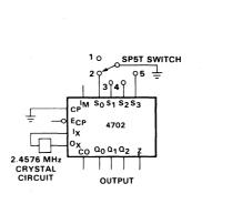
ate enerator Configuration Providing 5 Bit Rates
