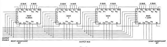
Fig. 1 16-BIT 9404 ARRAY
