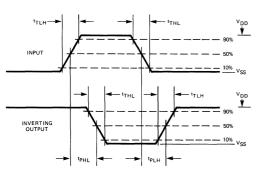
Fig. 4-16 Propagation Delay, Transition Time
