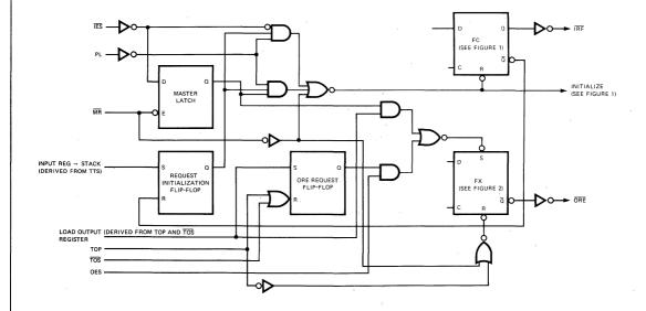
Fig. 10 CONCEPTUAL DIAGRAM, INTERLOCKING CIRCUITRY
