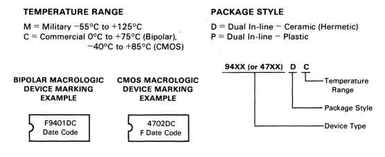
In order to accommodate varying die sizes (MSI, LSI, etc.), numbers of pins (16, 18, 24, etc.), and package outlines, a number of different package forms are required in each of the three package style categories.
