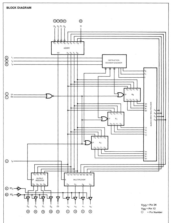
**FUNCTIONAL DESCRIPTION** – The 4707 contains a 4-bit slice of three registers ( $R_0 - R_2$ ), a 4-Bit Adder, 3-state address output buffers ( $X_0 - X_3$ ) and a separate Output Register with 3-state buffers ( $\overline{O}_0 - \overline{O}_3$ ), allowing output of the register contents on the data bus (refer to the block diagram). The DAR performs 16 instructions, selected by  $I_0 - I_3$  inputs, as listed in *Table 1*.
