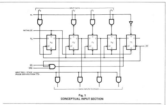
Serial Entry – Data on the D<sub>S</sub> input is serially entered into the F<sub>3</sub>, F<sub>2</sub>, F<sub>1</sub>, F<sub>0</sub>, FC shift register on each HIGH-to-LOW transition of the CPSI clock input, provided IES and PL are LOW.
