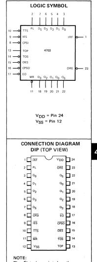
The Flatpak version has the same pinouts (Connection Diagram) as the Dual In-line Package.
