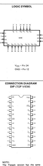
pinouts (Connection Diagram) as the Dual In-line Package.
