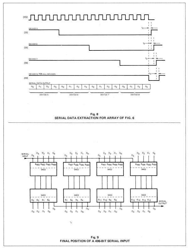
Interlocking Circuitry – Most conventional FIFO designs provide status signals analogous to IRF and ORE. However, when these devices are operated in arrays, variations in unit to unit operating speed require external gating to assure all devices have completed an operation. The 9403 incorporates simple but effective "master/slave" interlocking circuitry to eliminate the need for external gating.
