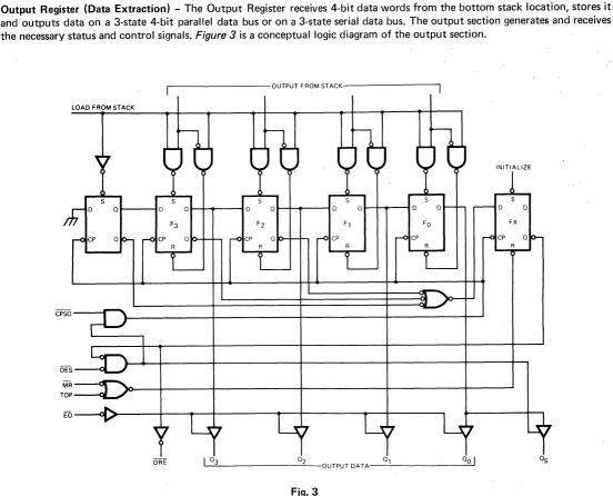
Fig. 3 CONCEPTUAL OUTPUT SECTION
