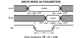
Fig. 3 WRITE ENABLE PULSE WIDTH, SET-UP AND HOLD TIMES ADDRESS AND DATA TO WRITE ENABLE
