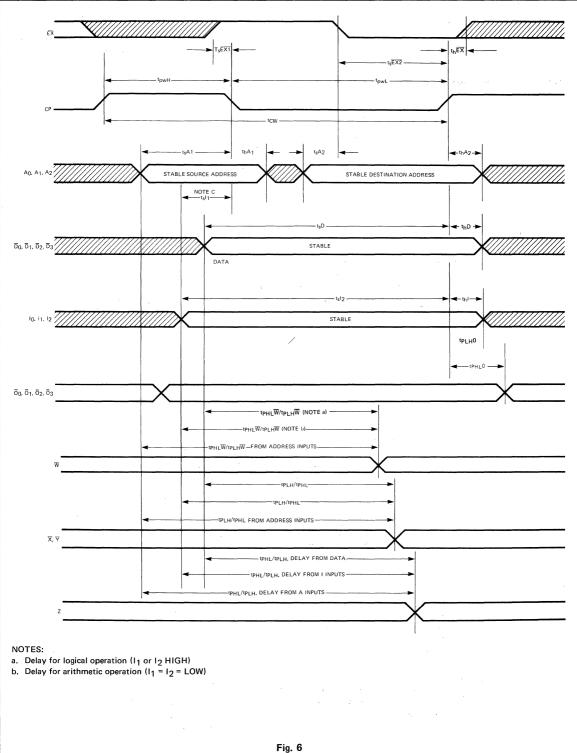
ALRS TIMING DIAGRAM-TWO ADDRESS MODE
