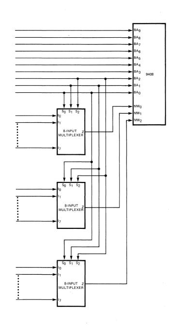
Fig. 5-6 Expanding Multiway Inputs
