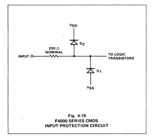
parasitic substrate diode would represent a poorly defined shunt to  $V_{SS}$  in this particular case.
