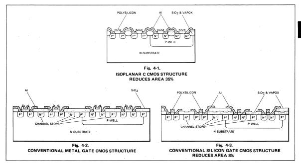
Originally designed for aerospace applications, CMOS now finds its way into portable instruments, industrial and medical electronics, automotive applications and computer peripherals, besides dominating the electronic watch market.
