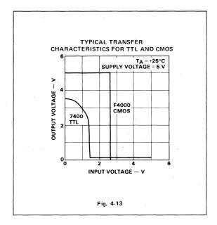
noise filter; 10 ns spikes tend to disappear in a chain of CMOS gates, but are amplified in a chain of TTL gates. Because of these features, CMOS is very popular with designers of industrial control equipment that must operate in an electrically and electromagnetically "polluted" environment.
