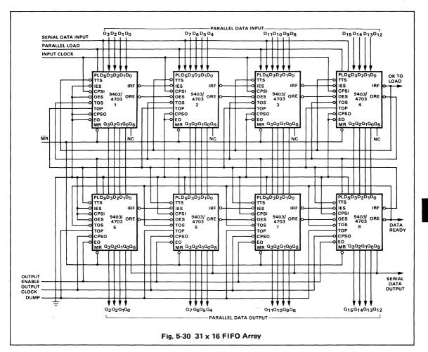
The D<sub>S</sub> inputs of the first four devices are bussed together and serial data is entered on this line. The CPSI inputs are also connected together for clocking the serial data. The IES input of device 1 is connected to ground, while the IES inputs of devices 2, 3 and 4 are each connected to the IRF output of the preceding device. The IRF output of device 4 feeds into the TTS inputs of all four devices.
