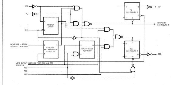
Fig. 10 CONCEPTUAL DIAGRAM, INTERLOCKING CIRCUITRY
