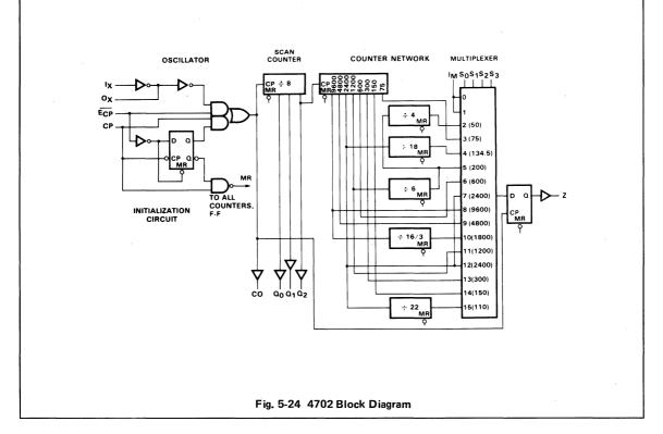
this counter provides another benefit, *i.e.*, it moves the input frequency to 2.4576 MHz which is ideal for low-cost crystals. If it were not for the scan counter, the 4702 would require a more expensive crystal of about 300 kHz.
