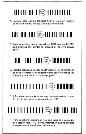
Figure 6. Examples of FIFO Handling of Differing Data Rates
