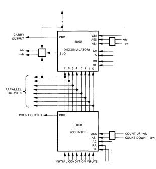
The DDA shown above utilizes one 3800 for a remainder register and a second 3800 for a y accumulator counter.
