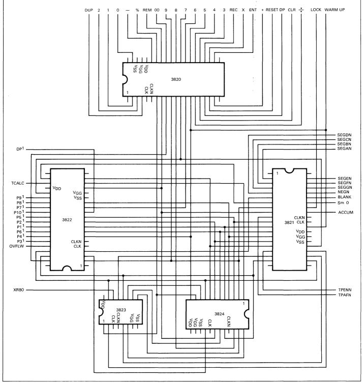
Fig. C-1. SPRINT Calculator Set Connection Diagram
