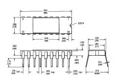
NOTES: All dimensions in inches Leads are intended for insertion in hole rows on .300" centers. They are purposely shipped with "positive" misalignment to facilitate insertion. Board-drilling dimensions should equal your practice for .020" diameter lead Leads are gold-plated kovar Package weight is 1.3 grams
