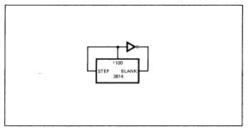
Fig. 11. Self-driven multiplexer with blanking between digits.
