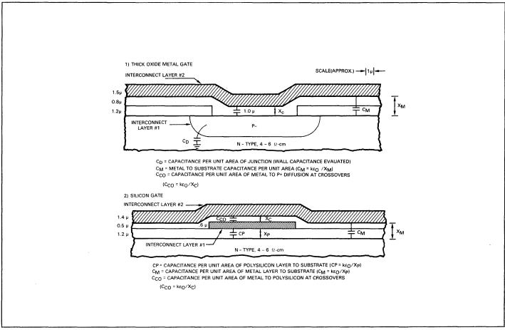
Fig. G-3. Thick Oxide Metal Gate (Top) and Silicon Gate Interconnection Segments and Capacitance Components
