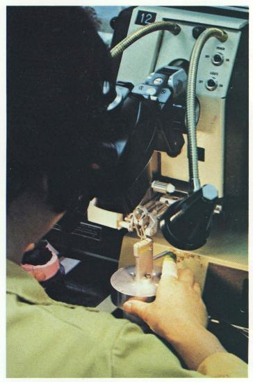
Wire bonding connects the pads on the die to the leads of the package.
