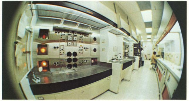
Diffusion furnaces drive controlled impurities into silicon to form parts of the MOS transistors.
