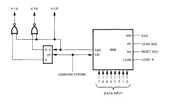
COMPARE OPERATION: To compare two numbers, simply insert the first into a previously cleared accumulator by pulsing ac. Enabling the subtract control will immediately indicate whether R>A, as a borrow output will appear. If the borrow output follows a pulse on the borrow input, the numbers are equal. If neither, then R<A. The logic is shown to the left.
