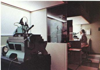
Silicon wafers become photographic plates after being coated with a layer of etch resist. The resist is then baked. These photo steps are all performed in a room with controlled lighting.
