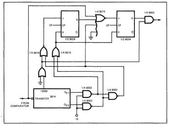
Fig. 10. Blinking under range indicator.
