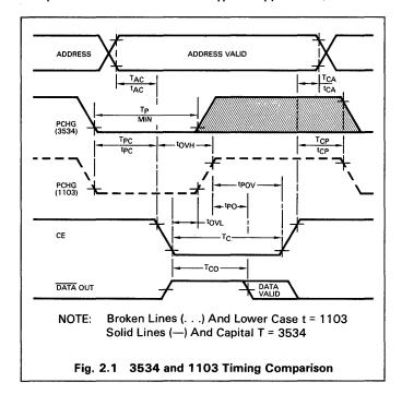
The elimination of overlap constraints provides another important system benefit, illustrated by the relationship between the leading edge of CE and valid DATA OUT. Data is available  $T_{CO}$  (165 ns max) after CE on the 3534 and is not referenced to the trailing (positive-going) edge of PCHG as in the 1103. At the system level, this eliminates the clock skew associated with the rising edge of PCHG, providing faster access and cycle times in a worst case design.
