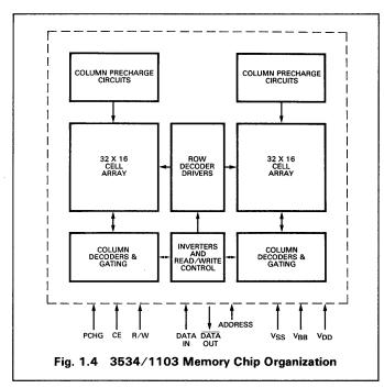
The peripheral circuits must perform a number of functions including address inversion, control signal inversion, address decoding, row and column selection, read/write cycle control, and data input/output buffering. Figure 1.5 is a partial schematic diagram of the 3534/1103 and identifies the memory cell and its interconnection with this support circuitry. A description of the function and operation of the peripheral circuits follows.
