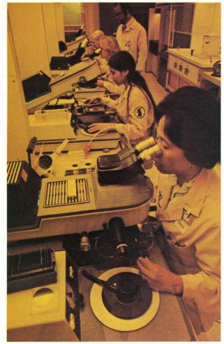
In these mask aligners, new mask patterns (from working plate) are aligned to the existing pattern on the wafer. A box of working plates is shown in foreground.
