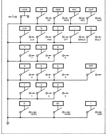
Fig. C-3. Keyboard Switch Schematic Single Pole Single Throw Switches
