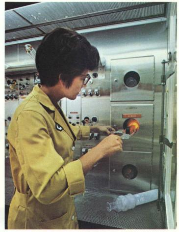
Wafers being unloaded from silicon reactor.
