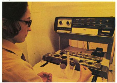
The coated wafers are stored in lightfiltered boxes prior to exposure.
