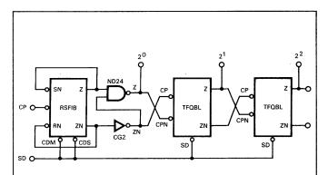
Ripple counter with asynchronous reset to all "1"s is clocked by an RSF1 master/slave flip-flop with the aid of NAND and clock generator cells. The RSF1 operates at 1 MHz and the TFQBL to 500 kHz with 0.5-pF loads connected to the counter outputs. Each TFQBL dissipates an average of 0.625 mW.
