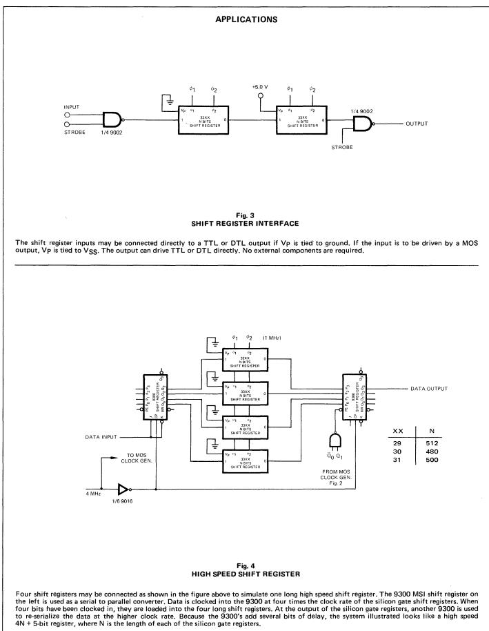
Note that the clock period of the 9300's must be greater than the input set up time on the silicon gate registers.
