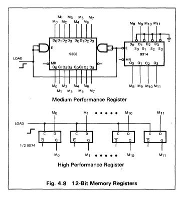
A register is usually required for output data and may also be required to latch input data. The device types used for the address register may also be used to construct data registers. With some additional gating, one register can be used for both input and output data.
