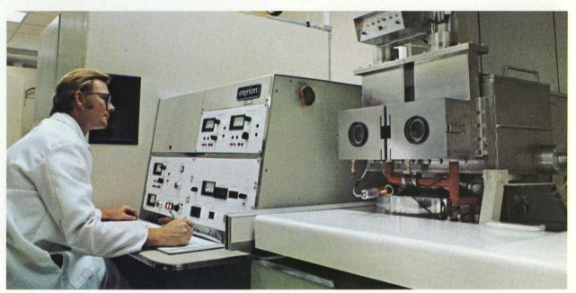
lon implantation equipment installed in production diffusion room for use with Isoplanar to provide superior density and performance.
