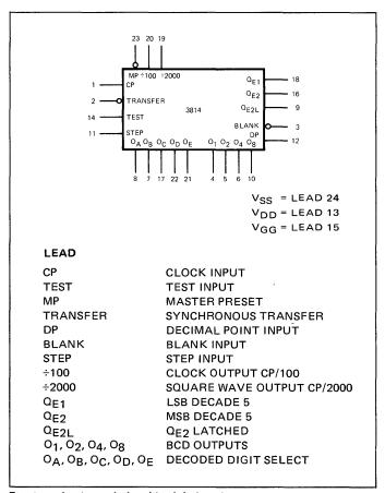
Fig. 1. Logic symbol and lead designation.
