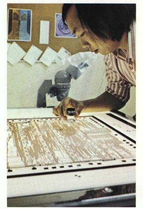
An 80X blowup of the artwork, is made for alignment and circuit verification.
