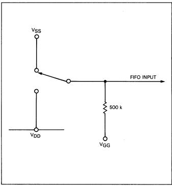
Figure 5. Switch Bounce Eliminator Using 3341 Unique Input Pullup Circuit
