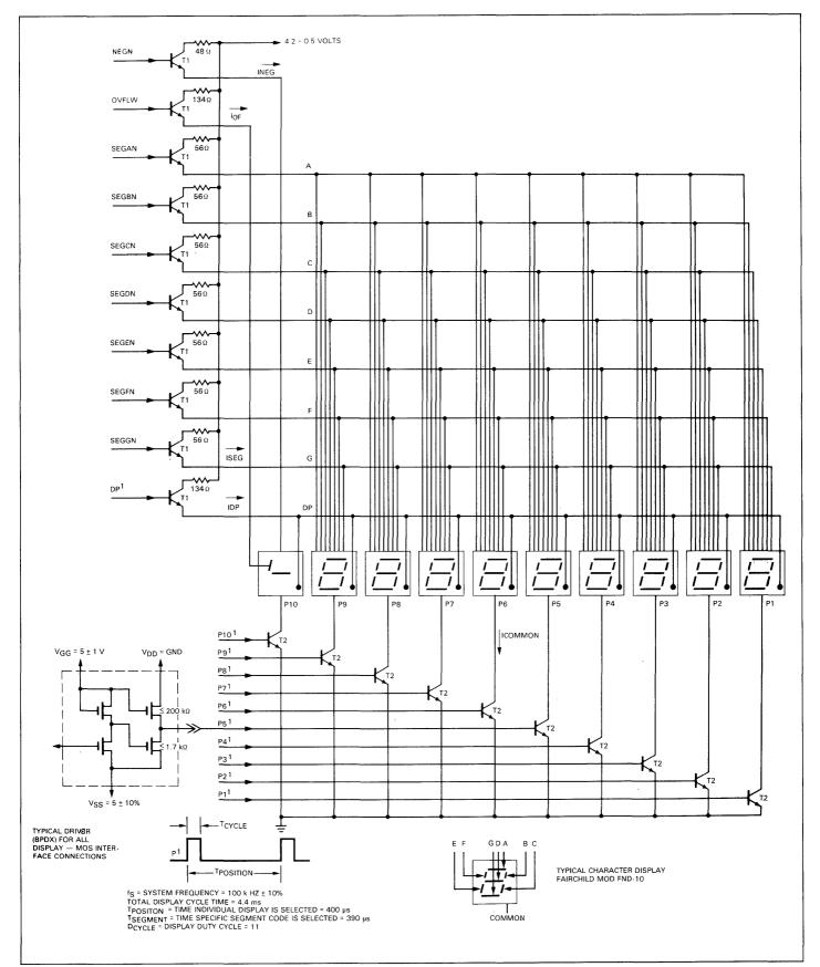
Fig. C-5. Light Emitting Diode Display System Schematic
