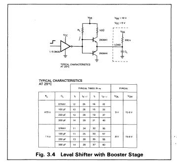
The mutual inductance associated with the PC tracks may cause ringing on the level shifter outputs due to the high peak currents. Typical inductance ranges from 10 to 20 nH/inch with 15 mil tracks. Therefore, current limiting resistors in the level shifter output stage or external series damping resistors may be required. Short line lengths and careful layout practices should minimize this effect.
