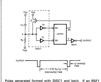
Pulse generated formed with DISC1 and latch. If an RSF1 flip-flop cell, connected as a toggle flip-flop, is used instead of a latch, the circuit becomes a square wave generator. Q is a discharge transistor.
