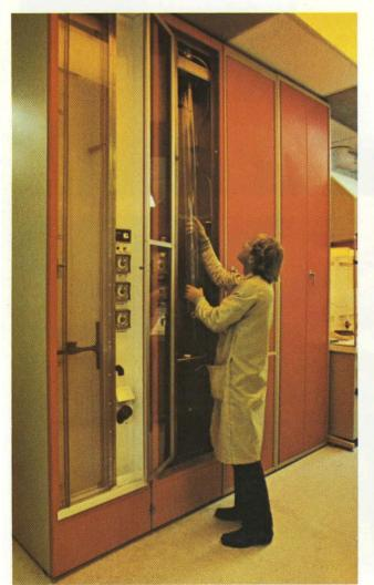
The diffusion furnace tubes are regularly cleaned by flushing with HF (hydrofloric acid), rinsed with DI water and dried with N2.
