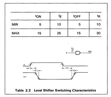
Assuming that the simplified timing and the level shifter characteristics are feasible, a comparison can be made between the 1103 and the 3534 operating in the same system. A memory cycle begins when a positive level is propagated down the delay line at  $t_0$ . At  $t_1$ , CHIP ENABLE time occurs and the CE level shifter output is guaranteed to be LOW after a delay. Therefore,
