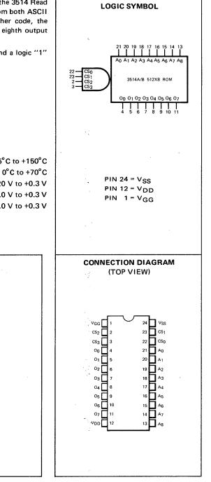
**FUNCTIONAL DESCRIPTION** — The 3514A and 3514B, Note 1, contain the complete code conversion bit pattern to convert any 7-bit ASCII code to EBCDIC or any 8-bit EBCDIC code to ASCII. Address A<sub>0</sub> through A<sub>6</sub> and outputs O<sub>0</sub> through O<sub>6</sub> correspond to the two basic codes as follows:
