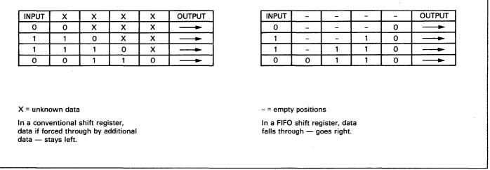
Figure 2. Input Data Storage in Conventional Shift Register Compared to FIFO Shift Registers
