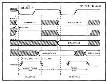
Fig. 5 Memory Interface Timing 256x8
