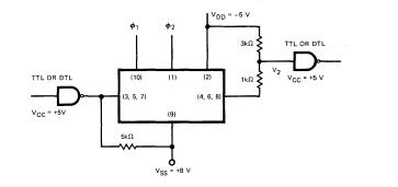
Clock amplitude  $V_{\phi}$  = +8 V to -16 V. Clock pulse width tpW ≥150 ns.
