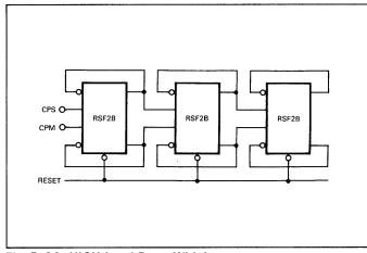
Fig. D-24. HIGH-Level Reset With Inverters
