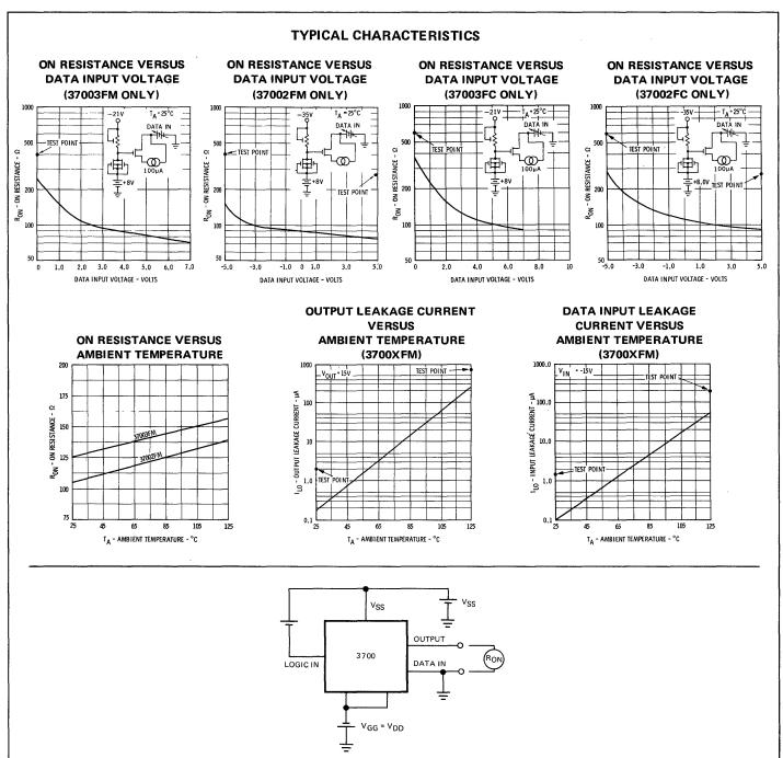
Voltage levels between semiconductor electrodes are normally referenced to one of the electrodes. In MOS, this electrode is the substrate (body). The voltages can be translated to an equivalent level and referenced to another electrode. In order to measure the ON resistance of the data channel accurately, the data input is at ground potential and all other terminals are changed correspondingly to test worst case conditions.
