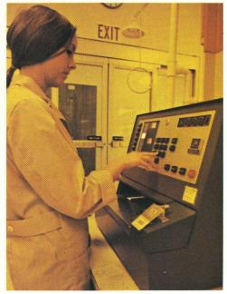
Wafer movement is recorded in a production control terminal that maintains control of all material in the production flow.
