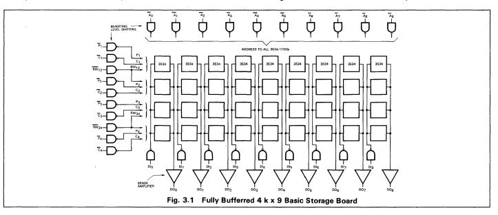
To reduce power dissipation on the board, PRECHARGE is decoded and inputs  $P_1$  and  $P_4$  select the memory row to be precharged. This allows a memory design in which only the accessed devices dissipate power during a cycle. For a refresh cycle, the storage board is refreshed by enabling all of the PRECHARGE and CHIP ENABLE inputs, simultaneously refreshing all four rows.
