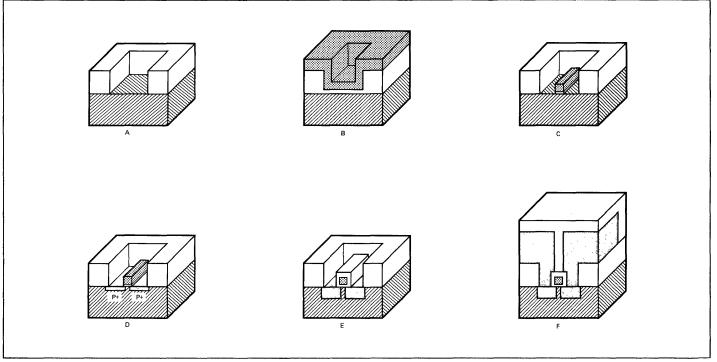
Fig. G-2. Silicon Gate Process Steps
