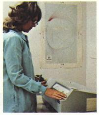
Film thickness measurements are made on an interferometer. Thickness can also be monitored on an ellipsometer (see chart on wall).
