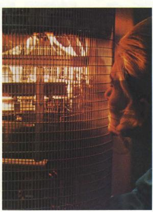
Aluminum metal is deposited in vacuum chambers. A planatary gear arrangement insures that the metal forms evenly over the steps in the oxide surface.
