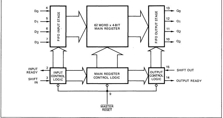
Figure 3. The 3341 Logic Block Diagram
