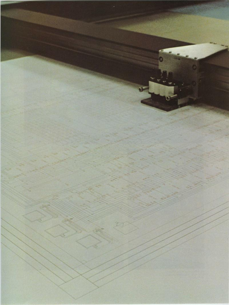
The RETGEN program converts the LAYOUT output to a David Mann Reticle Generator. This system eliminates the rubylith cut and peel step by exposing photographic plates (reticles) with a 10 to 1 image.
