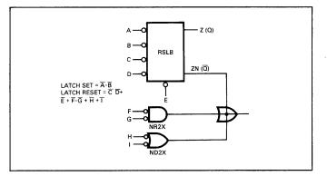
Fig. D-23. Latch Control With Expanders
