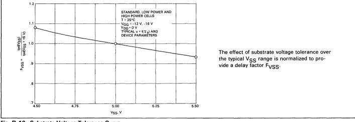
Fig. D-10. Substrate Voltage Tolerance Curve
