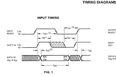
Input data must remain stable during timing window  $t_{DSI}$ . Both SI and IR must be HIGH for  $t_{OV}$ +. Similarly, both SI and IR must be LOW for  $t_{OV}$ -.
