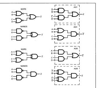
Substituting a complex gate for several simple gates saves chip area. The AO4, for example is five grids long while three NAND gates take nine grids.
