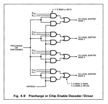
As the memory system size increases, it may also be desirable to generate card select signals from the most significant address bits. This permits all but the selected storage boards to remain in a low power mode. Addresses  $A_0$  through  $A_9$  can then be gated and are active only on the selected storage boards.
