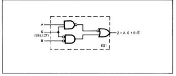
Fig. D-17. EXCLUSIVE-OR Cell Connected as a 2-Input Multiplexer.
