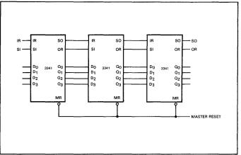
Figure 7. Stacking of the 3341 for Longer Words
