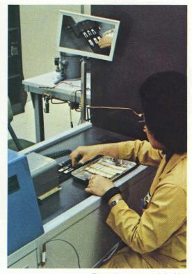
The packages are sealed with a lid to provide environmental and mechanical protection to the die.
