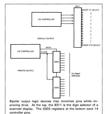
Fig. D-4. MOS with Bipolar Augmentation
