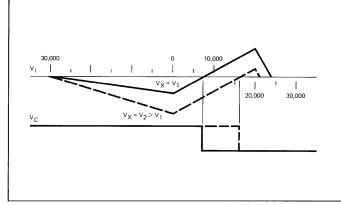
Fig. 4. Integrator and comparator waveforms.
