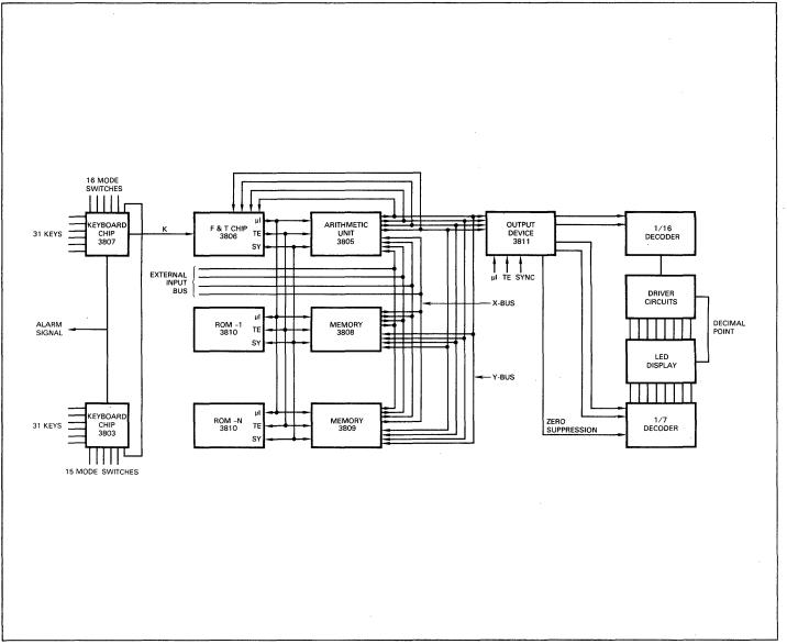
If special interfaces are required, such as printers or mag card readers, custom interfaces can be provided directly from the destination buss or ROMs can be utilized to emulate the desired interface within the structure of the system.
