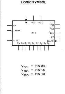
**FUNCTIONAL DESCRIPTION:** The 3814 is intended for use as the digital logic portion of digital voltmeter systems. An input clock (CP) drives 4-1/2 decades of BCD counters, with the counters changing state on the LOW to HIGH clock transition. The output of the second decade is gated with the input clock (CP) and brought off chip (÷100) for use as an additional clock. This clock may be used to drive the multiplexer input (Step).
