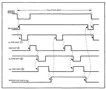
Fig. 6 Memory Internal Timing 256x8
