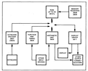
Fig. B-1. PPS-25 Micro-Programmed Processor System
