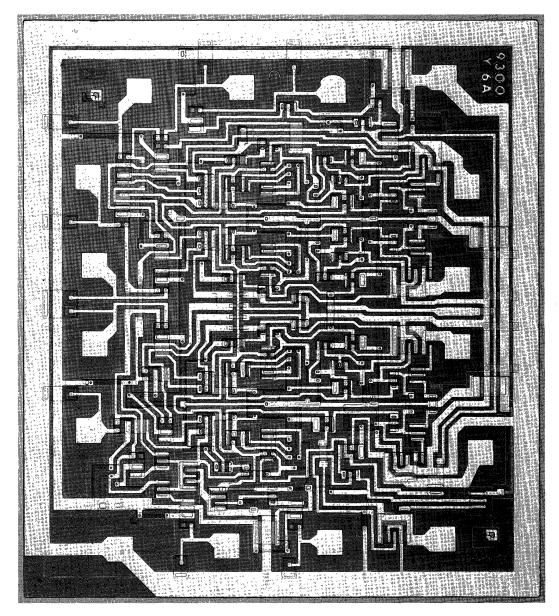
Photomicrograph of the TTL/MSI 9300 4-Bit Shift Register
