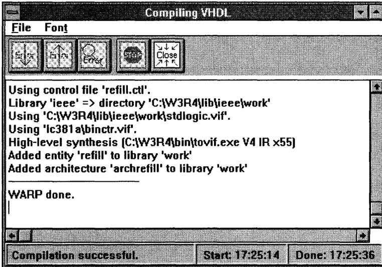
Figure 4-8 A *Compile* window showing a successful compilation
