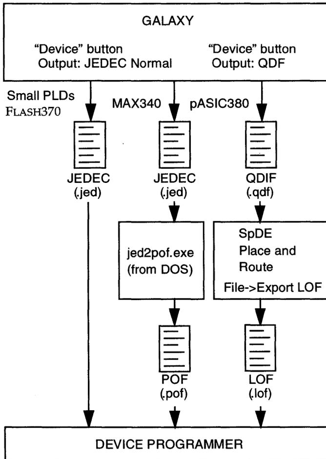
Figure 10-1 Design flow for device programming
