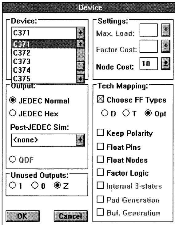
Figure 3-30 The Device window with a C371 selected
