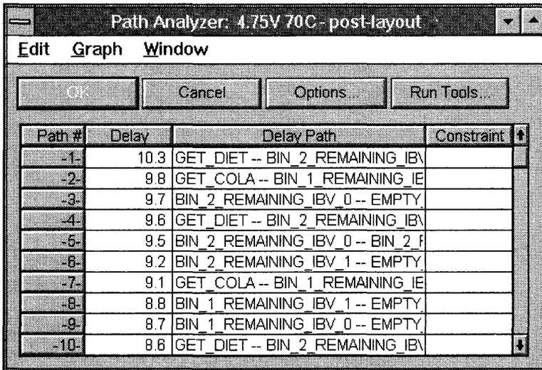
The screenshot shows a window titled "Path Analyzer: 4.75V 70C - post-layout". It has a menu bar with "Edit", "Graph", and "Window". Below the menu bar are four buttons: "OK", "Cancel", "Options", and "Run Tools...". The main area contains a table with the following data:
