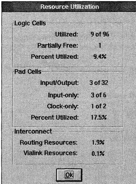
Figure 5-9 Typical Cell Utilization dialog box
