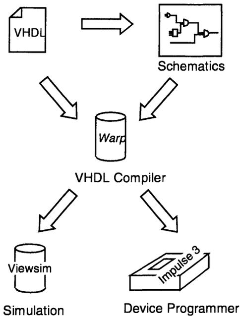
Figure 7-1 *Warp3* design flow
