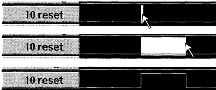
Figure 6-9 Setting a Portion of a Signal High or Low
