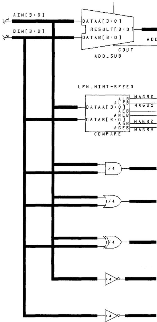
Figure 3-55 Connecting the A and B input buses
