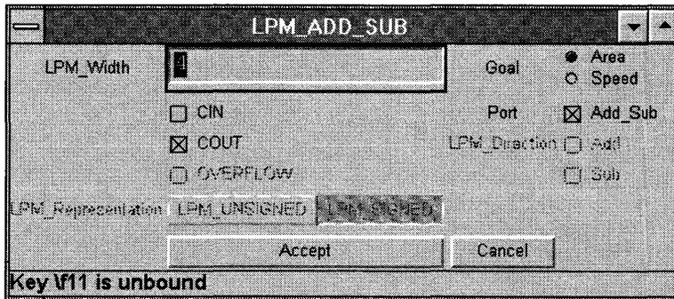
Figure 3-39 Dialog box for the adder/subtractor component
