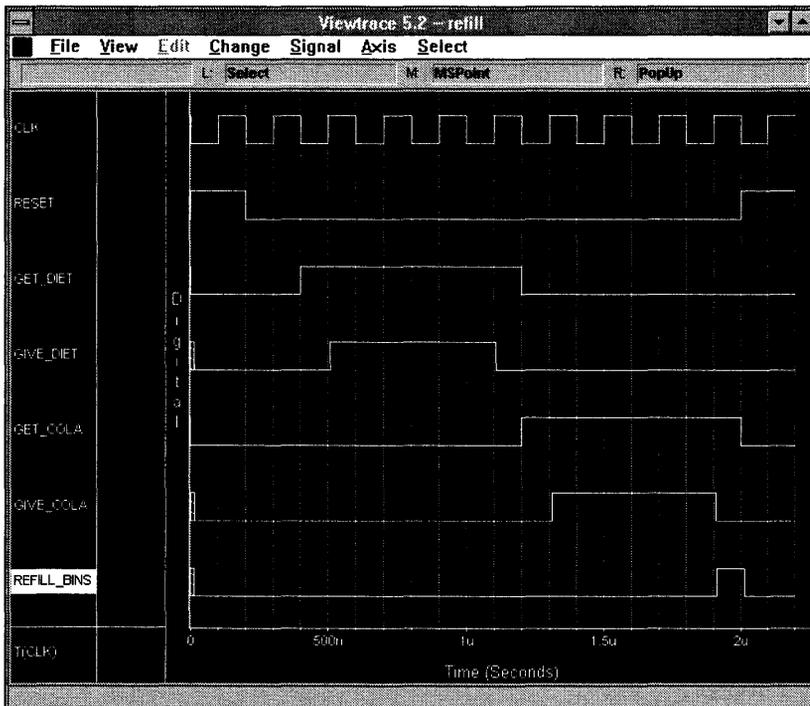
Figure 3-24 ViewTrace output window for refill.vhd
