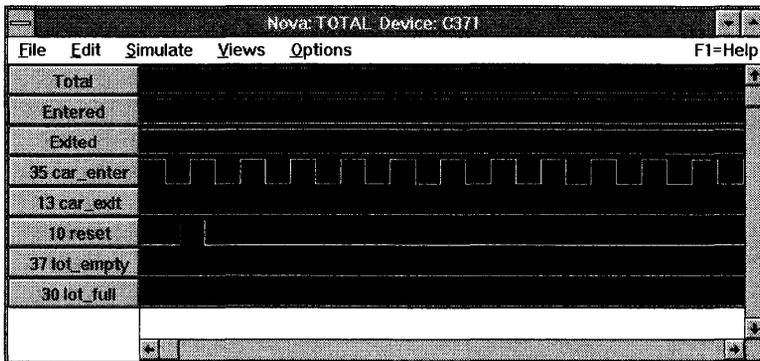
Figure 3-32 Nova screen with car enter signal set
