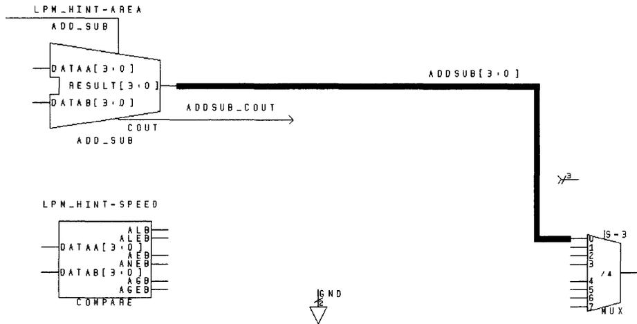
Figure 3-52 Connecting the mux to the comparator
