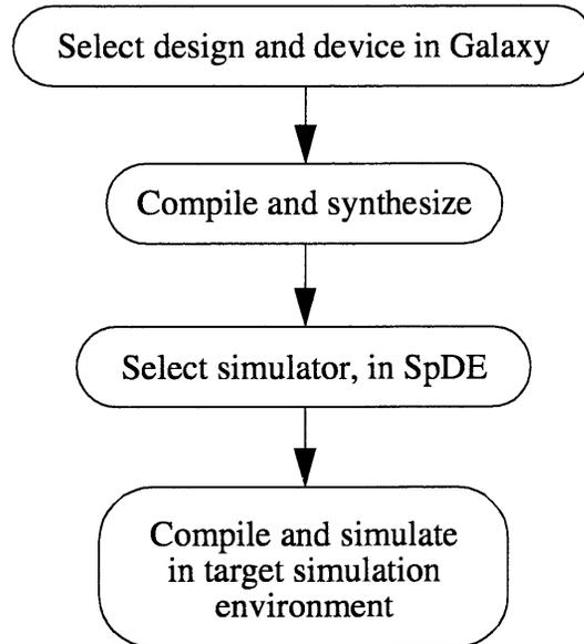
Figure 8-2 Simulation design flow for FPGAs
