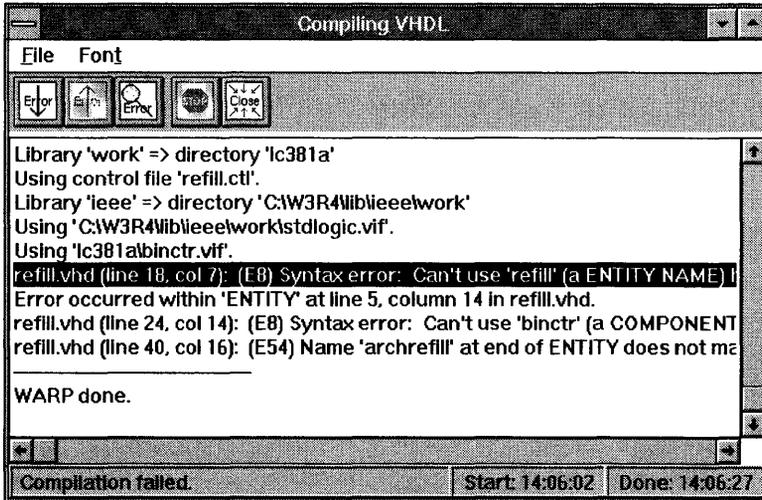
Figure 3-31 Compile window with an error message
