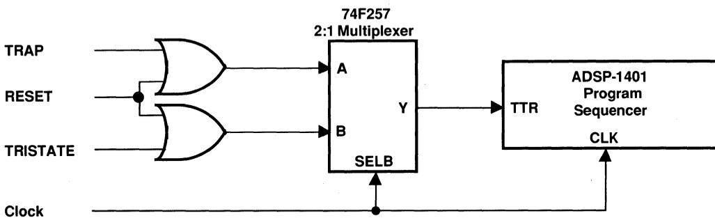
Figure 2.9 TTR Multiplexing Circuit
