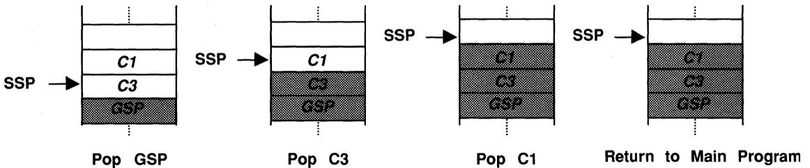
Figure 3.9 Restoring Registers and Counters
