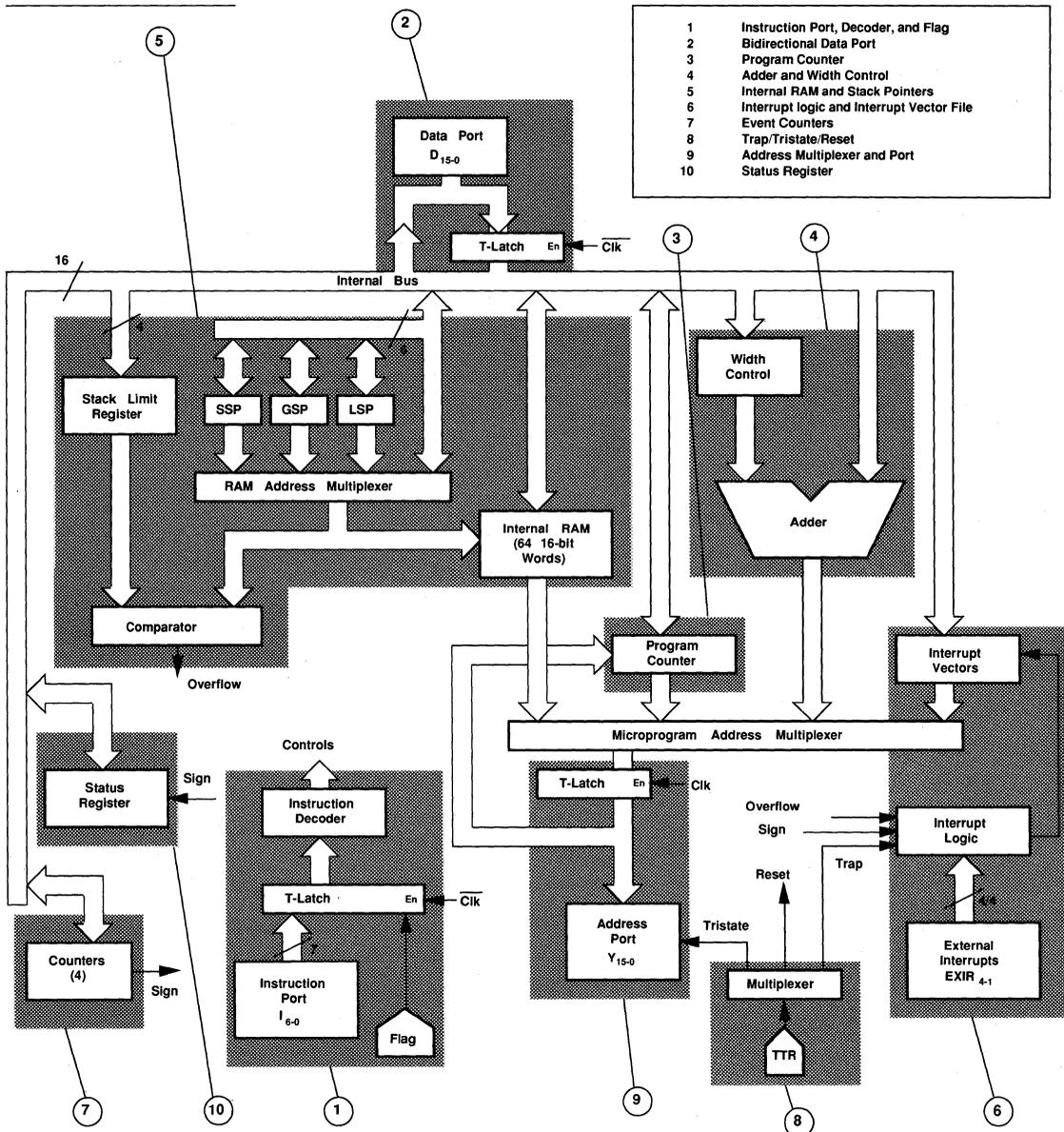
Figure 2.1 ADSP-1401 Block Diagram
