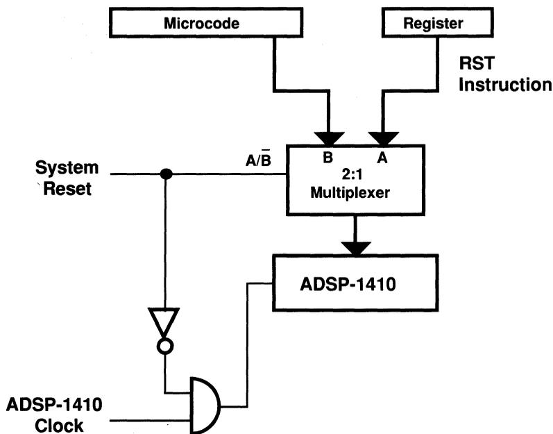
Figure 10.7 System Reset Initializes ADSP-1410
