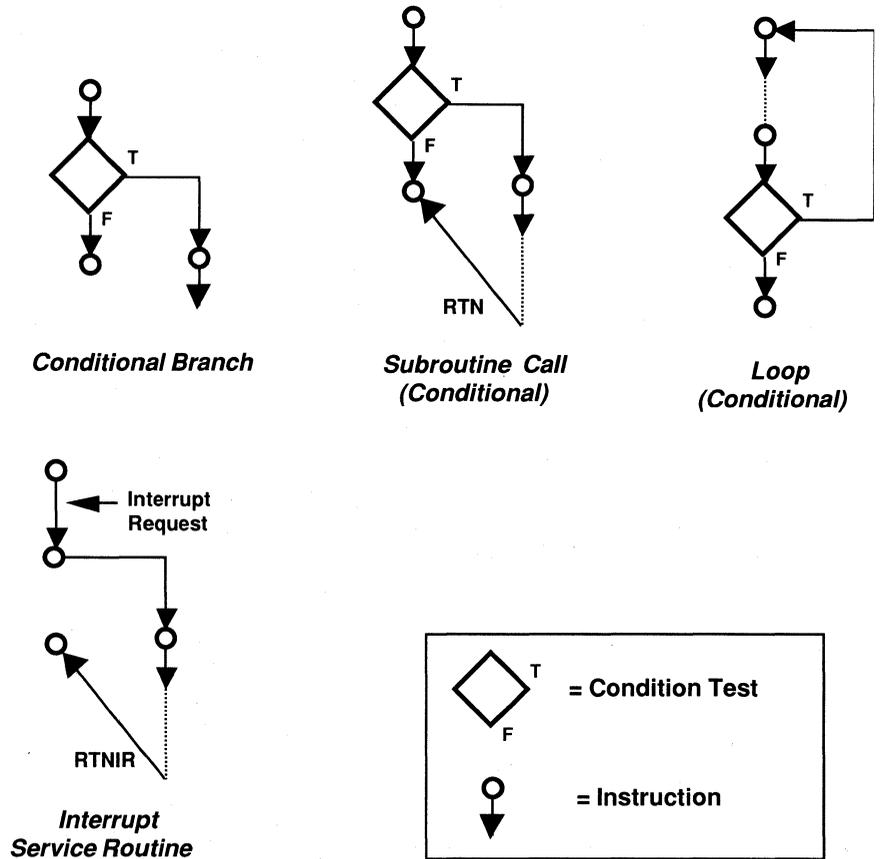
Figure 3.1 Branches, Subroutines, Loops, and Service Routines
