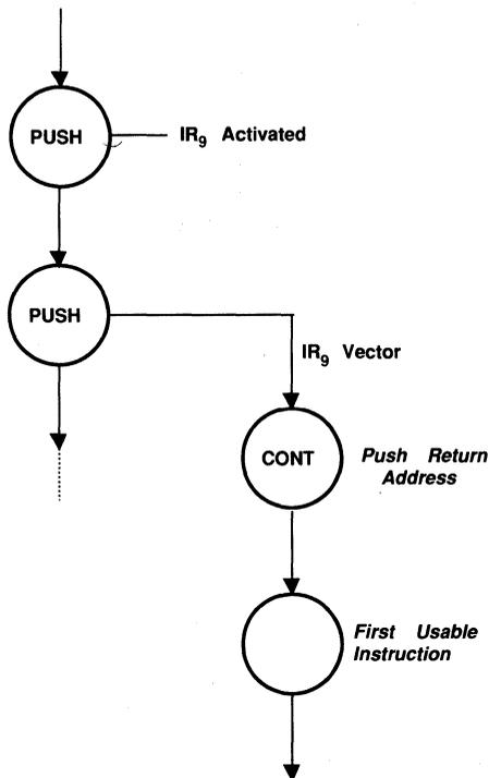
Figure 4.7 Three Pushes On Stack Overflow
