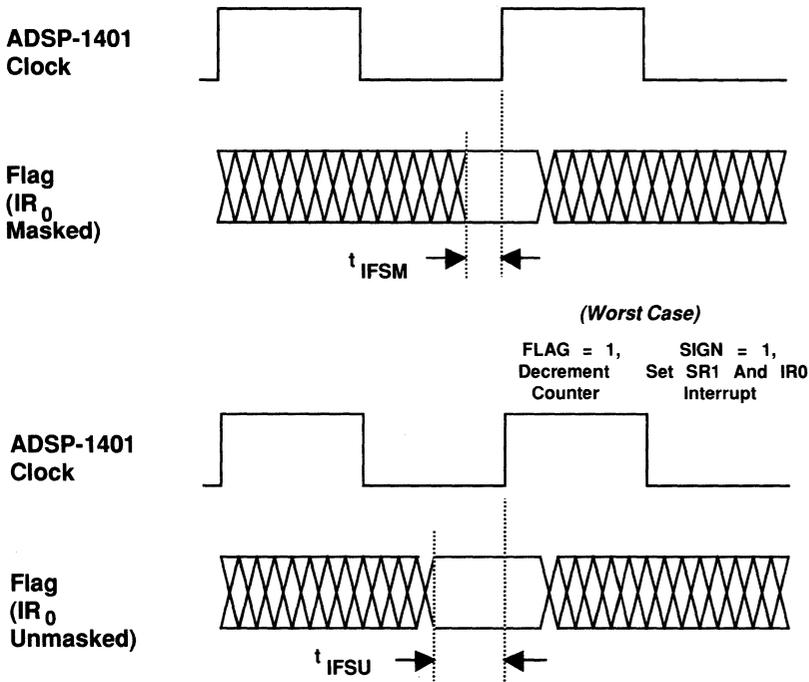
**Figure 3.3 Flag Setup Time With and Without IR<sub>0</sub> Masked**
