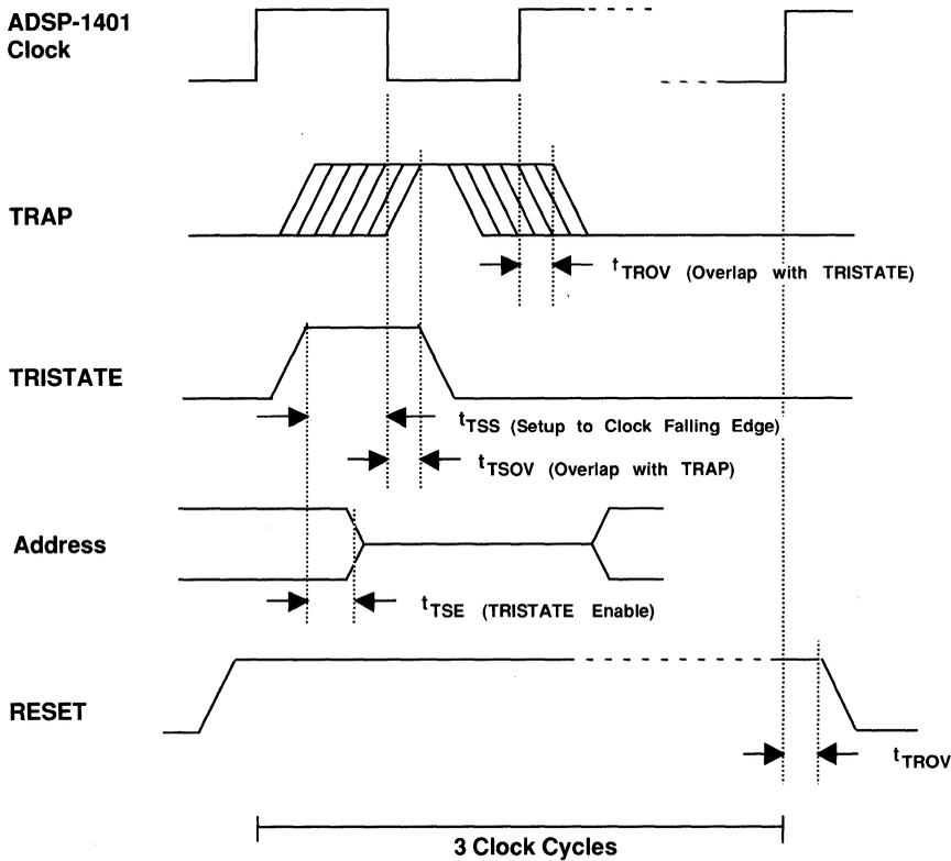
Figure 2.8 Timing for Trap, Tristate, and Reset
