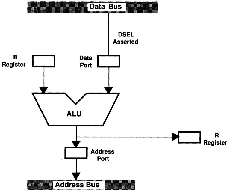
Figure 8.5 DSEL for Single-Cycle Input, Update, and Output
