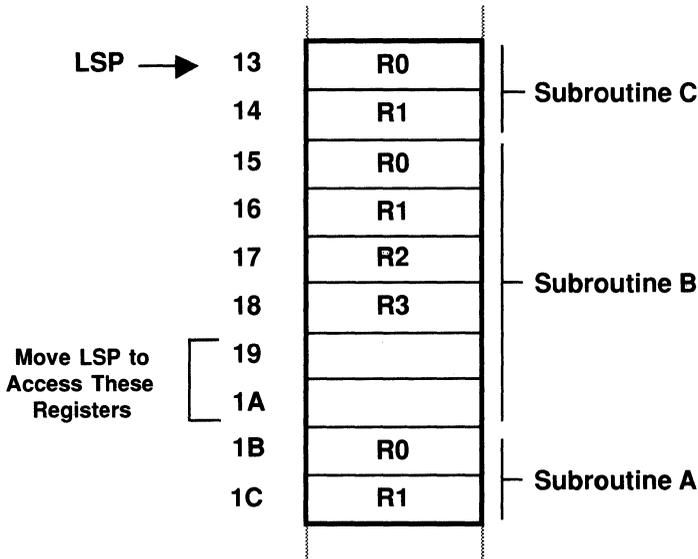
Figure 3.7 Local Stack After Three Subroutine Calls
