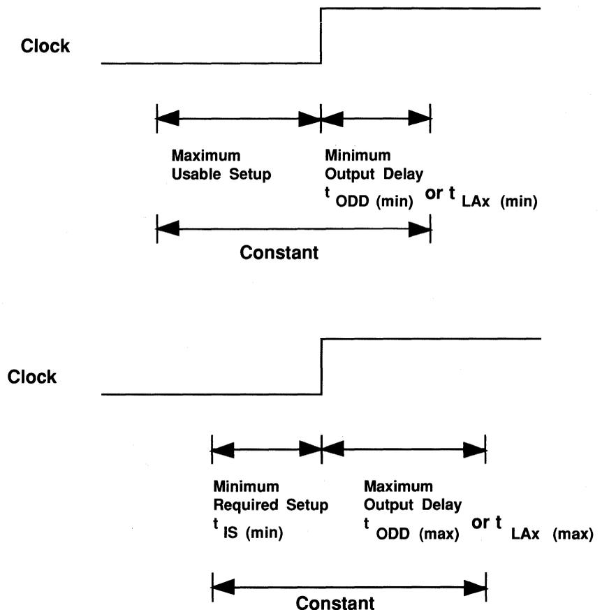
Figure 10.2 Sliding Window Timing
