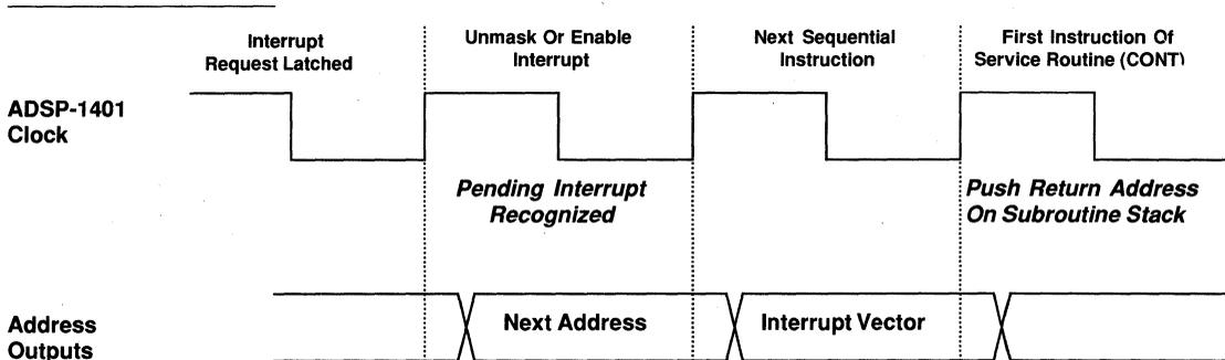
Figure 4.1 One-Cycle Latency After Enabling Interrupts
