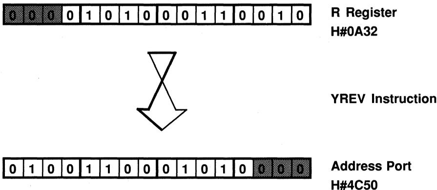
**Figure 10.5 First Bit-Reversed Address**
