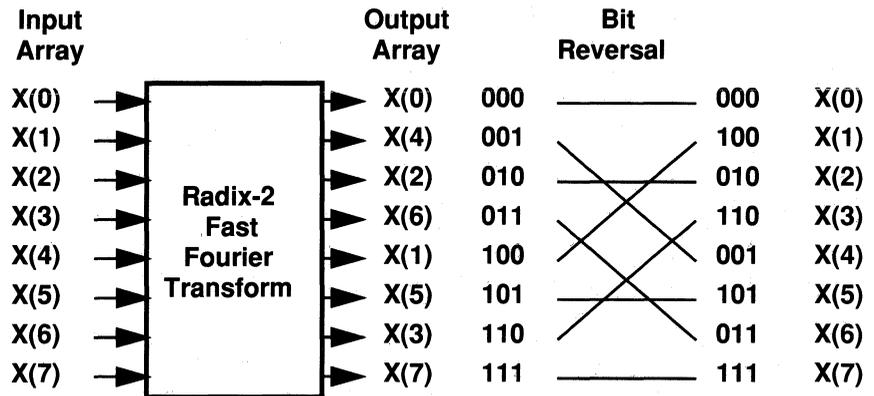
Figure 10.3 Output Addresses From FFT
