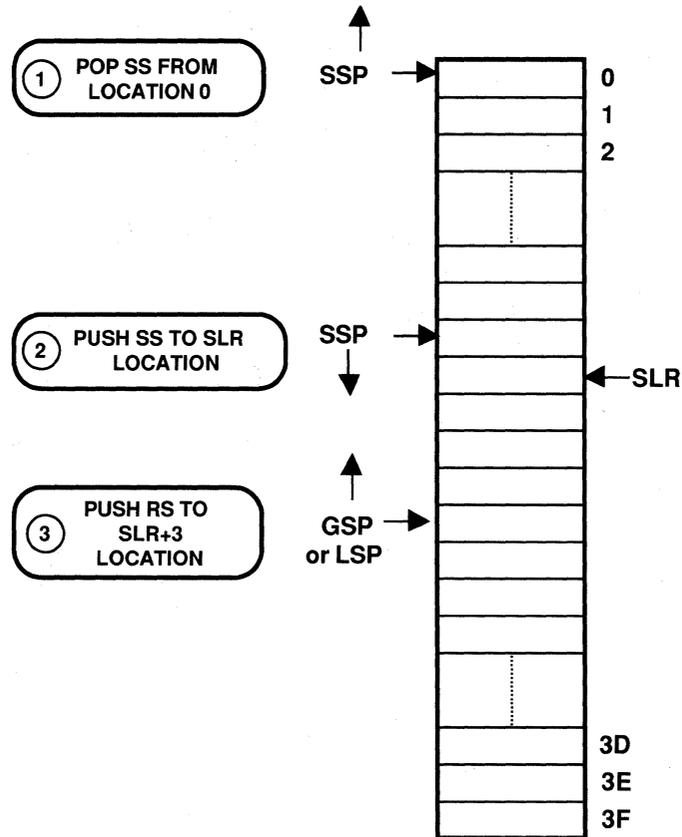
Figure 4.6 Stack Underflow and Overflow
