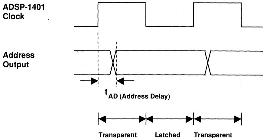
Figure 2.10 Address Output
