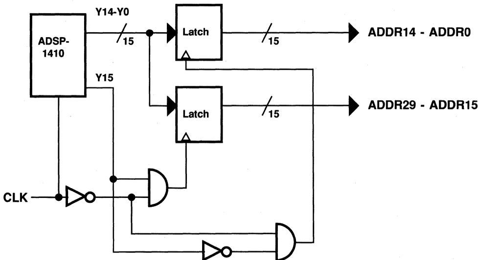
Figure 9.1 Single-Chip Connections to 30-Bit Address Bus
