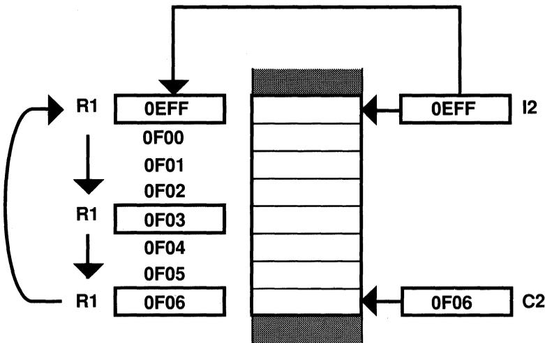
Figure 8.2 Reinitialization to Form Circular Buffer
