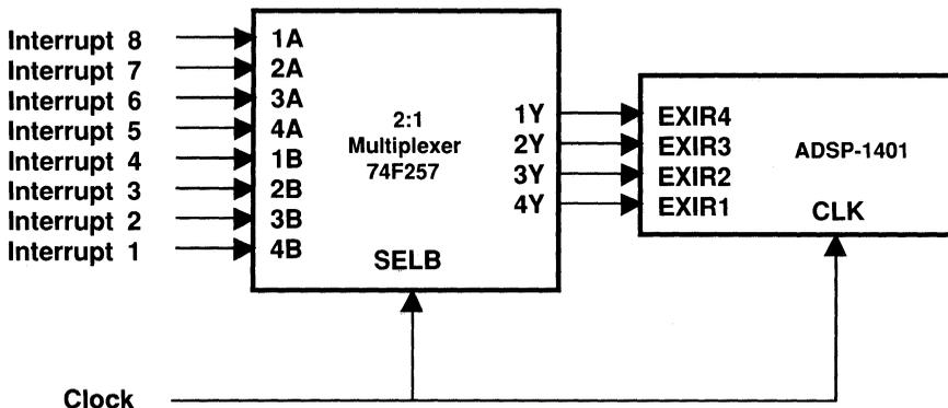
Figure 2.7 Supporting Five to Eight External Interrupts
