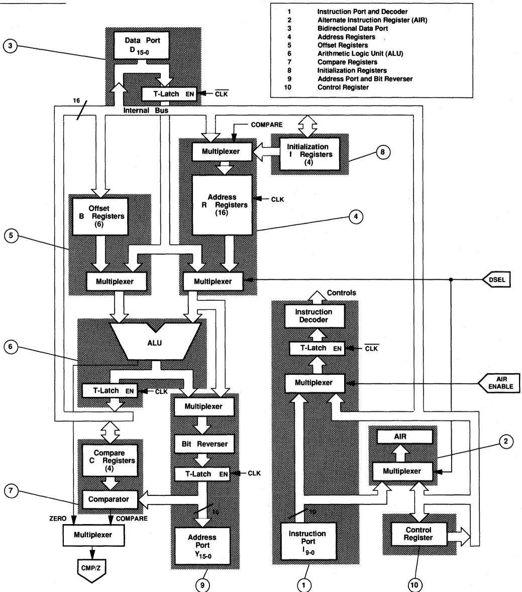
Figure 7.1 ADSP-1410 Block Diagram
