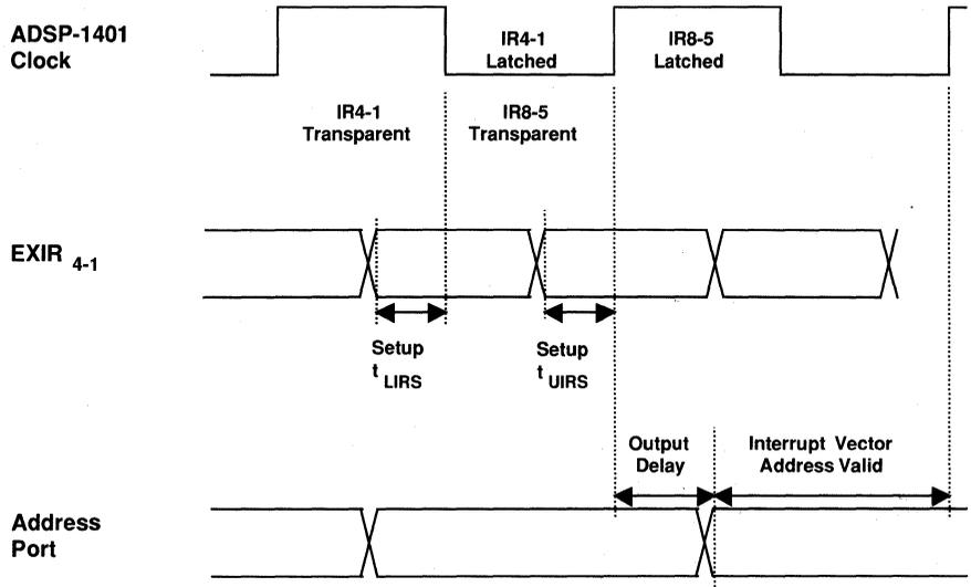
**Figure 2.6 External Interrupt Latching**
