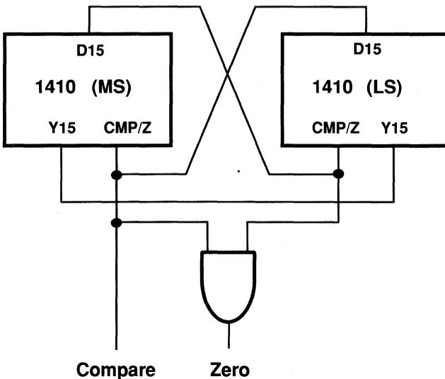
Figure 9.2 Two-Chip Cascade Connections
