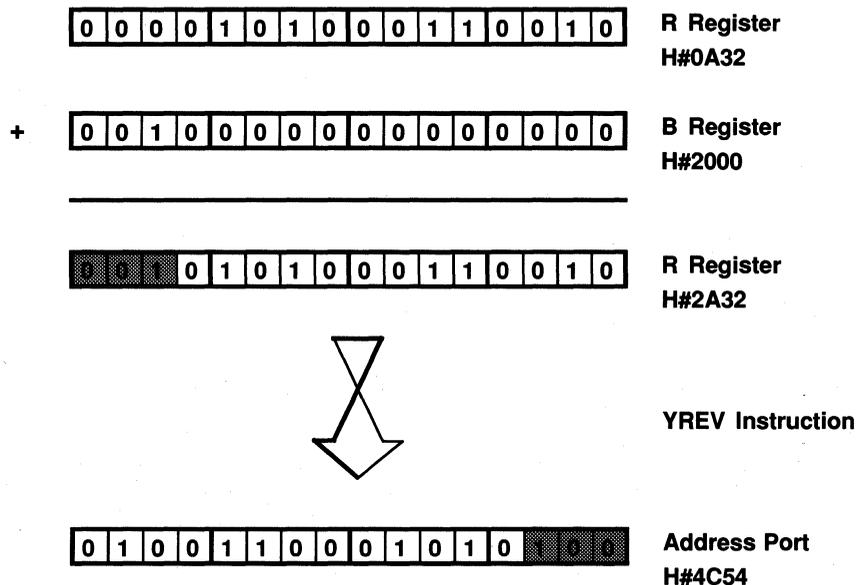
Figure 10.6 Second Bit-Reversed Address
