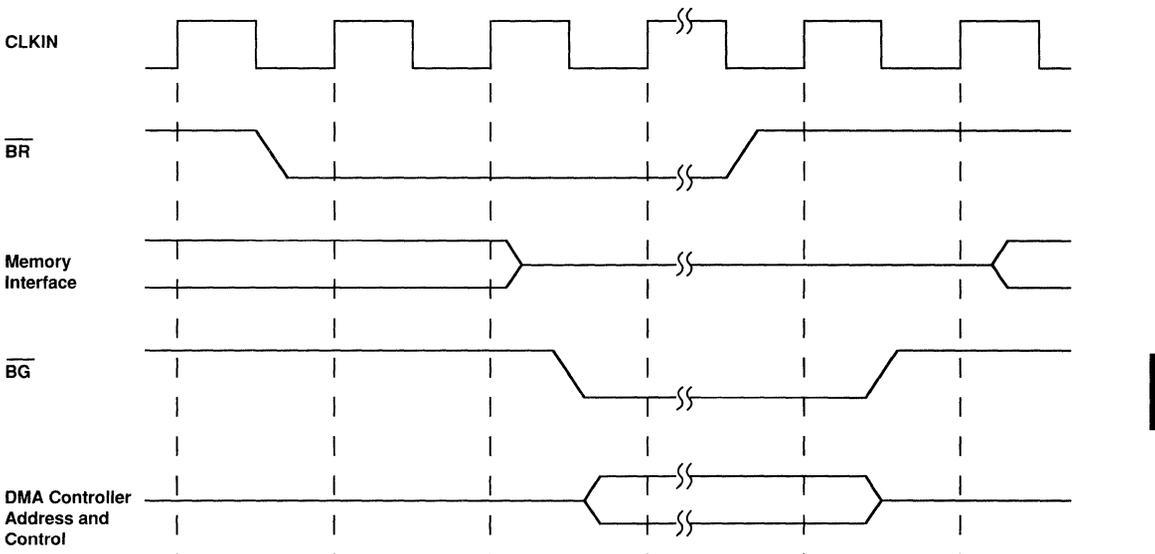
Figure 9.12 Bus Request Timing for DMA
