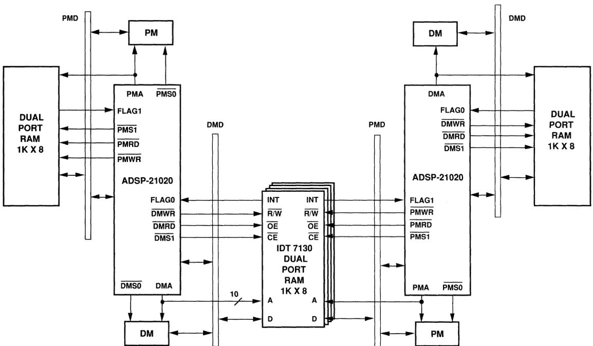
Figure 9.16 Serial Data Flow Using Dual-Port RAM
