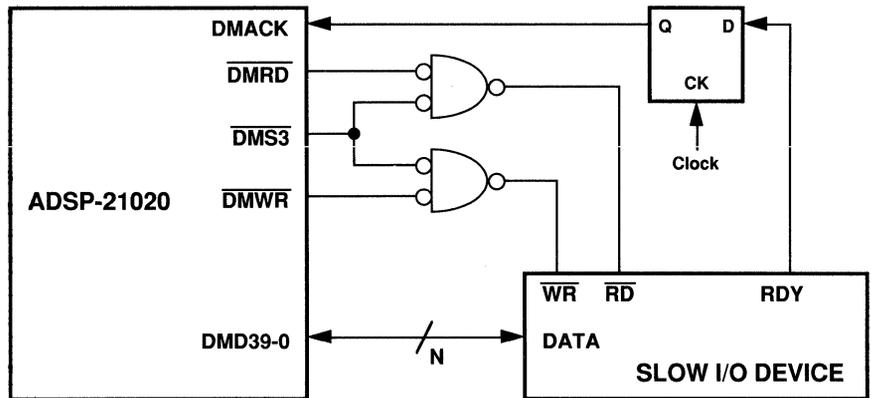
Figure 9.7 I/O Device Interface with Hardware Acknowledge
