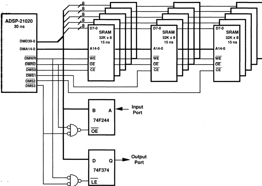
Figure 9.6 Interface to Three Data Memory Banks and Two I/O Devices
