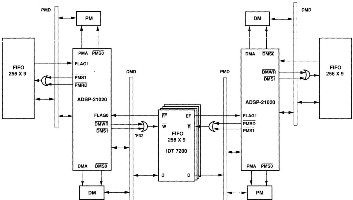
Figure 9.15 Serial Data Flow Using FIFOs
