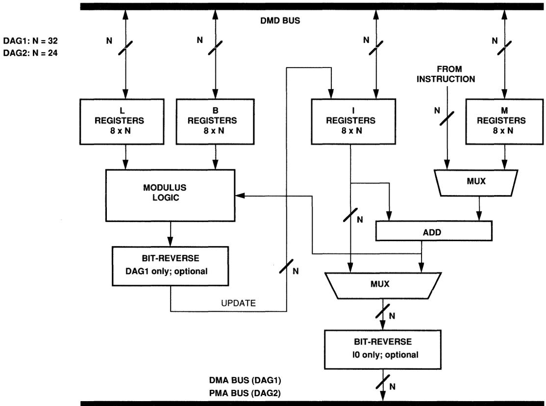
Figure 4.1 Data Address Generator Block Diagram
