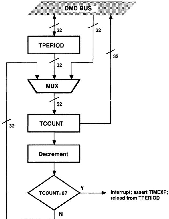
Figure 5.1 Timer Block Diagram
