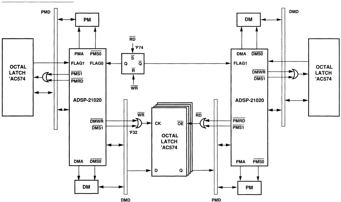
Figure 9.14 Serial Data Flow Using Buffers
