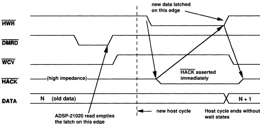
Figure 9.23 Host Write Timing
