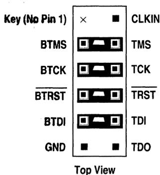
Figure 9.20 Target Board Connector For EZ-ICE Probe (jumpers in place)
