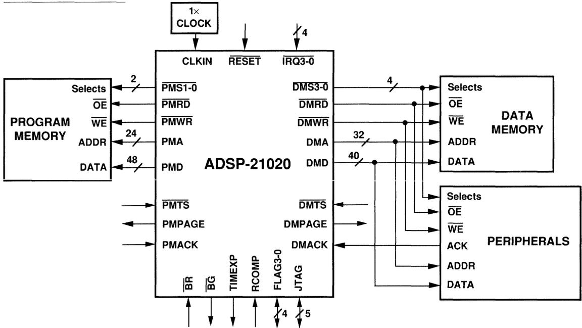
Figure 9.1 Basic ADSP-21020 System Configuration
