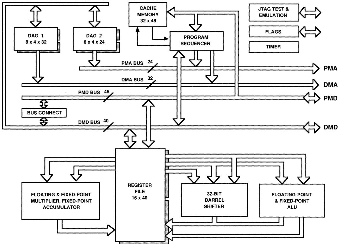
Figure 1.1 ADSP-21020 Block Diagram
