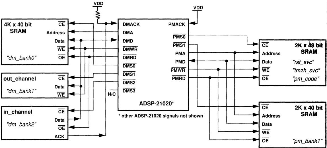
Figure 8.5 Physical Memory Architecture Described in "iirq.ach"
