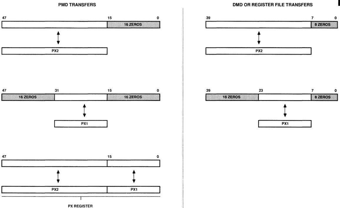
Figure 6.5 PX Register Transfers
