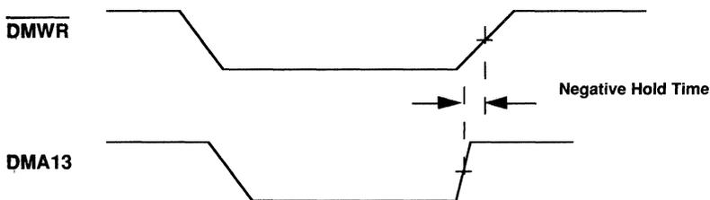
Figure 9.19 Effect of Unequal Capacitive Loads
