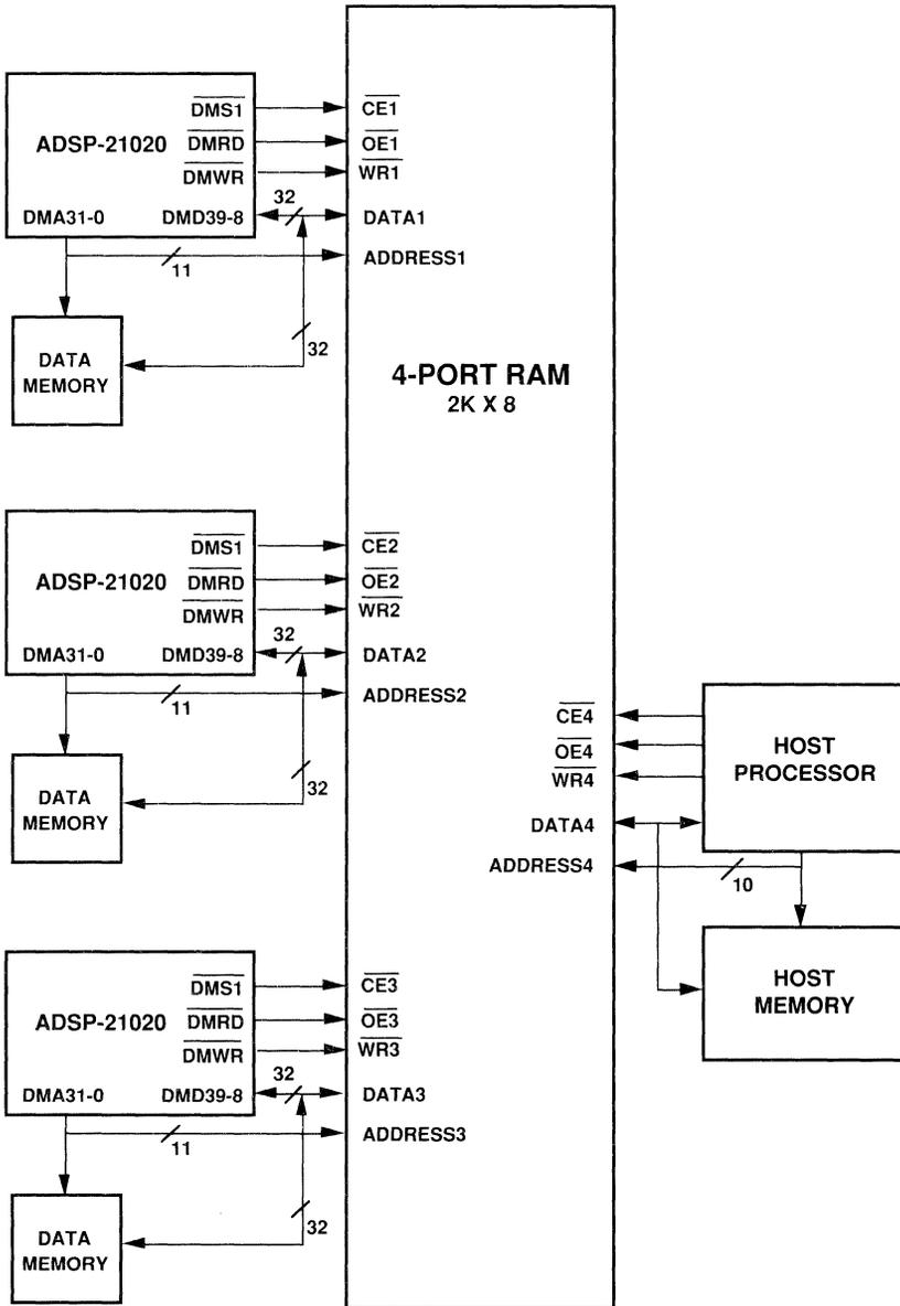
Figure 9.13 Four-Port RAM Configuration
