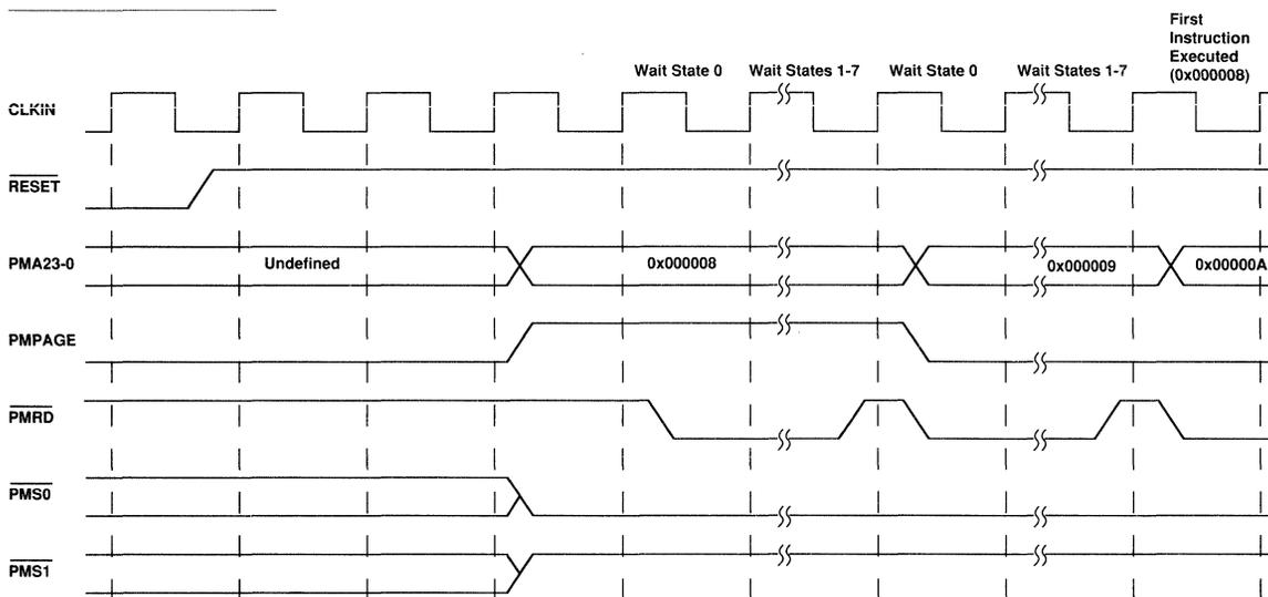
Figure 9.2 Program Memory Interface Timing at Reset
