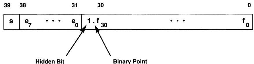
Figure D.2 40-Bit Extended-Precision Floating-Point Format
