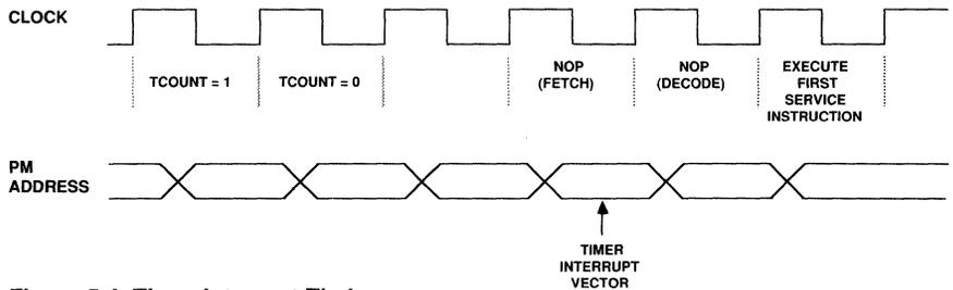
Figure 5.4 Timer Interrupt Timing
