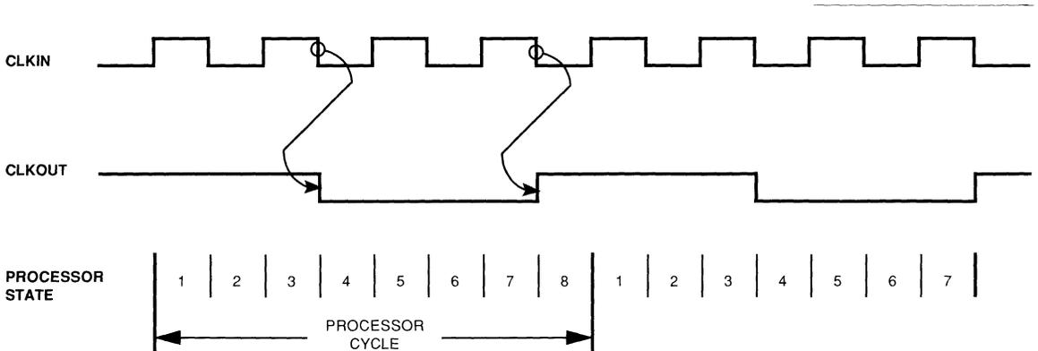
Figure 5.2 Clock Signals & Processor States
