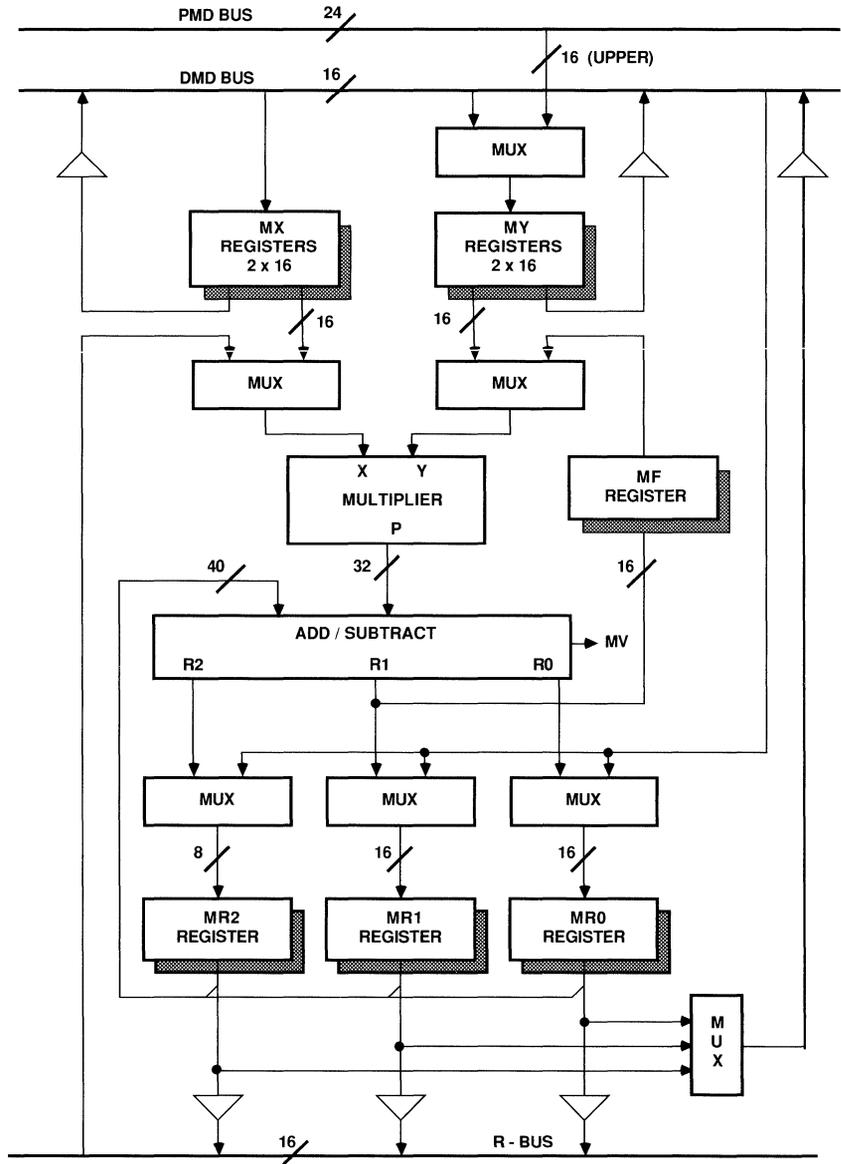
Figure 2.5 Multiplier/Accumulator Block Diagram
