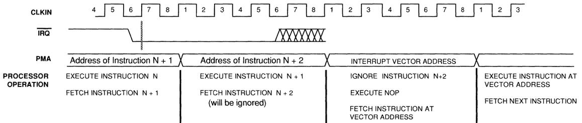
Figure 5.11 Interrupt Service Timing
