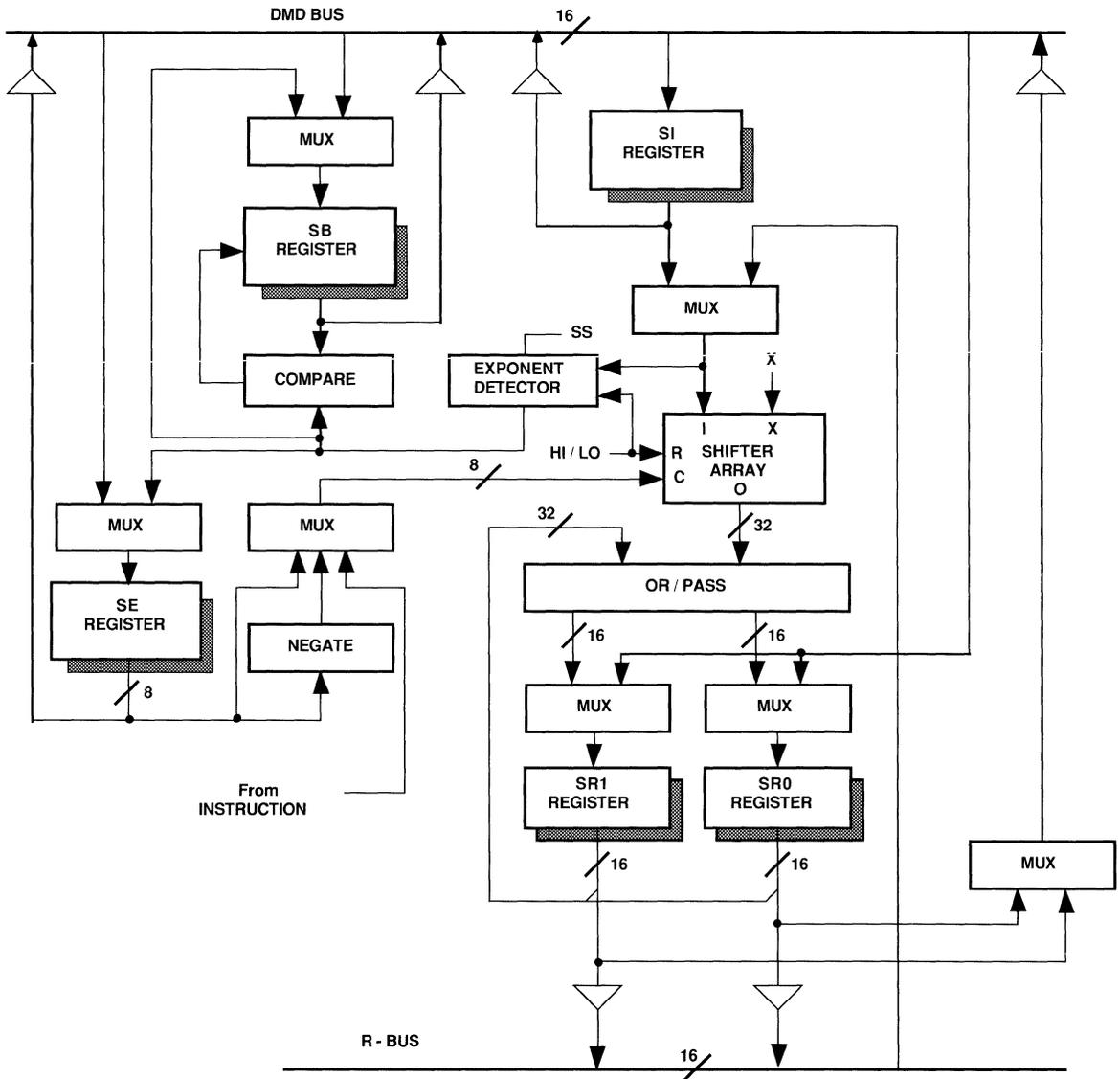
Figure 2.7 Shifter Block Diagram
