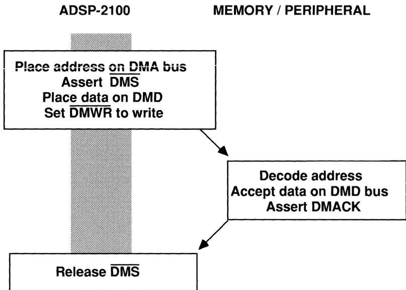
Figure 5.9 Data Memory Write Flowchart
