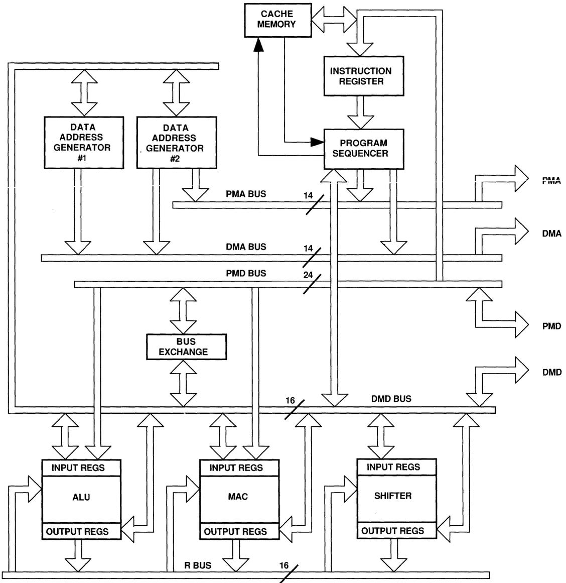
Figure 1.2 ADSP-2100 Internal Architecture
