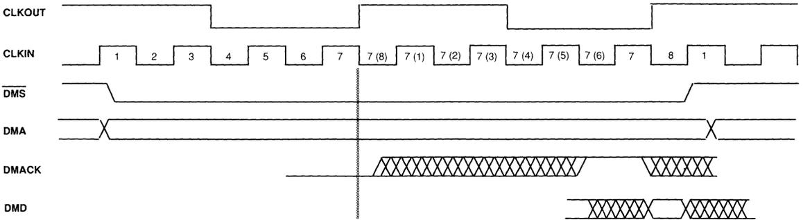
Figure 5.7 Data Memory Read Extended by DMACK
