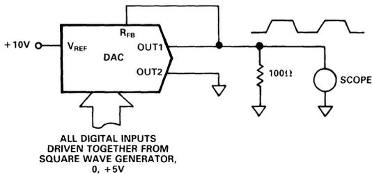
Figure 2.7 Test Circuit for Current Settling Time
