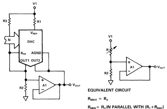
Figure 6.3.3 Potentiometer Circuit with Reduced Range and Improved Resolution
