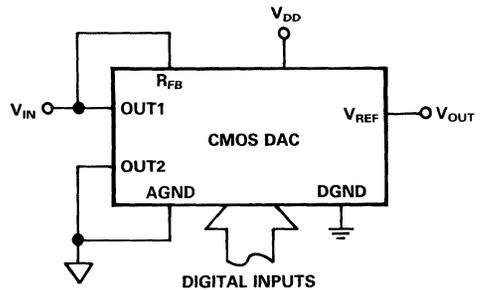
Figure 4.2 Single Supply D/A Converter Using Voltage-Switching Mode
