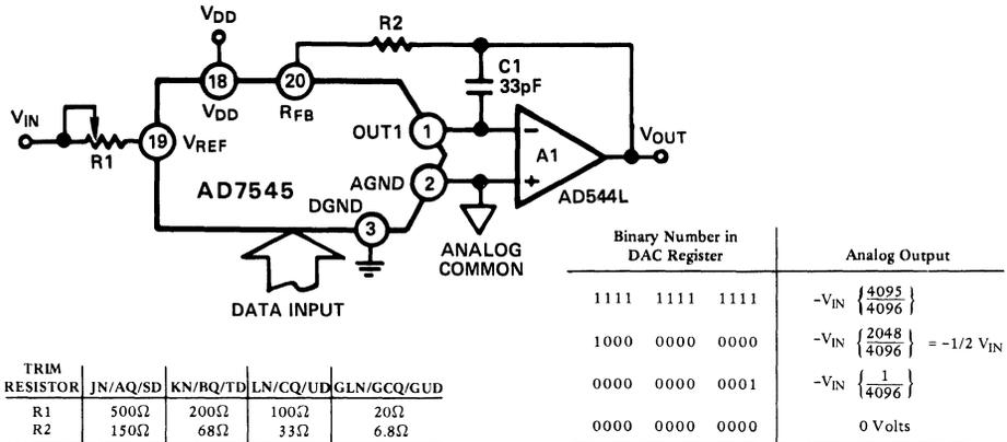
Figure 6.2.1 Low Cost 12-Bit Unipolar D/A Converter
