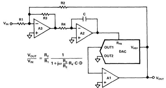
Figure 6.7.3 Low Pass Filter with Digitally Programmable Time Constant
