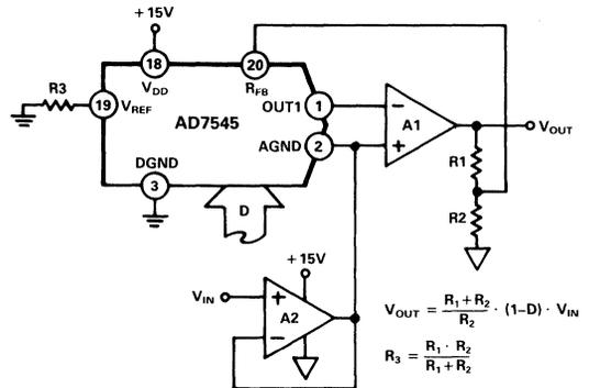
Figure 6.2.4 12-Bit D/A Converter for High Temperature Operation
