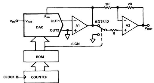
Figure 6.5.1 Basic DAC Based Low Frequency Function Generator
