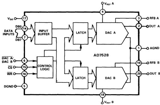
Figure 5.3 AD7528 – Dual 8-Bit DAC – 20-Pin DIP
