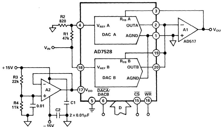
Figure 6.2.6 Low Cost 14-Bit Resolution D/A Converter
