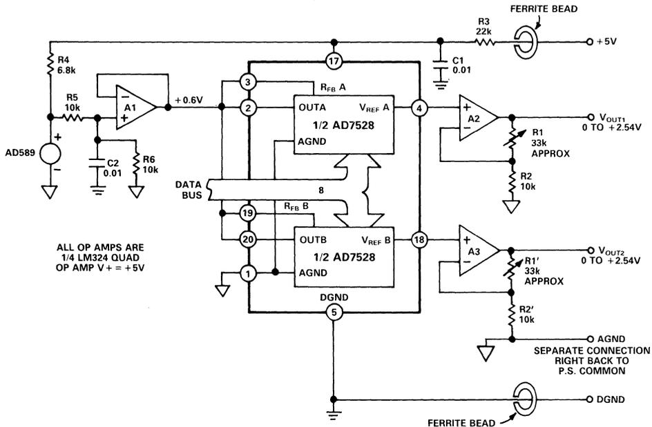
Figure 6.2.5 Dual DAC – Single 5V Supply
