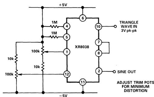
Figure 6.5.6 Monolithic Triangle to Sine Wave Generator
