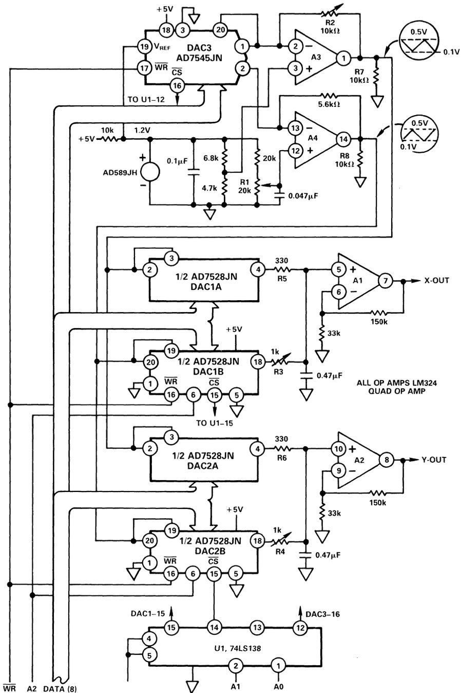
Figure 6.5.9 X-Y Plotter Interface Using +5V Supplies Only
