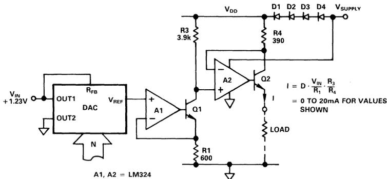
Figure 6.4.5 Single Supply Current Source to AGND
