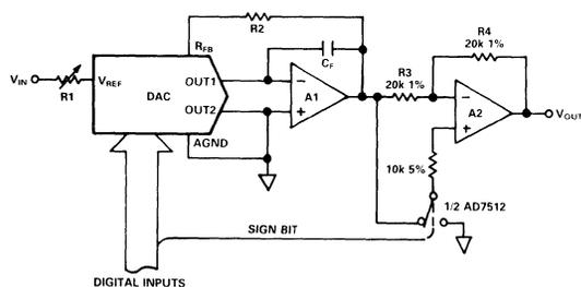
Figure 3.5 Alternative Sign Plus Magnitude D/A Converter
