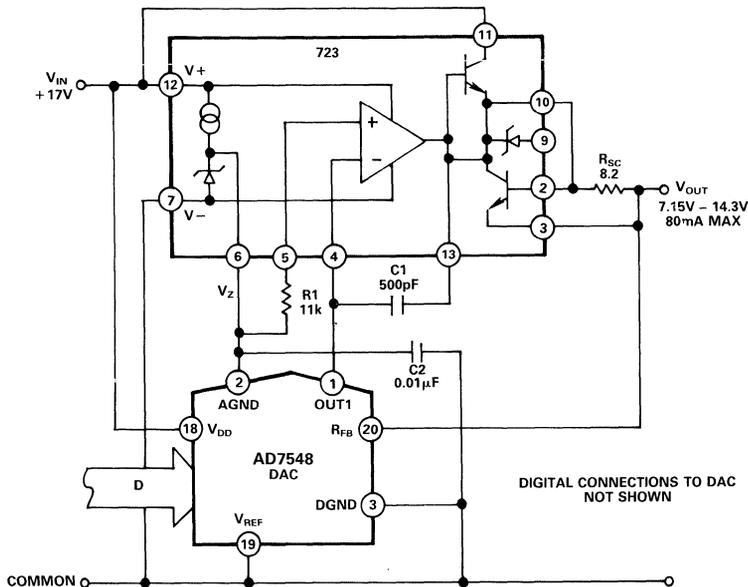
Figure 6.3.7 Simple 2 IC Programmable Power Supply
