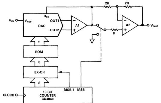
Figure 6.5.2 Block Diagram of Sine Generator
