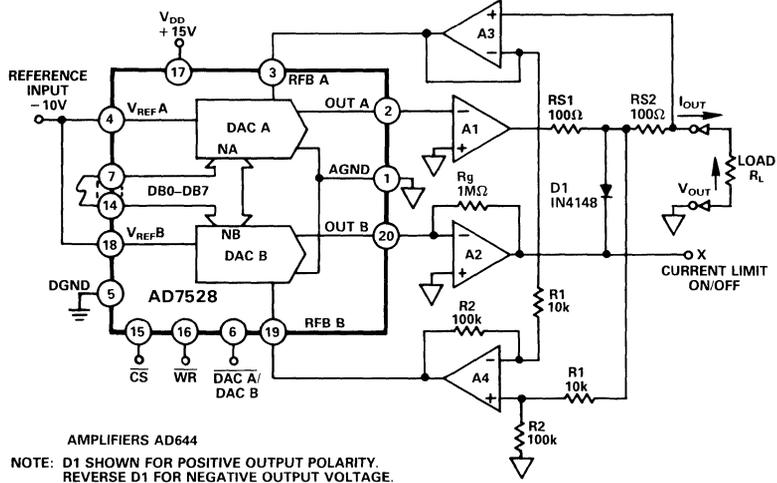
Figure 6.2.8 Programmable Voltage/Current Source  $V_{OUT} = 0$  to  $+10V$ ,  $I_{OUT} = 0$  to  $+10mA$
