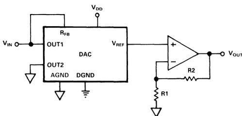
Figure 4.6 Voltage-Switching D/A Converter
