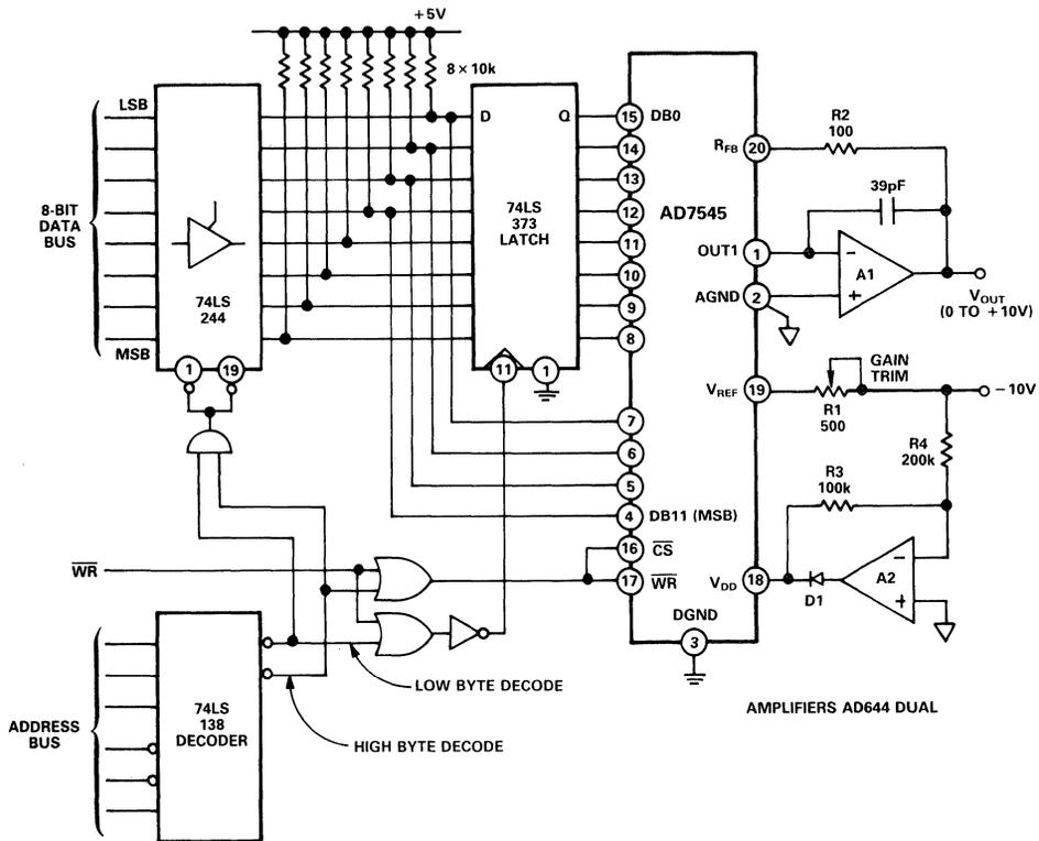
Figure 6.9.1 AD7545 to 8-Bit Data Bus Interface
