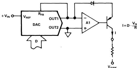
Figure 6.4.1 Simple Programmable Current Source to  $V_{SINK}$
