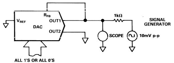
Figure 2.6 Circuit for Measuring Output Capacitance of DAC
