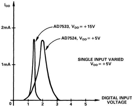
Figure 5.1 Typical  $I_{DD}$  vs. Digital Input Voltage
