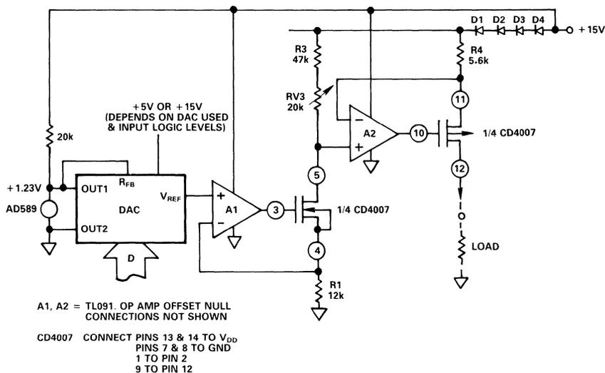
Figure 6.4.6 0 to 1mA Programmable Current Source - Single Supply
