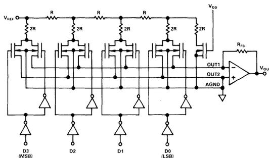
Figure 2.1 Simple CMOS D/A Converter
