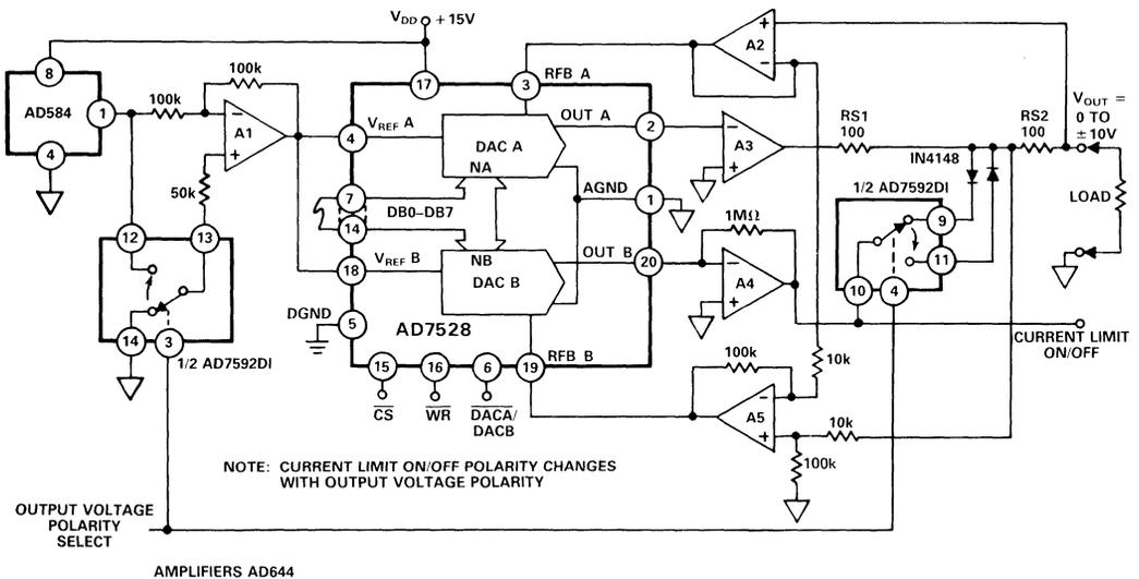
Figure 6.2.9 Programmable Voltage/Current Source with Bipolar Output
