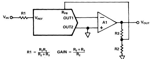
$$R_1 = \frac{R_1 R_3}{R_2 + R_3} \quad \text{GAIN} = \frac{R_2 + R_3}{R_2}$$
