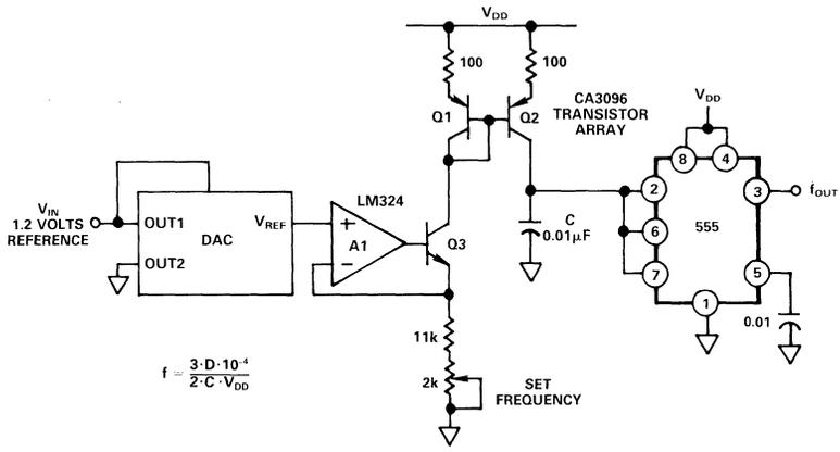
Figure 6.6.6 Single Programmable Oscillator Using 555 Timer
