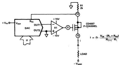
Figure 6.4.3 Programmable Current Source to  $-V_{SINK}$
