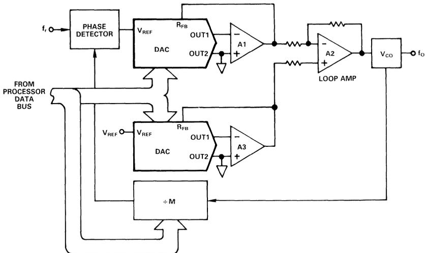
Figure 6.6.10 Phase-Lock Loop Stabilization Using Dual DAC
