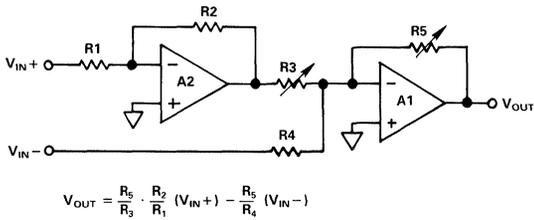
Figure 6.3.1 Instrumentation Amplifier
