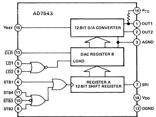
Figure 5.6 AD7543 12-Bit DAC – 16-Pin DIP
