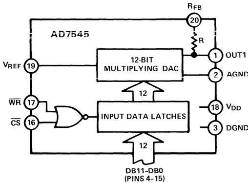
Figure 5.4 AD7545 12-Bit DAC – 20-Pin DIP
