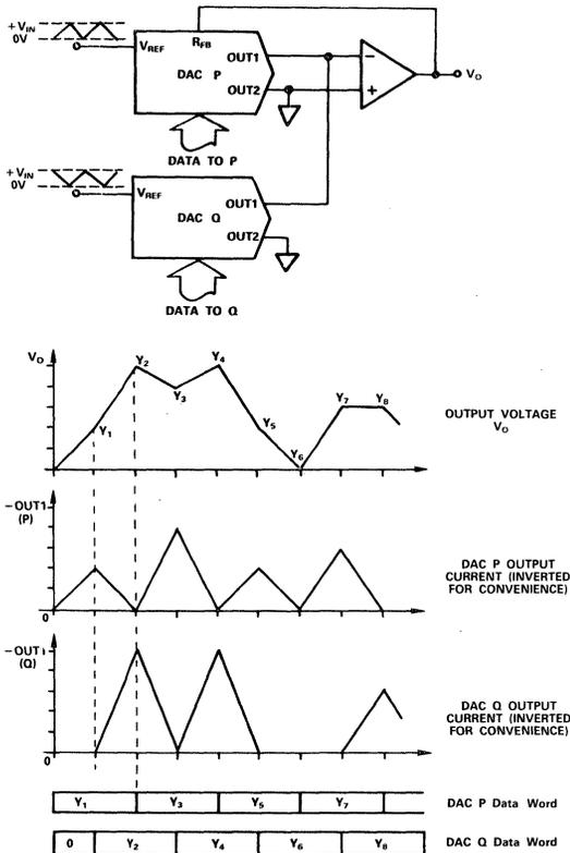
Figure 6.5.8 Simplified Interpolation Scheme for Function Generation
