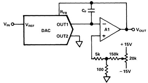
Figure 3.2 Alternative Method of Nulling Op Amp Offset
