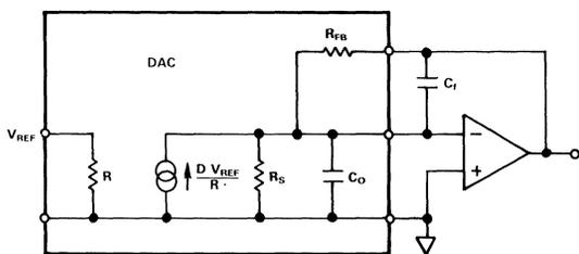
Figure 2.9 Equivalent Circuit of DAC
