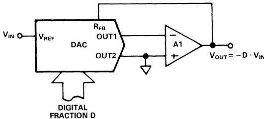
Figure 6.1.1 CMOS DAC as Multiplier or Attenuator
