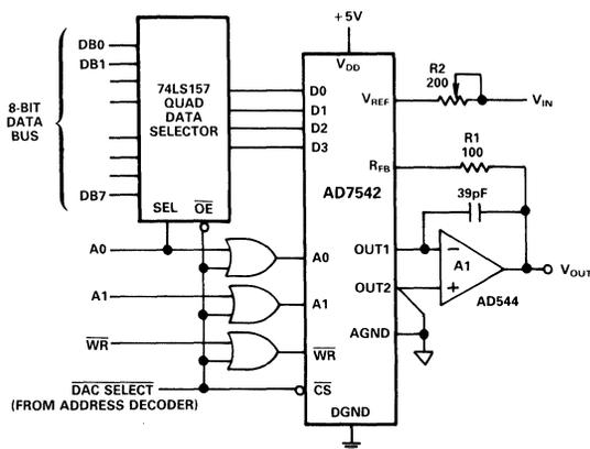
Figure 6.9.3 AD7542 to 8-Bit Data Bus Systems
