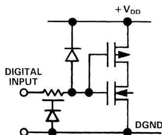
Figure 2.12 Digital Input Circuit Showing Protection Diodes
