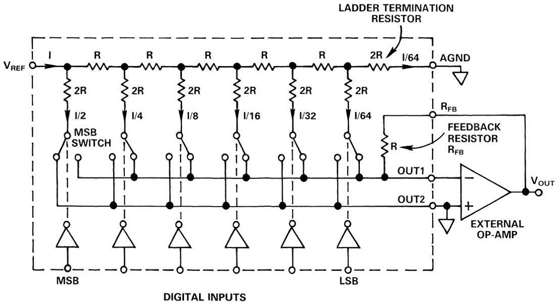
Figure 1.1 Simplified 6-Bit Current-Steering DAC
