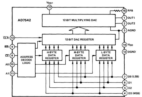
Figure 5.5 AD7542 12-Bit DAC – 16-Pin DIP
