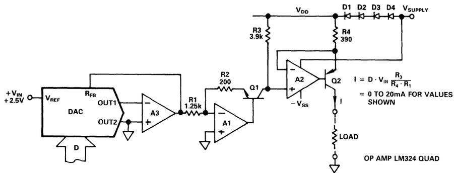
Figure 6.4.4 Programmable Current Source to AGND or  $-V_{SINK}$
