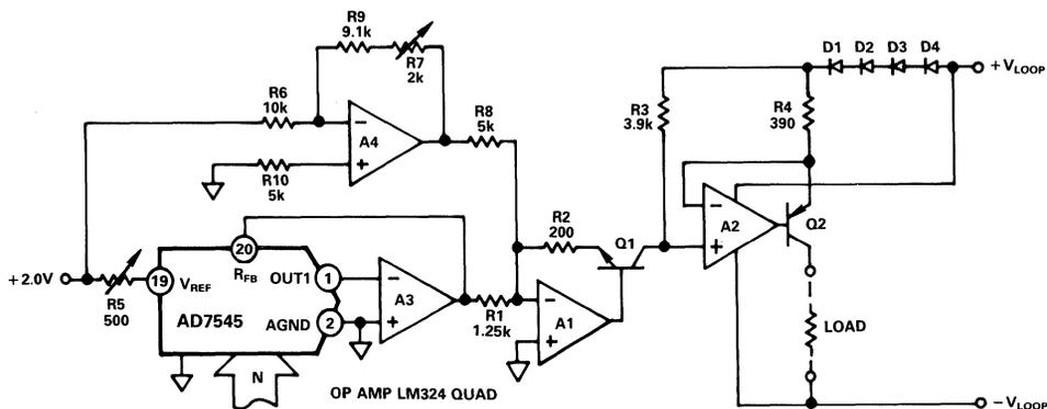
Figure 6.4.7 4-20mA Loop Circuit, Current-Steering Mode
