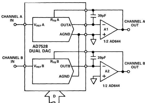
Figure 6.8.3 Dual 8-Bit DAC as Stereo Balance Control
