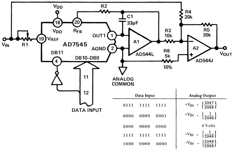
Figure 6.2.2 12-Bit Bipolar D/A Converter (2's Complement)
