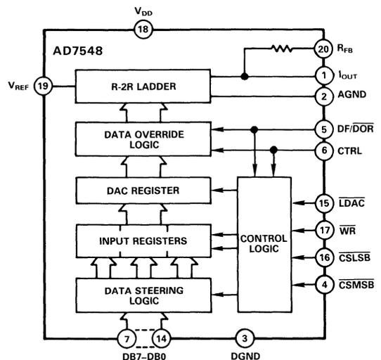
Figure 5.7 AD7548 12-Bit DAC – 20-Pin DIP
