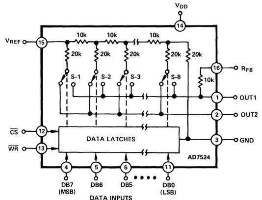
Figure 5.2 AD7524 8-Bit DAC - 16-Pin DIP
