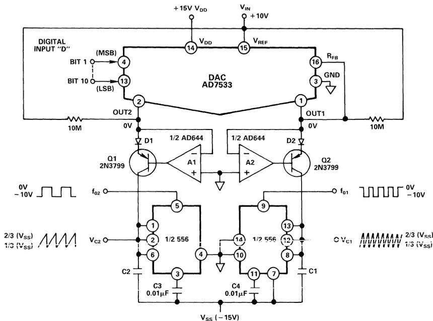
Figure 6.6.8 Programmable Oscillator with Complementary Output Frequencies
