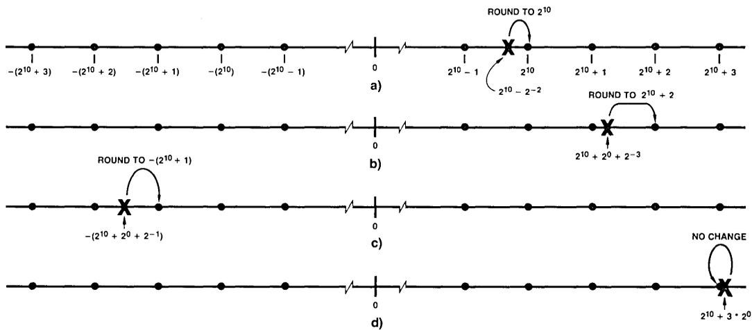
Figure 16 illustrates four examples of the round toward 0 process for operations having an integer destination format. The infinitely precise result of an operation is represented by an X on the number line; the black dots on the number line indicate those values that can be exactly represented in the integer format.
