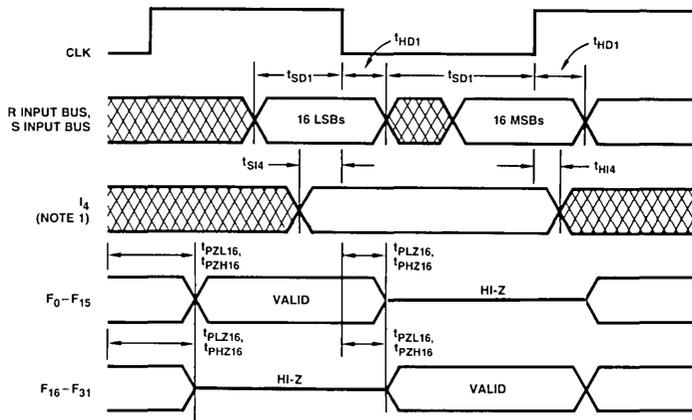
Note 1.  $I_4$  has special setup and hold time requirements in this mode. All other control signals have timing requirements as shown in the diagram
