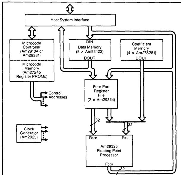
Figure 3: Am29300-based array processor.
