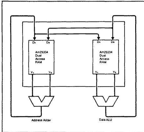
Figure 1: RAM with 4 read and 2 write ports.
