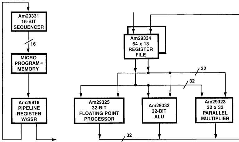
Figure 1. Am29300 Family High Performance System Block Diagram
