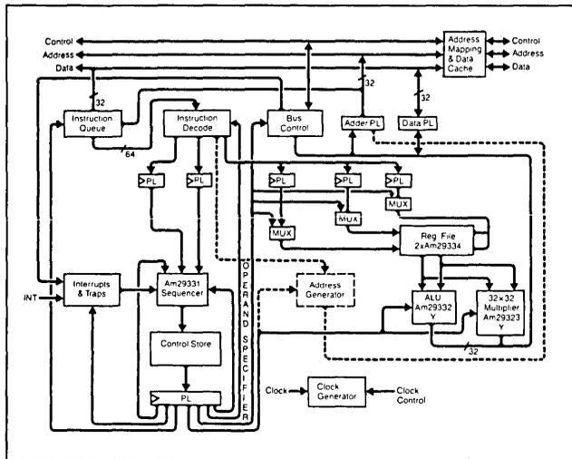
Figure 2: Am29300-based supermini emulation.
