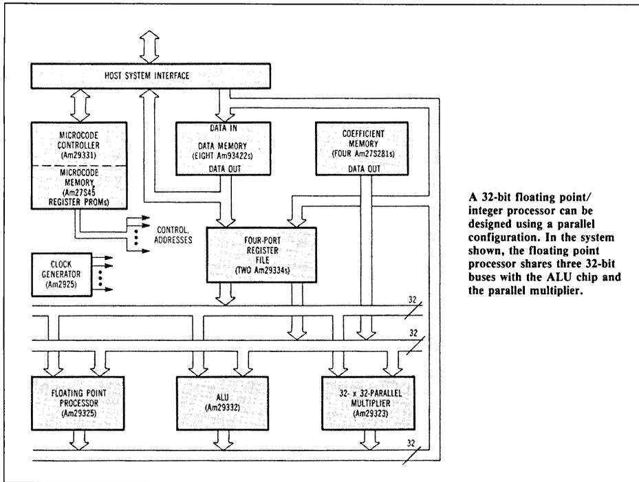
A 32-bit floating point/integer processor can be designed using a parallel configuration. In the system shown, the floating point processor shares three 32-bit buses with the ALU chip and the parallel multiplier.
