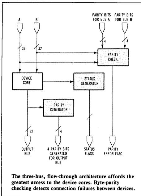
Both error checking schemes operate on a cycle-by-cycle basis so any detected fault triggers an interrupt at the microinstruction level. Unlike other redundant schemes, specialized software is not required, and system performance is not affected by the communication between redundant functional units.
