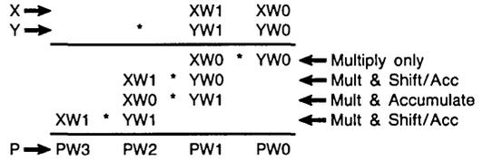
Table 4 details the movement of the input operands through the Am29323. Table 5 defines the microcode required to perform a signed 64 x 64-bit multiplication. For an unsigned multiplication, TCX and TCY are LOW for all cycles. The operations and data movement are scheduled to produce a single product in seven clock cycles or a new pipelined product every four clock cycles.
