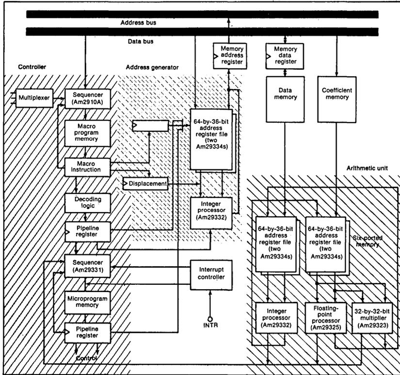
6. A versatile, yet high-performance microprogrammable system can be built by including both the floating-point processor and the 32-bit multiplier into a system that uses the other Am29300 building blocks to form the control and address generation sections.
