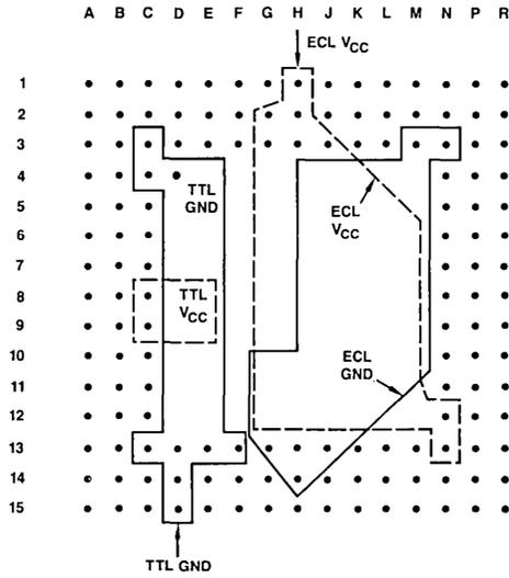
Note: 1. D4 (alignment pin) is not connected internally—may be wired to TTL ground or left unconnected.
