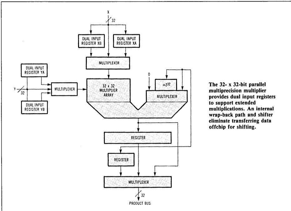
The 32- x 32-bit parallel multiprecision multiplier provides dual input registers to support extended multiplications. An internal wrap-back path and shifter eliminate transferring data offchip for shifting.
