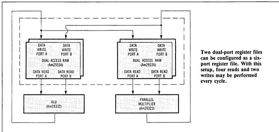
Two dual-port register files can be configured as a six-port register file. With this setup, four reads and two writes may be performed every cycle.
