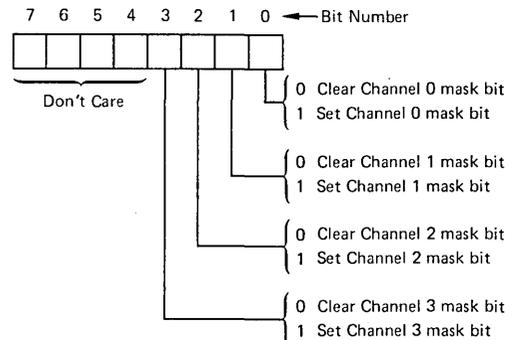
**Status Register:** The Status registers may be read out of the Am9517A by the microprocessor. It indicates which channels have reached a terminal count and which channels have pending DMA requests. Bits 0-3 are set each time a TC is reached by that channel, including after each Autoinitialization. These bits are cleared by Reset and each Status Read. Bits 4-7 are set whenever their corresponding channel is requesting service.
