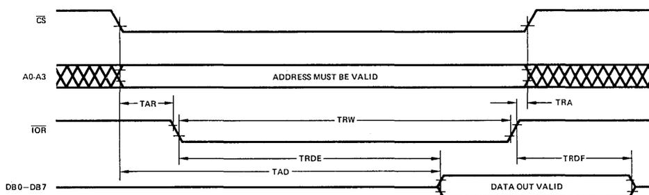
Timing Diagram 2. Program Condition Read Cycle (Note 9).
