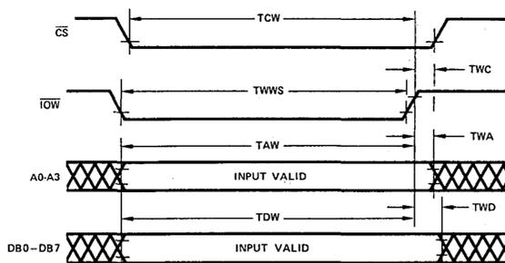
Timing Diagram 1. Program Condition Write Timing (Note 9).
