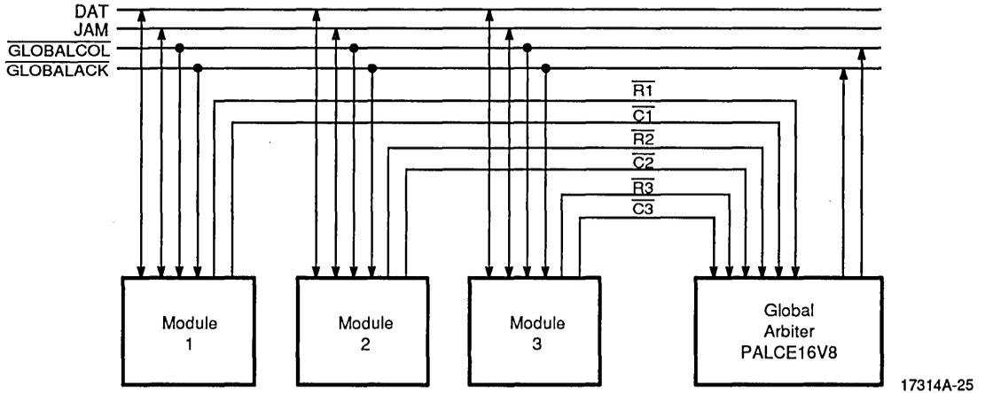
**Figure 5-10 Repeater Module with Three IMR+ Devices**
