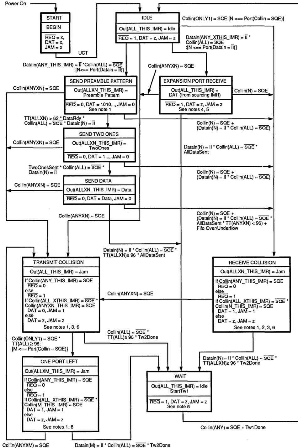
Referring to Figure 3-8, the upper box in each block contains the name of the state. The center box refers to the output at the AUI and TP ports. The lower box describes the state of the  $\overline{\text{REQ}}$ , DAT, and JAM output pins for the IMR+ device with this state machine embedded.
