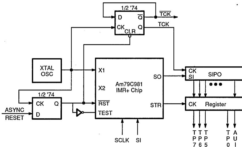
In this configuration, the IMR+ device will continuously output one of four status conditions on the SO pin, dependent on the programming of the TEST and SI pins. The programming of SI and TEST allows any one of the following status indications to be reported on SO:
