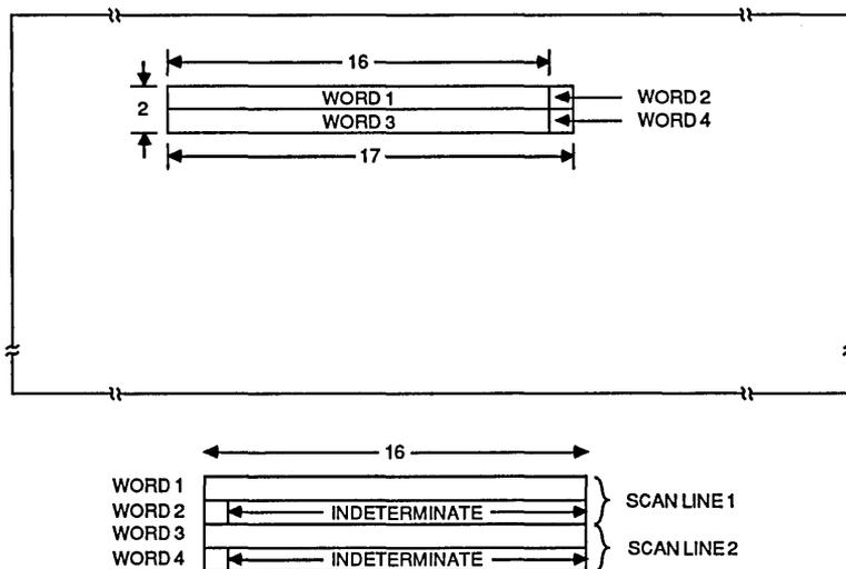
Figure 14-14 Output Block by Plane
