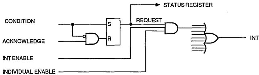
Figure 3-2 Interrupt Logic
