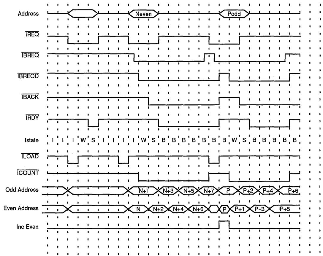
Interleaved Instruction Access: Simple, Burst (even1\*), Terminate, Burst (add 1\*), Suspend 10623C-017
