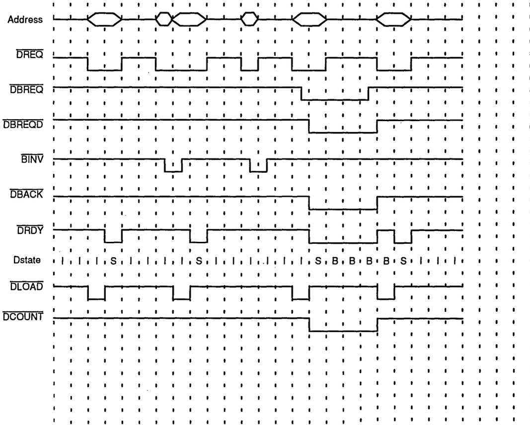
Simple and Burst Data Access, including  $\overline{\text{BINV}}$
