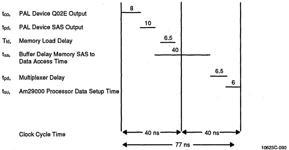
**Figure 9-19 VDRAM Instruction Burst Timing**
