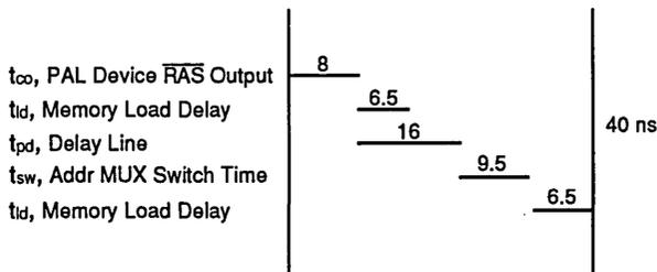
**Figure 7-22 SCDRAM Interleaved Bank Memory Burst Access**
