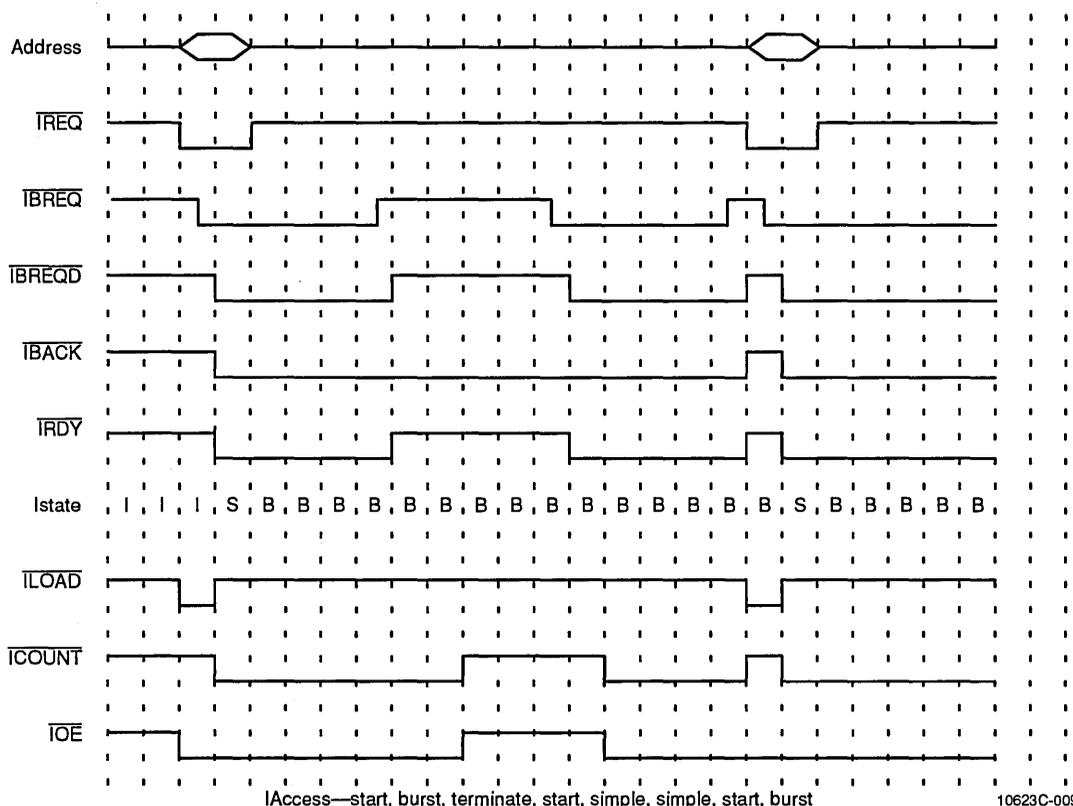
$$\text{Instruction Load (ILD)} = (\text{idle} \bullet \text{IMA}) + (\text{Iburst} \bullet \text{IMA})$$
