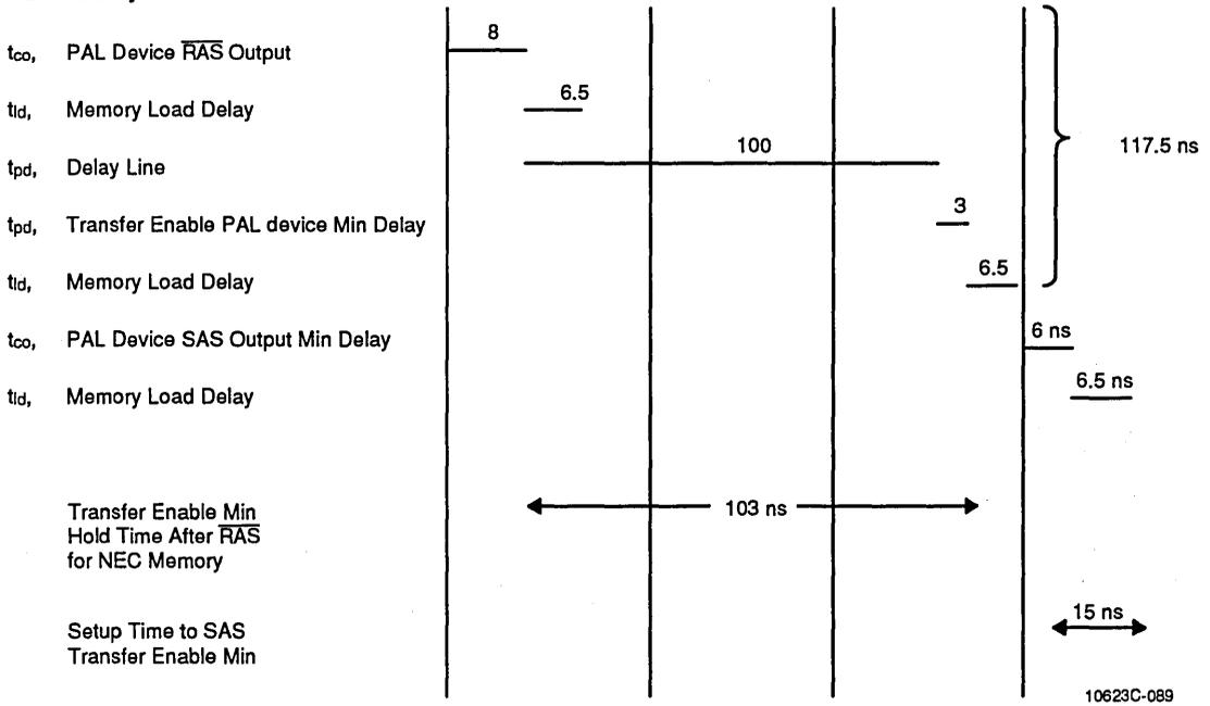
**Figure 9-18 Burst Access Timing**
