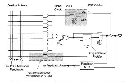
The eight product terms of the programmable-AND array feed the 8-input OR gate, which then feeds one input to an XOR gate. The other input to the XOR gate is connected to a programmable bit that allows the array output to be inverted. Altera's MAX+PLUS II software uses the XOR gate to implement active-high or active-low logic, or uses De Morgan's inversion to reduce the number of product terms to implement a function.
