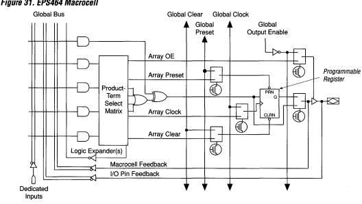
Combinatorial logic is implemented in the product-term array, which consists of five product terms. Four product terms feed the product-term select matrix; the fifth feeds one input of an XOR gate, making it possible to implement active-high or active-low logic. The XOR gate is also used to build complex arithmetic logic functions and to perform De Morgan's
