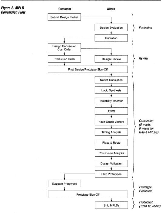
After the customer submits an order for the Design Conversion Cost (DCC), an Altera engineer reviews the design and submits a *Final Design Sign-Off Form* for customer approval. This form describes the specifications of the MPLD in detail. After the final design has been signed off, Altera begins the design conversion.
