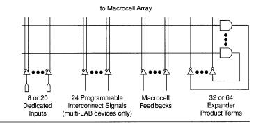
Expanders are fed by all signals in the LAB. One expander can feed all macrocells in the LAB or multiple product terms in the same macrocell. Since expanders also feed the secondary product terms of each macrocell, complex logic functions can be implemented without using additional macrocells. Expanders can also be cross-coupled to build additional flipflops, latches, or input registers. A small delay (**t**<sub>SEXP</sub>) is incurred when shared expanders are used.
