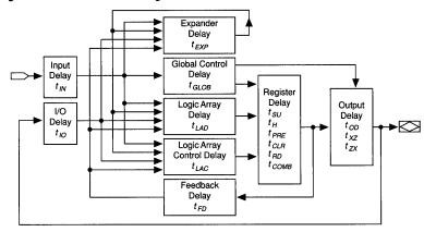
Figure 4. EPS464 EPLD Timing Model
