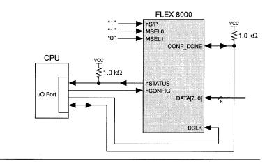
Figure 8. Passive Parallel Synchronous Device Configuration
