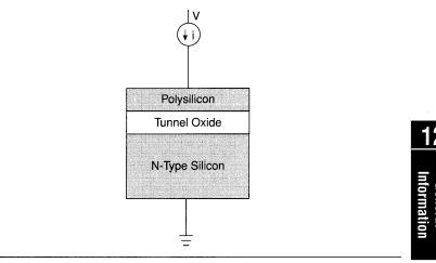
Figure 5. EEPROM Floating-Gate Electrode, Tunnel Oxide & Heavily Doped Diffusion Electrode
