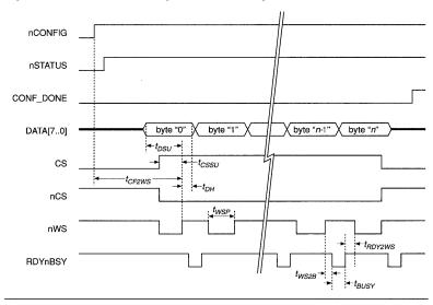
The CPU must poll the RDYnBUSY signal to establish when the FLEX 8000 device is ready to receive more data. RDYnBUSY falls immediately after the rising edge of the DCLK signal that latches data, indicating that the device is busy. While the FLEX 8000 device processes the data byte, RDYnBUSY remains low. On the eighth falling edge of DCLK, RDYnBUSY returns to V<sub>CC</sub>, indicating that another byte of data can be latched. Table 6 shows the timing parameters associated with PPA configuration.
