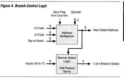
The address multiplexer provides the next-state address to the microcode memory. The next-state address can come from the Q-field, the D-field, or the top-of-stack. The selection is based on the instruction in the pipeline register and the condition of the zero flag from the counter.
