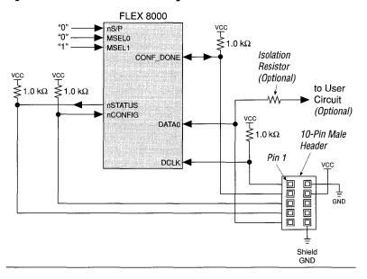
Figure 14. Passive Serial Device Configuration with the FLEX Download Cable
