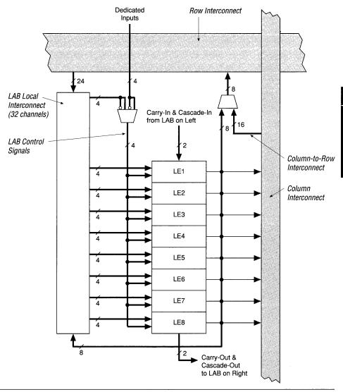
Data signals enter the LAB local interconnect from either the row interconnect or the dedicated inputs. The outputs of all eight LEs are also driven back into the LAB local interconnect via local feedback lines. Each LE in the LAB can drive signals out to the rest of the device via both row and column interconnect paths.
