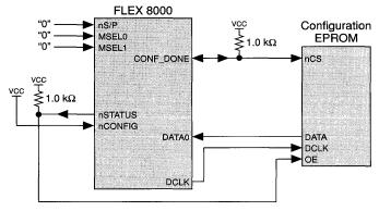
The Altera serial Configuration EPROMs are designed for performance that is compatible with the setup and hold time requirements of FLEX 8000 devices. Refer to the *Configuration EPROMs for FLEX 8000 Devices Data Sheet* in this data book for complete details on timing and circuitry. Details on device programming are given in "Programming a Serial Configuration EPROM" later in this application note.
