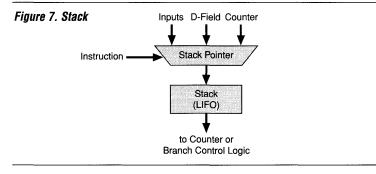
The pushing or popping of the stack occurs on the leading edge of the Clock. The stack is "zero-filled" so that a pop from an empty stack resets all 8 bits to zero. On the other hand, a push to a full stack writes over the top-of-stack, leaving the other 14 values unchanged.
