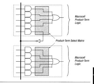
Parallel expanders are unused product terms from macrocells that can be allocated to a neighboring macrocell to implement fast, complex logic functions. With parallel expanders, up to 20 product terms can directly feed the macrocell OR logic—5 product terms provided by the macrocell and 15 parallel expanders provided by neighboring macrocells in the LAB.
