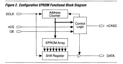
The control signals for Configuration EPROMs (DCLK, nCS, OE) interface directly to the FLEX 8000 device control signals. A FLEX 8000 device can control the entire configuration process by retrieving the configuration data from the Configuration EPROM without an external intelligent controller. Configuration usually occurs automatically at system power-up.
