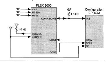
Figure 3. Active Serial Configuration
