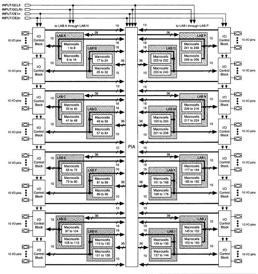
Figure 35. EPM7256 Block Diagram
