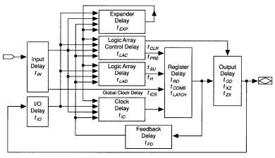
Figure 2. Single-LAB MAX 5000 EPLD Timing Model
