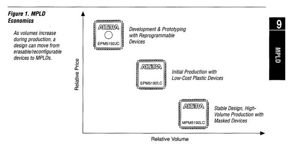
Altera handles the programmable logic device-to-MPLD conversion so that no redesign effort is required. Altera guarantees that the MPLD meets the worst-case AC and DC parameters of the original Altera programmable logic device. In addition, Altera automatically generates test vectors with 98% fault coverage.
