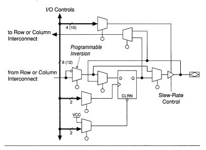
I/O pins can be used as input, output, or bidirectional pins. Each I/O pin has a register that can be used either as an input register for external data that requires fast setup times, or as an output register for data that requires fast Clock-to-output performance. The MAX+PLUS II Compiler uses the programmable inversion option to automatically invert signals from the row and column interconnect when appropriate.
