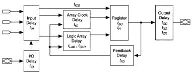
If the register is bypassed, the delay between the logic array and the output buffer is zero.
