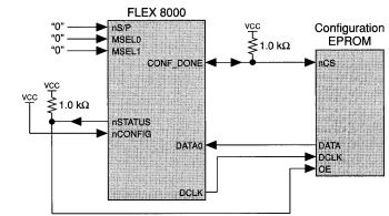
Figure 5. Active Serial Device Configuration with Automatic Reconfiguration on Error
