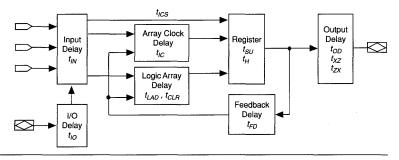
Timing information can be derived from the timing model and parameters for a particular EPLD. External timing parameters can be calculated from the sum of internal parameters and represent pin-to-pin timing delays. Figure 5 shows the internal timing relationship for internal and external delay parameters. For more information on EPLD timing, refer to *Application Brief* 100 (Understanding EPLD Timing) in this data book.
