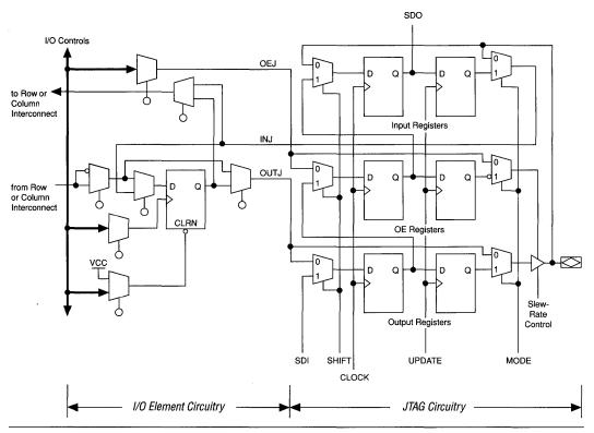
The JTAG BST registers shown in Figure 10 also exist for dedicated input and configuration pins in FLEX 8000 devices. However, only some of these pins provide output and Output Enable signals.
