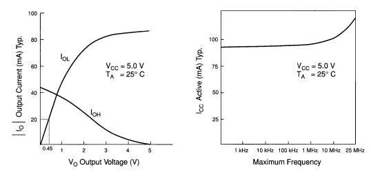
Figure 12. EPS448 Output Drive Characteristics and I<sub>CC</sub> vs. Frequency
