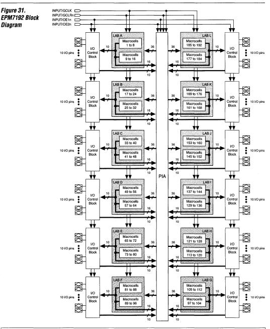
The high density and high I/O pin count make the EPM7192 appropriate for prototyping gate arrays. The EPM7192 can accommodate both logicand I/O-intensive designs.
