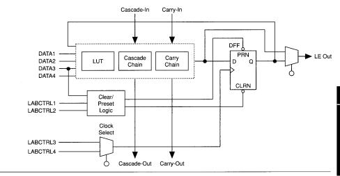
The LUT is a function generator that can compute any function of four variables. The programmable flipflop in the LE can be configured to emulate D, T, JK, or SR operation. The Clock, Clear, and Preset control signals on the flipflop can be driven by dedicated input pins, general-purpose I/O pins, or any internal logic. For purely combinatorial functions, the flipflop is bypassed and the output of the LUT goes directly to the output of the LE.
