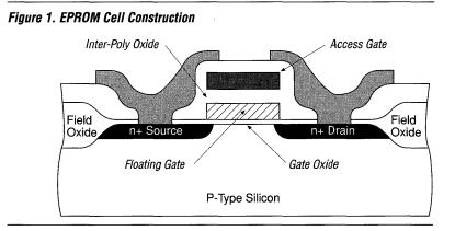
EPROM transistors are programmed to a high-threshold voltage with hot electron injection. When a programming voltage  $V_{PP}$  (normally 12.5 V) is applied to the access gate of an EPROM cell and a slightly lower voltage is applied to its drain, electrons flow from the source to the drain. As these electrons pick up kinetic energy, their path is altered by an electric field located between the access gate and substrate. This electric field is generated
