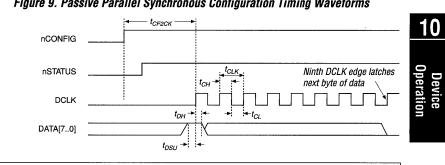
Figure 9. Passive Parallel Synchronous Configuration Timing Waveforms
