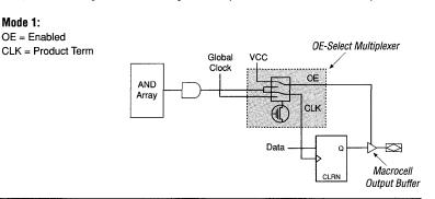
individually configured for each macrocell. In Mode 0, the tri-state output buffer is controlled by a single product term. If the output of the AND gate is high, the output buffer is enabled. If the output is low, the output buffer has a high-impedance value. In this mode, the macrocell flipflop is clocked by its global Clock input signal. (The EP330 supports only Mode 0.)
