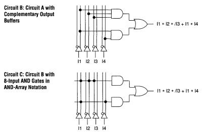
Figure 6. AND-Array Notation (Part 2 of 2)
