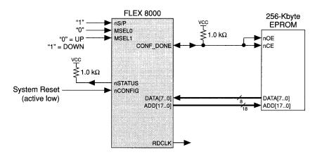
Figure 5 shows the timing associated with the circuit in Figure 4. The highlow-high pulse on the nCONFIG pin starts the configuration process. The nSTATUS pin is pulled low for up to 100 ms, and the CONF\_DONE pin is pulled down to GND. Once the CONF\_DONE pin is low, address generation begins. The low logic level on the CONF\_DONE pin also enables the output of the EPROM. In an APU configuration scheme, the first address generated is 00000H; in an APD configuration scheme, it is 3FFFFH.
