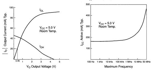
Figure 24. EPM5130 Maximum Output Drive Characteristics & I<sub>CC</sub> vs. Frequency
