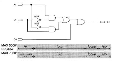
S1 is the output of macrocell 21 (\_LC021), which contains combinatorial logic. The combinatorial logic LCELL (\_EQ026 \$ C0) represents the XOR of the intermediate equation \_EQ026 and the carry-in C0. In turn, \_EQ026 is logically equivalent to the XOR of inputs B1 and A1. Therefore:
