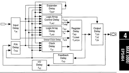
Timing information can be derived from the timing model and parameters for a particular EPLD. External timing parameters are calculated with the sum of internal parameters and represent pin-to-pin timing delays. Figure 6 shows the internal timing relationship for internal and external delay parameters. For more information on EPLD timing, refer to *Application Brief* 100 (*Understanding EPLD Timing*) in this data book.
