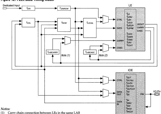
Figure 12. FLEX 8000 Timing Model
