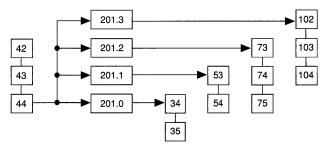
Any of the 13 available commands can be enhanced with multiway branching. For example, location 44 in Figure 10 can be a CALL to a subroutine, and address 201 can contain the starting instruction for 4 unique subroutines. The routine that is actually executed depends on the user-defined condition of the inputs. The following ASM code can be used to implement this example:
