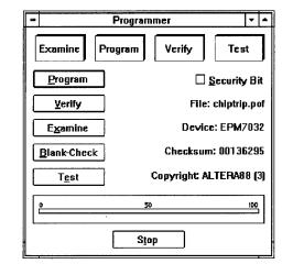
supports functional testing, so that vectors created for simulation can be applied to a programmed device to verify its functionality.
