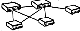
Mixture of Masters and Subs up to an overall total of 10 stations. Masters can call; Subs can only answer.
