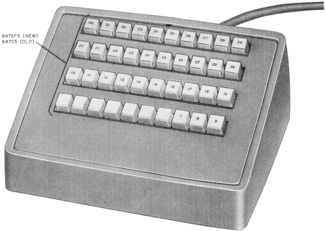
Fig. 10—7B1 Selector Console (MW)
