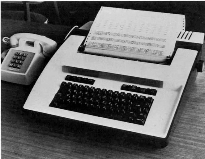
Figure 11-8. The 43 teleprinter.
